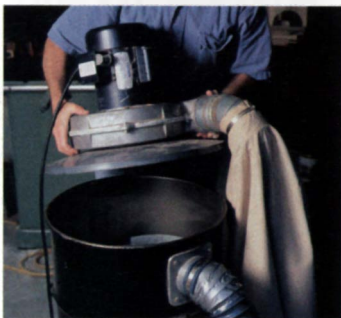
The lid can be heavy with this kind of two-stage collector. One option would be to install a block and tackle nearby with a wall cleat to tie off the rope.
