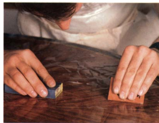
Use a rubber squeegee to clear slurry. The 1,200-grit paper works slowly, so keep rubbing and clearing the slurry until all the high spots are gone.
