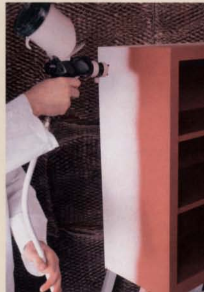
5 Do the exterior cabinet sides and front corners.
