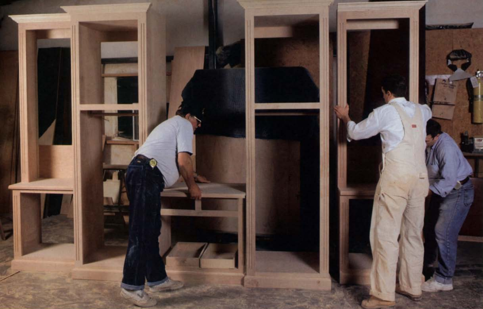
MDF-core birch cases with alder faces —From left to right, Ron Barzyk, his son Brook and Floyd Parker of Madison, Tenn., dry-fit wall-unit cases. Barzyk prefers MDF core over any other.
