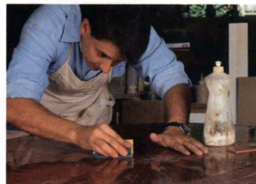
Rub out nubs or bumps with 1,200-grit paper wrapped around a wooden block (above). Water, naphtha or mineral spirits may be used to lubricate the surface.
