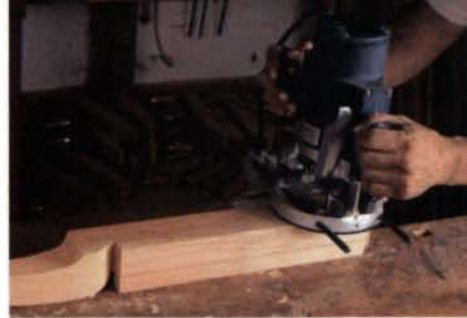
A plunge router with a spiral bit roughs out the mortises. The full stock width of the blank provides support for the router.
