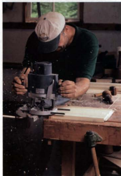
Cutting tenons by the batch saves time. Clamping the runners and kickers together also makes it easier to keep tenons uniform.
