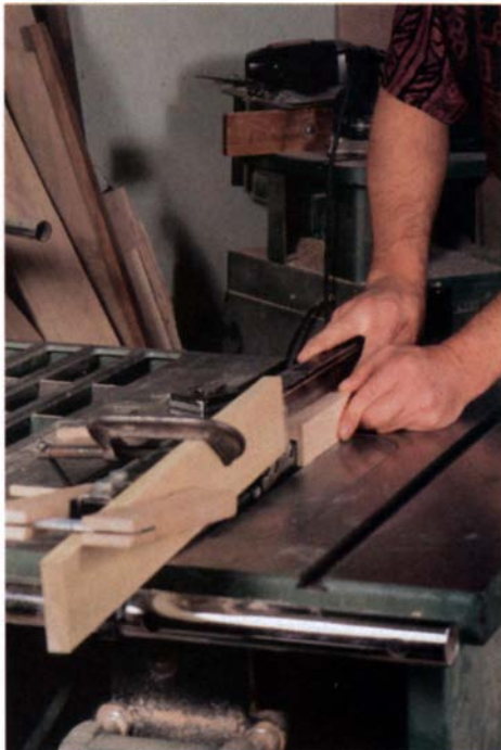
A stopped block clamped above the dado cutter controls the cam-slot length.
