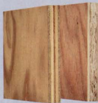
Fiber-Ply (left) and Multi-Core are strong and less expensive than standard veneer-core plywood.
