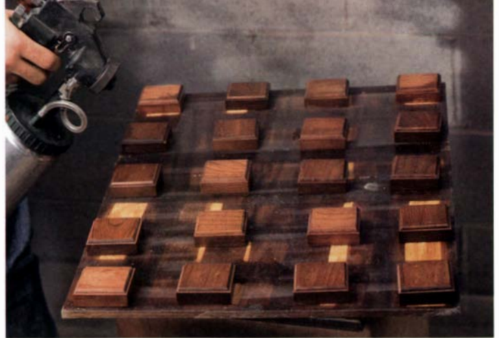
Turntable for even, quick coats —After arranging trophy bases on a lazy Susan, the author sprays with an HVLP gun.
