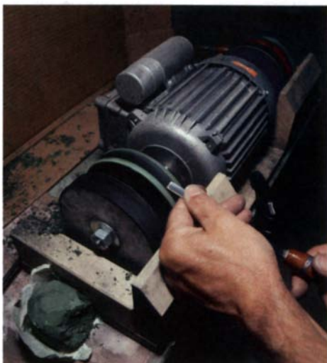
A razor-sharp edge in three seconds. The Koch system uses a proprietary honing paste and special buffing wheels.
