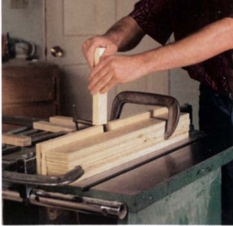
A simple jig makes plunge cutting the bar kerfs fast and safe.
