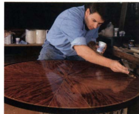
Brush out the varnish at 90° to the direction you laid it on (above), usually with the grain. Use a light touch. Just skim across the surface without exerting any downward pressure.
