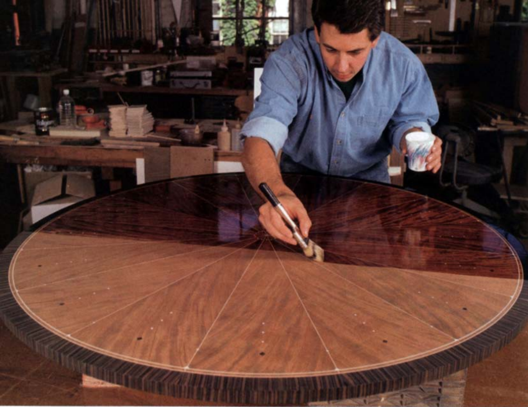
Brush on the varnish in long, smooth strokes (left). On a surface with a single or a predominant grain direction (unlike this sunburst veneer pattern), start by applying the finish across the grain. The first coat of varnish should be a 50/50 solution of varnish and solvent.
