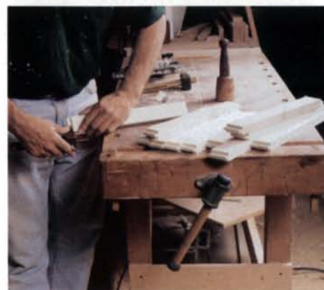
Mark the shoulder line on the narrow edge of each tenon. Cut the waste away on the bandsaw.
