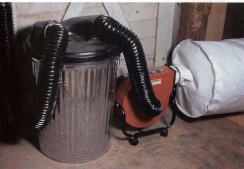
A built-in cyclone does an excellent job separating chips and dust before they reach the blower. This Delta 50-903 collector has a 5-hp motor.
