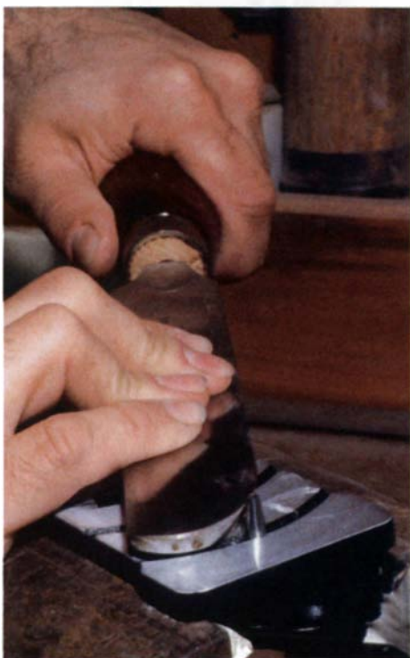
Raising a burr by burnishing gives turning scrapers a uniform edge.
