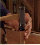
Hammer the hoop squarely on the handle using a slightly larger hoop as a driving ring.
