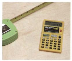
The InchMate+ makes working with fractions easy. It also calculates rise, run, diagonal and slope for triangles.
