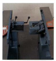
Two types of center-mounted fences—Both the Reliant (left) and Enlon jointers have centermounted fences. Enlon's fence is fixed by three points, so it's stable. Reliant's fence, fixed by a sliding dovetail, isn't easy to position and can't be set acutely.
