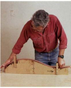
Test a ply by bending it over the form. If the ply bends easily, the thickness is correct.
