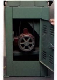
Look in the cabinet to inspect motor mounts and belt tensioning. The General is compact, and belt-tightening is simple because of a pivoting motor base. The motor comes with rubber isolation bushings and a big, balanced pulley.
