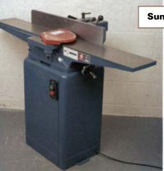
Comments: Fence comes unassembled. It was difficult to set its positive stop to 90°. Fence works okay after tweaking. Bolt-on extension wings add 7 in. to table length.
