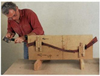
**Separate the form.** Sometimes a rap with a well-placed chisel and mallet is needed to free the cured part.
