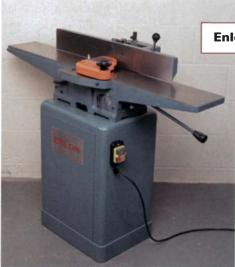
Comments: Excessive protective coating. Machined surfaces are highly polished. Nylon pads prevent the fence from scratching the table. Jointed very smoothly.
