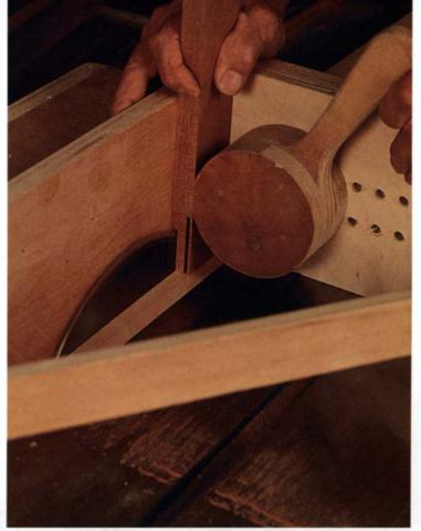
Cheek cuts for the tenon—To test the tenon setup, cut the cheeks first. The height of the sawblade off the table does not change. One pass per side is sufficient.
