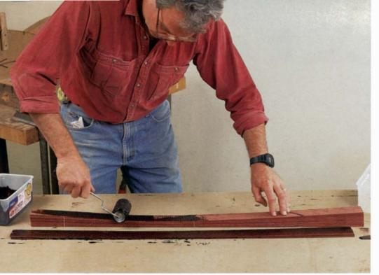
A stippled roller helps spread the glue with speed and consistency. Apply glue to all but the two faces that will contact the form.
