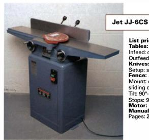
Comments: Fence is difficult to adjust and use. Fence stops don't always repeat exact tilt settings. The table height-adjustment cranks are easy to get to (on front).
