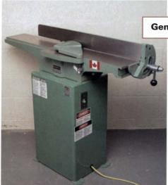
Comments: Best fit and finish. Quietest of all machines. Blade guard for back side of fence is optional. Compact footprint. Long power cord but only 16-gauge wire.
