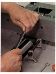
Installing knives—A couple of jointers come with knife-setting jigs, which gauge knife height above the cutterhead. Here, the author installs a knife in the Grizzly jointer's cutterhead, which has spring-loaded slots.
