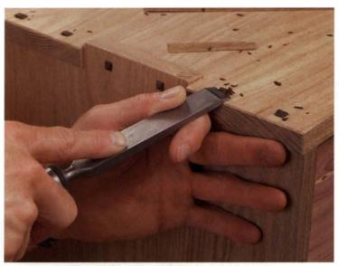
Plugs are easy to chamfer. Chamfering all 40 plugs took less than an hour. Plastic laminate protects the chest when the author levers his chisel to pare the inner faces of the plugs.
