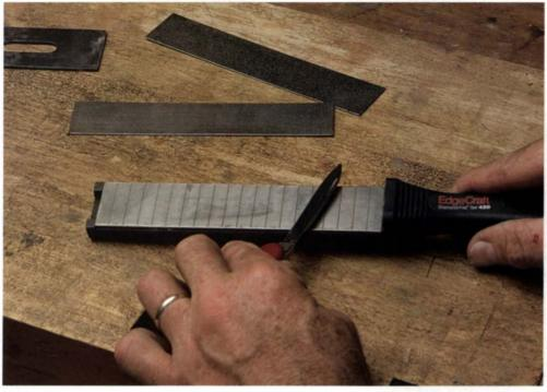
Edgecraft diamond file cuts quickly and doesn't require lubrication.
