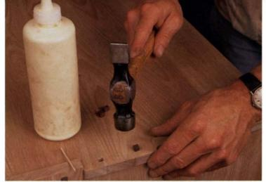
Slightly tapered plugs seat easily. Wenge plugs are cut to length, planed to fit and then tapered so that they'll enter the squared screw holes easily. A dot of glue holds them in place.
