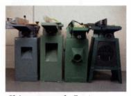
Chip removal: Designs vary widely and include (from left) open dust chutes on the Enlon and General machines, a dust-collection hose adapter on the Wood-Tek jointer and no chute at all on the outfeed end of the Bridgewood machine.
