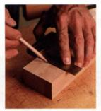
Mark the shoulder line. All pieces cut by hand must be marked on every side and end.
