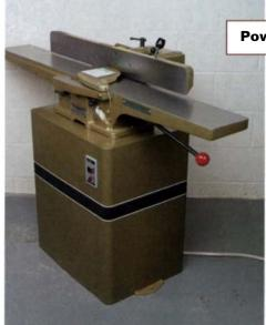
Comments: Large stable base and the longest tables. Castings are heavy. No power cord supplied. Small on/off switch. Machine is loud. Awkward belt tensioning.
