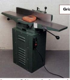
Comments: Bolting together the stampedsteel stand and wiring switch takes longer than setting up other machines. Bracket prevents fence from tilting to full 135°.
