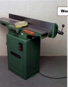
Comments: Only machine with pick-up boot for dust-collection hose. Includes guard for back side of fence. Fence stops require trial-and-error bolt turning.
