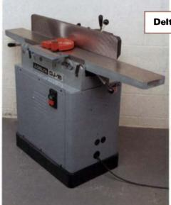
Comments: Guard has stiff spring and blunt front face, making stock feed difficult. Nice depth-of-cut gauge. Replaceable table inserts around cutterhead.
