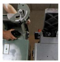
Hand cranks are better. The author prefers a hand crank (left) over a lever for adjusting table beds because hand cranks make precise adjustments easier. The fence on the General jointer (left) is mounted at the end of the infeed table.
