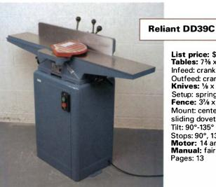
Comments: Fence is difficult to adjust, set and use. Stand and castings are virtually identical to Jet and Sunhill jointers but Reliant has a slightly different fence mount.
