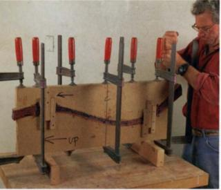
Use plenty of clamps, and space them so the plies are compressed against the form. To avoid springback, keep the clamps on the form until the glue has completely cured.
