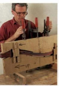
Start clamping in the center, and work out to prevent bubbles between plies.
