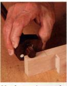
Mark mortises and tenons at the same setting. Fill in the scribed lines with pencil marks, so the lines are easier to read.
