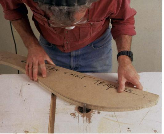
Making a pattern saves time. Identical layers of form stock are made by pattern routing with a flush-trimming bit.
