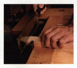
Cut the shoulders with a dovetail saw. For well-fitting joints, make sure that you cut to the same line on all the pieces.
