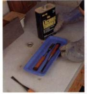
Remove the factory coating from blade and handle. Soak new chisels in lacquer thinner.
