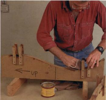
Wax forms thoroughly, especially around the keys, so they don't stick together. Forms should get two coats of finish first.
