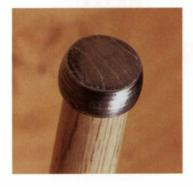
Carefully mushroom the end—Using a household iron, the author steams the handle butt. With glancing hammer blows, he peens the end as he rotates the chisel.
