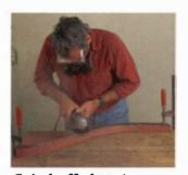
Grind off glue. A coarsegrit sanding disc and minigrinder quickly remove squeeze-out once the glue has dried.
