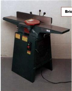
Comments: Fence is difficult to adjust and won't tilt to stops. Stamped-steel stand lengthens setup time. Fence bowed .021 in. over its length. No dust chute.
