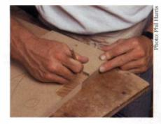
Bandsaw takes out most of the waste. The author removes all but the last ½16 in. of waste between the fingers.
