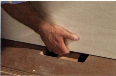
Stored sheets are easier to lift —When the author has to carry a full sheet (top), he lifts it upright to keep his back straight. A cutout gives his hand clearance to grab the sheet's lower edge.
