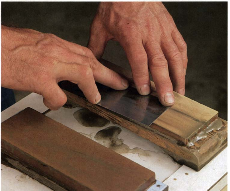
Hone the faces to remove the burr left from filing or honing. Start with a medium stone, and work up to your finish stone. Spread pressure evenly over the scraper.
