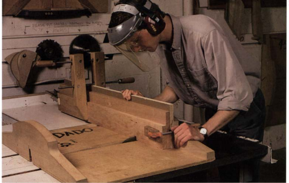
Mortises on the table saw —The tabletop mortises are cut with a dado blade and a cross-cut sled. Mating boards are clamped face to face against the sled's fence.
