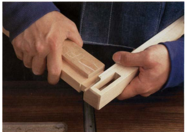
Set correctly, the fixture will yield tight joints, whether the tenons are straight, angled or compound-angled. Here, the author tests the fit of a seat-rail tenon into a leg mortise.
