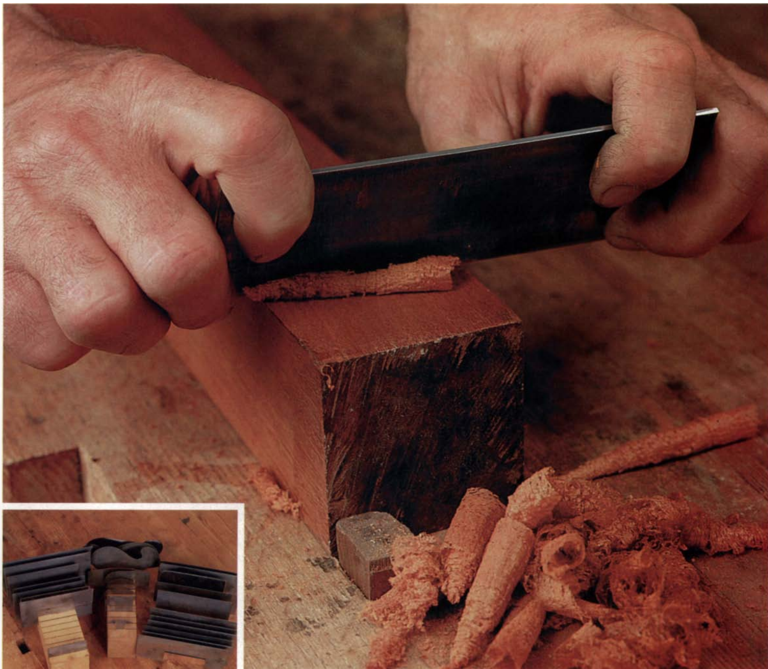
Shavings, not dust. A well-prepared scraper works like a plane, cutting shavings and leaving a gleaming surface in its wake. Scrapers are available in different profiles and thicknesses.
