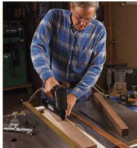
Making jigs, like the one the author is putting together, to taper a leg.
