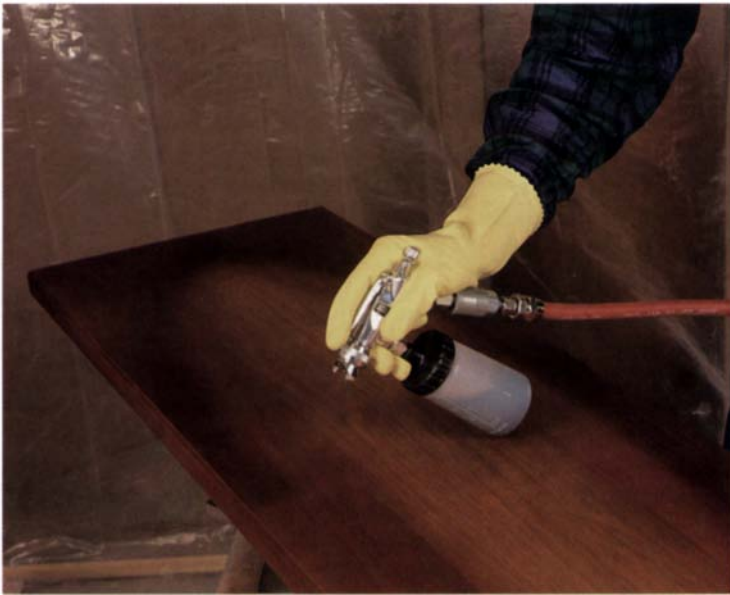
Dyes are great for special color effects. After building a case for his son's electric guitar, the author custom-finishes the lid. Successive bands of color create a sunburst effect.
