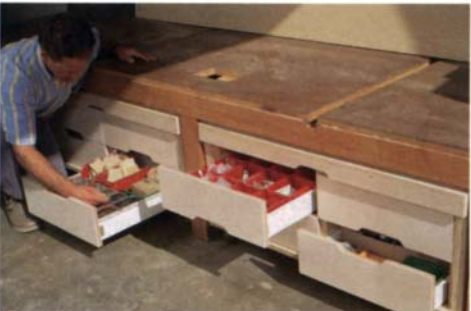
Drawers make use of floor space —A two-part assembly table rolls under the platform when not in use. Aligned by biscuits and clamped together, the table has slide-out bins in back (bottom).
