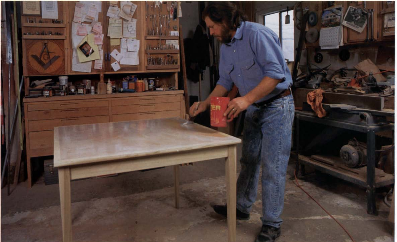
Two coats of glue on both surfaces. The author uses a brush to spread thinned glue on the top of this game table.
