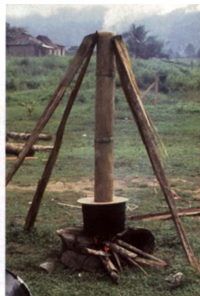
Necessity is the mother of this steambox. A makeshift bamboo steamer (right) built by Curtis Buchanan and his students may be unorthodox, but it was perfect for bending chair legs. Before steaming, parts are split from logs (left).
