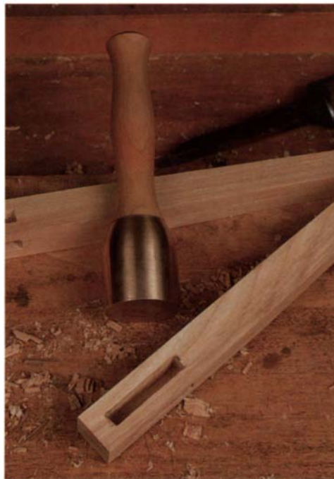
Bronze joiner's mallet is a pleasure to use. This mallet, with its heavy bronze head, is more efficient and requires less effort to use than wooden mallets.
