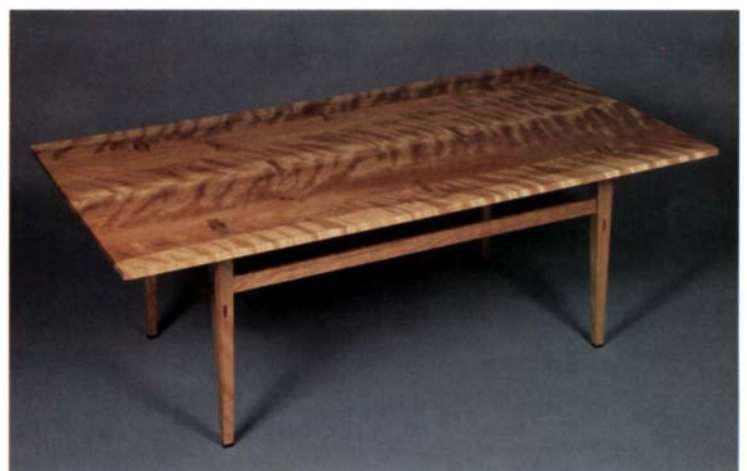
A low coffee table makes the most of wildly figured wood. Mortises are cut in the top before glue-up.
