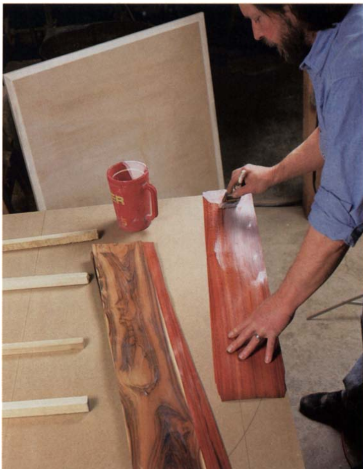
Thin the glue, and paint it on. Aliphatic resin glue thinned about 10% with water spreads easily with a brush, eliminating the bubbles that can occur with a roller.
