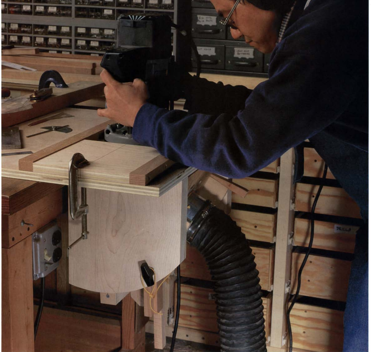
Guide frame determines thickness and width of tenons. The author keeps the router's base against the inner edges of the guide frame and routs clockwise to prevent tearout. Guide frames can produce round-cornered or square-cornered tenons.
