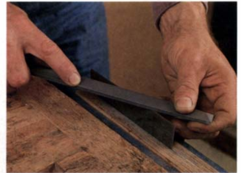
File the edge flat and square. To avoid a belly on the edge, take two or three strokes at each end first. Then file the full length of the scraper. Follow with light passes with a smooth-cut mill file.
