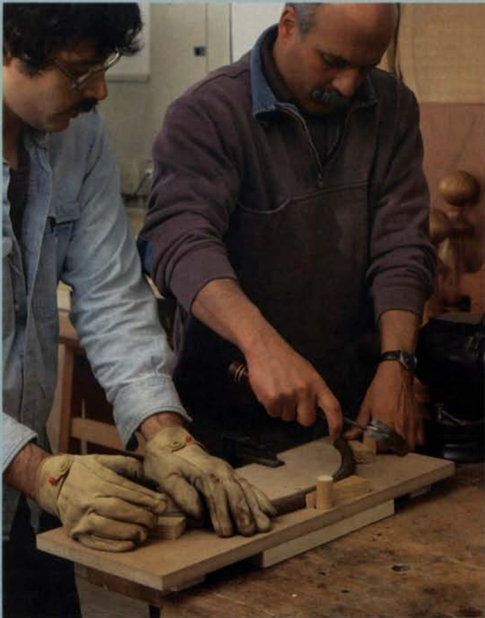
Rail-bending jig. Four hands are better than two for forcing the steamed rail into shape. The author is assisted by Les Katz, one of his students. Wedges hammered between the plywood form and the wooden pegs hold the rail tightly in place.
