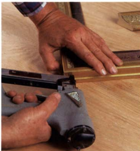
Pinning together mitered frames and other delicate assemblies.
