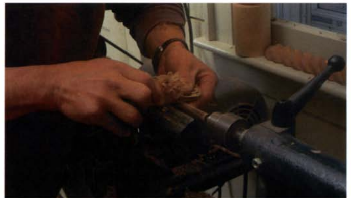
Rough out the spindles with a gouge, and clean them up with a block plane. Cut the tenons with a parting tool.
