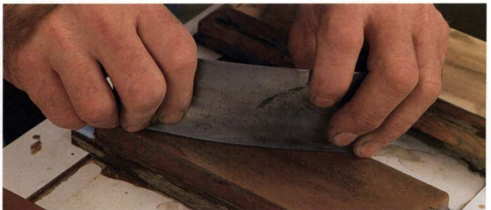
Hone the edge. Hold the scraper perpendicular to the stone and slightly flexed. Apply pressure, and move the scraper back and forth in line with the stone. For waterstones, take the edge to 6,000-grit or higher; for oilstones, finish up with a hard Arkansas.
