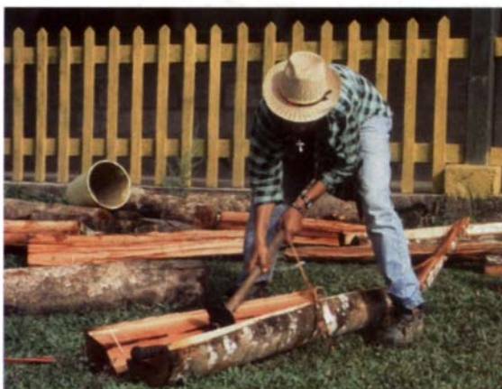
Necessity is the mother of this steambox. A makeshift bamboo steamer (right) built by Curtis Buchanan and his students may be unorthodox, but it was perfect for bending chair legs. Before steaming, parts are split from logs (left).
