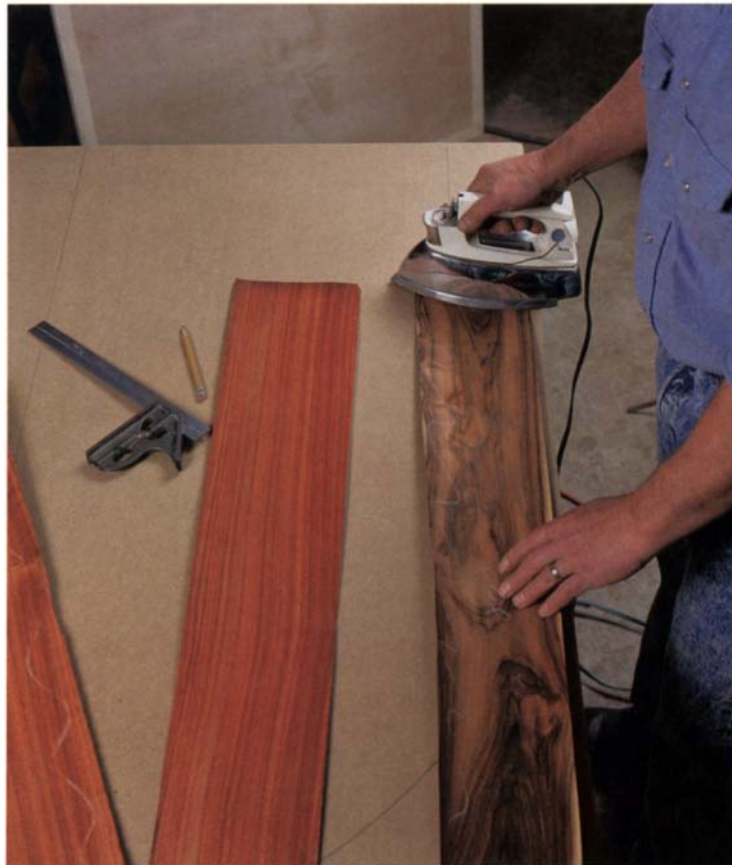
Getting the shrink out. Because some veneers shrink dramatically during the bonding process, the author starts by pre-shrinking all the veneer with the iron at a three-quarter setting.
