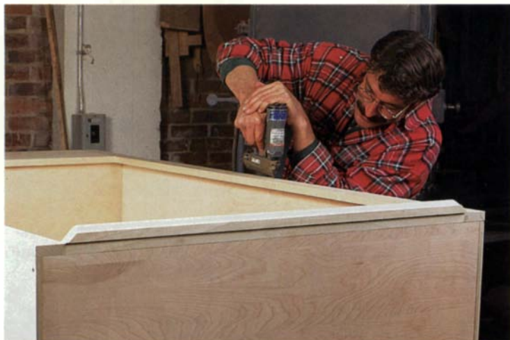
Installing face frames, cabinet backs and drawer bottoms.
