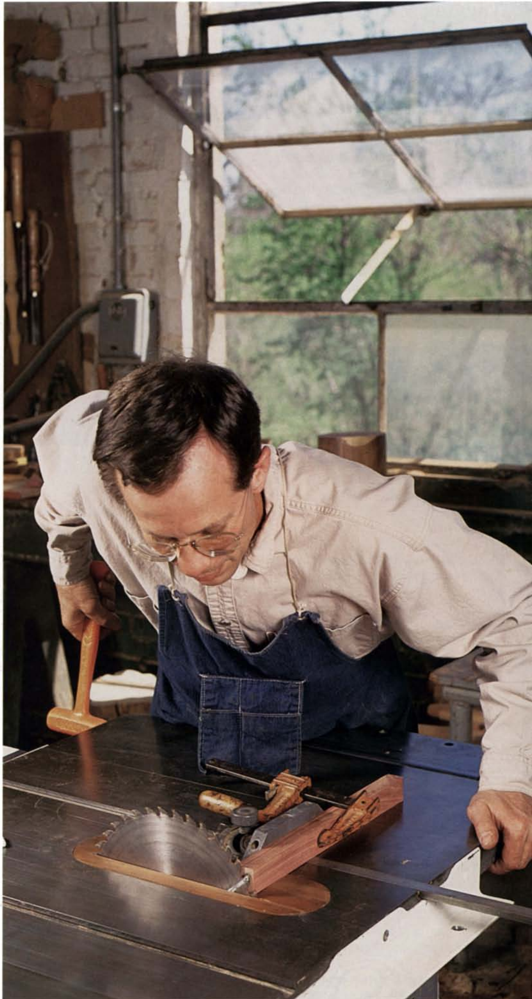
Tap the edge of the table to nudge the miter-gauge slot parallel to the blade.
