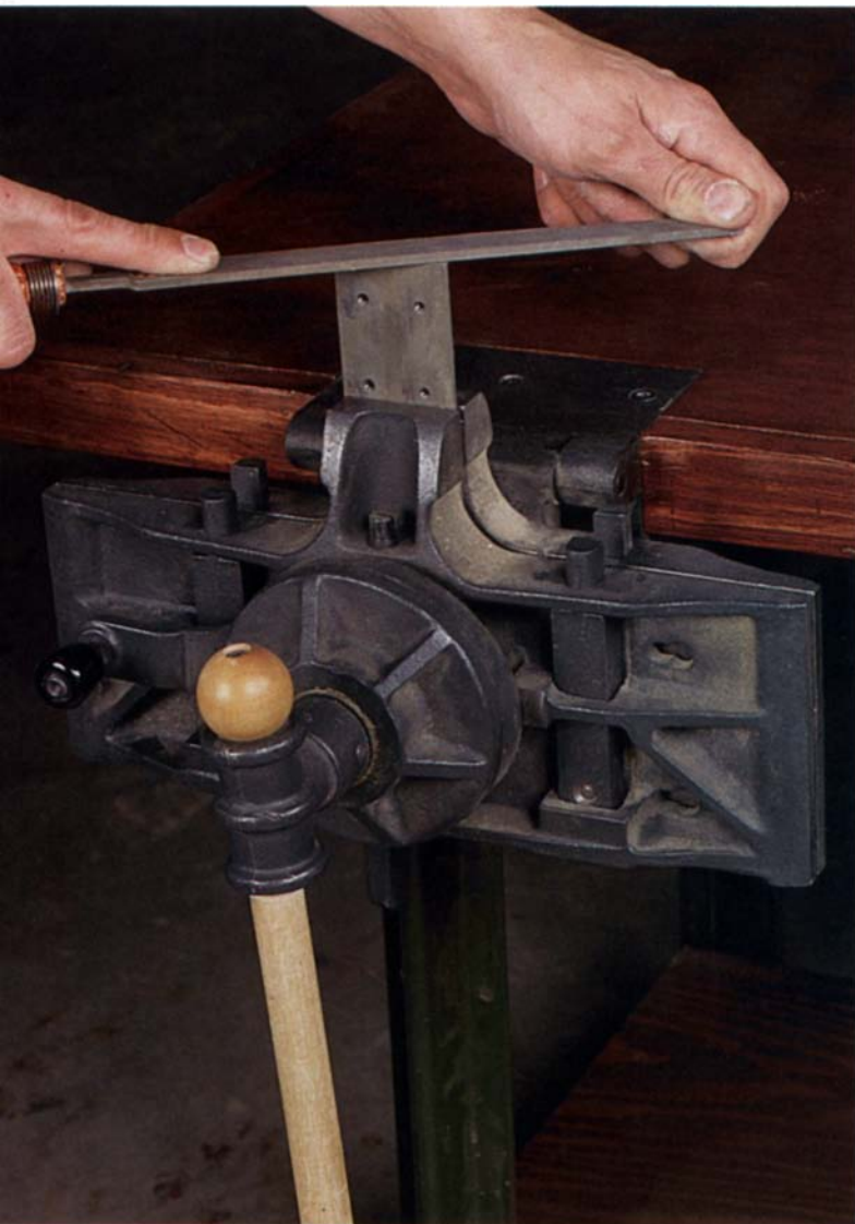
Vise handles metal, too. Rotate this American Machine & Tool Co. vise 180°, and you'll have a pair of jaws for metalworking (above). A set of jaw inserts, which are lined with soft rubber (right), prevents dings in soft material.
