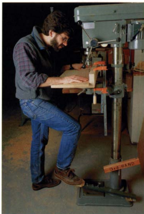
Foot-feed frees your hands. With both hands free for the workpiece, you can work faster and more accurately.
