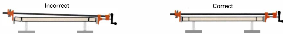
Fig. 1: Clamping a frame. Clamps should be applied parallel to the rails to keep the frame flat.
