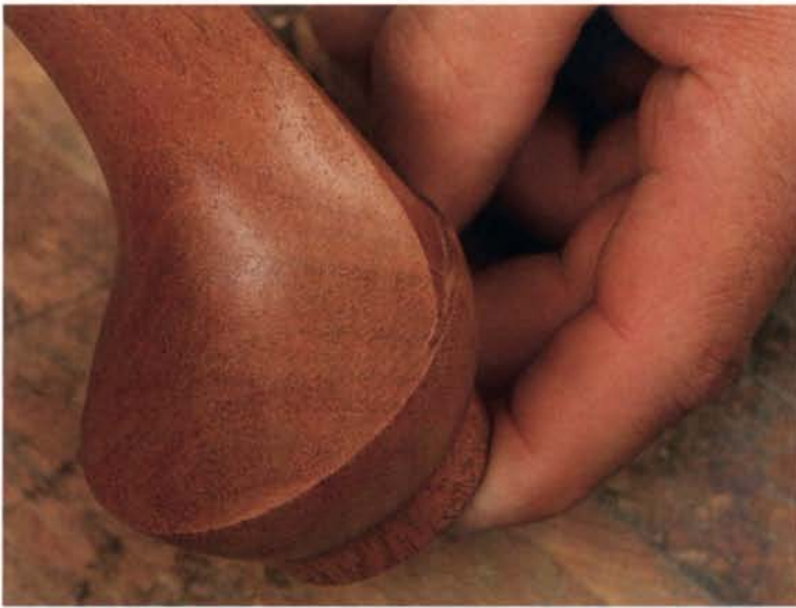
Filed, not sanded. The author put a coat of shellac on this cabriole leg after shaping it with a file, but without sanding it. Only minor tool marks are still visible.
