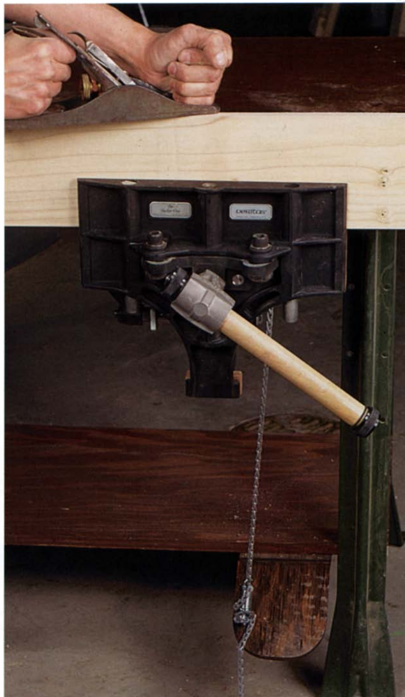
Modern version uses alloy casting. Made by Veritas Tools, this Tucker vise uses a zinc-aluminum alloy instead of cast iron, making it strong and light. A quick-release feature can be operated by a foot pedal (above). The vise's cork-lined jaws protect delicate workpieces (left).
