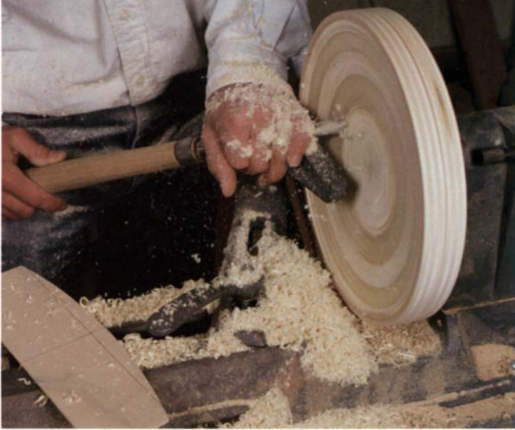
The baseplate is turned from plywood. A template on a lathe bed helps the author shape a camber in the baseplate (colored yellow in the drawing on the facing page).
