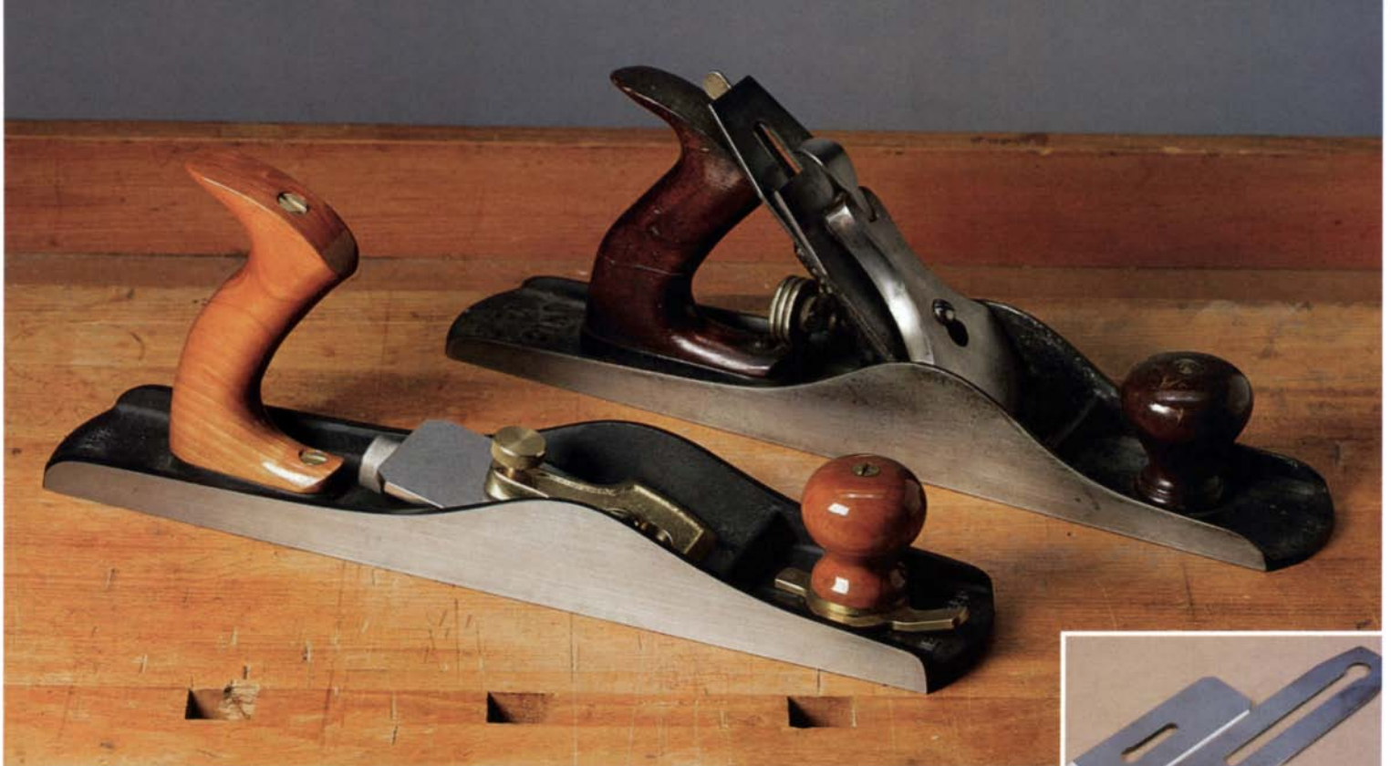
These planes are cousins, not twins. A Union No. 5 plane (rear) and a low-angle jack plane from Lie-Nielsen show similarities but big differences, too. The Lie-Nielsen delivers high performance at a high price. The Lie-Nielsen blade (see inset photo) is thicker than the Union's.
