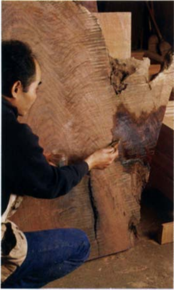
Bringing out the figure—Ed Koda wets claro walnut with mineral spirits to see how it will appear when finished.
