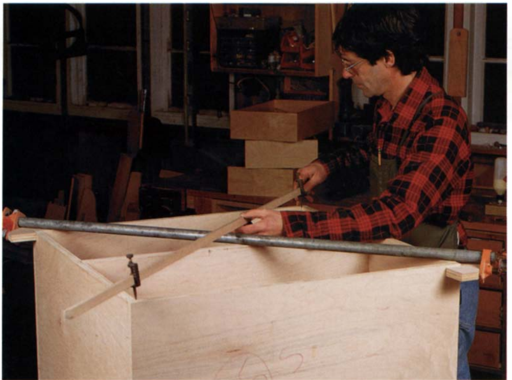
Trammel points and bar work to check square on carcasses, too. The author uses a clamp across the longer diagonal to draw the case to square.
