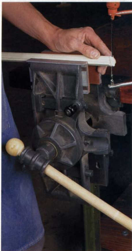
Vise handles metal, too. Rotate this American Machine & Tool Co. vise 180°, and you'll have a pair of jaws for metalworking (above). A set of jaw inserts, which are lined with soft rubber (right), prevents dings in soft material.
