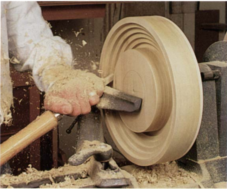
A series of steps in the jaw plate of the compression chuck accommodate a range of bowl sizes (the jaw plate is red in the drawing on the facing page).
