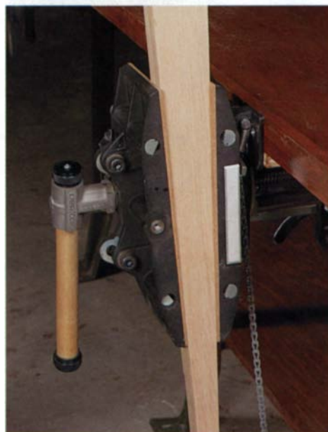
Modern version uses alloy casting. Made by Veritas Tools, this Tucker vise uses a zinc-aluminum alloy instead of cast iron, making it strong and light. A quick-release feature can be operated by a foot pedal (above). The vise's cork-lined jaws protect delicate workpieces (left).
