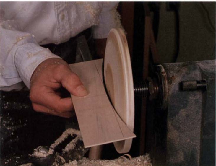
The platen is turned with a crown to match the dish in the baseplate. The curved platen (green in the drawing on the facing page) flexes the jaw plate.
