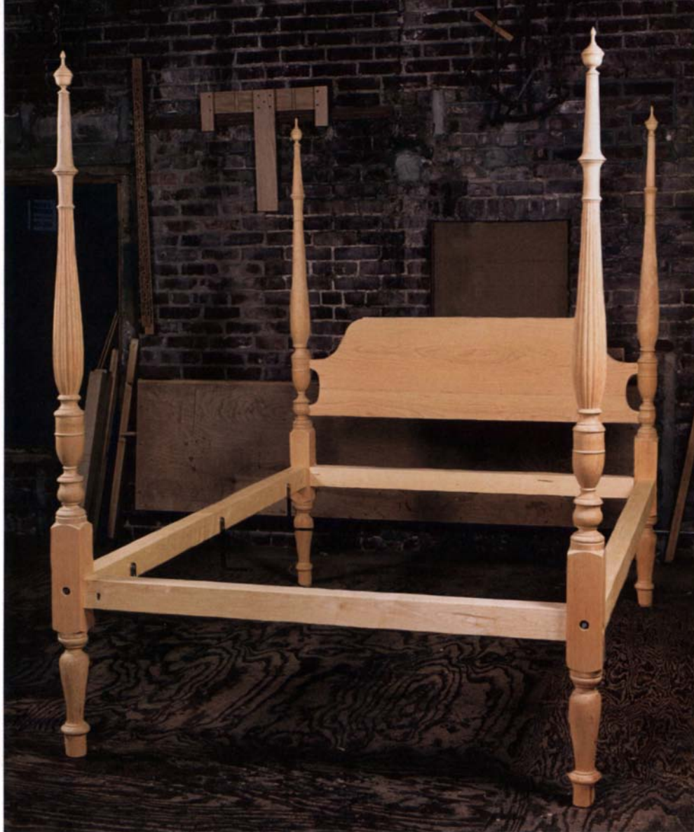
A Sheraton-style bed is easy to make, despite its complicated appearance. Reeding is time-consuming, but optional, and the joinery is straightforward. On this bed, the author skipped the reeding on the less-prominent headboard posts.
