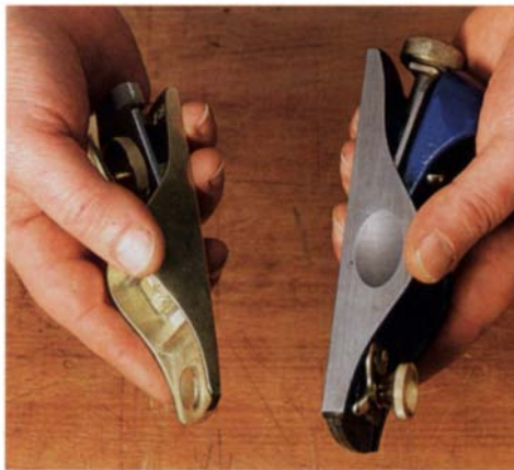
The Lie-Nielsen is smaller. Its low-angle block plane (left) is smaller than a Record and contoured for a more comfortable fit.
