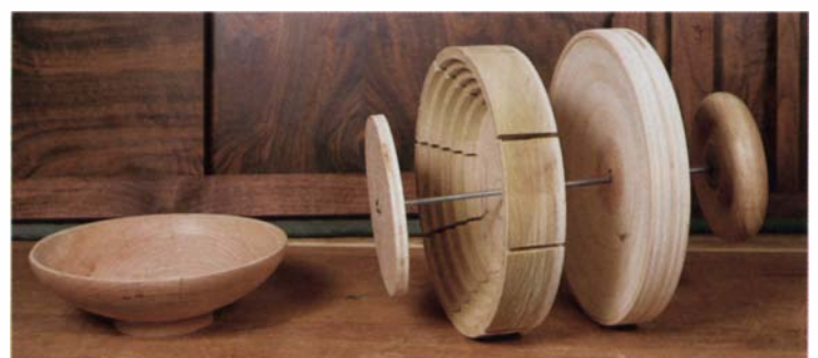
The parts are simple. A compression chuck consists of a platen, jaw plate, baseplate and handwheel (from the left), all connected with a threaded rod. Tightening the handwheel flexes the jaw plate, so it grips the edges of a bowl.
