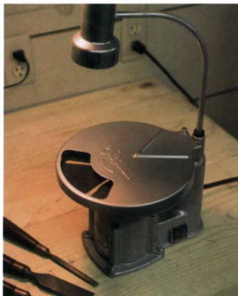
It's fast, but doesn't have a tool rest. The Stephan grinder uses a horizontally mounted, Carborundum-impregnated steel disc to grind tool edges. Slots in the disc make the tool visible as you grind.
