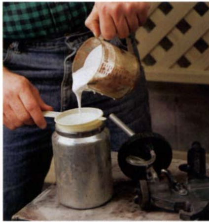
Clean finish, clean gun —To get blemish-free finishes, the author filters the finish before he sprays, and he cleans the gun afterward. He often tints his paint basecoats with pigment, so the topcoat covers better.
