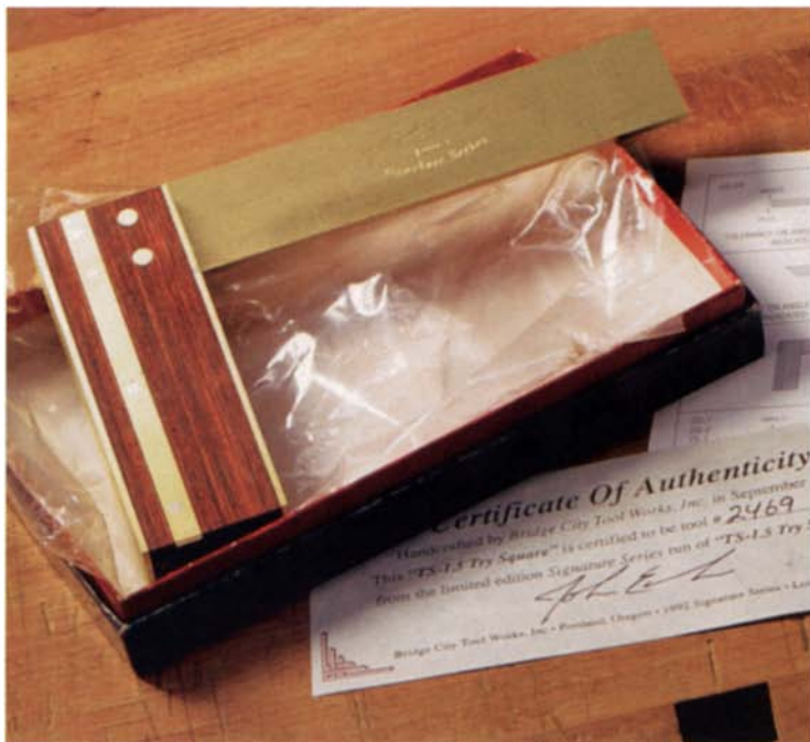
Careful packaging, guaranteed accuracy. The Bridge City try square is made of heavy brass and a laminated wooden handle. It comes with a certificate of accuracy.
