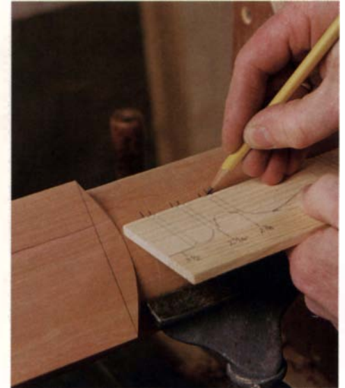
Use a story stick to lay out accurate and consistent turning details. And the story stick is a handy reference when turning because the shape and diameter of each post section is drawn right on it.
