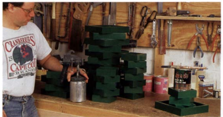
Spray guns increase production. Charron compares the number of clock frames he sprayed (left) vs. those painted with a brush.
