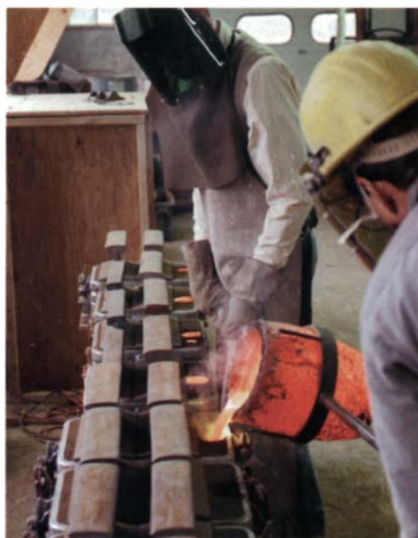
Production runs are very small. Molten manganese bronze is poured into sand molds at Lie-Nielsen Toolworks to form plane bodies.
