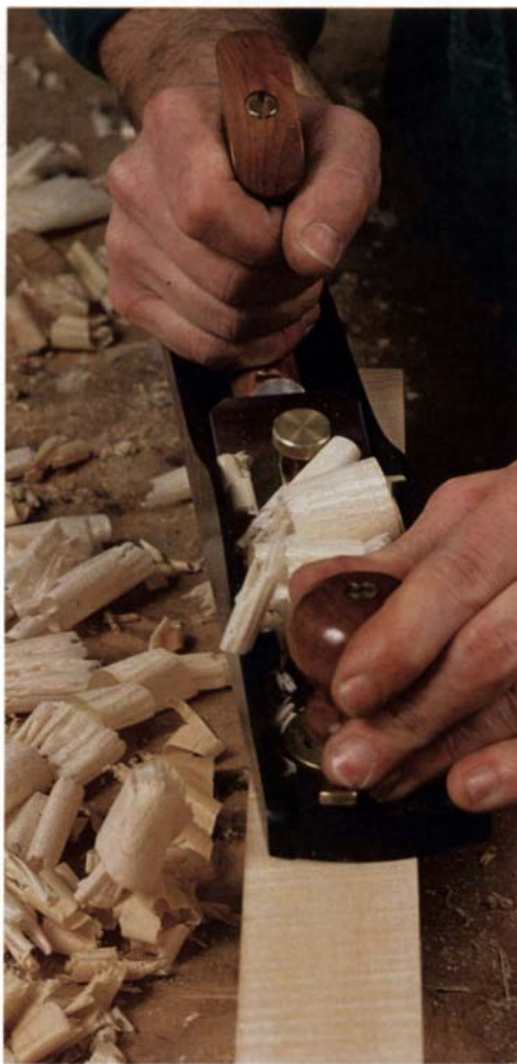
That's curly maple. The Lie-Nielsen jack plane can get paper-thin shavings from a piece of curly maple, a wood whose wavy grain makes chips and peck-outs all too common.
