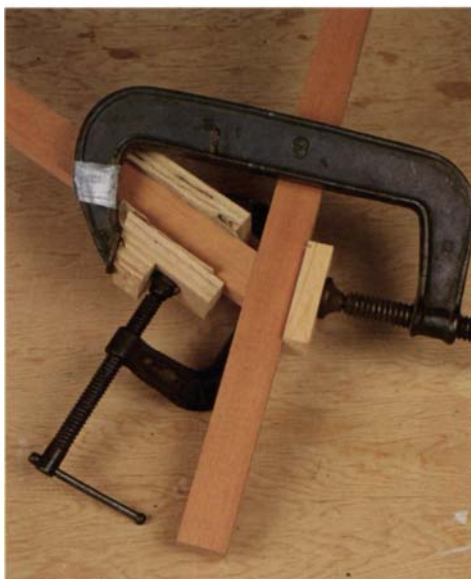
Caul clamps angled joint. By cutting an angle on the end of a plywood caul, the author can exert clamping pressure perpendicularly to the joint, drawing it tight.
