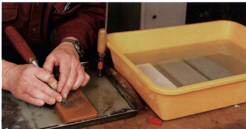
American-made waterstones are available in four grits. The Norton Co. has introduced a set of four waterstones in grits of 220, 1,000, 4,000 and 8,000.
