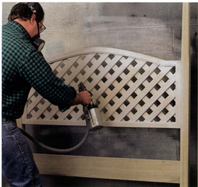
Spraying gets finish in nooks and crannies. One reason Andy Charron switched to spraying is that it gets finish where other applicators won't. Here, he sprays water-based sealer on the latticework of a poplar headboard.
