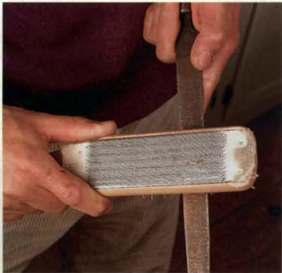
File card cleans rasps and files. Clean rasps and files cut more aggressively. File cards generally have a brush side and a wire side.
