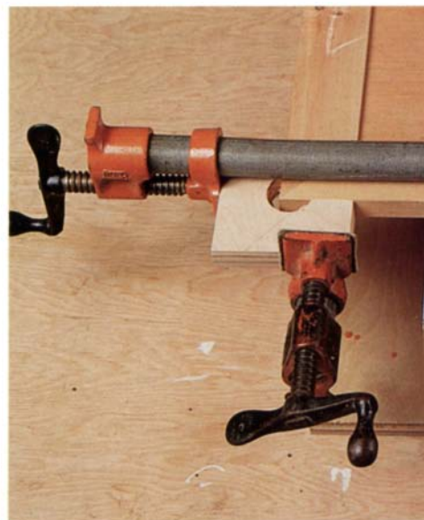
Notched cauls allow clamping of mitered frame. This simple plywood caul provides a bearing surface for clamps in two directions without getting in the way.
