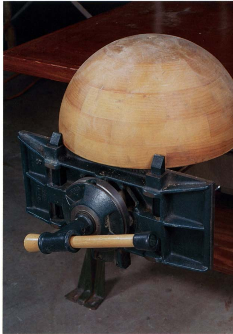
Cadillac of vises. With a price tag of more than $1,500, the Kindt-Collins vise isn't for everyone. Machined, hand-fitted parts explain its ease of operation, and the vise handles big, unwieldy objects (above). A tilt plate that fits between the jaws (left) allows the jaws to hold tapered stock firmly.
