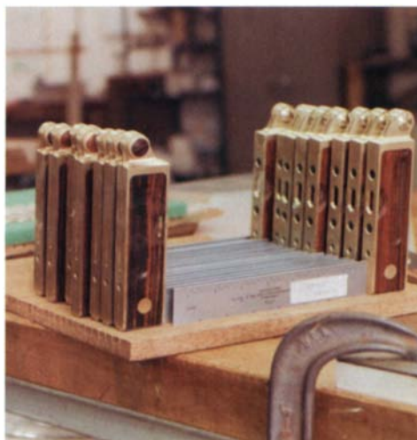
Tools are made one step at a time. Modern milling machines at Bridge City take care of the heavy work, but tools spend more time making the rounds in small batches for hand fitting and polishing.
