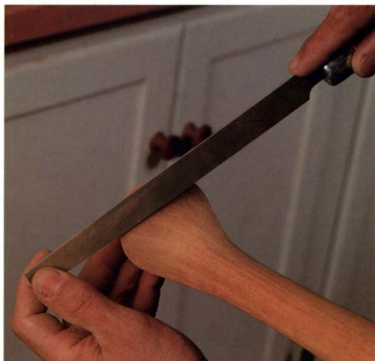
For best control, use two hands. Grasp the file or rasp handle with one hand, and hold the steel tip between thumb and forefinger of the other hand.
