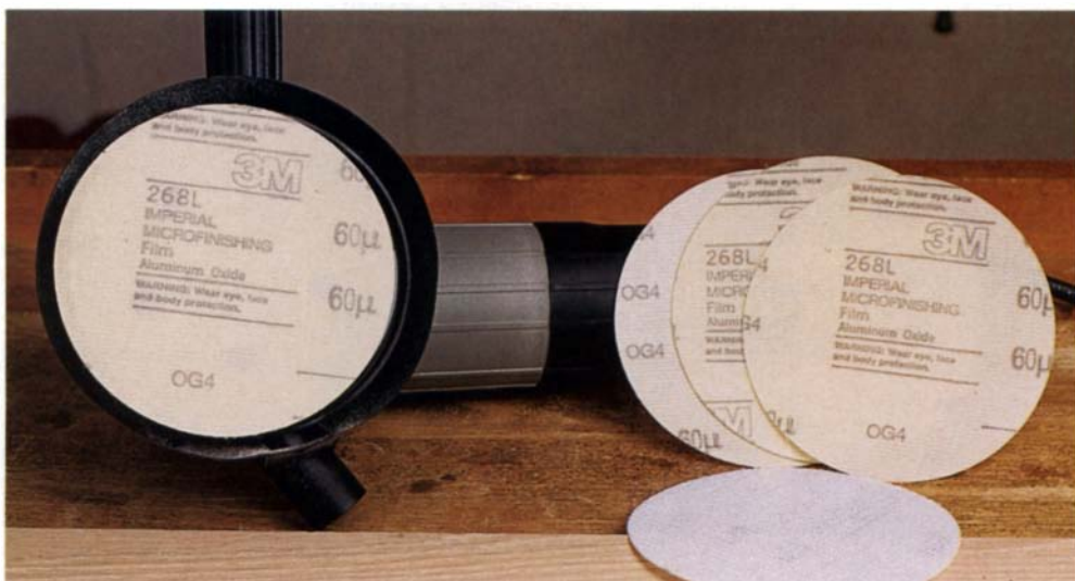
3M's Microfinishing Film discs work better and faster than standard sandpaper. These discs, which have a polyester backing, last much longer than paper-backed discs and can be used for wet-sanding.
