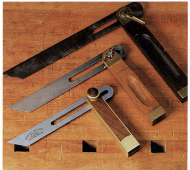
Adjustable sliding bevels in three grades. The Bridge City bevel (bottom) is built to last, with a price tag to match. The other two are from Stanley, one old (top) and the other recent.
