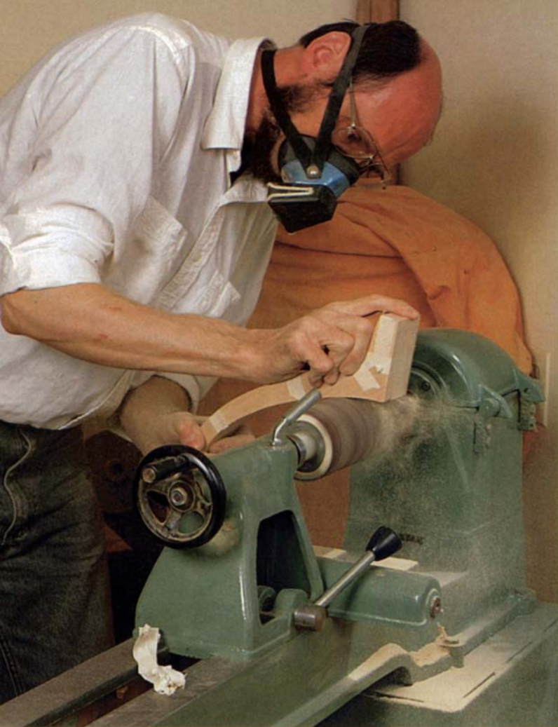
Sanding all the legs to the same shape is easier if the blanks are taped together before sanding to the layout lines. Bandsawing the legs close to the line reduces sanding.
