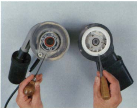
Brake parts wear but are easy to replace. No special tools are needed, and the parts are readily accessible.
