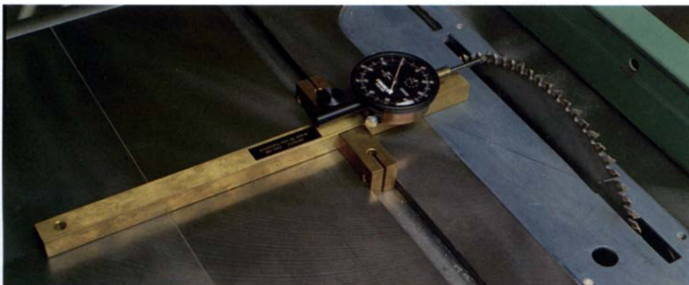
Quick, accurate machinery setups. The Infinitii alignment tool can be used to align and tune up a number of shop machines, but it's most useful on the tablesaw. The tool can be used to align the blade to the miter-gauge slot and set the blade angle.
