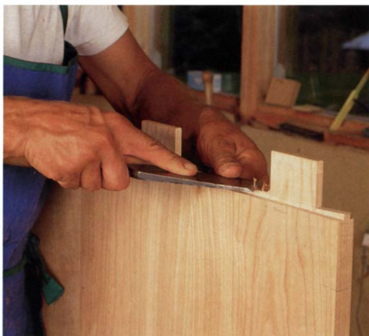
Pare the tongue to the line. Use a sharp chisel between the tenons to clean up where the waste was sawed away.
