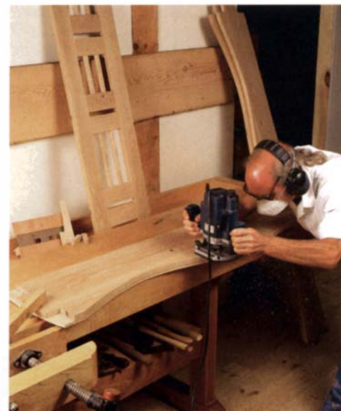
Templates and a router take care of shaping and mortising —Vogt made a plywood master template, so he could form the shelves, complete with tenons, using a straight router bit and a rub collar. The other templates are for shaping the slats, mortises and wedges.
