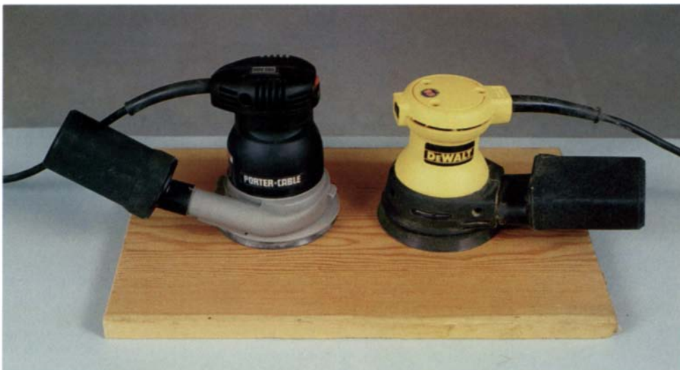
Aggressive sanding but no gouging. These new in-line random-orbit sanders are just as aggressive as their precursors but have a soft-start, non-gouging feature.
