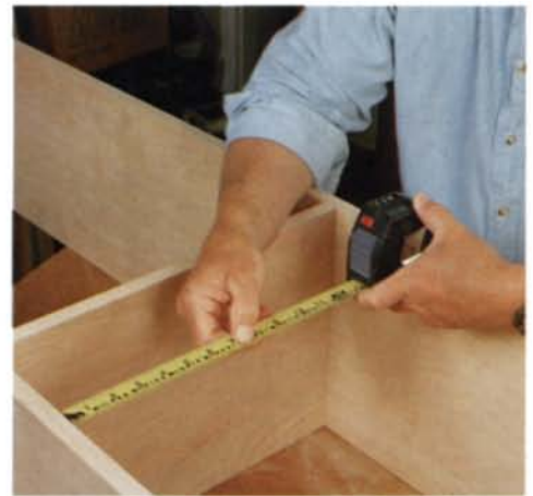
The Starrett Digitape allows you to easily measure the insides of cabinets, drawers and such, displaying the measurement in the LCD on top of the case.
