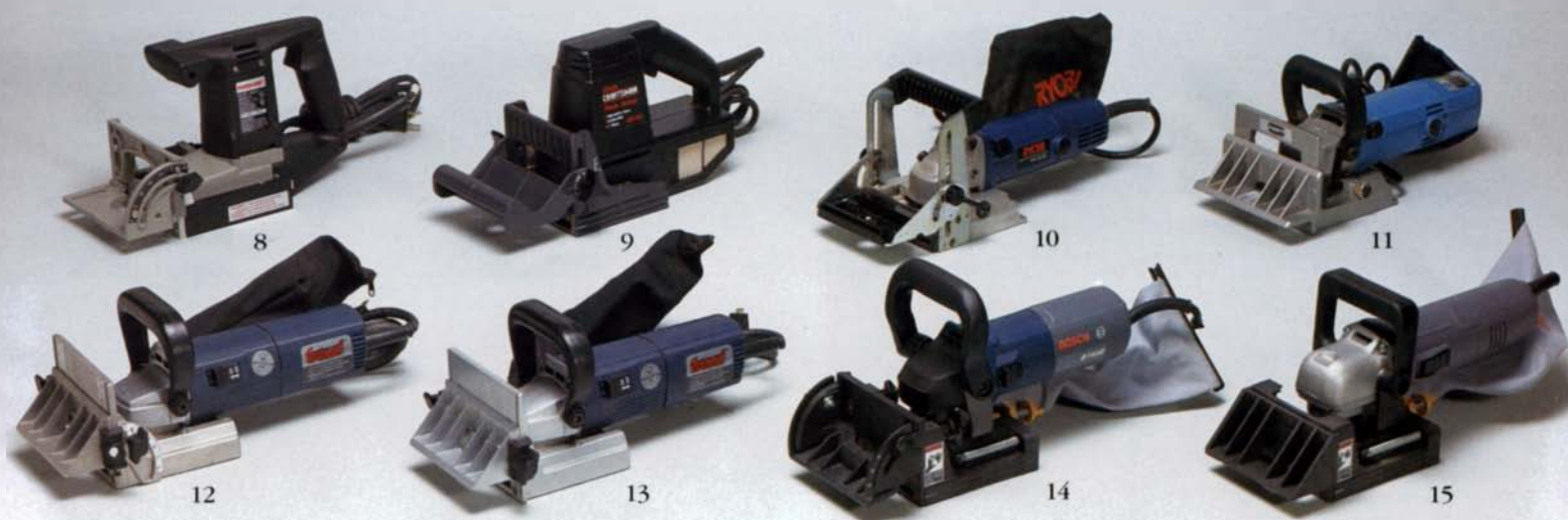
Plate joiners come in a variety of designs. Pictured from upper left are (8) Porter-Cable 556, (9) Sears Craftsman 17501, (10) Ryobi JM100K, (11) AMT 4960, (12) Freud JS102 and (13) JS100A, (14) Bosch B1650 and (15) Skil HD1605. The Porter-Cable 555 is not shown.
