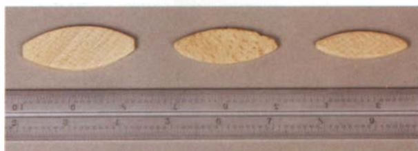
Biscuits come in three standard sizes: #20, #10 and #0. For the greatest joint strength, use the largest plate possible, and doubleup on thicker stock.
