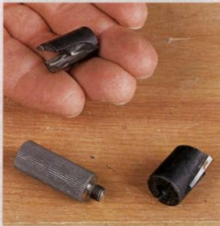
Panel-routing bits change easily. The only things the author uses from industrial panel routers are the bits, which have interchangeable cutter tips.
