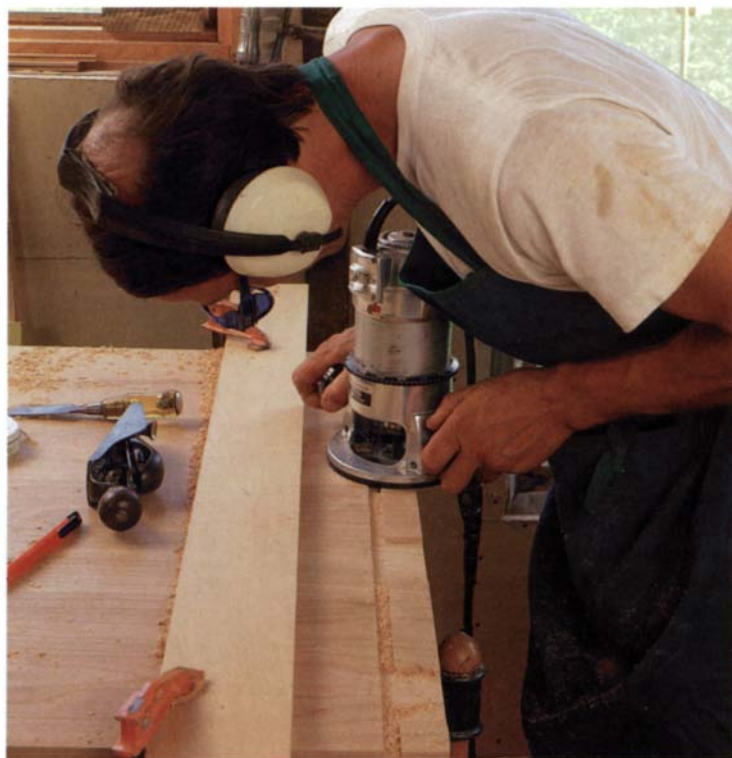
Waste stock between tenons supports the router base. A series of passes with the router takes tenons to thickness.
