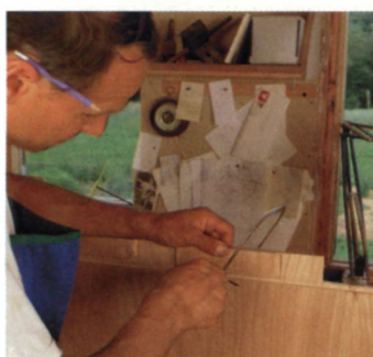
Waste stock between tenons supports the router base. A series of passes with the router takes tenons to thickness.
