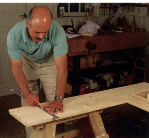
Layout speeds assembly —Laying out positions for the plinth, center and upper sections of the pilasters makes it easy to clamp the pieces in place, drill and countersink and then screw them home.
