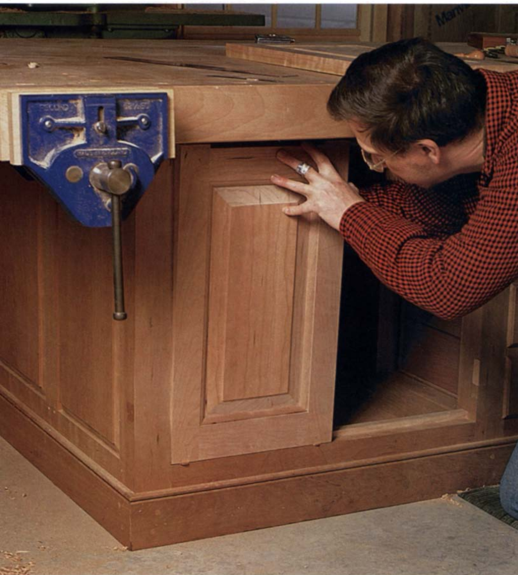
A knife is more precise than a pencil —Scribing around the hinge accurately marks its position. Darken the scribe line with a pencil to make the line easier to see when routing away the waste.
