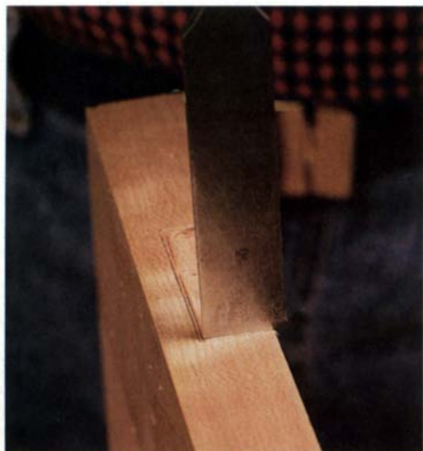
Pare mortises gradually to the scribed line, alternately cutting down and from the side. Be patient, and work slowly for best results.
