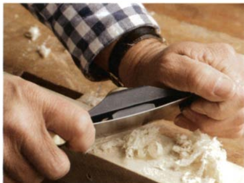
Scraper holder prevents burnt fingers, cut hands. Veritas Tools' new scraper holder grips the scraper firmly but permits plenty of adjustment.
