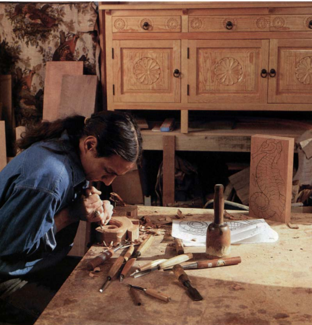
Carving for furniture —Nearly all of Patrick Trujillo’s furniture contains carving. To rough-out this mahogany sea horse, he uses both Japanese and English carving tools. Trujillo also made the traditionally carved pine sideboard in the background.
