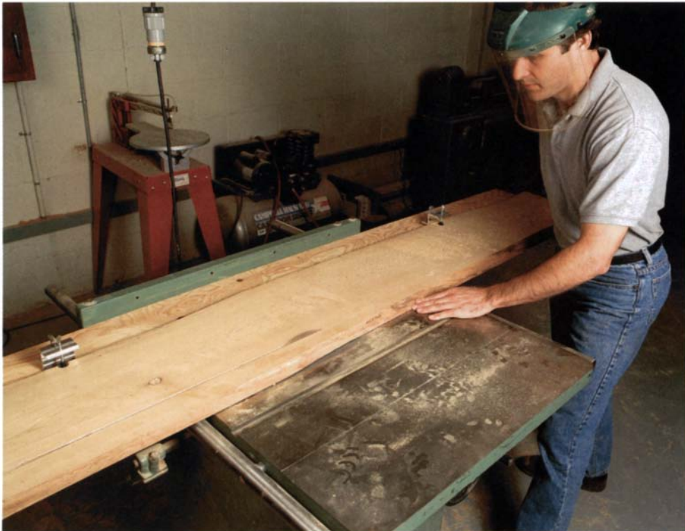
Use your table saw to put a straight edge on a wavy board. The Joint'r Clamp consists of two sections of aluminum extrusion that are drilled and tapped to accept thumbscrews. One thumbscrew grabs a straight strip of sheet stock, which acts as guide; the other thumbscrew grabs a crooked board you'd like to straighten. Then you just rip.
