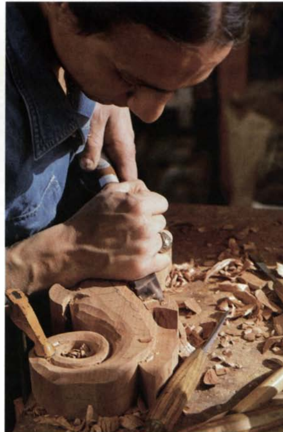
Carving new life into wood —Like Gepetto shaping Pinocchio, Patrick Trujillo turns a piece of mahogany into a lifelike creature. Starting with a block, and occasionally referring to his sketch, he carves a sea horse for a built-in cabinet at Evangelo’s bar in Santa Fe, N.M.
