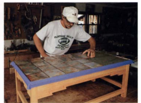
Setting the tiles— Jordan keeps the tiles in sequence to maintain the pattern. With these handmade tiles, he must pay extra attention to placing them, so there are no protruding edges.
