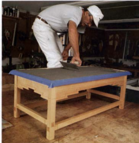
Setting the tiles— Jordan keeps the tiles in sequence to maintain the pattern. With these handmade tiles, he must pay extra attention to placing them, so there are no protruding edges.
