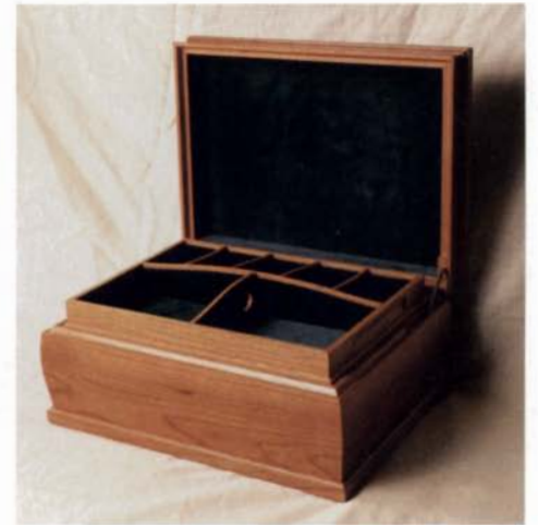
The velveteen-lined tray fits neatly into the box, resting on corner blocks to leave a space below. Curved-top dividers echo the curvature of the lid.
