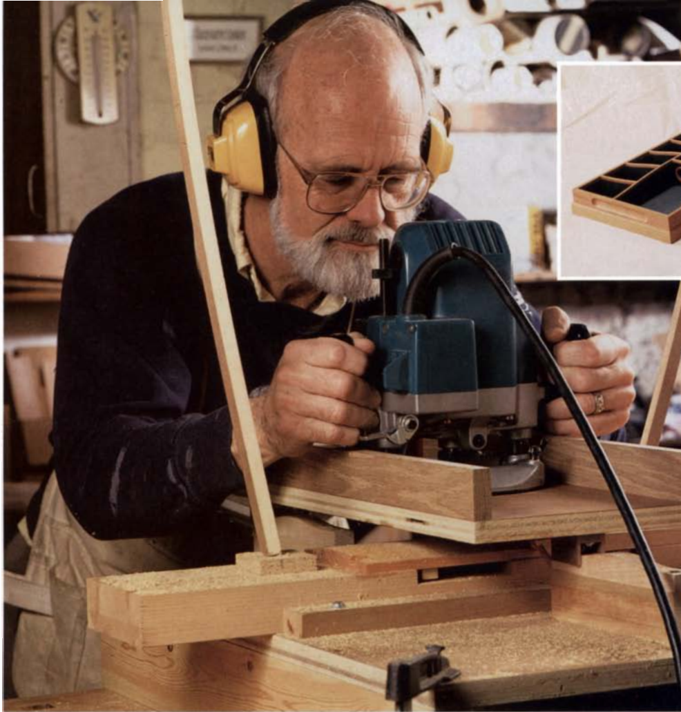
Jig lets router follow any contour—Working like a router sled, the author's jig allows quick, consistent shaping of the curved side of a box. The author wedges a pair of poles (go-bars) against the ceiling to hold the workpiece carrier in place.
