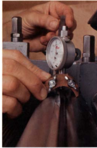
A cutterhead gauge enables knives to be set consistently to within one or two thousandths of an inch. The wing nuts on the base allow plunger height adjustment.
