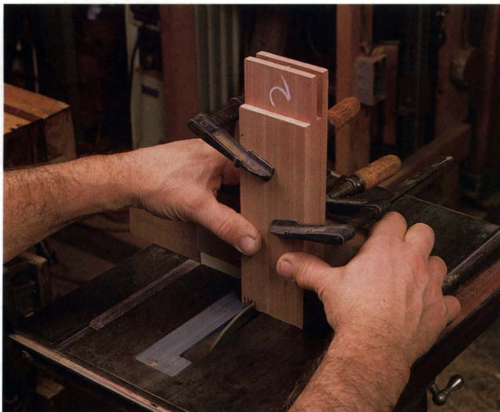
Gang-cutting box sides speeds the work. The author clamps all four sides together and makes multiple kerf-width passes using a guide pin to index each successive pass.
