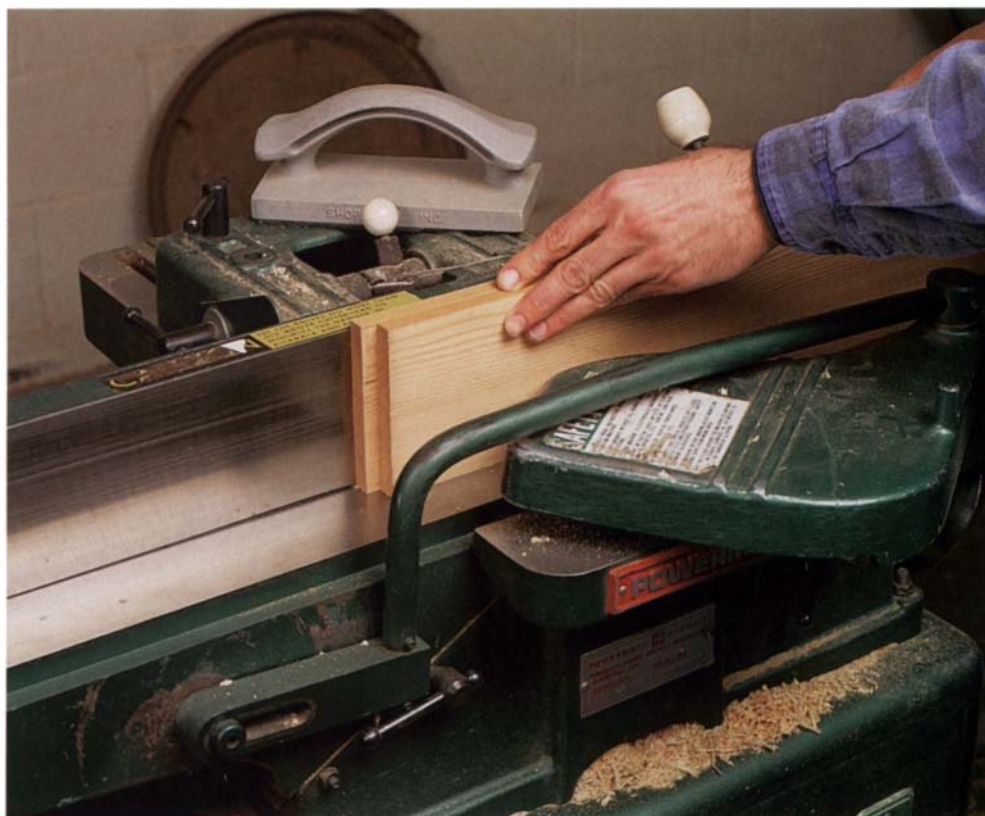
Fig. 2: Jointing complementary angles for edge-gluing
