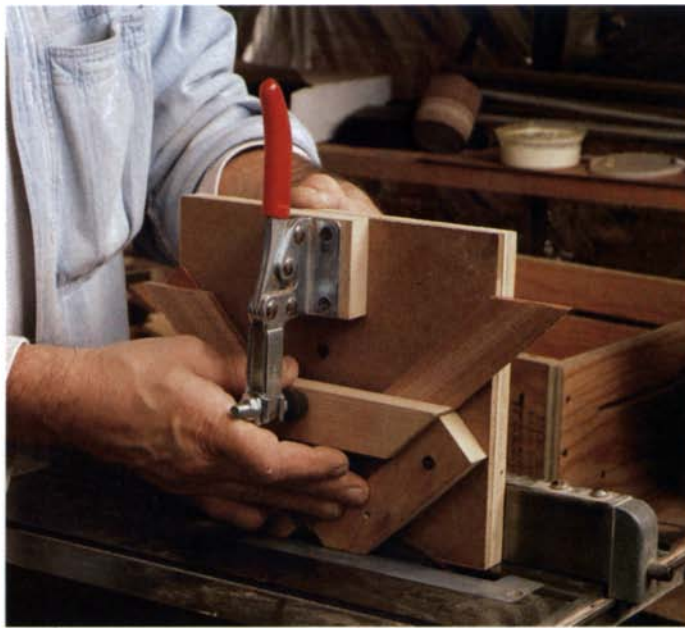
Cut spline slots safely and precisely with simple jig. A toggle clamp and caul hold frame members in place while a pair of screwed supports position the frame members at exactly 45° to the saw table.
