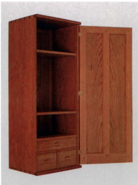
Adjustable shelves and drawers with carved pulls enhance the simple features of the dovetailed carcass. Also shown is the routed finger pull used on the carved, flush panel door.
