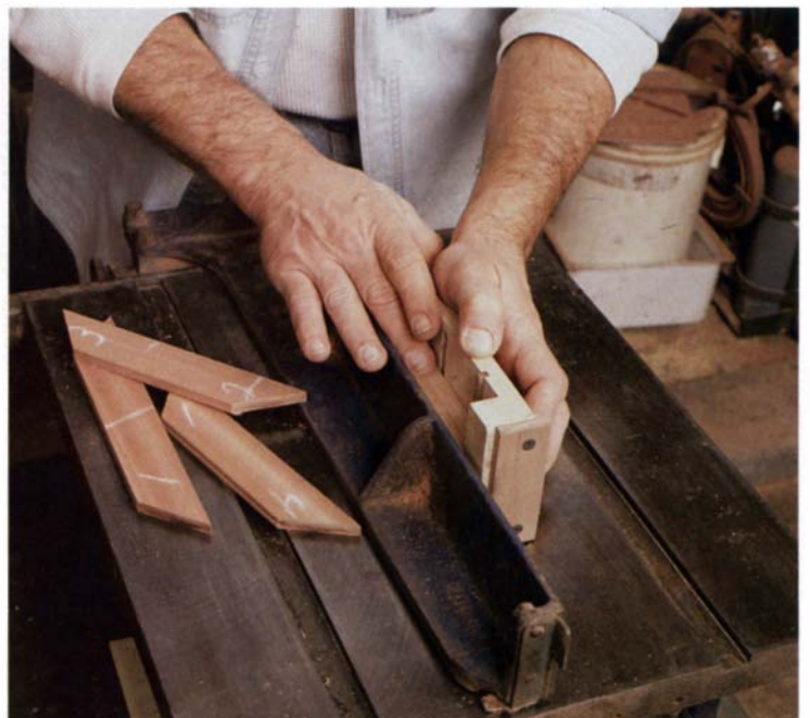
Cut small parts accurately and keep your fingers out of danger by using an adjustable push box. This jig exerts downward and lateral pressure to keep the workpiece flush against table and fence.
