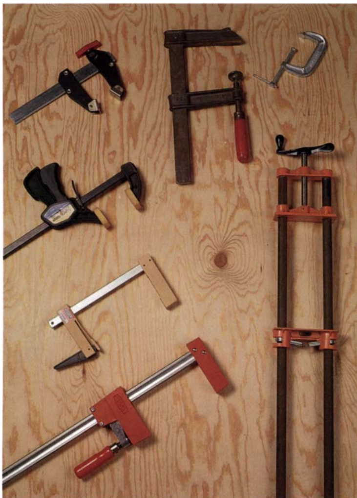
How clamps clamp —Here's a sampling of clamp jaws (from upper left down): Jet Clamp (turn-screw pivot); Quick-Grip (trigger clutch); Bessey's Klemmy (cam lever) and K-Body (friction slide). For handles, Maas likes Wetzler's wooden grip (top center) and Jorgensen's crank (bottom right) but not the C-clamp's staked rod.
