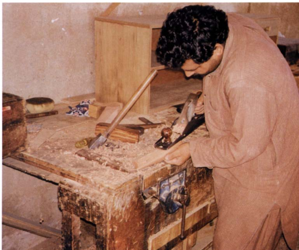
"Turning" without a lathe—After adzing a rough billet round, a craftsman in Oman trues up the cylinder for a bed leg with a bench plane.
