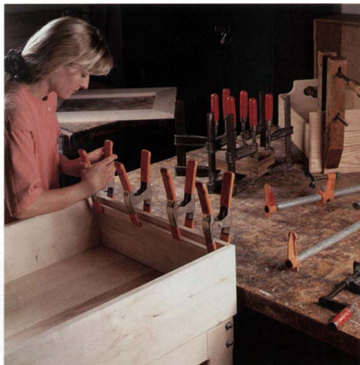
Older style clamps still work well —Spring clamps, used here by student Leisa Goerlich to clasp a cleat, are one type the author uses regularly. Two others on the bench are Wetzler bar clamps (laminating walnut) and a hand screw clamping an oak drawer front.
