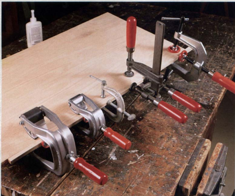
Clamps for edge-banding —Edge clamps (photo above) are lined up here for an end run on plywood. From left to right, the models are two sizes of Kantenfix (carried by Tape & Tools), Jorgensen Pony, Wetzler and Bessey three-way edge clamps. The Kantenfix models were the quickest to use, and the Wetzlers exerted the most force.
