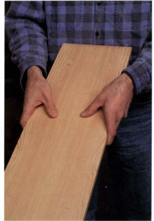
Sprung joint keeps ends together —The slight concavity of a sprung joint adds an inward stress to the ends of the jointed boards, making the joint less likely to open. The gap between the two boards at center is no more than 1/32 in.; hand pressure should be enough to close it.
