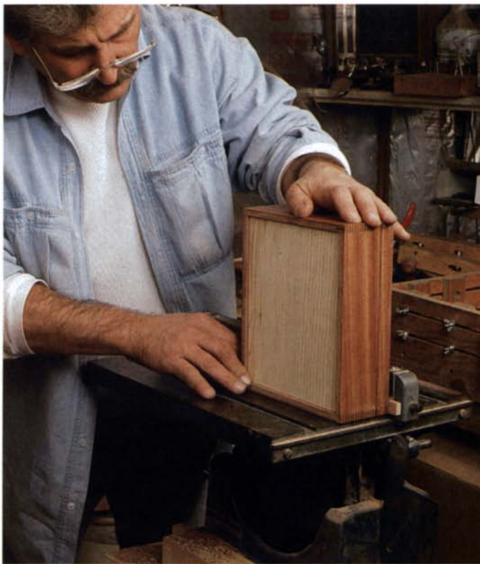
Cutting open the box to make the top—Kerf 1/64 in. shy of going through the sides, so the box won't come apart on the tablesaw. A utility knife finishes the job.
