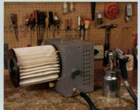
High volume, low pressure (HVLP) in a small package. At 15 in. sq. and 18 lbs., the shop-built turbine-powered HVLP spray unit in the photo below is a fraction of the size and weight of the standard medium-sized compressed air setup in the photo at left.
