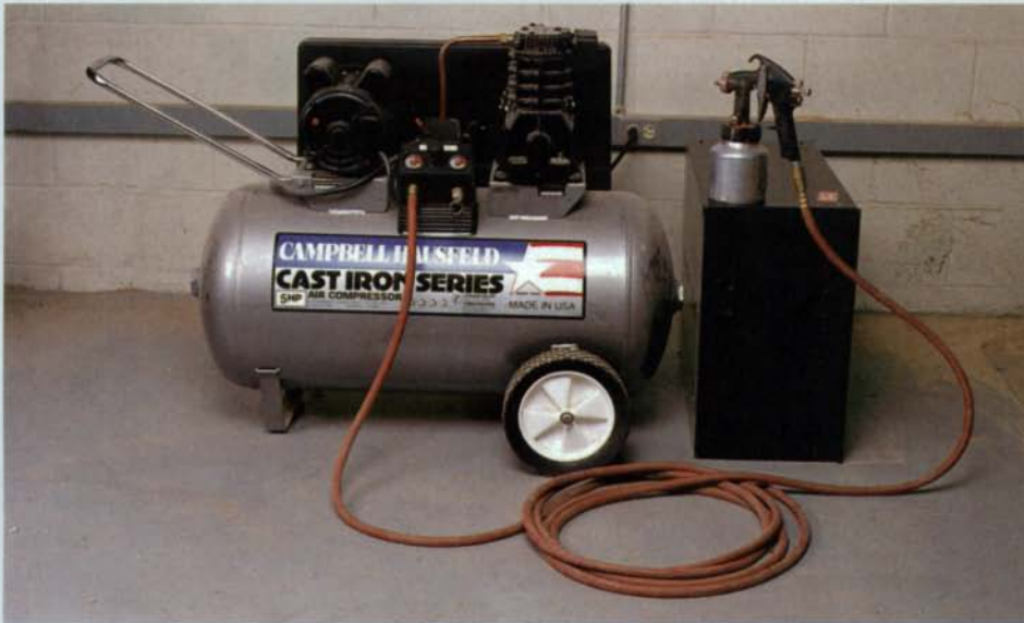
High volume, low pressure (HVLP) in a small package. At 15 in. sq. and 18 lbs., the shop-built turbine-powered HVLP spray unit in the photo below is a fraction of the size and weight of the standard medium-sized compressed air setup in the photo at left.
