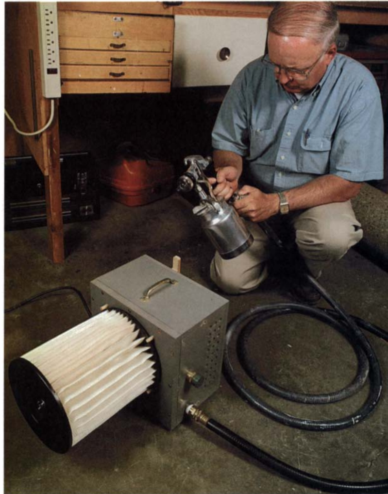
Shop-built spray unit —A high-volume, low-pressure unit like this one that the author built is ideal for on-site work or in the shop.
