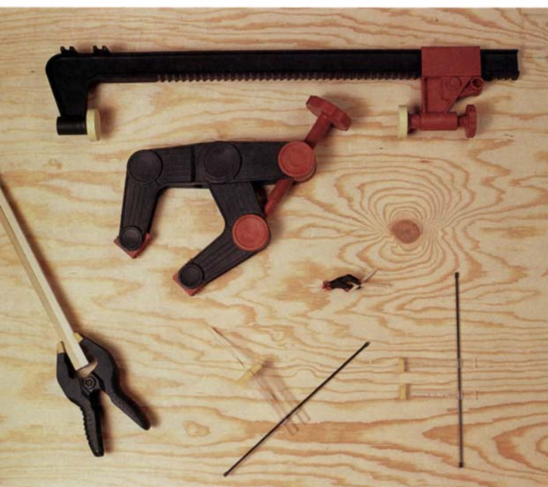
Plastic clamps suit delicate jobs. The rubber pads of Quick-Grip's spring clamp (left) are gentle on work. BTM's lightweight polymer clamps (top) resist rust and solvents. Their miniclamp and Testfabric's clear acrylic clamp are good for restorations.
