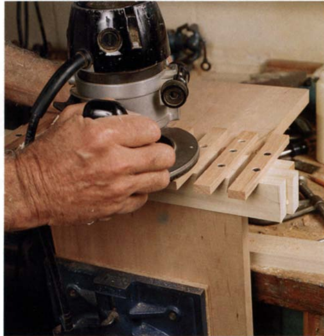
To make a tail jig, build a holding fixture that forms a collar around the stock, screw guide fingers to the top edge and then rout between the fingers to create the sockets.
