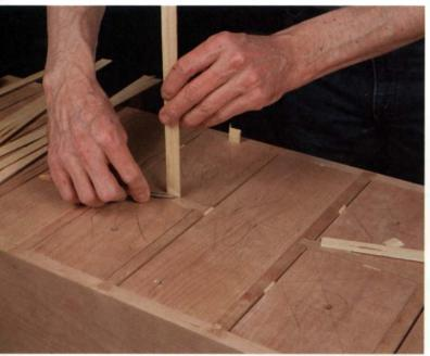
Wedging the drawers in place holds them for beltsanding. The drawers should be wedged on each side to center them in the opening and wedged at the top to hold them firmly against the drawer dividers and stops. The entire front of the cabinet can then be sanded to one flat, smooth plane.
