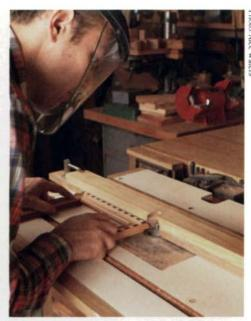
Relying on his shopmade router table for shaping work, Segal advances an assembled frame by the bit, taking multiple passes. He uses a custom-made fence with an appropriately sized cutout for the bit.
