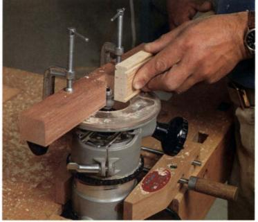
Beads on every corner—Rodriguez machines all four edges of an extra piece of frame stock to generate molding for a door. For short lengths, use an inverted router; for longer ones, use a router table.
