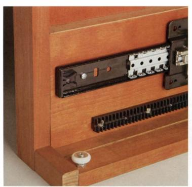
Glide-mounting strips position the hardware flush with the inner edge of the frame so that pocket doors can be used on cabinets with conventional face frames.
