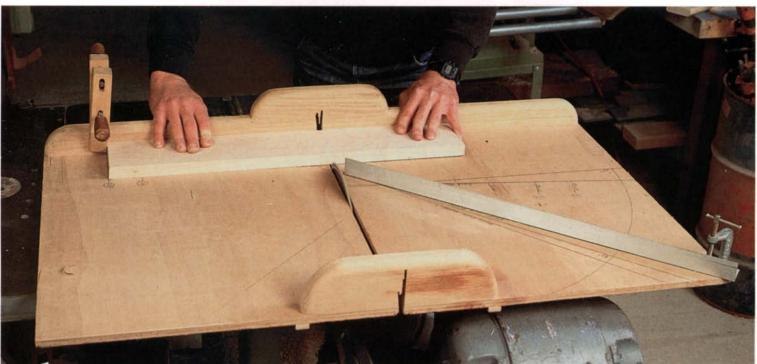
The dedicated crosscut box lets the author make virtually identical copies of his design next week, next year or in 10 years. All angles, stock widths, part names and cutoff points are marked on the box, making production a simple matter of running through the cut list.
