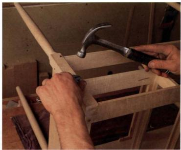
Rosewood pegs strengthen the joint, and they add a distinctive touch to the author's table. The adjustable wrench keeps the pegs properly oriented, parallel to the case's top and sides.
