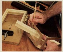
Marking and clamping miters—Ted Myers made two fixtures to help him make frames from salvaged moldings.
