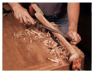
Shape and blend the curves of the cabriole legs with rasps and files. The leg should be round at the ankle and square with rounded corners just below the knee.
