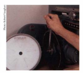
Everlast SMT 1210 blade—According to contributing editor Robert Vaughan, this Everlast circular sawblade is the quietest he's used, as registered on a decibel meter. When installed on his radial-arm saw, the 12-in., 100-tooth, alternate top bevel blade (\$100-\$190 for a 10 in., about \$200 for a 12 in.) crosscut birch plywood and medium-density fiberboard (MDF) effortlessly and without tearout.
