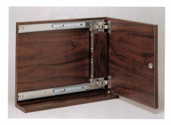
Passive followers are solid struts that keep the hinge-slide mechanism aligned so that the door doesn't sag and jam when it's opened or closed. A wooden follower is used in this mechanism (above).
