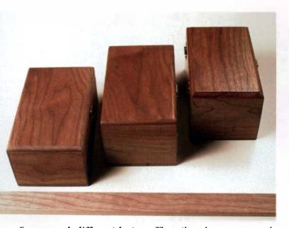
Same wood, different lusters—These three boxes were made from a single piece of walnut (a strip is shown at bottom), but finished differently: The left box was coated with linseed oil to give a dull look; the center box was wiped with shellac and waxed to a satin sheen; the right box (with the reveal on the lid) was brushed with polyurethane varnish and burnished to a low gloss. The finishes also bring out variations in color and grain contrast.
