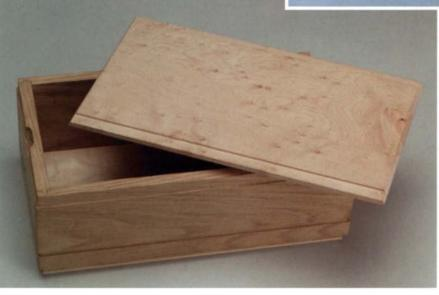
Straight components and crisp joinery are the hallmarks of this router-shaped box (left). Patrick Warner of Escondido, Calif., capped the 9-in.-wide by 3-in.-high white-oak box with a bird's-eye maple top. In keeping with the clean look, he left the wood unfinished.
