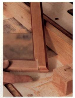
Access slot—After routing a picture-entry slot by sliding this frame between two stop blocks on his router table, Segal checks the fit of the glass. The frame back was coved to show more of the spline.
