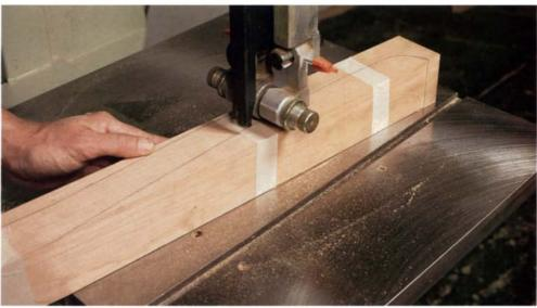
Billet rebuilt—With the blade guide lowered to just above the stock, bandsaw along the layout lines. Tape the cabriole cutoffs back in place, and turn the billet 90° to make the second pair of cuts. After turning the foot, clean up the bandsawn curves with a spokeshave.
