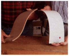
Curved panels are a lot easier to build when you start with a material that's meant to curve. Wiggle wood (left) and Italian bending poplar (right) both take curves naturally.
