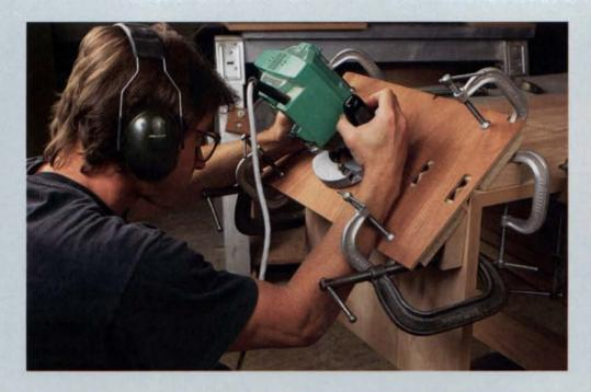
Keyed miters—Two sides of an alder toy box (above) show how attractive a keyed miter joint can be. To rout key grooves in big mitered carcases (left), it's safer with a simple jig.
