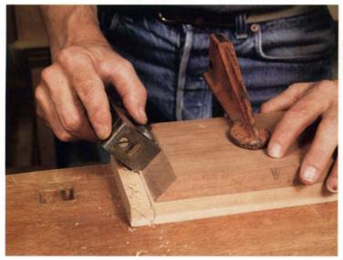
Run a rabbet plane along a guide block to cut the chamfer that limits the swing of the knuckle joint hinge.
