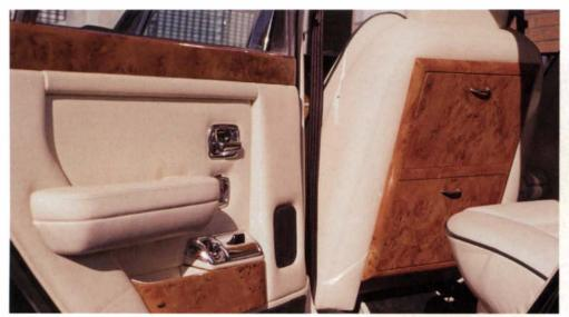
Complete interior of wood and leather—In addition to leather seats, curved veneer trim and door pockets, this Hooper limousine's custom woodwork includes a burr yew console, which elegantly houses a television, VCR, compact disc player and crystal ware.
