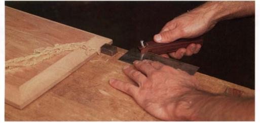
Timberline Tools' scraper burnisher is an attractive, functional and reasonably priced tool. The hardened-steel dowel pin set at a fixed angle ensures a consistent burr every time, making scraper preparation no longer a hit-or-miss affair.
