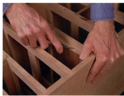
Scribed lines accurately position stops—The author uses a 4-in.- to 6-in.-wide board, cut to the appropriate length, as a gauge to scribe alignment marks for the drawer stops. Measuring from the cabinet back eliminates any variations that may have occurred when gluing in the dovetailed drawer dividers.
