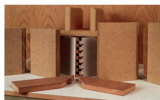
A wide variety of joinery is possible with MDF. Examples shown here surrounding a routed dovetail joint are, clockwise from left, biscuits, dado, rabbet and dado, spline miter and biscuited miter. The background is a sheet of factory-veneered MDF.
