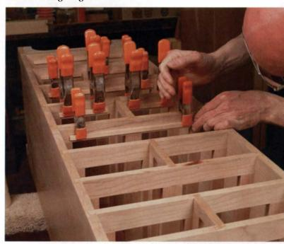
The drawer stops are glued, positioned on the dividers and held in place with spring clamps. The stops must be thin enough to clear the drawer bottoms and short enough to allow drawer side clearance at the ends. Leather bumpers are temporarily glued to the stops to position the drawers for sanding.
