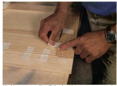
Masking tape supplies all the clamping pressure you need to glue up the molding. The shadow line created by the quirk behind the bead gives a bit of leeway in correcting small mitering errors.
