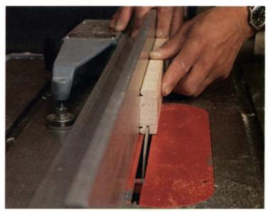
Kerf between the beads to cut their back edge, and then rip the two pieces from the board.
