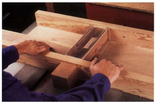
Crosscuts safe and simple—A three-sided box over the line of the cut reduces the chance of accidental blade contact on the author's crosscut jig. The box, with 3%-in. wood sides and a 1/8-in. Plexiglas top, is held in place at one end by two cleats and rides up and down between them. An exit block guards the blade at the end of the cut.
