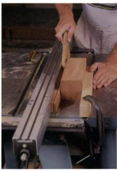
Resawing reconsidered—A chunk of 4x4 screwed to a stick is all that it takes to keep the stock vertical and the blade safely hidden while resawing. If you resaw often, you can screw the guard block directly to a dedicated throat plate.
