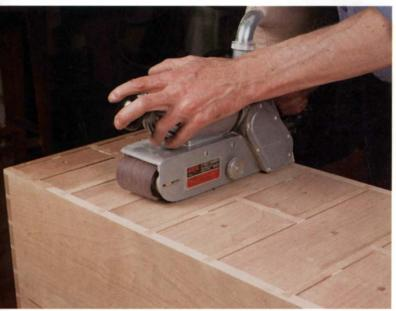
Sanding the cabinet front, with the drawers held in place by front-mounted stops and wedges, ensures that the entire face of the cabinet will be flat and smooth. The drawers support the sander and prevent gouging the face frame. This technique eliminates the need to set each drawer individually.
