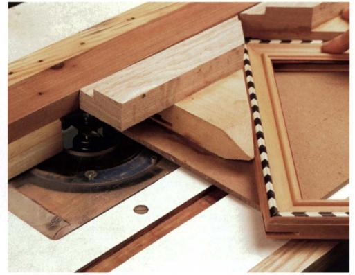
With a groove-cutting jig and a slot-cutter in his router table, Segal plows grooves in this inlaid frame for the miter splines. The jig cradles the frame corner securely at a 45° angle to the fence and keeps his hands out of harm's way.
