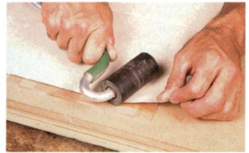
A laminate roller works bubbles or wrinkles from canvas that's been glued to the back of slats. This canvas forms a fabric hinge that allows the tambour to run flexibly.
