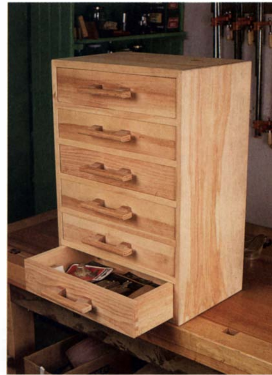
Workmanlike utility furnishings, like the author's little cabinet for storing nails and screws, make the shop efficient and pleasant. Rabbeted corners, screwed and plugged, join the pine case, which measures 17 in. by 24 in. by 10½ in. deep.
