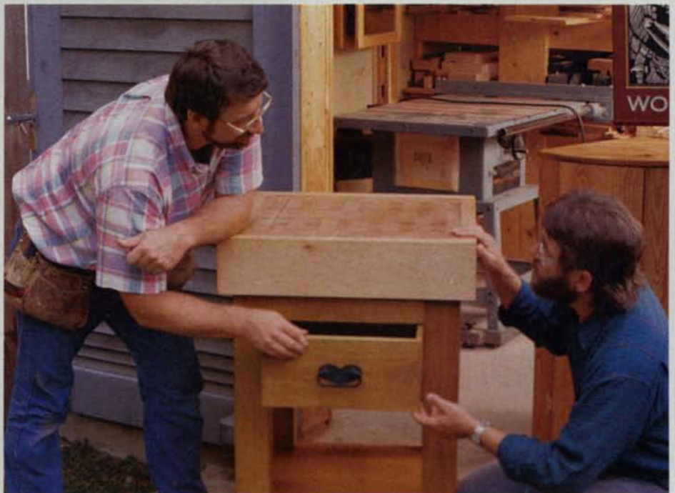
Handling wood movement gets top priority. This table's endgrain butcher-block top is beveled on four sides and floated within an oppositely tapered 2x6 frame. Although Abram admits the construction is experimental, he says it's designed to allow an expanding top to slide upward in the frame. As the author looks on, Abram explains how the top works and how the rest of the table was built.
