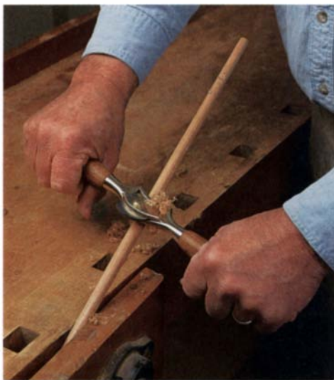
Well-balanced, precisely machined and hand fit, Brian Boggs' concave-sole spokeshave is a fine finishing tool.
