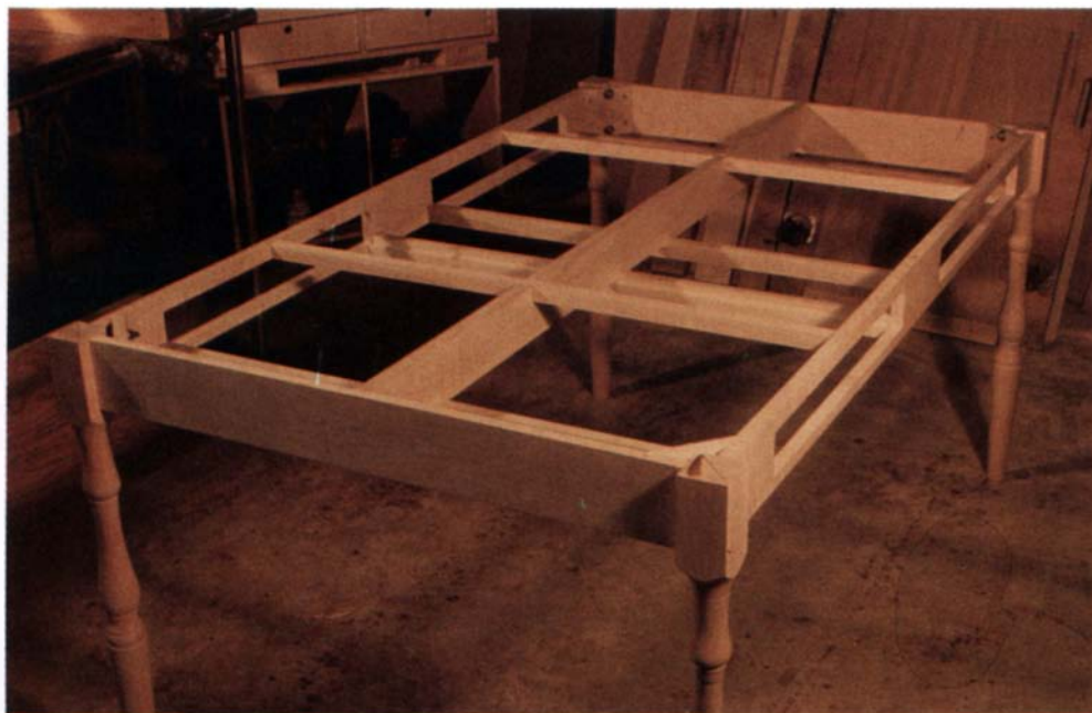
The strongback runs the length of the table and is secured to the end aprons, the drawer runners and kickers, and the top to tie the components together into a strong unit.
