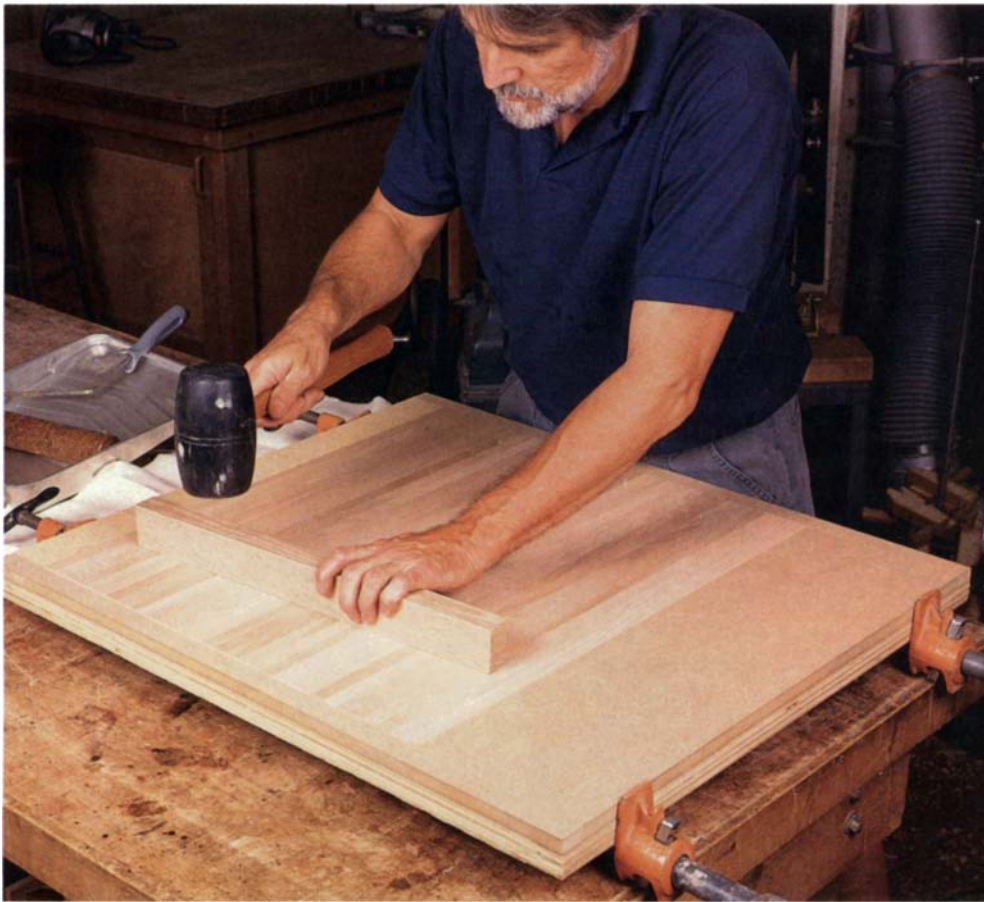
A shopmade fixture secures the slats for gluing on the canvas backing. Pipe clamps and a wide batten board cinch the slats tightly together; a few blows from a mallet ensure that all slats are flat.
