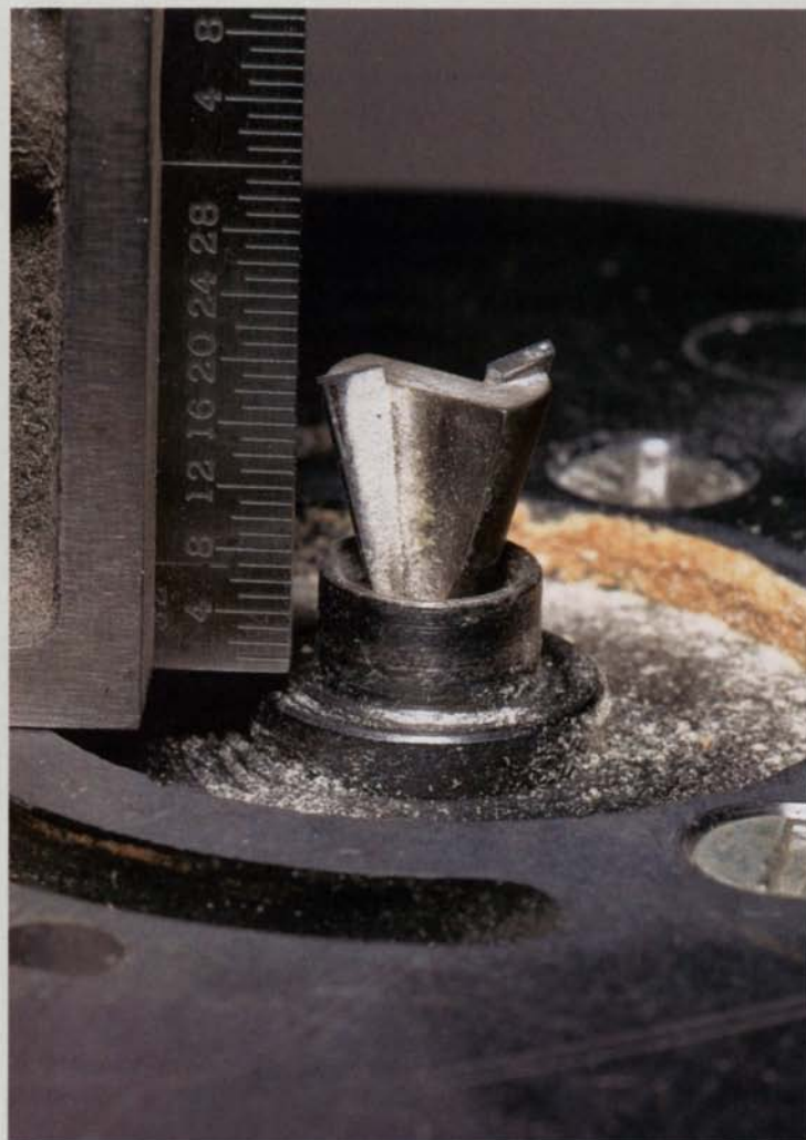
Bit setting determines joint tightness. Owner's manuals typically specify a depth-of-cut setting, which determines how the joint fits. The deeper the cut, the tighter the joint. But finding that just-right setting for your router and template is really a matter of tedious trial and error. A carbide-tipped bit is best for dovetailing because you cut to full depth in a single pass, which calls for cutting edges that stay sharp.
