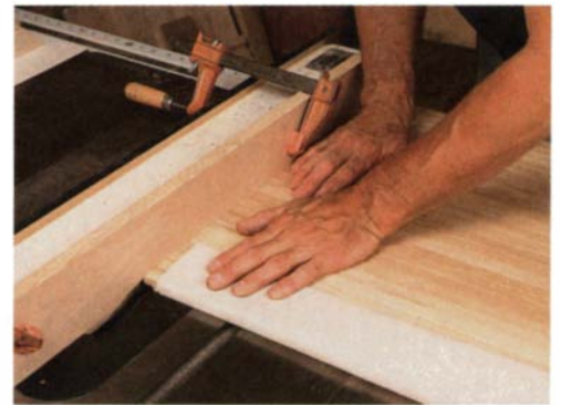
A shopmade fixture secures the slats for gluing on the canvas backing. Pipe clamps and a wide batten board cinch the slats tightly together; a few blows from a mallet ensure that all slats are flat.
