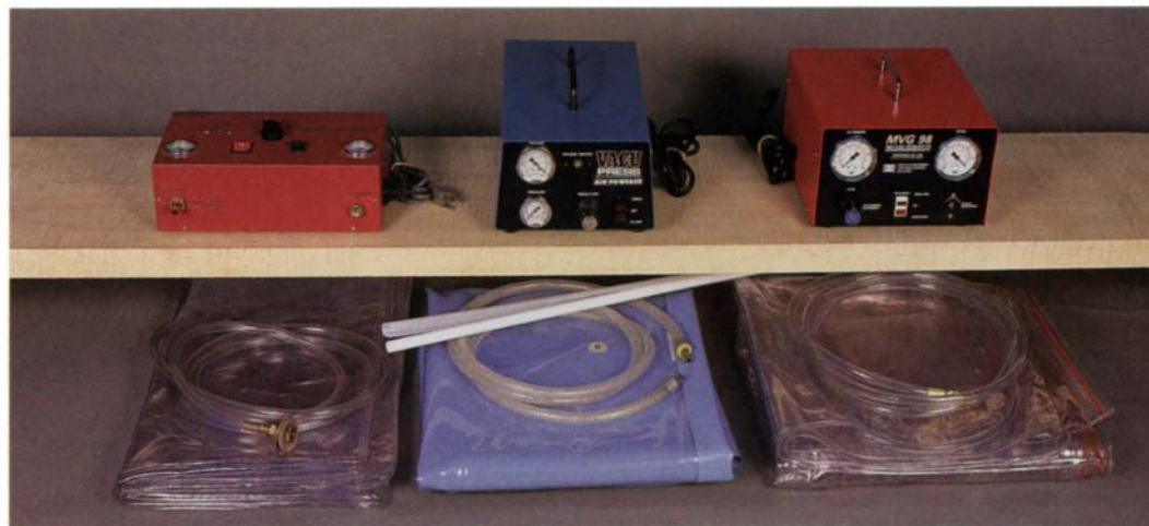
Automatic venturi pumps with bags , arranged from left to right by price: Quality VAKuum Products, Vacuum Pressing Systems and Mercury Vacuum Presses. Powered by an air compressor, venturis are generally a little slower than rotary-vane pumps but usually a little cheaper as well and are suitable for light-to-moderate vacuum pressing.
