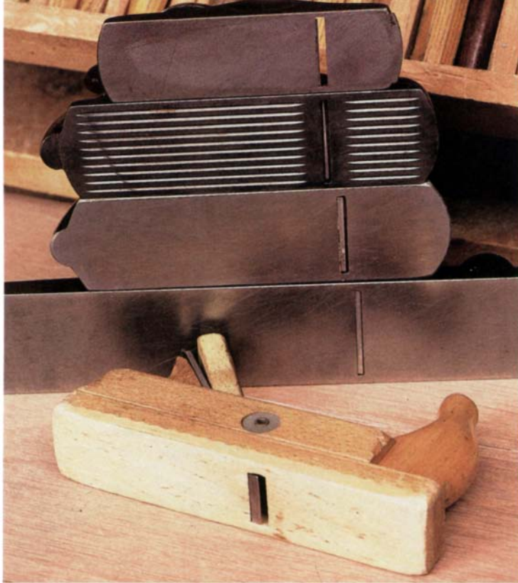
Plane soles vary mostly in width and length, but there are other differences, too. From the bottom up: a wooden scrub plane with horn-beam sole, a #8 jointer plane with narrow throat, a #4 smooth plane, a #4 with corrugated sole and a low-angle block plane with adjustable throat.
