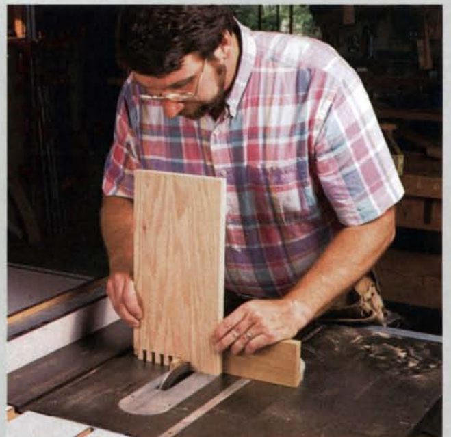
Finger-saving finger joints: Abram uses jigs, especially when a machine's guard has been removed for photographic clarity (or otherwise). To make tablesaw operations logical and safe, he builds jigs, for example, that ride in the saw's miter grooves, as shown here.
