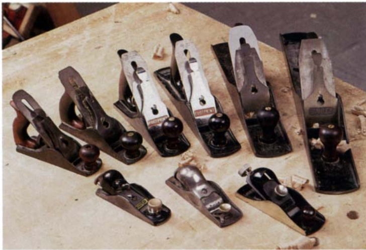
Commonly available metal handplanes. The back row (from left to right) displays Stanley-style bench planes: #2, #3 and #4 smoothers; #5 jack; #6 fore and #8 jointer. The front row shows block planes: a low-angle Stanley (left), a standard-angle (right) and an old low-angle type that has a knuckle-joint lever cap (center). Both low-angle models have adjustable throats.
