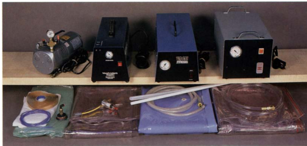
Rotary-vane vacuum pumps , arranged from left to right according to increasing list price, include units from Vacuum Tool Co., Woodworker's Supply, Vacuum Pressing Systems and Mercury Vacuum Presses. Rotary-vane pumps are the best choice for moderate-to-heavy vacuum pressing requirements. Also shown under each unit are its closure systems and vacuum line connections.
