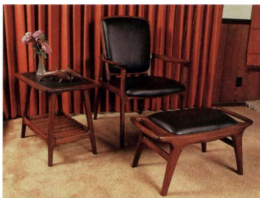
Angled tenons—some compound—were used almost exclusively in the construction of this walnut chair, stool and side table. Legs on two of these pieces splay in two directions, requiring slightly angled tenons at both ends of apron pieces, stretchers and seat supports.
