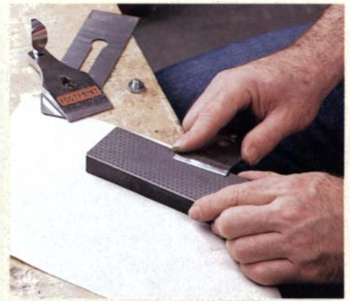
Flatten the edge of a cap iron using a sequence of coarse, medium and fine diamond stones. Next flatten, or lap, the back of the plane's blade before honing its bevel. Then dress the edge of the lever cap.
