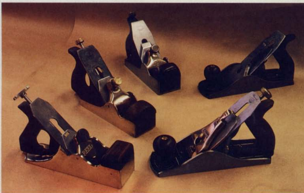
Inspiring smoothers: The mint-condition used planes in the background (an A-6 Norris, left, and a Stanley #4½, right) are hard to find. But, a few new planes borrow features from these originals, as shown in the foreground: Bristol Design's P-40 (left center), J. Warshafsky's 04 Reed (left front) and Record's Calvert-Stevens CS-88 (right front).
