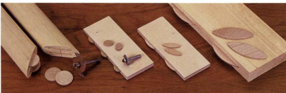
New biscuits (from left): Lamello #11 rounds with four-winged router bit, Woodhaven Itty-Bitty bits with cutter, Lamello's smallest #H9 and jumbo #6 biscuits.
