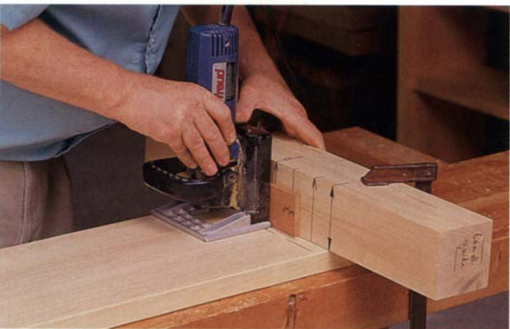
To slot the faces of the uprights, square a line that locates one edge of the fixed shelf. Clamp the 4x4 gauge right on the line, and with the machine vertical, run the first row of slots. Then place a spacer— \frac{5}{16} in. thick in this example—between the machine's base and the 4x4 to cut the second row of slots.
