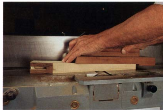
8) Frid tapers both sides of each leg
