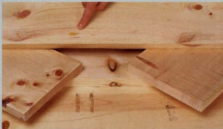
Defects in pine boards can cause problems. All knots radiate from the tree's center, so boards containing pith also contain spike knots (top). Black knots (bottom) are encased stubs of broken branches. They're dangerous if they fall out during machining. Tight red knots (center) may crack and split, but they don't fall out.
