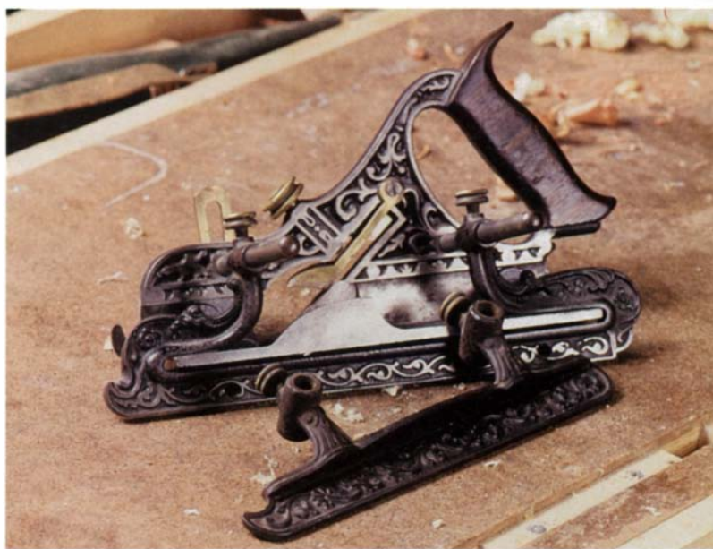
Put together for less than one-fourth the price of a complete plane, this Stanley combination plane is the author's pride and joy. Assembled from parts acquired from flea markets, auctions and tool dealers, this non-original plane makes a perfectly good woodworking tool, even though it's unacceptable to a collector.
