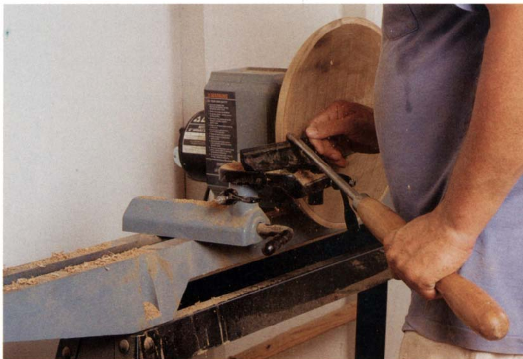
Billed as a home-shop tool, the Delta pivot-head lathe is much more than that moniker might imply. The offset base extension for the tool rest shown above is a necessary optional accessory for off-the-front turning.
