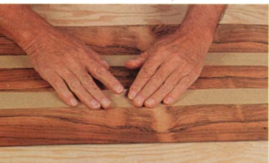
3) Gummed package tape holds the veneers in place
