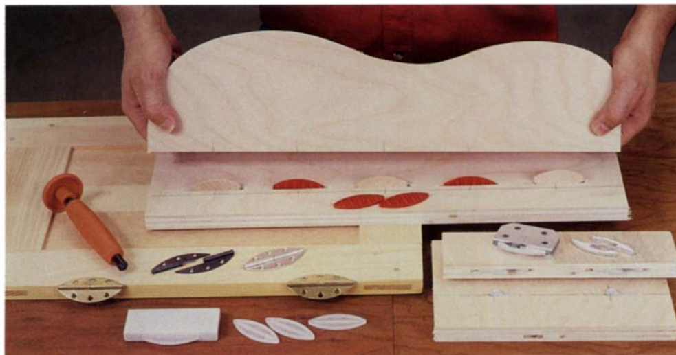
Lamello biscuit-slot hardware (from left): Paumelle hinges with spring-loaded awl for starting screw holes, translucent biscuits for joining solid-surface materials, red K-20 self-clamping biscuits, hook-shaped Simplex knockdown plates with insertion tool.
