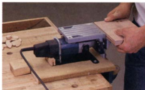
Lamello system includes the Assista slot positioning jig, the Spanbox clamping set and an optional pistol handle for the biscuit joiner. Woodworker's Supply stand (below) converts portable biscuit joiner to a stationary tool.
