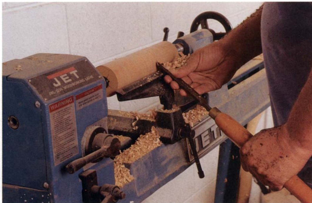
Spindle work is still possible on pivot-head lathes by keeping the headstock in the normal position. The author was impressed with the quality of all the lathes but found he used the Jet the most for his own work, both spindles and bowls.
