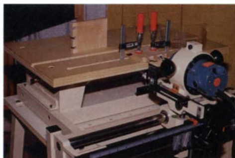
The Stanfield JS-1010 Joiner/Shaper makes many traditional joints and can do some minor shaping too. It costs $1,150. For more information, Stanfield Manufacturing, Inc., 2730 San Pedro N.E., Albuquerque, N.M. 87110; (505) 889-0022.
