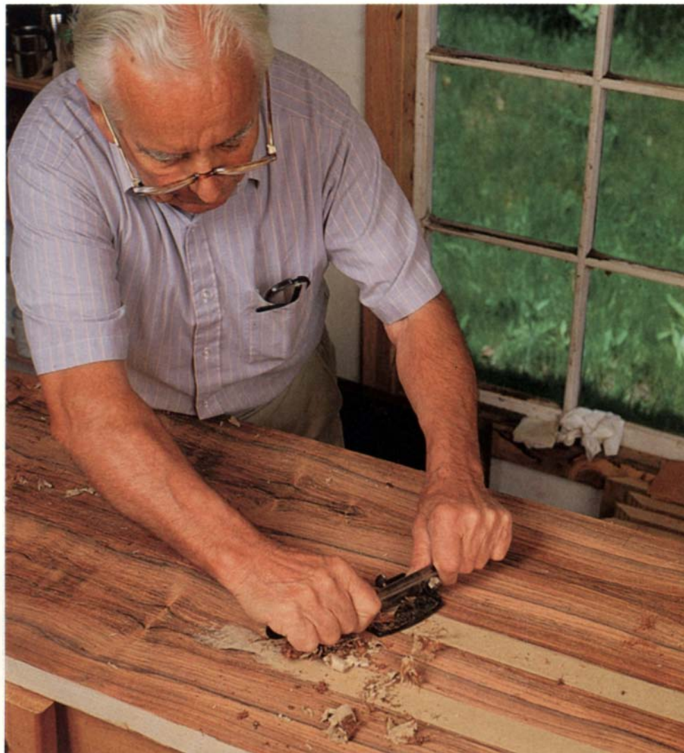
5) Frid scrapes the package tape from the veneer
