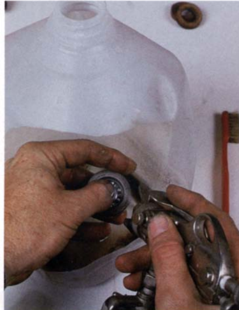
Forty years of dust, dirt and resin had taken their toll on the back blade guides, but they weren't damaged—just frozen. Vaughan removed the bearing from the shaft with two screwdrivers (above), popped the cap off the bearing with a hammer and dowel (left) and sprayed the bearing clean with lacquer thinner (right). The cleaned guide works like new.
