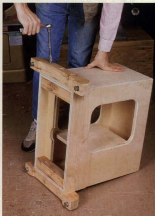
Glued joints are the key to building a good machinery stand, but lag bolts are good insurance against failed joints where the legs meet the carcass. Elaborate joinery isn't necessary for a strong and sturdy stand.
