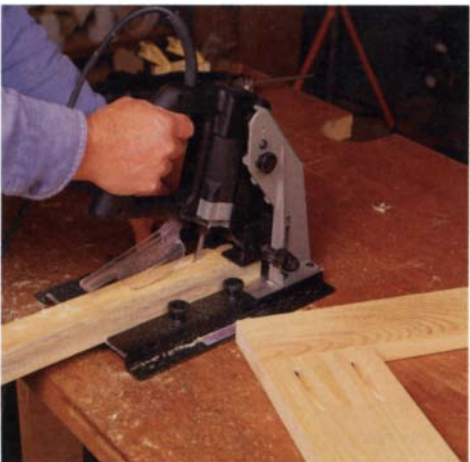
Porter-Cable's Model 550 Pocket Cutter makes quick, strong face frames. It lists for $330. For more information, contact Porter-Cable Corp.
