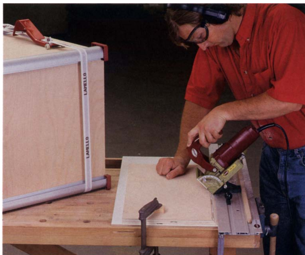
Lamello system includes the Assista slot positioning jig, the Spanbox clamping set and an optional pistol handle for the biscuit joiner. Woodworker's Supply stand (below) converts portable biscuit joiner to a stationary tool.
