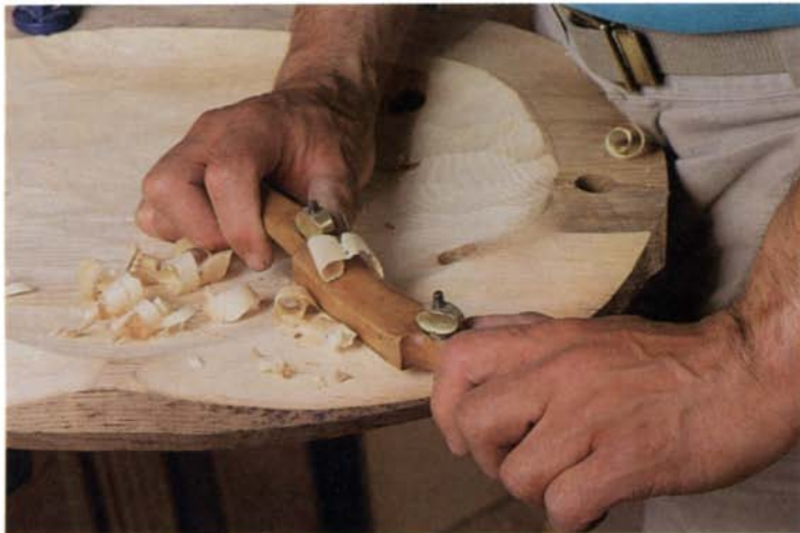
Step 4: Remove gouges and ridges with spokeshaves.
