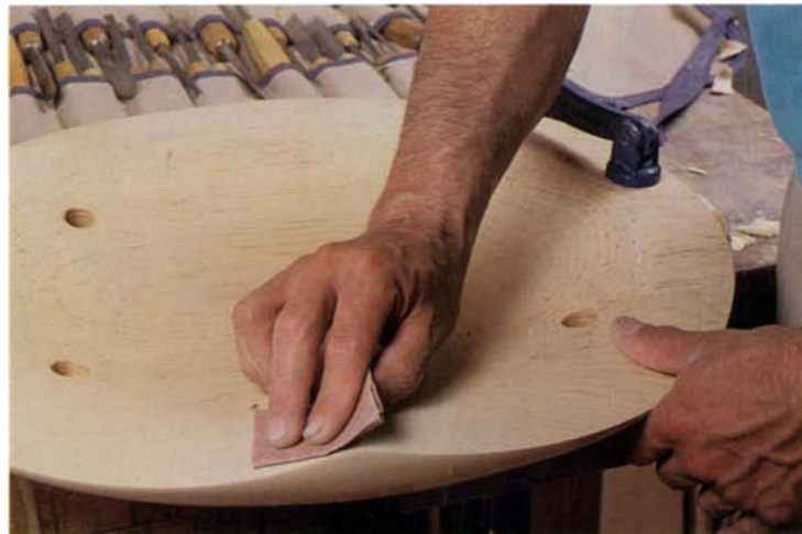
Step 6: Smooth the seat contour with sandpaper.
