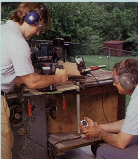
The performance of the plunge routers was compared by timing how long it took each unit to cut through a 12-in.-wide piece of 3/4-in. plywood. Vaughan checks the time while FWW editor Sandor Nagyszalanczy does the routing, monitoring the motor's power draw on an ammeter.
