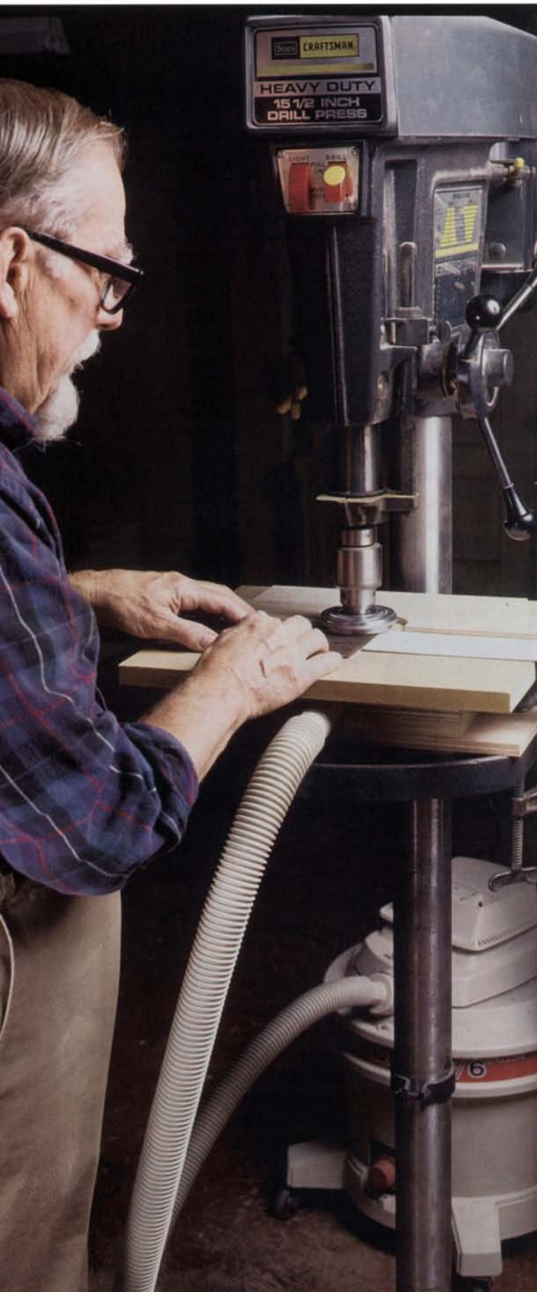
Evan Kern built a vacuum table to hold down thin stock when he's rotary planing with his drill press. To increase the table's suction, he covers holes ahead of the cutter with cardboard. Here, Kern advances the cardboard with a walnut workpiece as he guides it along a fence that's clamped to the table.
