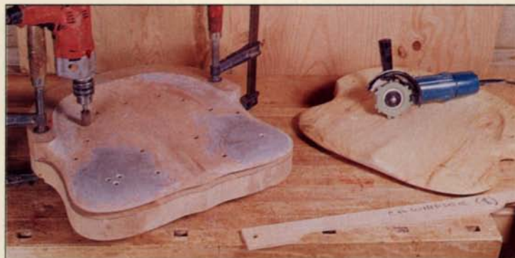
Both Bill Turner and Mac Campbell use depth holes to guide them when roughing out seats. Campbell modified the shape of this pattern (left) several times by adding fiberglass auto-body compound and grinding away wood. As he's carving, he periodically checks the seat's profile with a centerline template.
