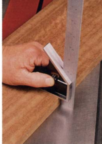
As a depth gauge, the combination square can be used to check the thickness of planed stock, as shown here. The square also can check mortise and dado depths and the lengths of tenons and tongues.
