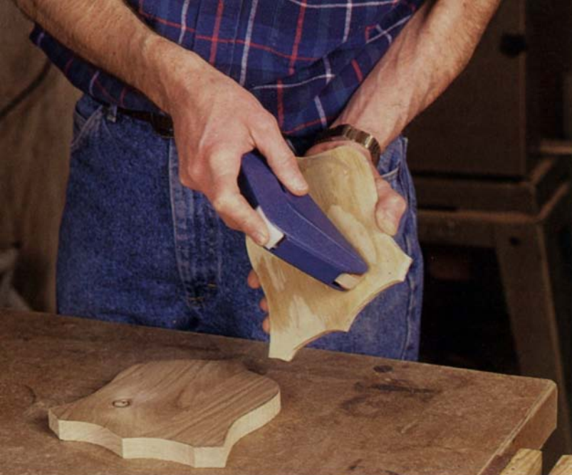
Temporarily attaching a template to a part to be routed is quickly done with a special adhesive tape made by 3M, which dispenses from an applicator like tape but sticks like glue.
