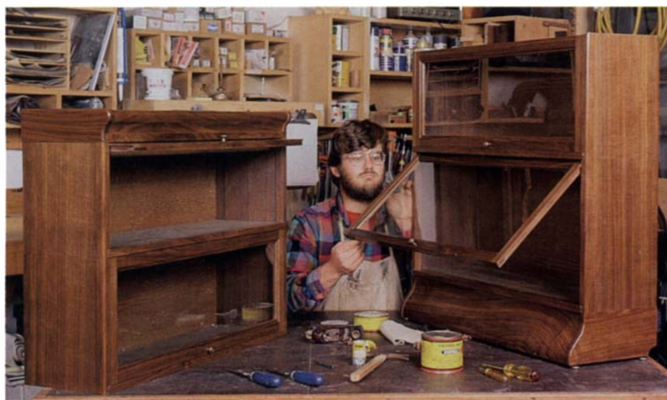
Jeff Greef's walnut lawyer's cabinet resembles a garage for books, complete with overhead doors. A pair of carcass modules capped with a top unit (left) waits to be stacked onto another pair resting on a base unit (right). Greef waxes the back side of one of the retractable doors, which is guided by a simple pulley mechanism that's patterned after the guide system used in the 1906 cabinet in the photo below.
