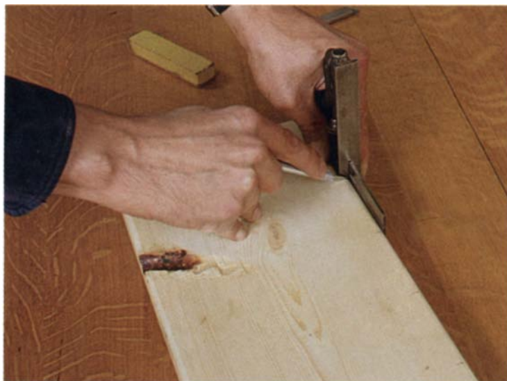
Lay out evenly spaced divisions with the combination square by first setting the square to the desired increment. Then align the rule's end with the starting point, and score a mark at the square's head. Without lifting the knife, move the square along the board, butting the rule's end to the knife blade, and make the next mark at the square's head, as shown here.
