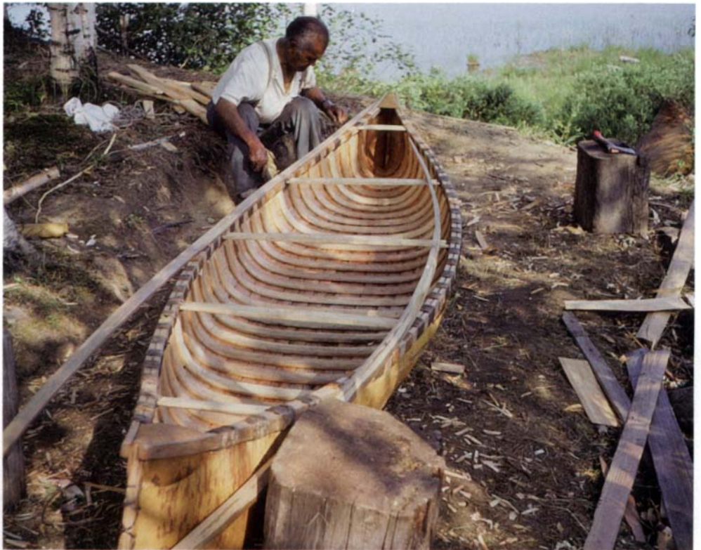
Birchbark-canoe building classes offer a challenging option for a summer vacation. The 16-day class is comprehensive, from harvesting the bark to launching the finished canoe. Here, a student fits the cedar gunwale caps on a nearly completed canoe.
