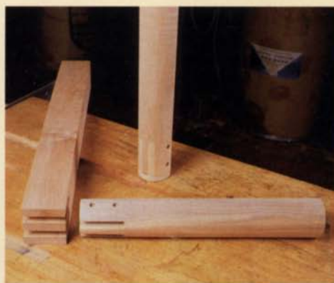
Weiland glues filler blocks and end caps to a leg blank to keep its rail mortises and ends from tearing out during turning. First he cuts mortises in the square leg blank using a tablesaw tenoning jig (left); then he adds the filler blocks and end caps. Once the leg is turned (right), he taps the blocks and caps loose with a hammer.
