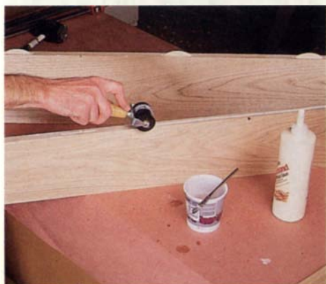
Applying glue with a rubber veneer roller is one way to ensure that the adhesive is spread evenly over the edges to be joined. The small parts brush setting on the water container (foreground) is handy for getting glue into joints, like the plate-joinery biscuit kerfs in the boards shown.
