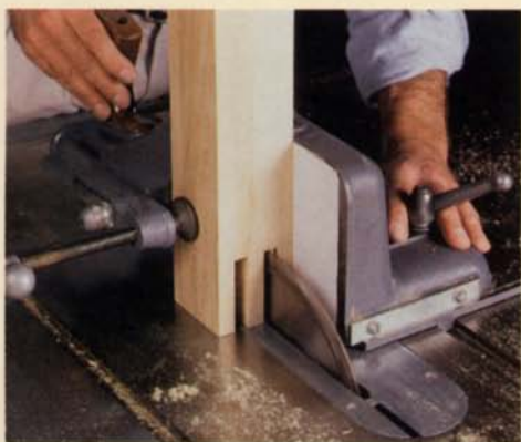
Weiland glues filler blocks and end caps to a leg blank to keep its rail mortises and ends from tearing out during turning. First he cuts mortises in the square leg blank using a tablesaw tenoning jig (left); then he adds the filler blocks and end caps. Once the leg is turned (right), he taps the blocks and caps loose with a hammer.
