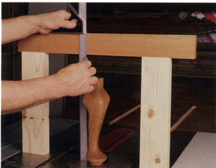
With a set of parallel uprights and a story stick, you can accurately lay out and transfer measurements from irregularly shaped objects. Mark the top edge of the story stick to be sure that it is properly oriented when transferring measurements.
