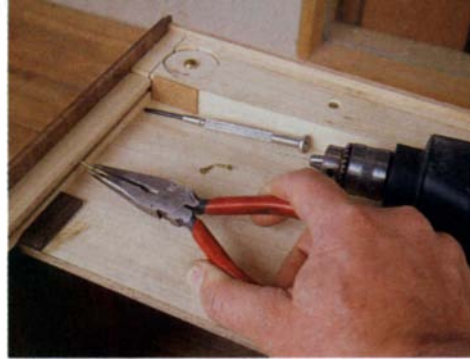
To allow for wood movement in the side of his case, Greef fastens a guide channel by first drilling oversized holes in the guide. Then he installs three screws within the channel using needle-nose pliers and a tiny screwdriver. To complete the door-guide system, he glues a pair of walnut skids at the front of the case and a pair of cork bumpers at the rear.
