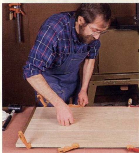
Even clamping pressure ensures uniform squeeze-out of excess glue and a maximum strength bond. To keep dripping glue off his workbench, Minick covers the surface with water-resistant kraft paper.
