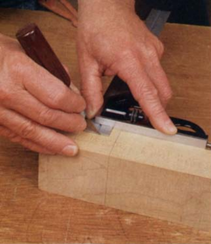
The combination square also can serve as a marking gauge. Simply hold a knife or pencil against the end of the blade while drawing the square's head along the edge of the stock.
