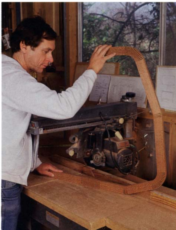
Kerfing a mirror frame: a test strip (above) is cut to determine the number of kerfs needed for the piece to bend into a right angle. This number, multiplied by four, yields the kerfs needed for a closed frame. After kerfing on the radial-arm saw (below), the frame is rolled up to check its shape.
