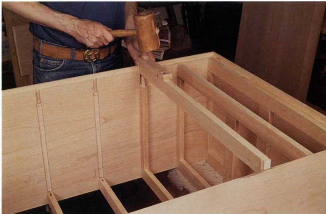
After installing the front drawer dividers and runners, the back dividers are slipped onto the runners' back tenons and glued into dovetail slots in the carcass. The runners' front tenons are glued, but not the back, to allow for movement of the carcass sides.
