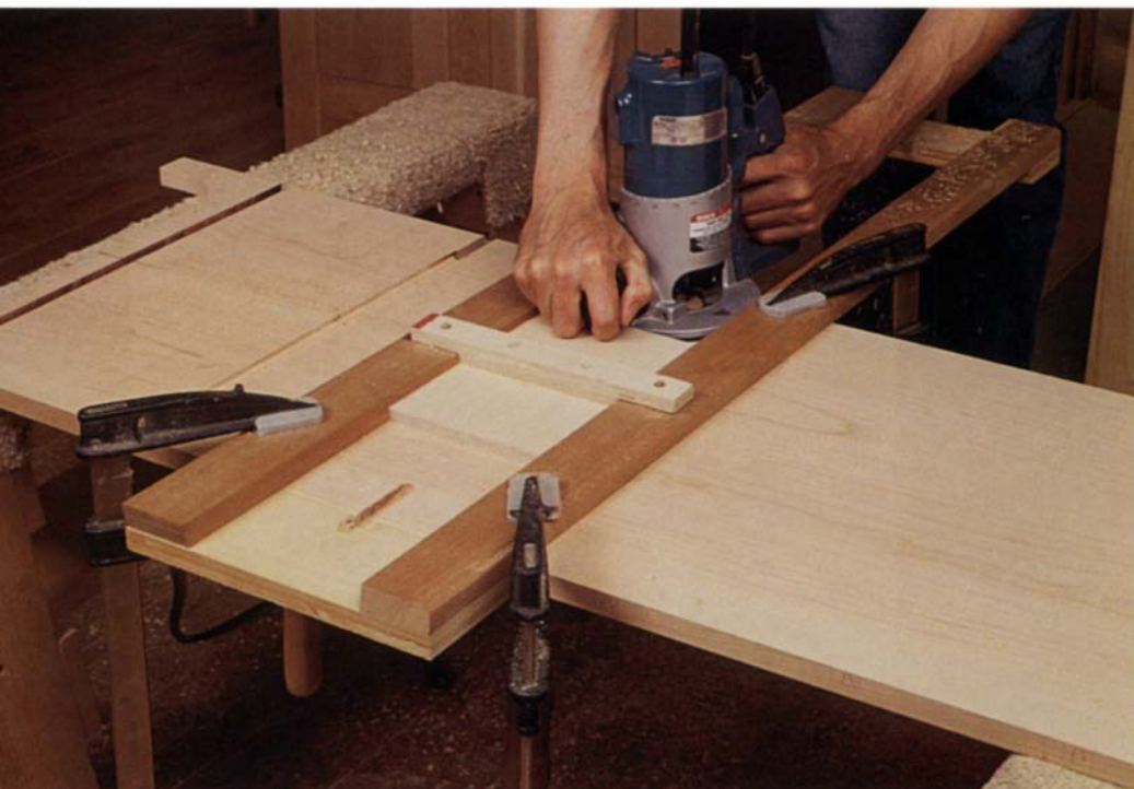
Becksvoort routs the dovetail slots for the drawer dividers with a jig that traps the router base. After routing both dovetail slots, he removes the jig's center stop, changes to a router with a straight bit and cuts the dado between the slots for the drawer runners.
