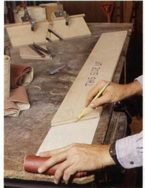
A pattern stick makes it easy to consistently cut abrasive strips to the correct length with uniformly angled ends. Angling the ends reduces bumping when the glued joint contacts the workpiece.
