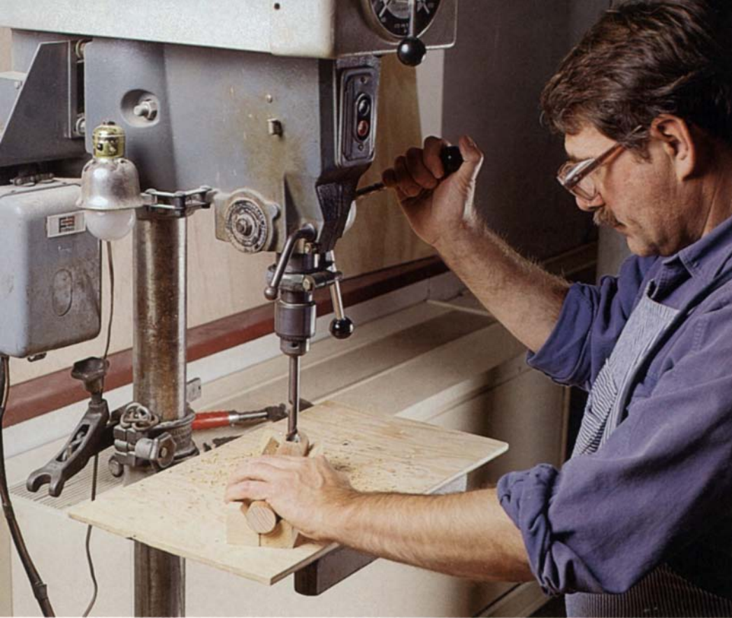
When boring angled holes for splayed legs, Maas uses ramps like the pair in the foreground (above). A pocket-hole fixture (left, background) makes sloped (75°) holes for recessed screws. The steel vise (right, background) serves as a tilting table, which can precisely hold small pieces.
