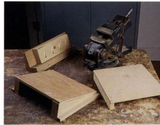
When boring angled holes for splayed legs, Maas uses ramps like the pair in the foreground (above). A pocket-hole fixture (left, background) makes sloped (75°) holes for recessed screws. The steel vise (right, background) serves as a tilting table, which can precisely hold small pieces.
