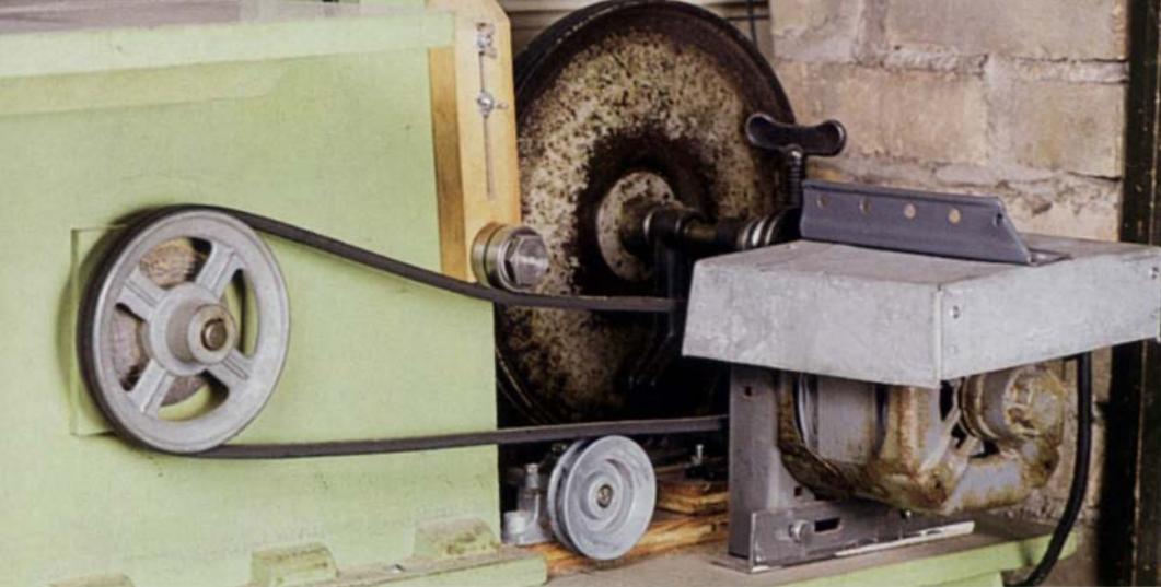
A motor recovered from an old washing machine powers the author's shopmade bandsaw. Because the 1/2-HP split-phase motor had no base, angle-iron brackets were built to mount the motor to the saw.
