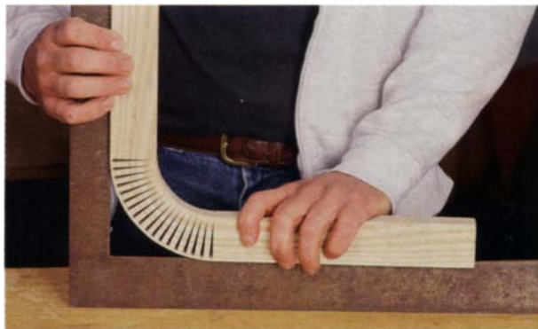
Kerfing a mirror frame: a test strip (above) is cut to determine the number of kerfs needed for the piece to bend into a right angle. This number, multiplied by four, yields the kerfs needed for a closed frame. After kerfing on the radial-arm saw (below), the frame is rolled up to check its shape.
