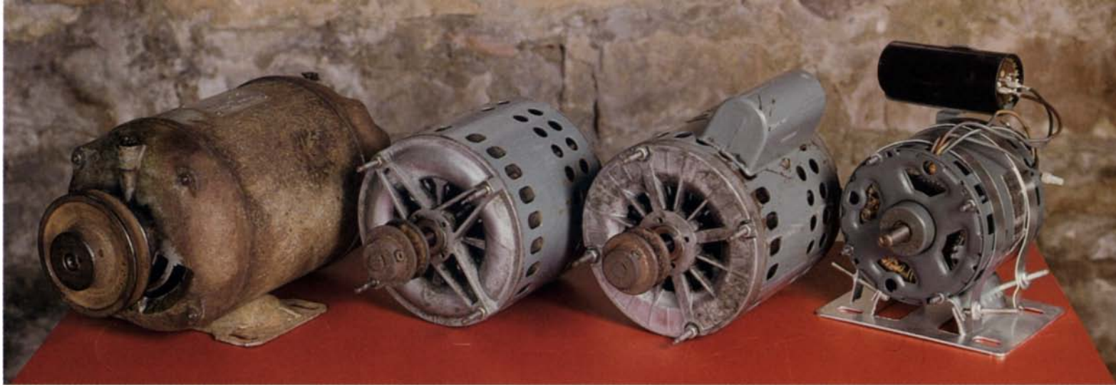
The different types of motors you're apt to find include (from left to right): the repulsion motor, a high-starting-torque AC motor with brushes; the slow-starting split-phase motor, commonly used
