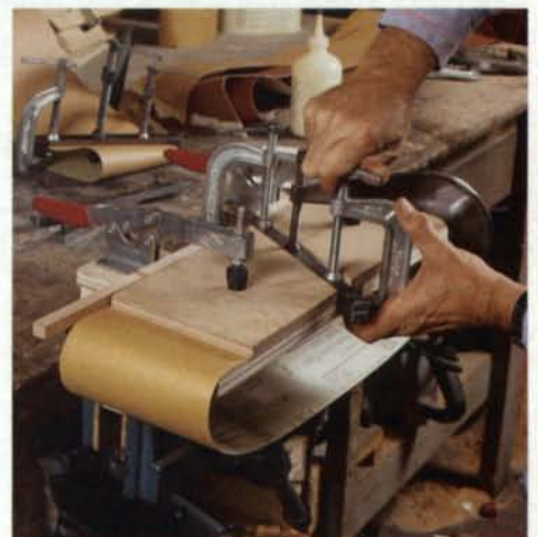
The gluing fixture aligns the belt while the lap joint is being clamped. Multiple steel pads permit the removal of one belt from the fixture to glue up others.
