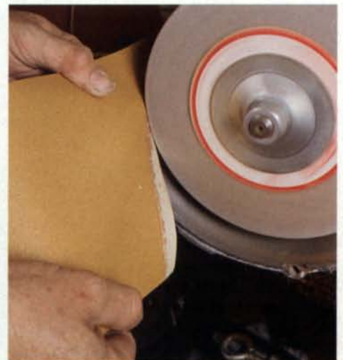
Grinding away the abrasive cleans up the belt for gluing the lap joint and makes for a thinner glueline and smoother running belt.
