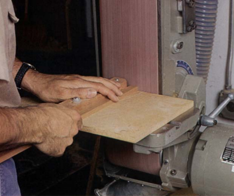
The author built two sliding tables: one with a 90° fence and one with a pair of 45° fences for accurate end sanding. The tables ride in the miter-gauge slots.
