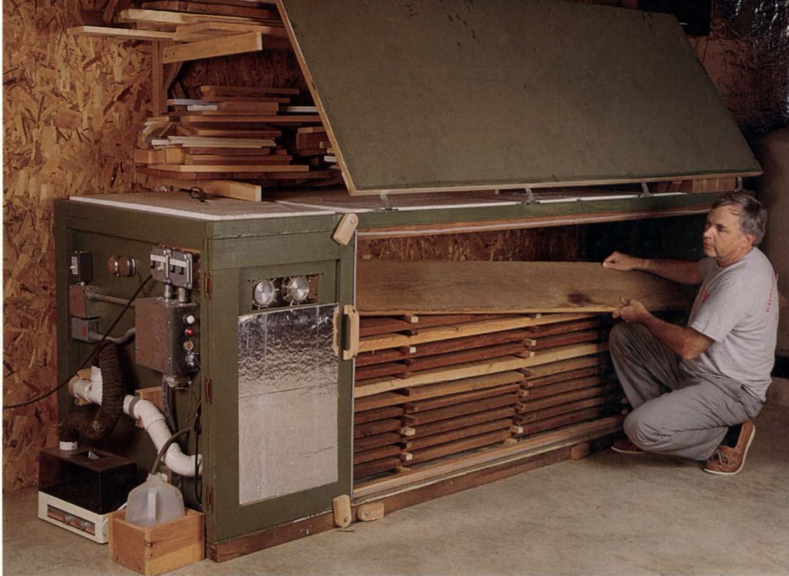
The author loads his kiln before shutting its airtight door and turning on the automatic dehumidifier and low-temperature heater. His kiln runs automatically, but shuts off and rings a bell if the air in the chamber gets too hot.
