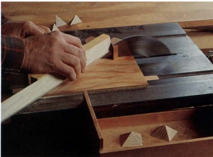
The author crosscuts with a diagonal-fence jig that slides on a runner in his table saw's miter groove. Both sides of the fence and two stop blocks are used when cutting stock into pyramids.
