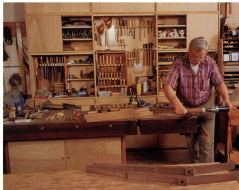
Portable benches and a portable shop-built router table allow John Nyquist to make flexible use of his shop space. His workbench sits between the cabinets that hold his hand tools and portable power tools and a 4-ft. by 12-ft. assembly table.
