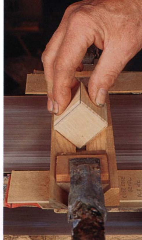
Coffin devised a simple chamfering fixture that he clamps on his stationary belt sander to consistently bevel block edges. The V-shaped cradle holds the blocks (half-blocks fitted temporarily into minicubes) at 45°.
