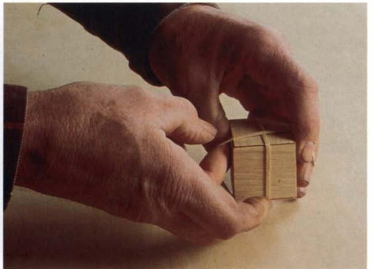
Rubber bands clamp the glued-up half-blocks, and the first half-block (with waxed inner surfaces) becomes a gluing fixture. Waxed paper over the corners prevents accidentally gluing joints.
