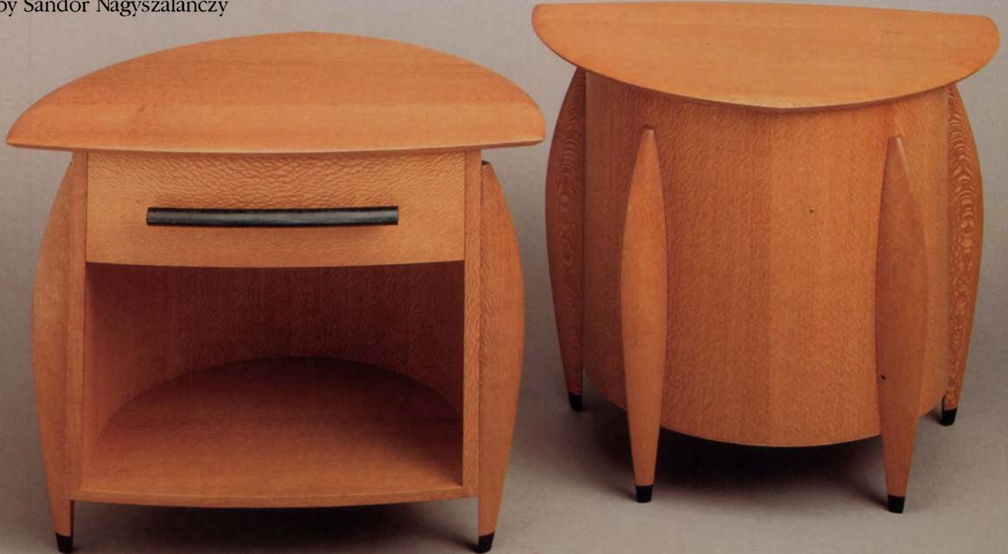
These 24-in.-high side tables, by Oakland, Cal., woodworker Colin Reid (nicknamed the "Batrille Tables"), employ a lacewood-veneered carcass built from 1/2-in. plywood and solid-lacewood parts. The drawer pulls and foot tips are ebony.
