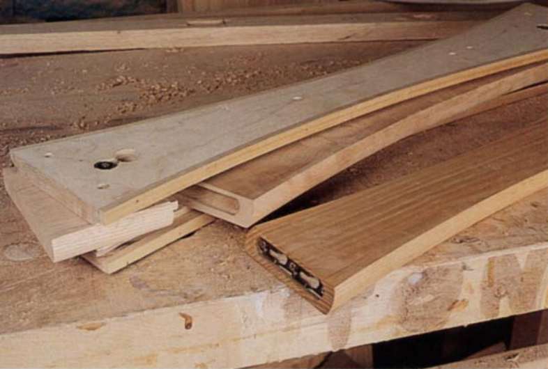
Shaping the curved edges —The author sandwiches a stretcher between two templates to shape its curved edges in one pass. Either template can follow the shaper's guide bearing. Note the knockdown hardware screwed into the stretcher's mortise.
