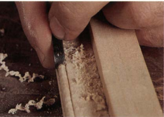
Cutting the bead with a scratch stock made by filing a piece of tool steel to the desired shape imparts hand-crafted quality to the piece. A sawkerf helps establish a uniform shoulder before final shaping.
