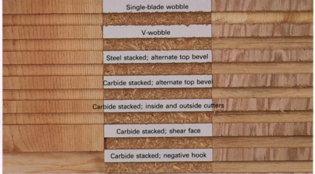
Tearout is common on cross-grain work. From left to right are solid pine, melamine-coated particleboard and oak-veneered plywood. The author found little or no tearout with any of the blades on Eastern maple and less on birch plywood than on the oak.
