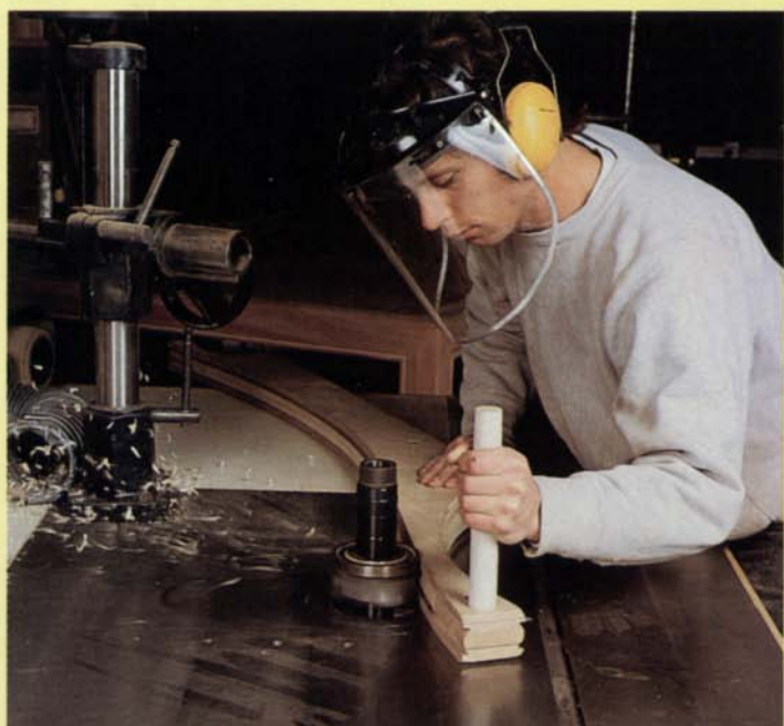
Safety measures —Bivona inserts a dowel handle into a hole in the narrow end of the leg's template jig to keep his fingers clear of the shaper cutter. His right thumb is hooked over the jig's edge to keep that hand from slipping. (Guard removed for photo.)
