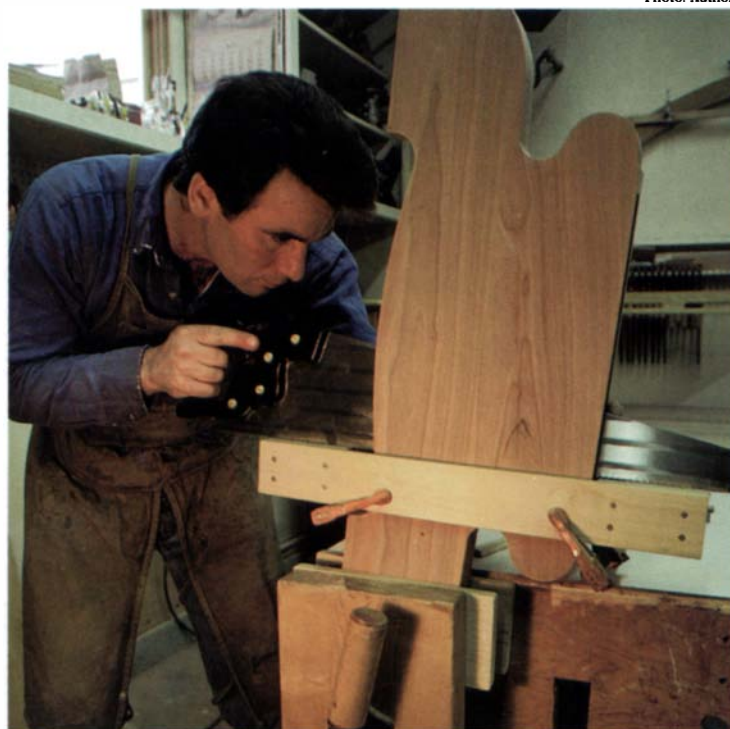
To enlarge the trestle-base mortise for the wedged tenon, Dunlap clamps a guide to the base at the wedge angle and cuts until the sawteeth touch the blocks at the ends of the guide. After sawing along each side of the mortise, he chisels out the waste.
