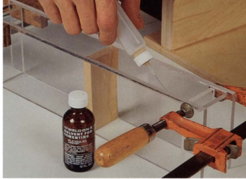
With the Lexan guard parts clamped together, Mebler squeezes one-minute cement into the joints. The ends of the guard's sides slide into dados in the box's fence and back support.
