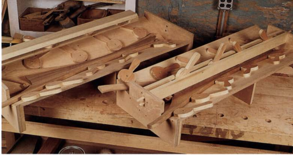
Gluing up the stands —jigs fitted with cam clamps are used to glue up mirror stands (left). On the left, a pair of legs registers against stops at each end and cam clamps press them together; on the right, clamps, held in place with dowels, press the center piece down.
