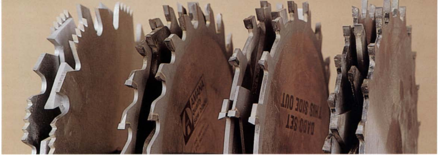
Stacking dado blades aren't all alike. Shown above are, from left to right: a high-speed steel set; a typical carbide-tip set; a carbide set sharpened with a beveled, or shear, face and a slight top bevel; and a carbide set with a reverse hook angle on its teeth.
