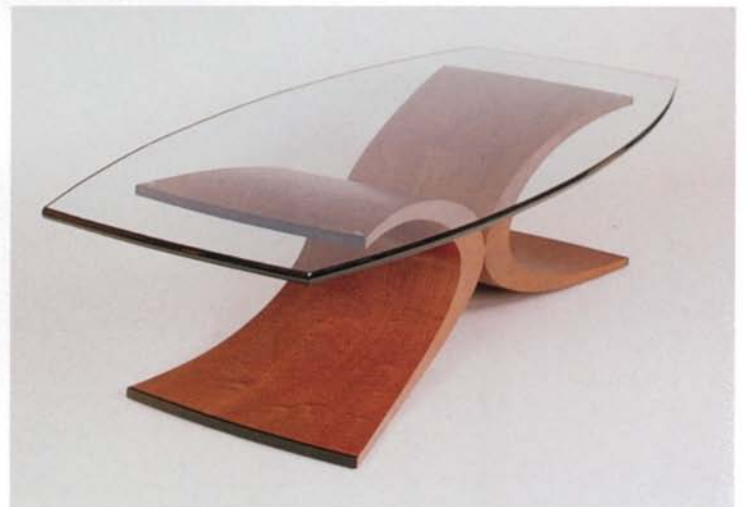
The base of Mason Rapaport's 60-in. by 30-in. glass-top coffee table , above, was built from four layers of \frac{1}{16} -in. Baltic birch plywood, vacuum-pressed over an armature of U-shaped plywood ribs and veneered with quilted African mahogany.
