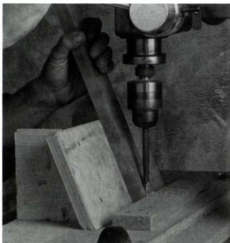
The angled pockets for the face-frame assembly screws are drilled with a special shallow-angle countersink bit and with the frame member held 22½° from vertical on a shopmade jig.
