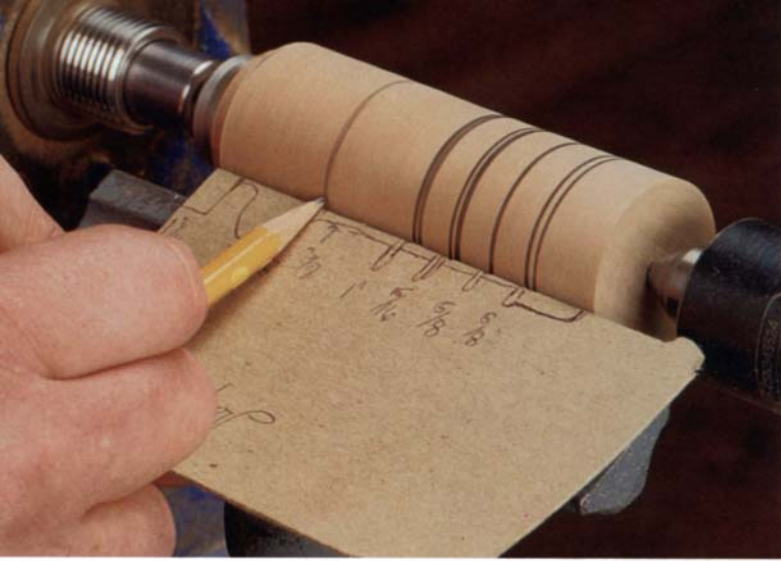
To lay out each chess piece, the author holds a cardboard pattern up to the turning blank, above, and uses a pencil to transfer key features. The blank is held in a screw chuck on the lathe.
