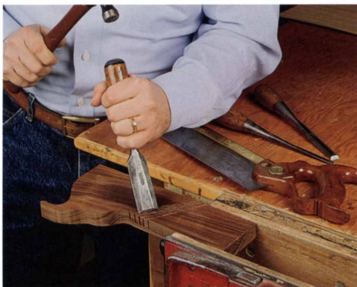
Carving out the tapered wedge slot was easy because the body is laminated. After using a backsaw to cut kerfs to depth on the mating pieces of morado and cherry, Barker chisels out the waste.
