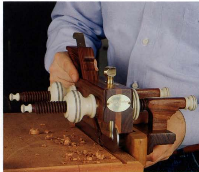
Wooden plow planes, with their adjustable fences and interchangeable blades for cutting various grooves, were the forerunners of metal combination planes, such as the Stanley #45. Fancy plow planes were made from exotic woods and detailed with precious materials. The author used Du Pont Corian in place of ivory on his reproduction plane shown here.
