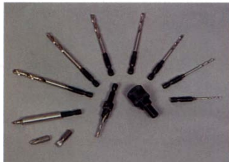
Insty-Bits make it easy for you to change bits without fumbling for a chuck key. Pushing the lock ring lets you slip a bit in and out of the chuck, while a groove on the shank locks the bit in place when the ring is released.
