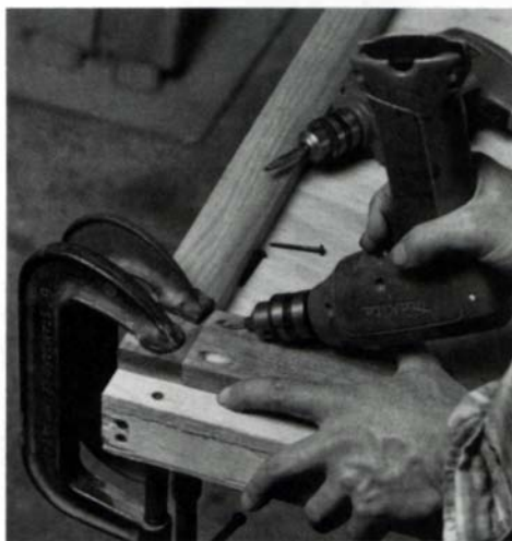
When joining the face-frame parts, Tolpin double-clamps one of the solid-stock workpieces securely to his bench to counter its strong tendency to slide out of flush as the screws are driven home.
