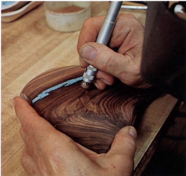
Favorite outlines the area to be inlaid with a fine burr, and then bogs out the waste in the middle with a larger bit. It requires a steady hand to maintain a depth of cut that will leave the silver just slightly below the surface of the wood.
