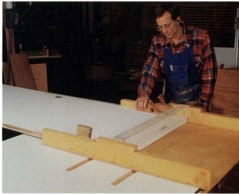
To demonstrate the capacity of his wide cutoff box, Mebler trims the end of a 30-in. paneled door. A wedge between the door and support presses the workpiece against the fence.
