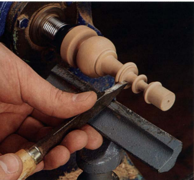
Mode's shopmade skewed parting tool (below) cleanly cuts the column of each piece without damaging the delicate discs.
