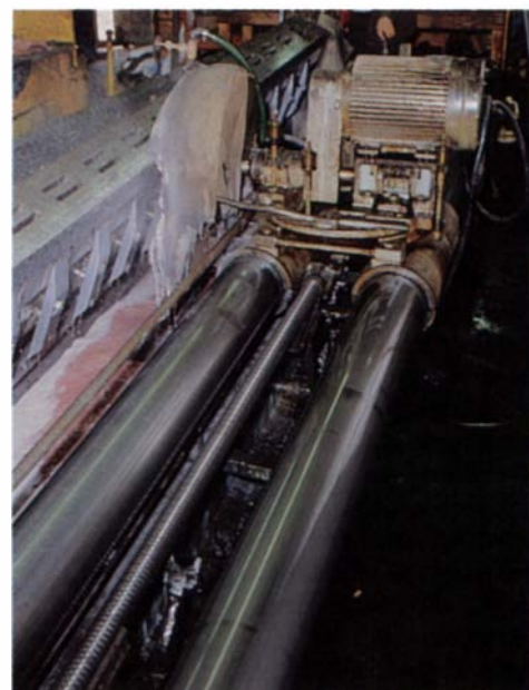
The veneer slicer's 16-ft.-long blade must be sharpened every day of use. First, the special knife grinder shown here regrinds the edge as the machine travels along huge, precise guide rails. Then the blade is honed using two hand-held slip stones.
