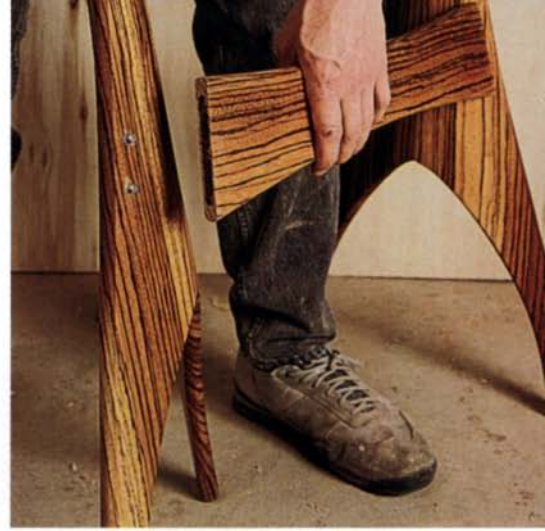
Attaching the stretcher to the legs —After hooking the stretcher's keyhole clip on the heads of shoulder screws in the back leg (right), Bivona will push the stretcher down to lock it against the leg. An awl poked through the shaping jig marks for the screws.
