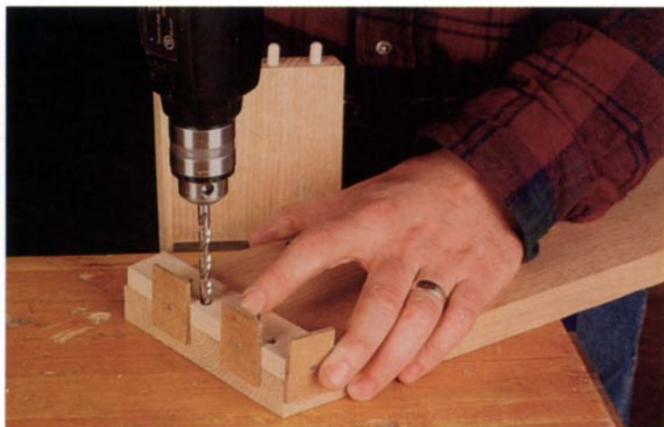
This jig guides the bit for drilling dowel holes, and serves as a depth gauge when setting the dowels. Be sure to position the cleats against the outside and back edges of the workpiece.
