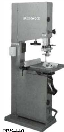
PBS-440 BANDSAW $1,395. Designed and made in Europe. 16" throat. 11" depth. Table tilts to 45° angle. Rip fence included. Cast iron table. Other models from 14" to 36" throats.
