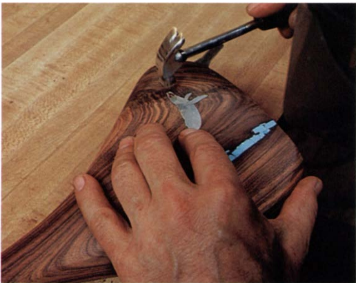
The silver inlay is glued into the routed recess with a couple of drops of cyanoacrylate adhesive and then gently tapped into place. Do not overheat the silver when sanding or buffing the piece or it will expand and pop out.
