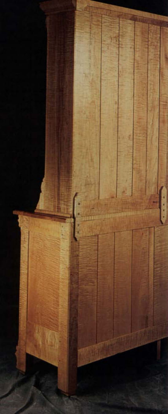
The back of the hutch is finished so that it doesn't need to be up against a wall. Wood brackets secure the upper carcass to the lower carcass.
