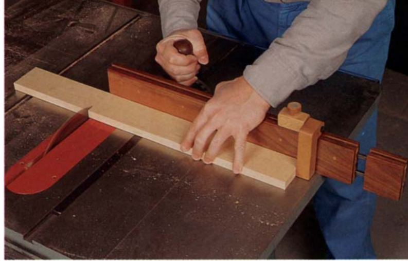
This shopmade miter gauge fence expands a tablesaw's crosscutting capacity and accuracy, and provides a drop stop for repeat cuts.
