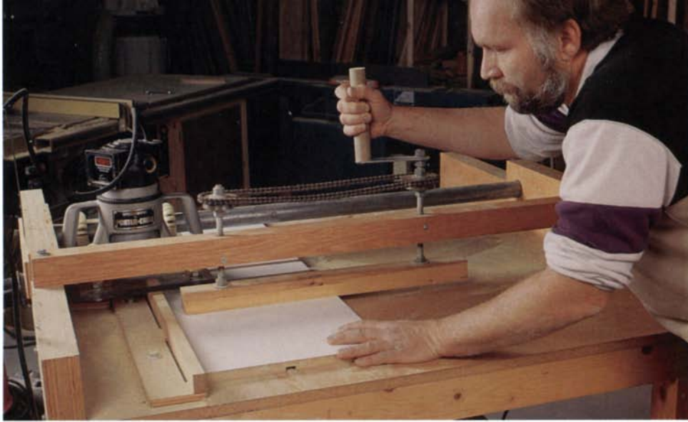
Left: To keep sheet goods steady during routing, the author built a special hold-down clamp; two threaded rods, connected by gears and chain, raise or lower a clamping bar via a crank on top. Above: By locking the router carriage in place with two wing-nut-tightened stop blocks, the author can run sheet materials through the panel router for lengthwise cuts.
