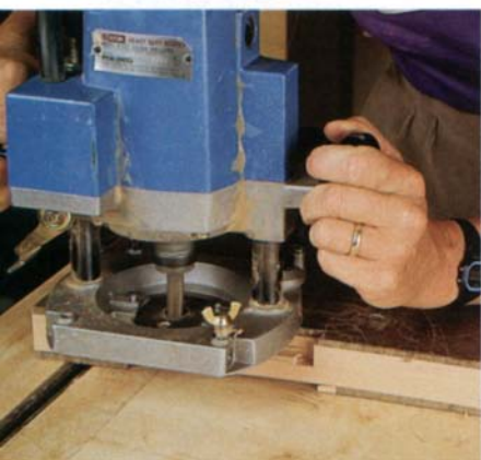
Left: Ames cuts a pocket for the drawer case with a leg mounted in a router jig, setup with a mortising bit and a guide collar screwed to the base. The leg's concave curve has been flush-trimmed in a similar jig, but without pocket cutouts. Above: The shelf-rail mortise is drilled with the leg still mounted in the pocket-routing jig. The jig's back is plumb relative to the curve of the finished leg, which ensures that the holes will be drilled at the correct angle.
