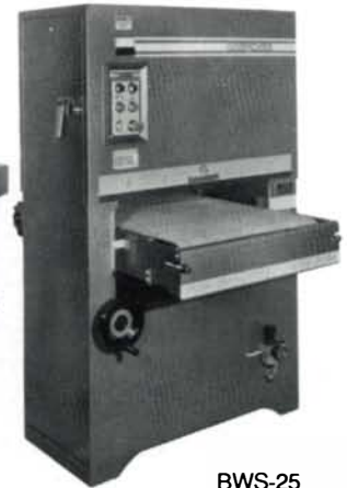
BWS-25 WIDE BELT SANDER $6395. Sands stock 25" wide by 5 7/8" thick. 10 HP 3 phase main motor. Fixed Feed Rate of 15'/minute. Other models from 13" to 37" wide, fixed and variable feed rates.
