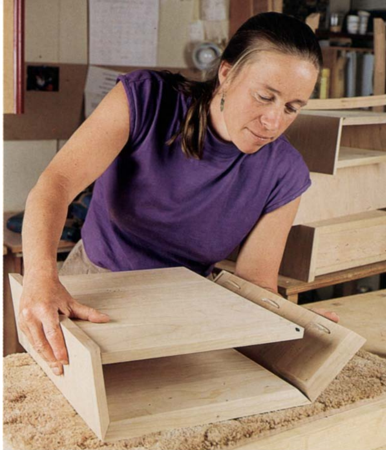
Above: After applying strapping tape across the case's top-to-side miter joints, Ames flips over the taped up parts, brushes glue on the joints, folds the sides up and inserts the splines into the slots in the bottom's edges. A few lengths of tape stretched from side to side across the bottom will provide adequate clamping pressure. Below: After gluing the mitered drawer body together, Ames cuts the grooves for the corner splines with a jig that holds the drawer at a 45^\circ angle to the saw table and rides along the rip fence.
