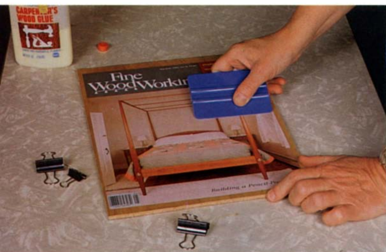
After rolling glue onto the plywood backing, Williams mounts the picture, smoothing from the center to the edges to eliminate air bubbles. For pictures printed on heavy paper, which tends to curl at the edges, she clamps the edges for 10 or 15 minutes.
