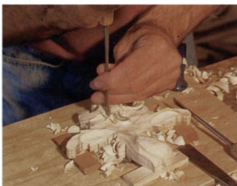
Left: Bacon uses a setting-in cut to form a vertical wall around the central leaf. He then carves up to the wall to create a flat area that will be the top of the trefoil molding (right).
