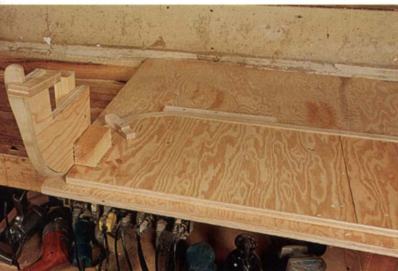
The settee bow bending form is a simple system of blocks and cleats mounted on a ¾-in.-thick plywood base that can be secured with the dogs on a workbench. The ends of the bow are secured by U-shaped pieces of plywood, which can be slipped on faster than clamps. Cleats and rotating blocks also save time, so the steamed bow can be secured before it cools.
