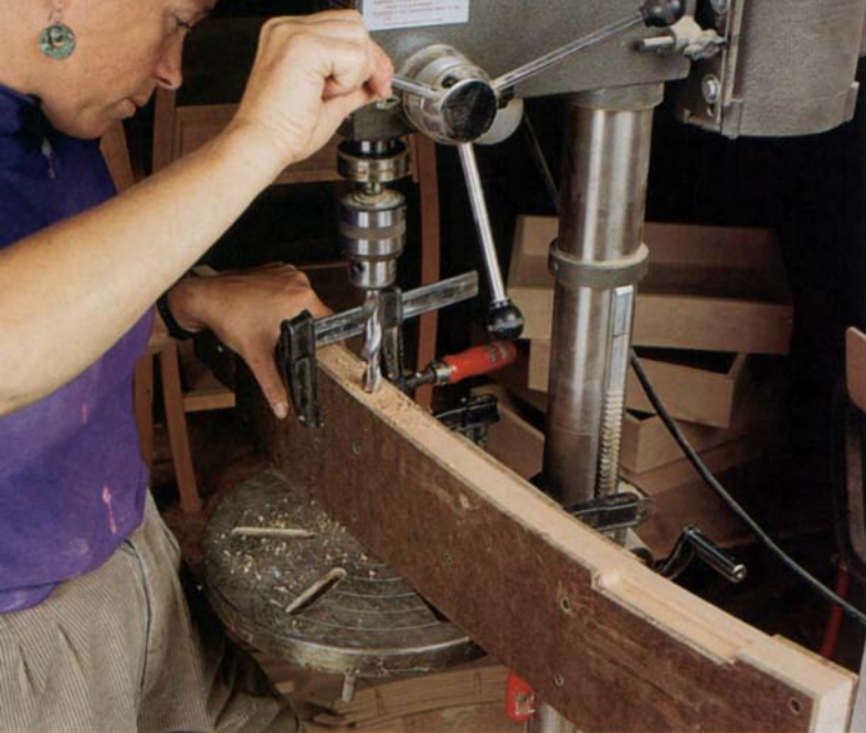
Left: Ames cuts a pocket for the drawer case with a leg mounted in a router jig, setup with a mortising bit and a guide collar screwed to the base. The leg's concave curve has been flush-trimmed in a similar jig, but without pocket cutouts. Above: The shelf-rail mortise is drilled with the leg still mounted in the pocket-routing jig. The jig's back is plumb relative to the curve of the finished leg, which ensures that the holes will be drilled at the correct angle.
