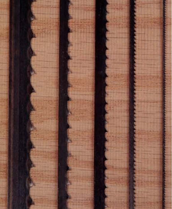
Above: Although hundreds of blades are available, Duginske uses only five for the majority of his bandsawing jobs. The blades are, from left to right: a 1/2-in., 3-t.p.i. hook tooth; 1/4-in., 4-t.p.i. skip tooth; 1/4-in., 6-t.p.i. hook tooth; 1/8 in. 14 t.p.i.; and a 1/16 in. 24 t.p.i. Right: A 1/16-in. blade's ability to make extremely tight turns and produce an exceptionally smooth cut make it ideal for intricate patterns, like this maple leaf Duginske is sawing from walnut.
