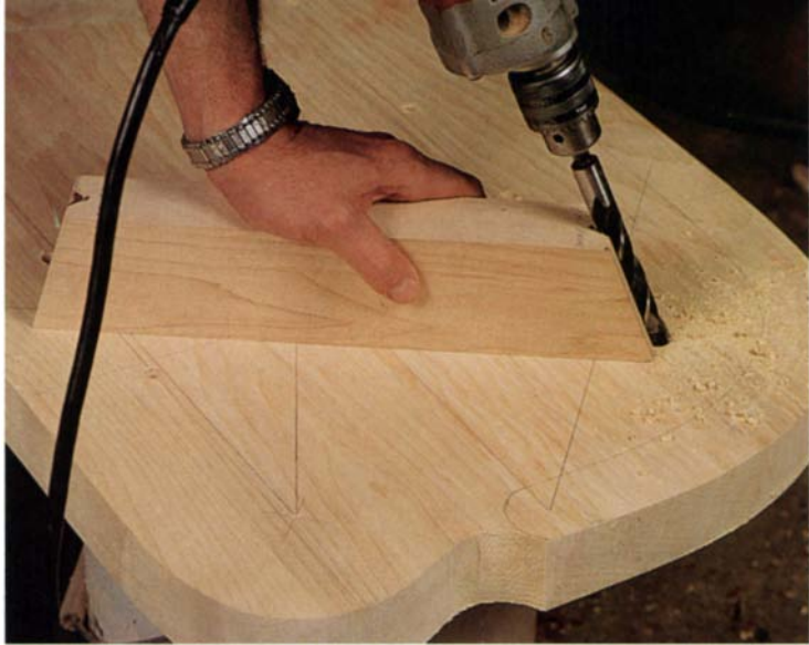
The leg and stump holes are bored from the top down, so any tearout is hidden on the bottom. The drill is guided by a notched scrap of 2x3x8 hardwood, crosscut on one end to the desired angle. Pencil lines drawn on the seat indicate the direction in which the angled legs lean.
