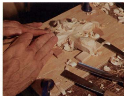
Left: Bacon uses a setting-in cut to form a vertical wall around the central leaf. He then carves up to the wall to create a flat area that will be the top of the trefoil molding (right).
