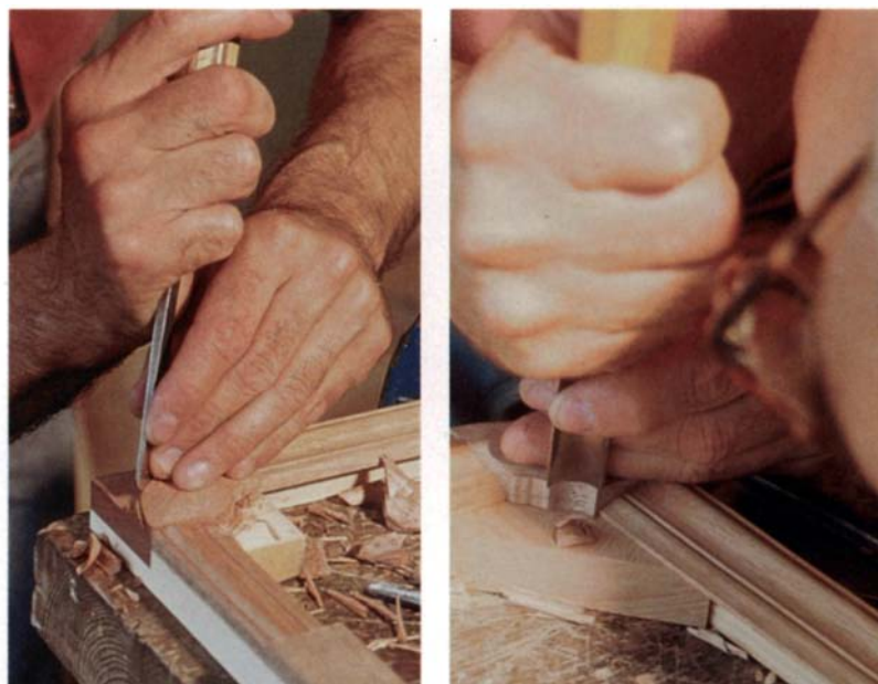
Left: After planing the mahogany block level with the moldings and then drawing the shape of the scalloped corner onto the block using a cardboard template, Bacon lowers the outside corner to the same level as the surface of the fretsawn veneer sections that will be attached after the corners are carved. Right: Carefully controlled vertical cuts with the appropriate gouge form inner and outer profiles that guide a viewer's eye smoothly around the frame's corners.
