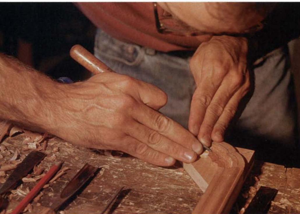
Above: The line of the quirk is drawn across the corner (a pair of dividers keeps the spacing right), and then the quirk is carved with a parting tool. Top, right: Following the quirk, Bacon forms the hollow of the lower ogee with a #8 gouge. Bottom, right: After lowering a step behind the high point of the upper ogee and cutting in the quirk with a parting tool, Bacon rounds the tops of the ogees and bead behind the upper quirk with a back-bent gouge.
