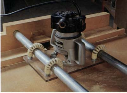
Above: The router carriage is made from clear polycarbonate, held by four U-bolts ringed with plastic rollers cut from delrin tubing. Right: The laminated-plywood sides support the steel tubes that guide the router carriage and the beam for the hold-down clamp. Slotted holes allow the sides to move up and down, and one side has a hole for vacuum hose connection.
