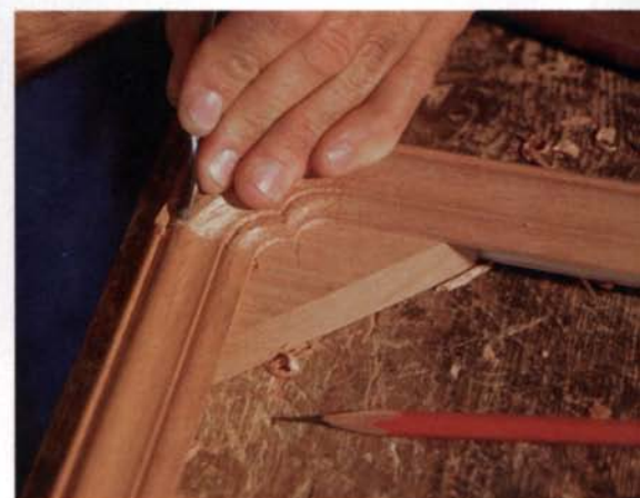
Above: The line of the quirk is drawn across the corner (a pair of dividers keeps the spacing right), and then the quirk is carved with a parting tool. Top, right: Following the quirk, Bacon forms the hollow of the lower ogee with a #8 gouge. Bottom, right: After lowering a step behind the high point of the upper ogee and cutting in the quirk with a parting tool, Bacon rounds the tops of the ogees and bead behind the upper quirk with a back-bent gouge.
