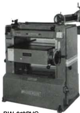
BW-612PVG PLANER $6,895. Planes 24" wide by 9" thick. Top & bottom rolls drive 10 HP US Main Motor. Other models from 12" to 24" wide.
