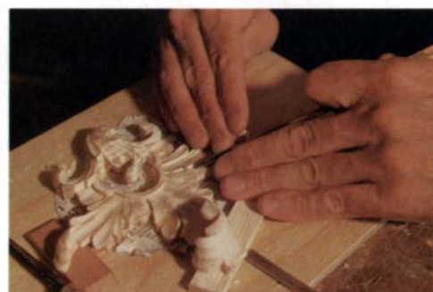
Left: After establishing a wall around the trefoil and then piercing all the way through within this wall, the author begins to refine the leaf details. Here he carves the individual leaf tips. Once the flowing, tapering hollows of the leaves are carved with various gouges, Bacon uses fine fluters to carve within the broad hollows (right). The narrow flutes must follow the flow of the larger hollows and run together as they reach the trefoil wall.
