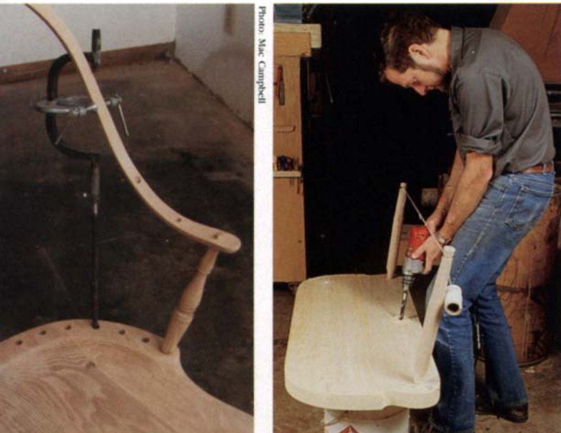
Left: Fanning the spindles out evenly causes the third spindle on chairs, shown here, and the fourth spindle on the settee to pierce the back bow diagonally from corner to corner, making the bore difficult to bore. So Campbell fabricated this guide from metal tubing, rod and a C-clamp. Putting the bottom rod into the seat bore makes it easier to align the bow bore. Right: To align the middle legs with the outside legs, Campbell stretches a string between the two outer legs and uses it to sight the hole with a hand-held power drill.
