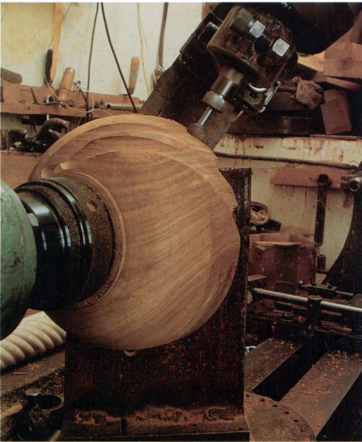
Above: For cutting exterior radial reeds, the author mounts the router vertically on the beam's high platform. The beam rotates on the baseplate pivot pin and depth of cut is adjusted with the slide rest. Below: The author routs angled flutes using the swing fixture. The router is pivoted via the swing arm, which is bolted through a bushing to the vertical section of a large U-beam that is in turn bolted to the compass fixture's baseplate.
