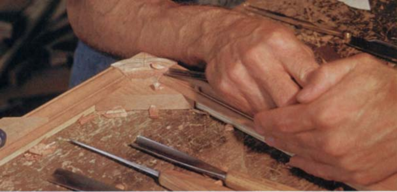
Working diagonally across the block, Bacon uses a gouge to carve out the molding's dominant curve.
