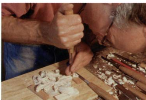
Left: After establishing a wall around the trefoil and then piercing all the way through within this wall, the author begins to refine the leaf details. Here he carves the individual leaf tips. Once the flowing, tapering hollows of the leaves are carved with various gouges, Bacon uses fine fluters to carve within the broad hollows (right). The narrow flutes must follow the flow of the larger hollows and run together as they reach the trefoil wall.
