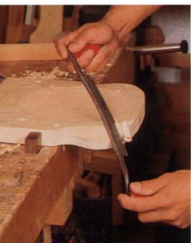
Above: Rodriguez scoops out the saddle with an inshave. Since the tool's long, angled handles prevent him from cutting steeply into the seat, he'll finish around the back edges with a wide gouge. Left: The author carves the front of the seat with a drawknife. He shaves to a line that is marked on the middle of the edge and that curves around the sharp corner where the top rolls over. Below: Rodriguez steam bends the combs for about 45 minutes in a closed plastic pipe connected to a wallpaper steamer. Then the combs can be wedged against forms on his plywood bending fixture.
