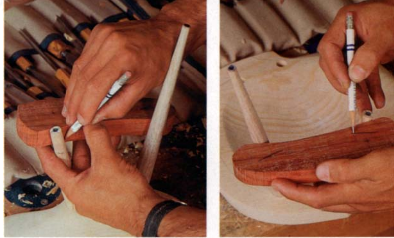
Left: Before drilling the armrest for the back posts and arm posts, the author holds it in position and marks the edge where each post will meet it. Then he sights the direction to point the drill, where each post appears plumb, and marks direction lines on the top of the armrest (right).
