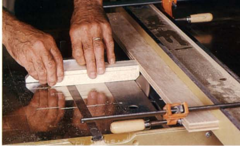
Above: An elevated guard attached to a standard tablesaw fence shields the blade from Brandli as he cuts corners off edging components. The cutoffs fall safely out of the way under the guard. Right: It's easy to bore holes into the ends of box components with this simple jig, which is made from an L-shaped plywood stand screwed to a base that can be clamped to a drill press table. Below: Rather than risk ruining a box frame by flattening it on a belt sander, the author trues the surface by repeatedly running it over sandpaper glued to a sheet of particleboard. The box is kept flat on the table and advanced at a slant.
