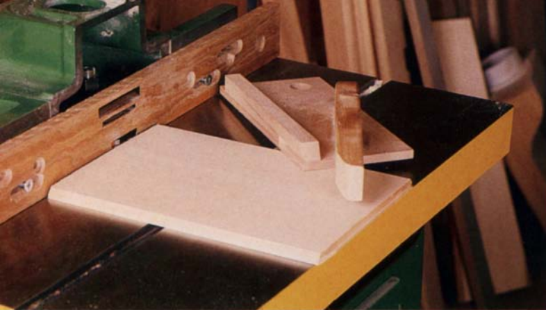
When working with power tools, Brandli uses several simple jigs and fixtures to speed production, ensure accuracy and keep fingers out of danger. This device serves as a backing board to push a workpiece past a shaper cutter. The arm on the top holds the piece snugly down on the table. The dimensions of the holding jig depend on the type of machine you're using.
