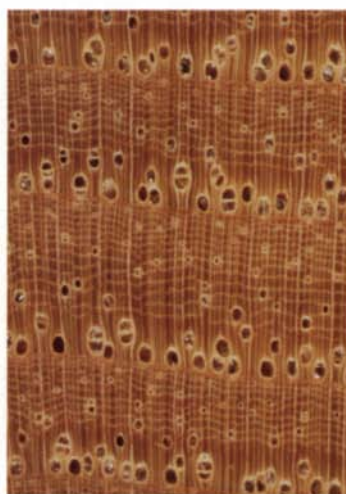
Shagbark hickory is ring-porous and distinguishable from pecan by an abrupt transition from earlywood to latewood and by thin bands of parenchyma that cross its rays only in the latewood.
