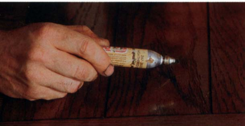
Grain patterns and lines can also be simulated with magic markers or special finisher's markers.
