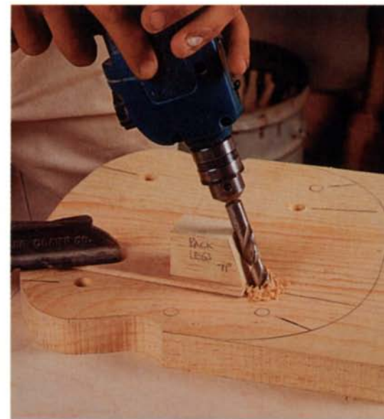
To drill through-sockets in the seat, for the legs and posts, the author uses a guide block to set the drill angle and points the drill bit in the direction of lines marked on the seat. He marked the direction lines and socket centers from a plywood seat pattern.
