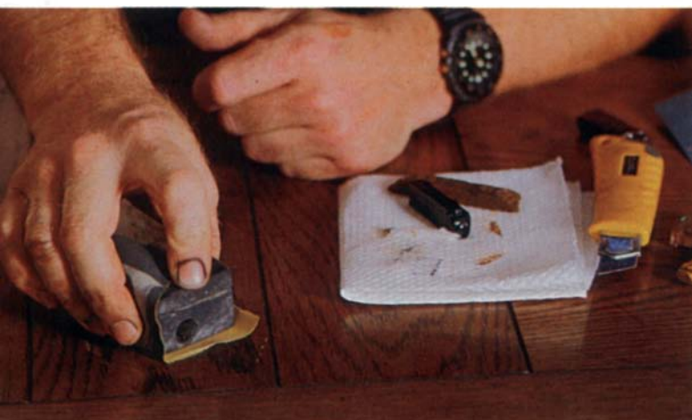
After the damaged area has been filled and the patch has been colored to match the surrounding grain area, the author levels the surface with microfine paper on a rubber block.
