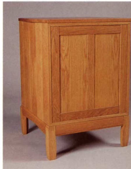
Above: This white-oak file cabinet was made with a variety of router shaping and joinery. Its boxy appearance is softened by recurring triangular designs that appear in the inlaid drawer fronts and the top, in the shape of the aprons and overhanging top edges, and in the routed detail on the side panels.
