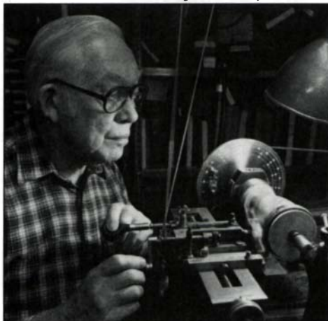
The late Frank Knox working on another ornamental turning on his Holtzapffel lathe in 1984.
