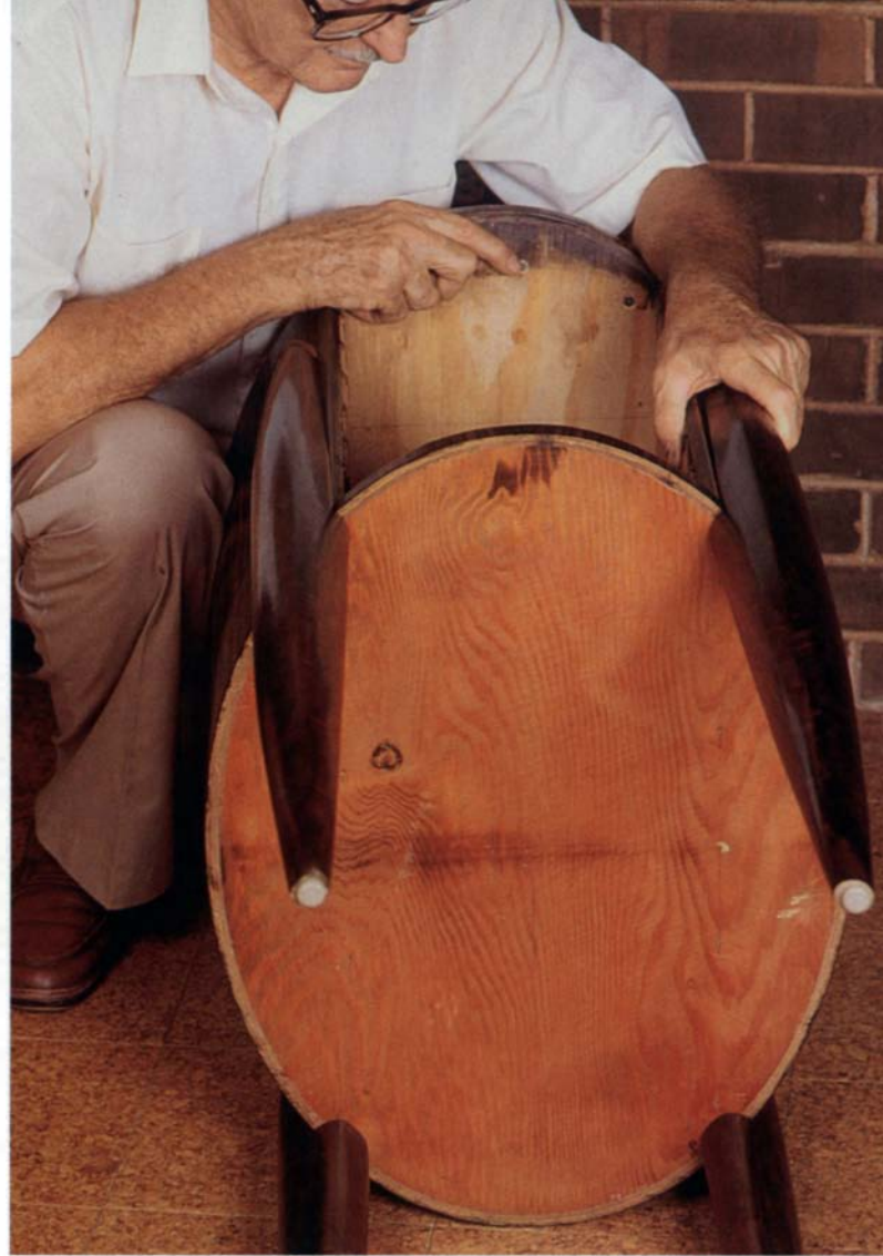
After lacquering the carcass, drawers, drawer pulls, legs and applied top separately, Leonard uses wood screws to join the parts together and complete his oval semainier.
