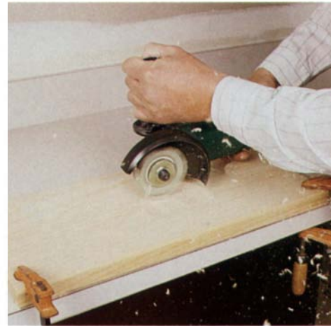
The Woodcarver imitates the cutting action of a chainsaw tip for rapid, safer and more easily controlled wood removal during freehand shaping.
