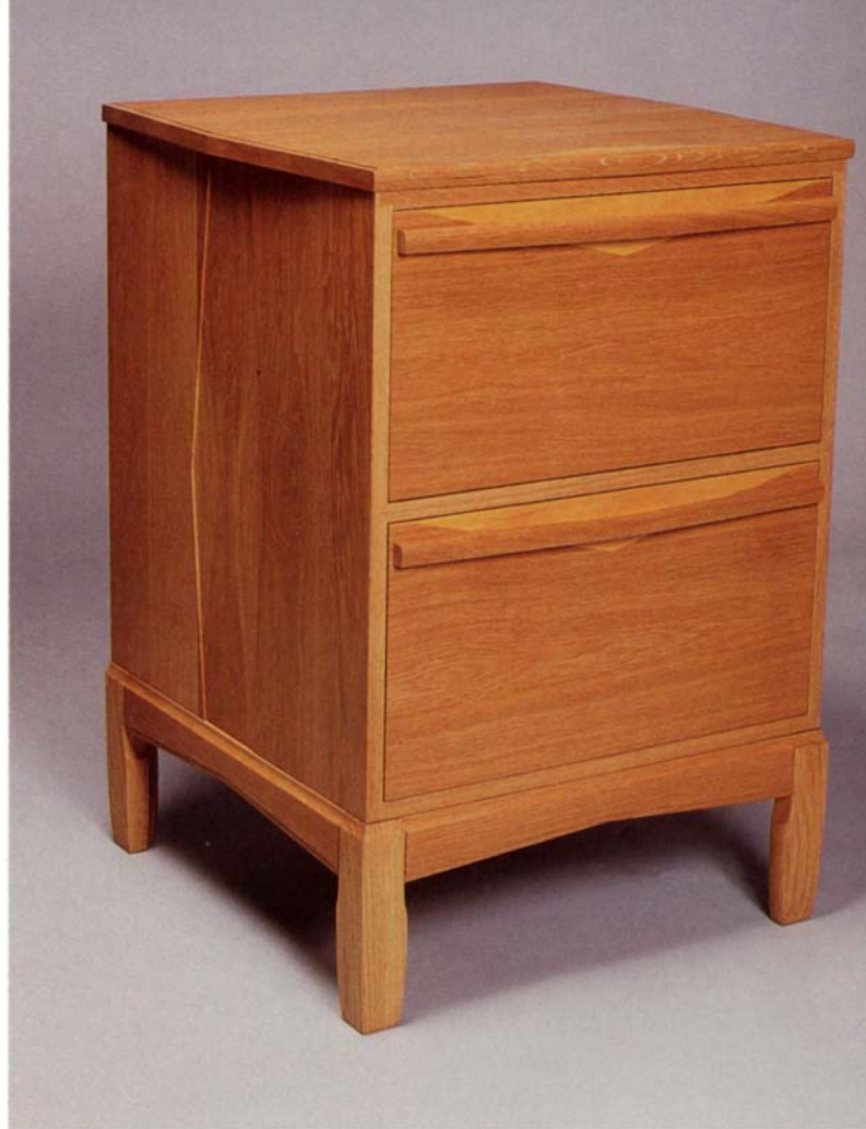
Above: This white-oak file cabinet was made with a variety of router shaping and joinery. Its boxy appearance is softened by recurring triangular designs that appear in the inlaid drawer fronts and the top, in the shape of the aprons and overhanging top edges, and in the routed detail on the side panels.
