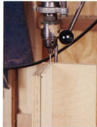
Above: An elevated guard attached to a standard tablesaw fence shields the blade from Brandli as he cuts corners off edging components. The cutoffs fall safely out of the way under the guard. Right: It's easy to bore holes into the ends of box components with this simple jig, which is made from an L-shaped plywood stand screwed to a base that can be clamped to a drill press table. Below: Rather than risk ruining a box frame by flattening it on a belt sander, the author trues the surface by repeatedly running it over sandpaper glued to a sheet of particleboard. The box is kept flat on the table and advanced at a slant.
