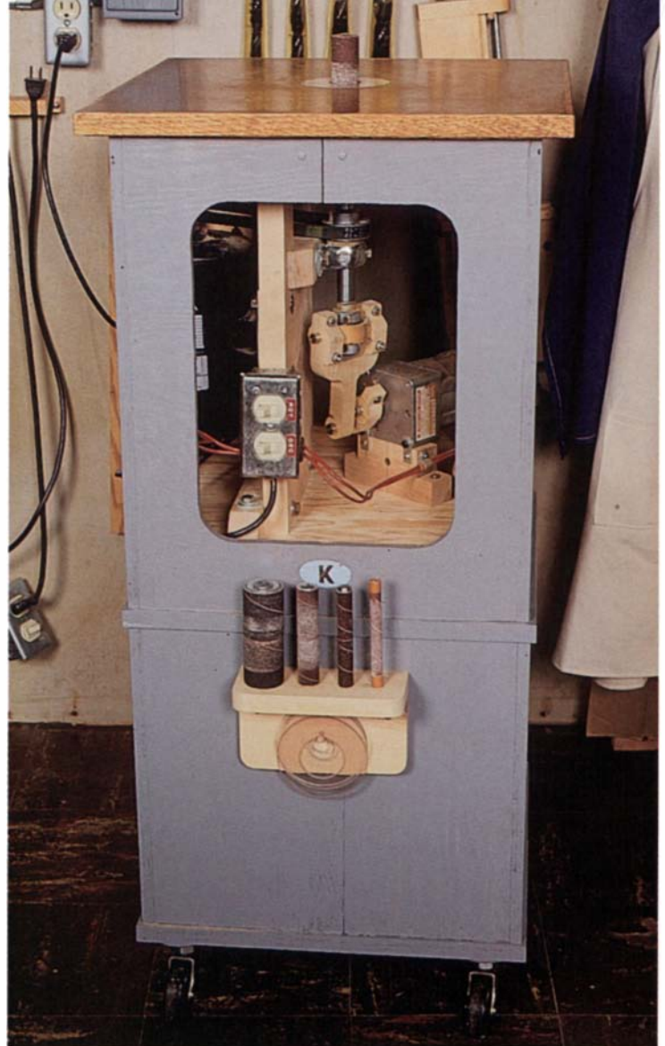
This oscillating-spindle sander is an economical and easy-to-build tool that's also a joy to use. It requires less than a sheet of plywood and except for the drive motor, the parts cost less than $100.
