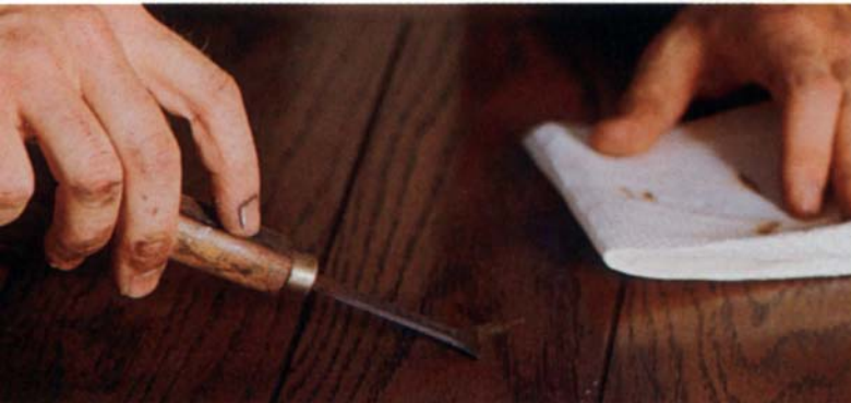
Two different colors of shellac sticks can be used to create a grain pattern in the patch area. Here Lawrence blends some dark lines into the lighter base patch with a hot knife.
