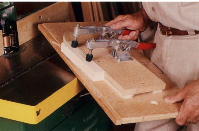
The author's tapering jig holds narrow lid-edging pieces at an angle, so a beveled cut is made when the assembly is pushed past the shaper knives. The clamps hold the pieces securely and the base is large enough to provide a firm handhold without bringing fingers near the cutting edge.
