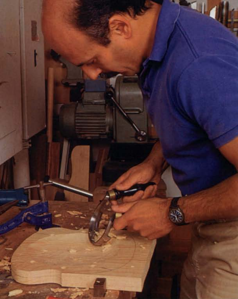
Above: Rodriguez scoops out the saddle with an inshave. Since the tool's long, angled handles prevent him from cutting steeply into the seat, he'll finish around the back edges with a wide gouge. Left: The author carves the front of the seat with a drawknife. He shaves to a line that is marked on the middle of the edge and that curves around the sharp corner where the top rolls over. Below: Rodriguez steam bends the combs for about 45 minutes in a closed plastic pipe connected to a wallpaper steamer. Then the combs can be wedged against forms on his plywood bending fixture.
