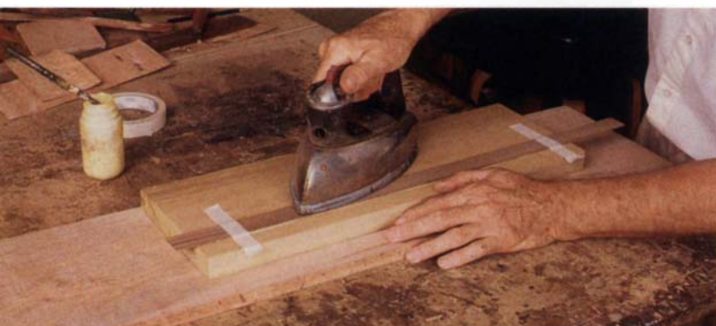
Leonard employs an unusual method to apply the veneer to the outside of his semainier: PVA glue that he quick-sets by heating the veneer with a clothes iron. Here, he tests the iron's heat on a scrap to make sure it won't scorch the veneer.
