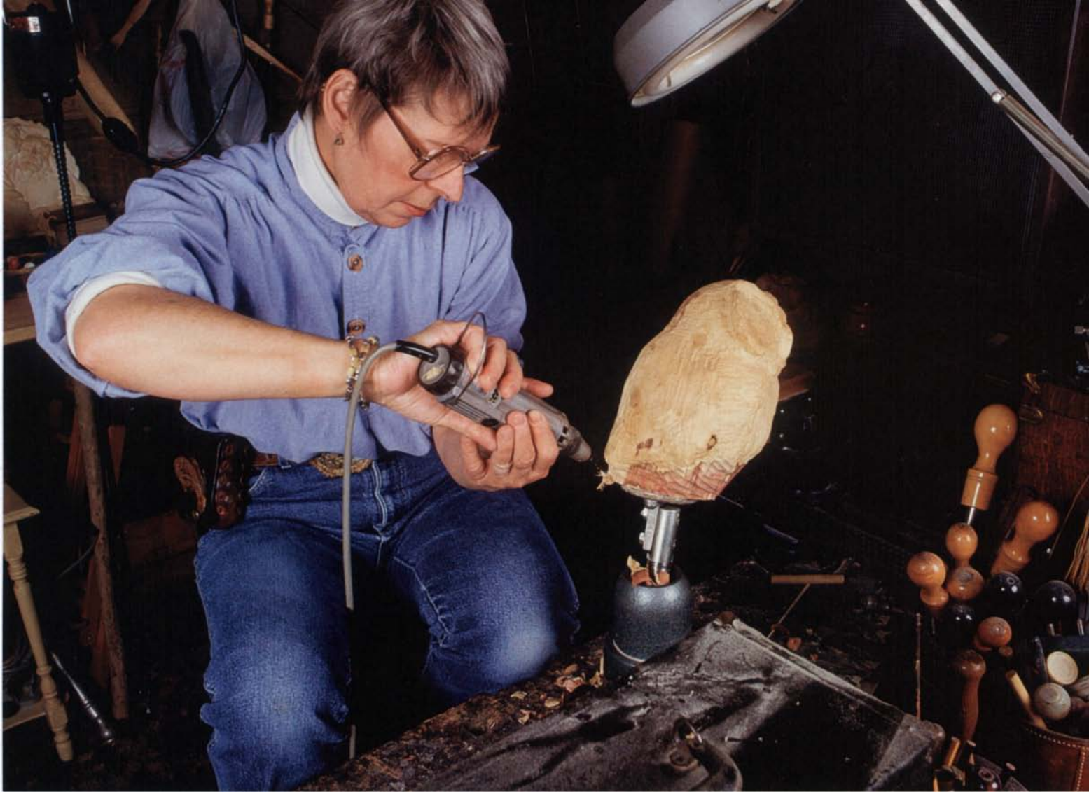
Small, electric power carvers are quick and efficient for roughing out stock and cutting fine details. Bartholomew uses a reciprocating carver to rough out a cedar owl. She will change to a flexible-shaft rotary grinder, like the one hanging by her shoulder, to carve finer details.
