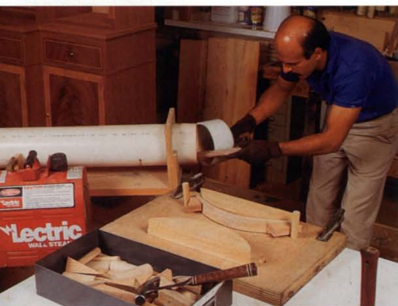
Above: Rodriguez scoops out the saddle with an inshave. Since the tool's long, angled handles prevent him from cutting steeply into the seat, he'll finish around the back edges with a wide gouge. Left: The author carves the front of the seat with a drawknife. He shaves to a line that is marked on the middle of the edge and that curves around the sharp corner where the top rolls over. Below: Rodriguez steam bends the combs for about 45 minutes in a closed plastic pipe connected to a wallpaper steamer. Then the combs can be wedged against forms on his plywood bending fixture.
