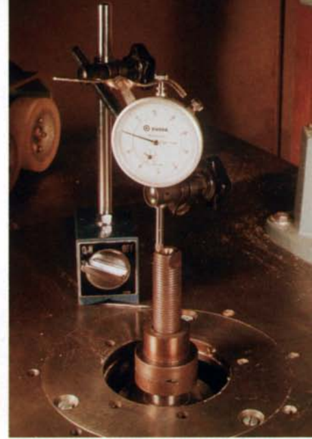
Right: The amount a shaper cutter is raised and lowered can be accurately gauged by setting up the dial indicator with the tip against the top of the spindle, as shown. After raising or lowering the spindle the desired amount, take a cut and use a dial caliper to check the results on the workpiece.
