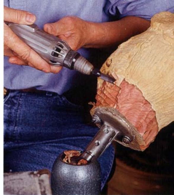
Right: Reciprocating carvers offer an option for those who prefer the look of tool marks and want to avoid dust. The tools, which cut only when pressed against the wood, as shown, cut smoothly when used across the grain or at a 45° angle to the grain.
