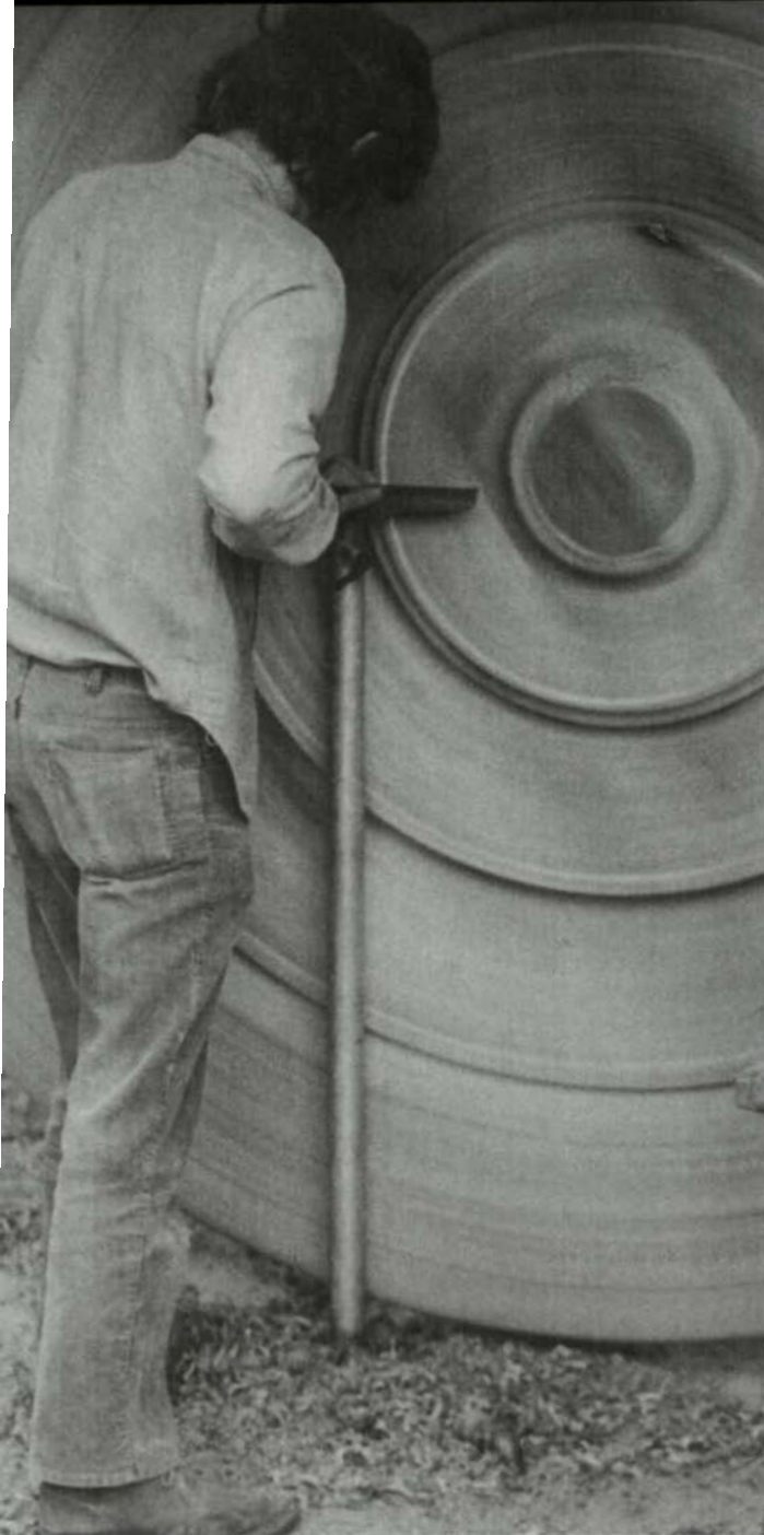
Above: Stephen Hogbin works the face of a 7½-ft.-dia. disc on his shop-built lathe. The lathe has a 1-HP motor that feeds power through a four-step pulley and a ¾-ton Ford truck axle and differential. Speeds range from 60 RPM to 1,000 RPM. Below: These 2¾-in.-high by 5½-in.-dia. bowls, produced in 1972 in cherry and cast aluminum, show technical control and beautiful proportions. The sensuality of wood is brought home as we respond to the handsome but stark translation in aluminum. The simple change in medium radically alters our perception and appreciation of the form.
