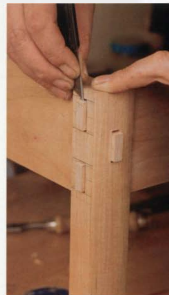
Left: After cutting the front-apron cheeks with a tenoning jig and dado blade on the tablesaw, Moore wastes the wood between the tenons. He uses a dado blade and a sliding table with stops to limit the space between tenons.
