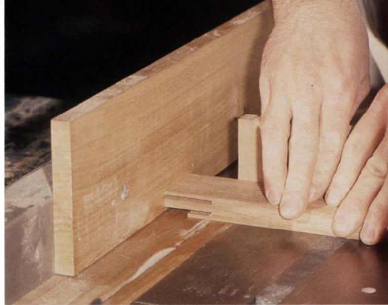
Tenons are sawn with stock held against a high auxiliary fence and supported by a miter gauge. Because of the danger of kickback, never attempt this cut freehand.
