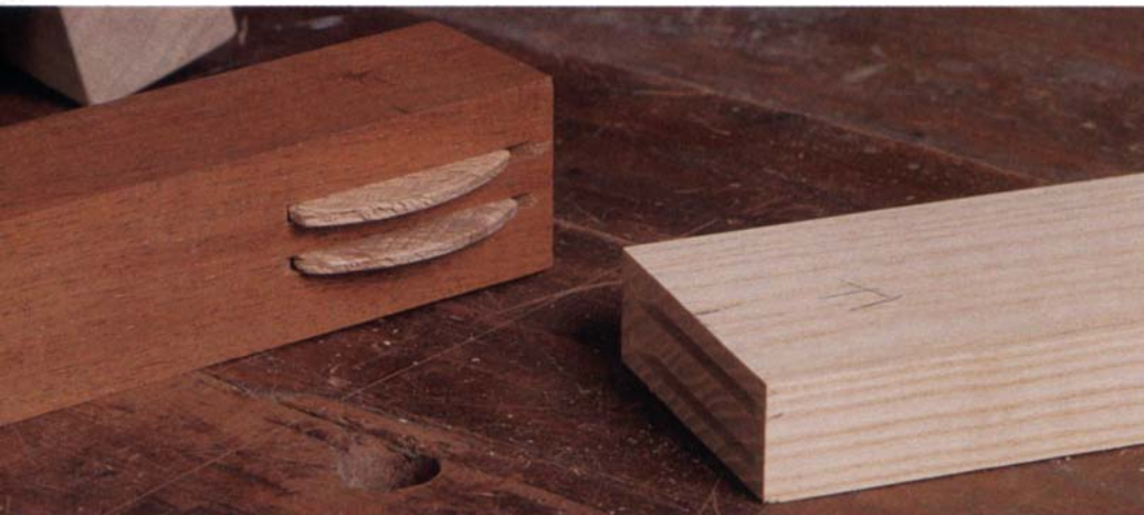
Above: Joints in large workpieces may be strengthened with two side-by-side biscuits. Right: To help prevent kickback when cutting pieces too narrow to contact the joiner's pins, Erickson screwed a rabbeting plane depth stop to the base. The stop also helps align workpieces.
