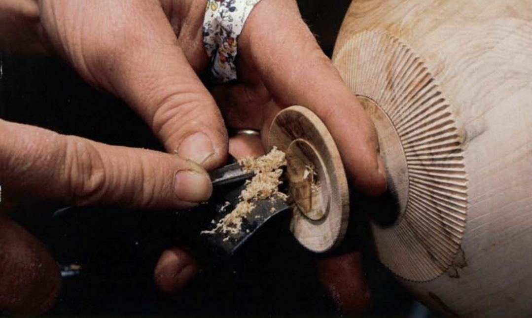
Left: Jordan supports the neck of the vessel with his left hand while taking very light cuts with a small gouge to shape the inside of the neck. Any mistakes at this stage can ruin the project.
