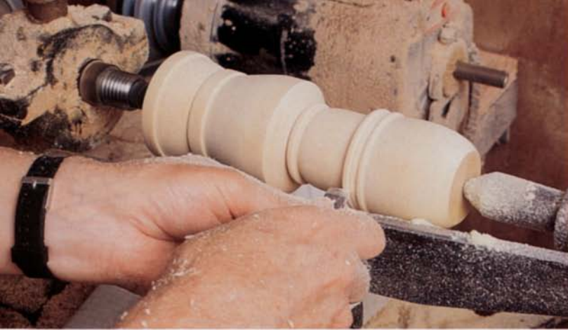
The torso, head and helmet are all turned together. Here the author rounds over the small beads that become the rim of the miter-type hat worn by Reginald, the green-clad nutcracker.
