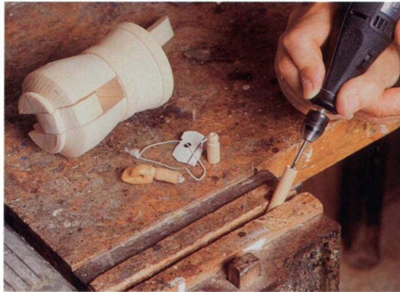
With a round-head carving bit in a rotary tool, Sneath forms a socket on the end of a \frac{3}{8} -in.-dia. dowel as part of the ball-and-socket wrist joint. After the socket is complete, a \frac{3}{8} -in. length of the dowel will be cut off and tied to the ball with elastic cord. Then the short socket dowel will be glued into a carved hand.
