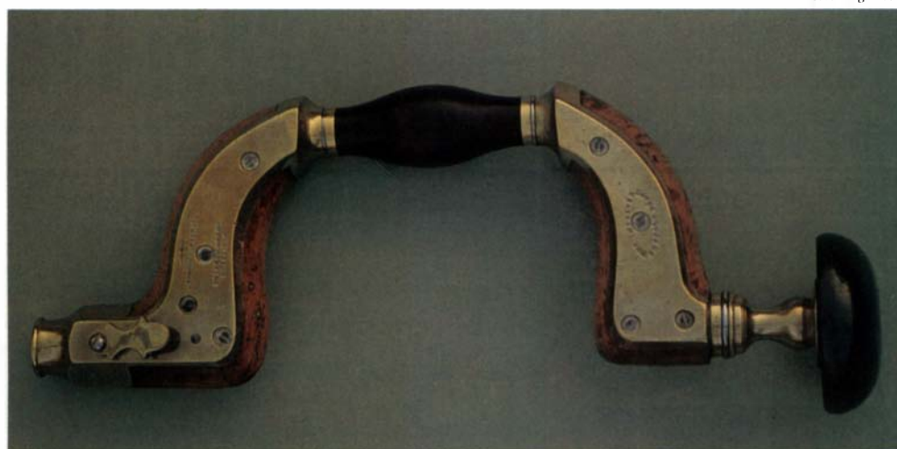
This brass-framed beech brace, made by Thomas Turner and Co., of Sheffield, England, has an ebony bead and handle, lever chuck and an internal bit-ejector spring.
