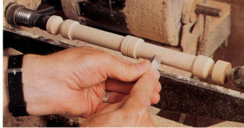
Sneath turns all the arm parts from a single spindle, which allows enough length to accommodate the overlap at the mortise-and-tenon elbow joint. The sleeve cuffs are in the middle of the spindle and the shoulders are at each end. Above, Sneath marks the point where he will saw the upper arm and forearm apart.
