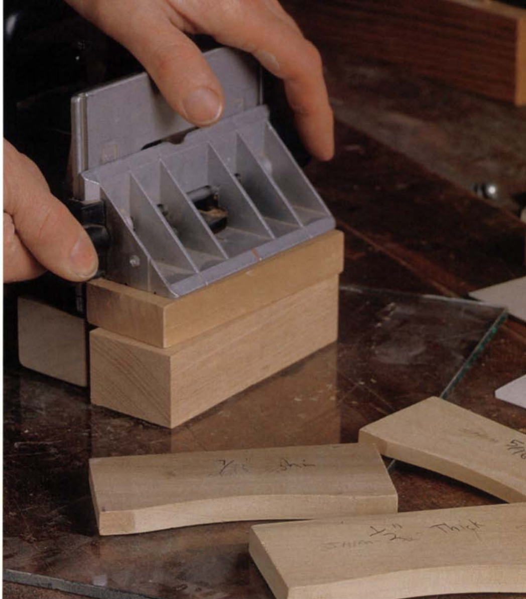
Erickson sets the fence height of his biscuit joiner and aligns it with the blade using wooden measuring blocks, which are 1/8 in. to 3/4 in. thick, that he made for the job. He uses plastic-laminate shims for thicknesses less than 1/8 in.
