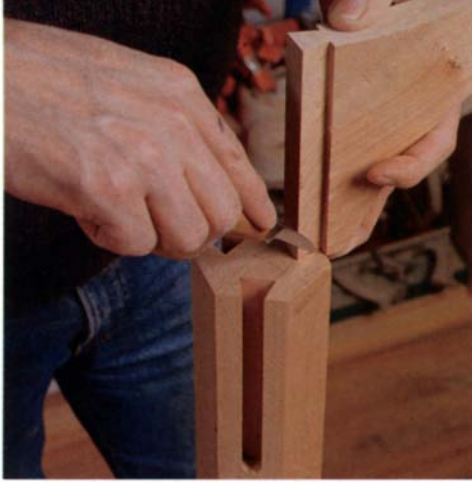
Using the dovetail pin on the leg as a guide, the author scribes the layout for the slot, which is cut with a dovetail saw and then chopped with chisels.
