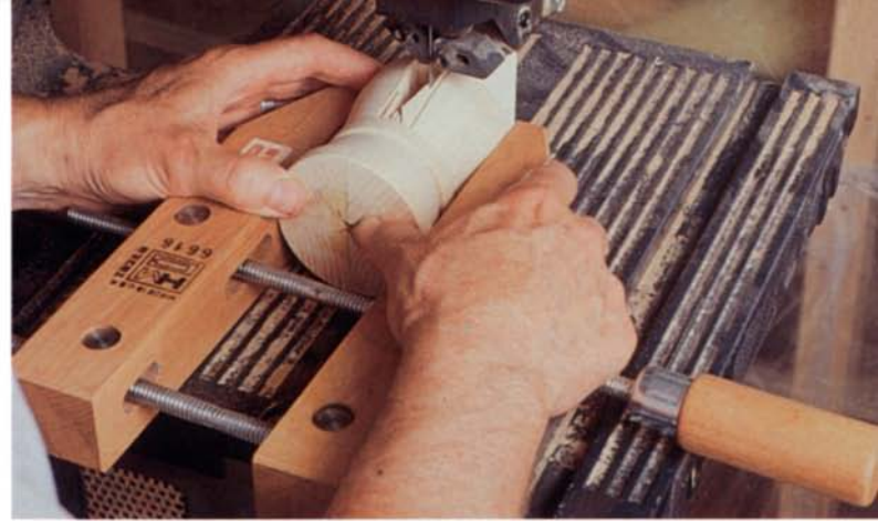
After bandsawing the head, including the helmet, from the torso, Sneath clamps the torso in a hand screw and bandsaws the channel that houses the jaw/crank.
