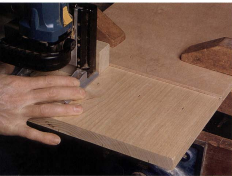
Above: For assembling a shelf to a carcass side, Erickson uses large biscuits. Right: A wooden faceplate extension is screwed to the joiner's base to stabilize the machine and make it safer for kerfing vertically held parts. Below: To kerf the carcass face, Erickson removed the joiner's fence and holds the faceplate against the workpiece. He guides the base against a plywood straightedge clamped to the work.
