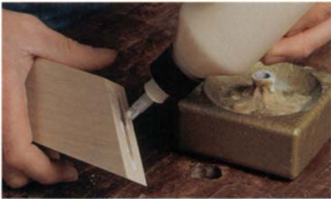
Next, spread glue in the kerf and on the joining surfaces. The Lamello dispenser is specially designed to spread glue in the kerf.
