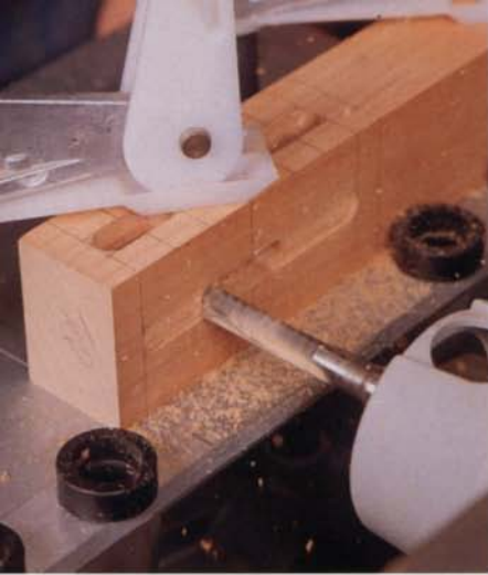
Left: The author uses a horizontal borer with a rotary miller bit to cut the through and haunched tenons on the top of a leg.
