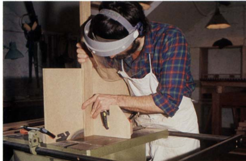
Tenon shoulders are cut on the tablesaw in two stages. The first cut removes about half the waste, and the second cut, as shown below, removes the rest and establishes the shoulder line. Cutting all the waste in a single pass could result in the scrap being trapped between the blade and fence and getting thrown out from the saw.
