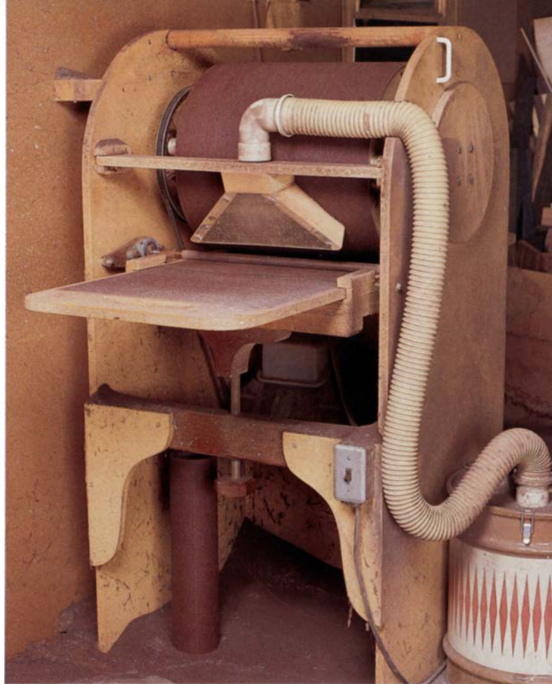
A large-drum thickness sander can provide even a small shop with the capacity to abrasive-plane and smooth wide stock. This sander, designed and built by Grit Laskin and David Wren, is economical to make: the drum and most parts were cut from \frac{3}{4} -in.-thick particleboard.
