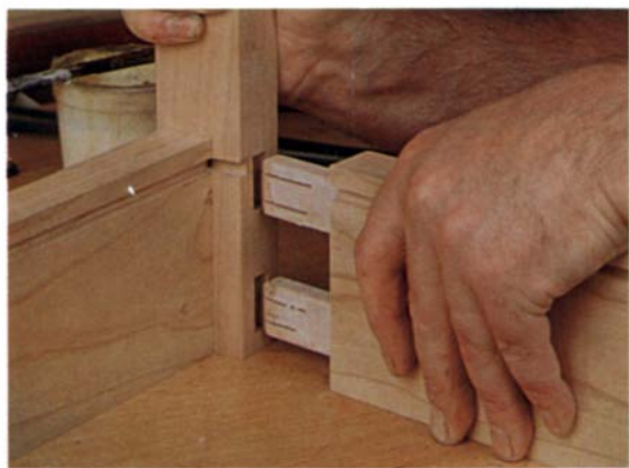
Terry Moore assembles a double-tenon joint for a small table. The tenons are kerfed for ebony wedges. See how he cuts the joint on p. 68. Cover: Nutcrackers make delightful holiday gifts (article on p. 76).
