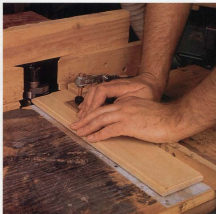
Below: Moore cuts the tongue on three sides of a divider on a shaper. He clamps the workpiece on a sliding table and uses two 1/2-in.-wide cutters with a 1/4-in.-thick spacer in between.
