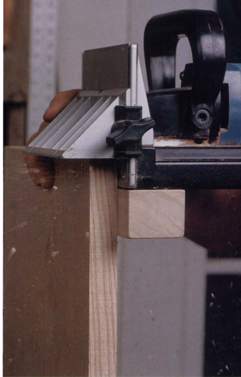
Above: For assembling a shelf to a carcass side, Erickson uses large biscuits. Right: A wooden faceplate extension is screwed to the joiner's base to stabilize the machine and make it safer for kerfing vertically held parts. Below: To kerf the carcass face, Erickson removed the joiner's fence and holds the faceplate against the workpiece. He guides the base against a plywood straightedge clamped to the work.
