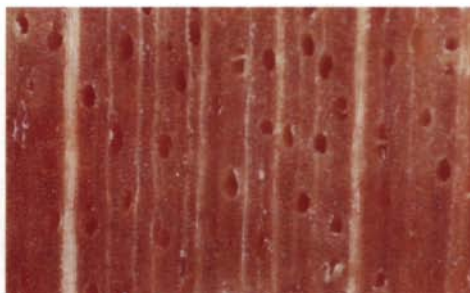
Sugar maple has two size rays and the widest are as wide or wider than its largest pores. Sugar maple is the most common maple cabinetmaking wood. This species is also related closely to black maple.
