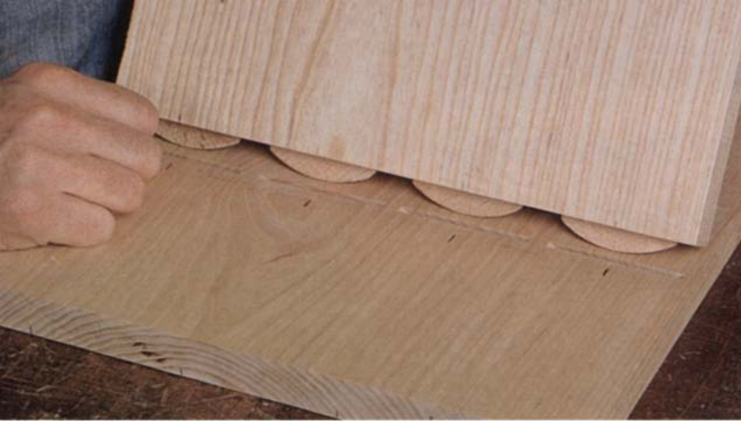
Above: For assembling a shelf to a carcass side, Erickson uses large biscuits. Right: A wooden faceplate extension is screwed to the joiner's base to stabilize the machine and make it safer for kerfing vertically held parts. Below: To kerf the carcass face, Erickson removed the joiner's fence and holds the faceplate against the workpiece. He guides the base against a plywood straightedge clamped to the work.
