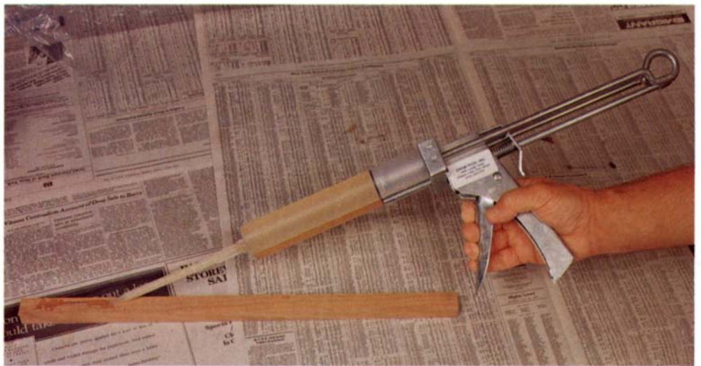
A squeeze of the Redimix gun trigger delivers properly measured and thoroughly mixed epoxy. Less than half a teaspoon of epoxy is left in the disposable mixing tip.
