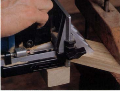
To join a mitered frame, align the joiner's faceplate to the end and its fence down on the top face, and plunge the cutter.
