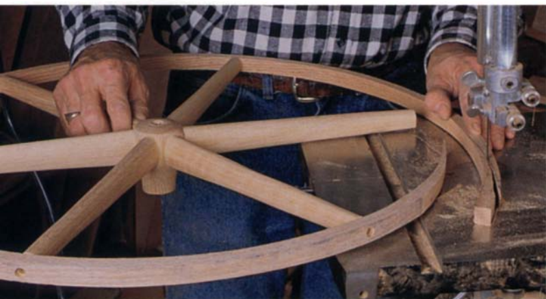
Dunham bandsaws close to the scarf joint line: above the line on one end and below the line on the other. Then, he will smooth the scarf joint's mating surfaces with a rasp.
