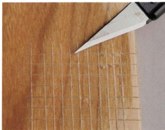
Above: Evaluate how well a film adheres to wood with the cross-cut test. Cut a grid with 100, 1/10-in. squares, and rate by counting the number of failed squares: right after making the cut, after trying to brush them off and after trying to pull them off with tape. Only the corners of eight squares have flaked off after pulling the tape on this sample; it is rated high: 4 to 5.
