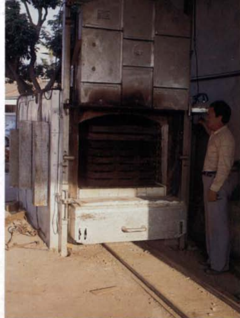
such as saw tables, must be heat-treated to relieve internal stress before machining them flat, so they don't warp later. C.F. Chang, president of Kuang Yung, handles this job himself, heat-treating tables for 12-in. tablesaws in a large electric kiln (right).
