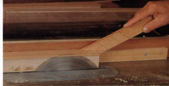
Above: Excess laminate on one side of the walnut leg extends over a 1½-in.-high auxiliary fence as the excess is ripped from the leg's other side. Below: After clamping a leg in the mortise jig, Frid guides the router fence against the jig's side and gauges the mortise's length with the jig's stops.
