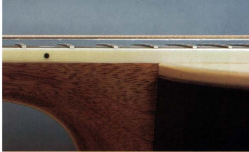
The distance between the strings and the 12th fret, marked by a black inlay dot, is crucial to the guitar's playability. The distance is checked with a thread and any adjustments are made at the saddle.
