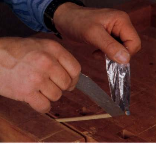
The mandrel-bend test evaluates a film's flexibility. Ratings are based on the smallest dowel that coated foil can be bent over without the film peeling. This film bent over a 1/8-in.-dia. dowel and rated high: 5.
