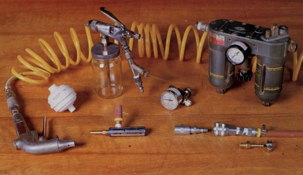
Compressed-air system accessories for cleaning and drying the air, as well as oiling and regulating it, are numerous. For instance, shown in the front row, left to right are a blow-off gun attached to a coiled air hose, for dusting work before finishing; a lipstick-size vacuum pump that is amazingly powerful; and a quick-change coupling system that allows air devices to be readily exchanged. Back row: This small, disposable air filter attaches directly to the gun or tool; a touch-up spray gun is handy for small finishing jobs; this regulator/gauge unit is made to attach at the device, to allow easy adjustment of the air flow; for air-powered tools, this combination device offers a filter, regulator, pressure gauge and oiler in one compact unit.
