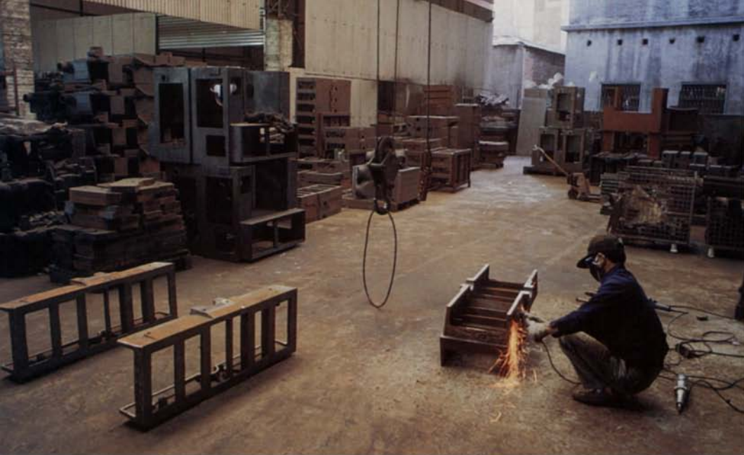
Cast-iron parts are so cheap in Taiwan that they're used in large and small woodworking machines. After arriving at the CKM factory from the foundry, castings for planers and jointers are cleaned with abrasive grinders before they're machined (left). Large iron castings,
