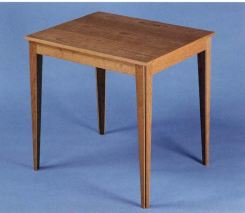
The lines of the author's end table are straight, the corners sharp and crisp, and the parts proportional to one another. The legs are thin strips of cherry and maple laminated to a walnut core, visible in the rabbet on the leg's corners.
