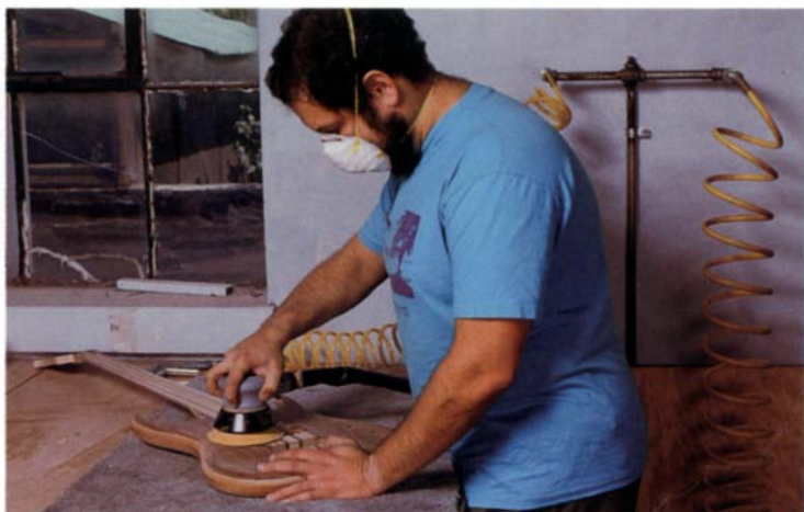
Practically every electric-powered hand tool has an air-powered equivalent that's stronger and faster. Here, the author sands an electric bass guitar with an air-powered orbital sander.
