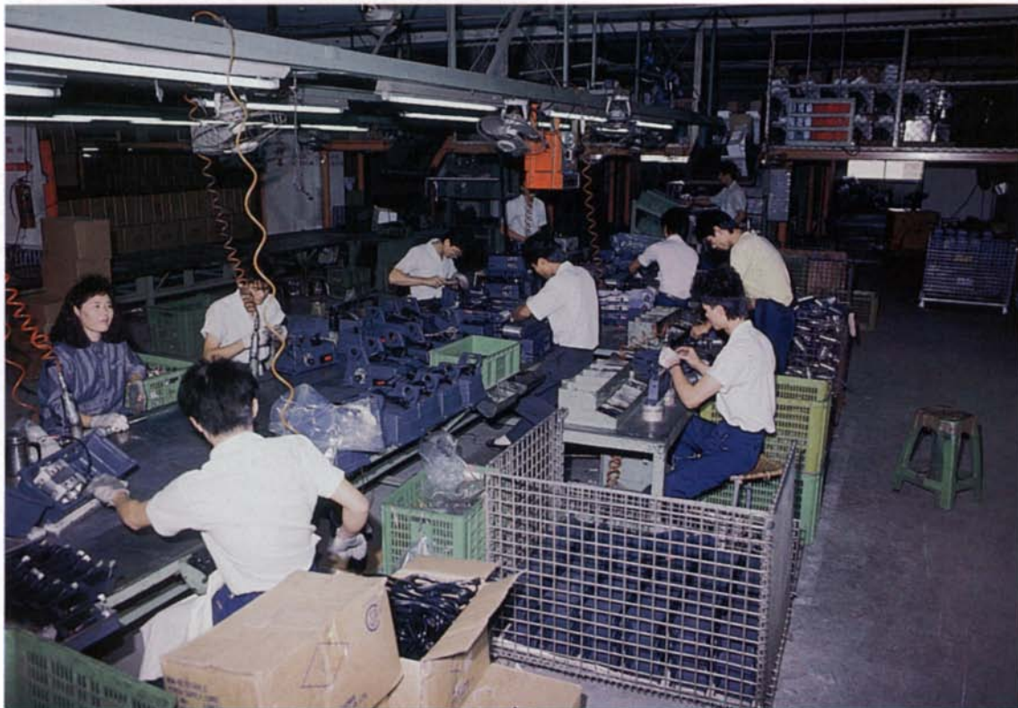
Above, left: Workers at the Chang Iron factory near Taichung assemble a batch of 18-in. planers destined for the U.S. market. Working six days a week, a handful of ambitious workers manage all the assembly tasks, bolting together parts that are mostly supplied by subcontractors.
