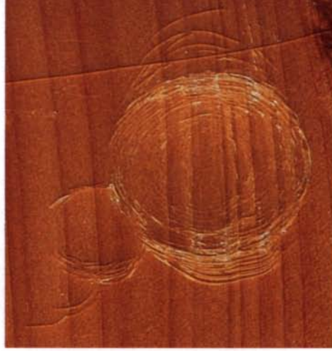
Test distortion resistance after a sudden shock by dropping a 1-in. steel ball from 3 ft. onto a test sample. Base ratings on the amount of cracking at the edge of the resultant crater. This film rated low: 1.
