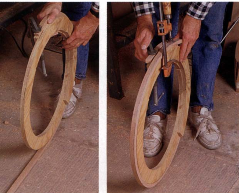
As soon as the rim stock is removed from the steam box, one end is clamped to the "spiral" form, as shown at left. Then, the rim is rolled up onto the form and its other end is clamped so that the ends overlap at least 6 in., as shown at right.
