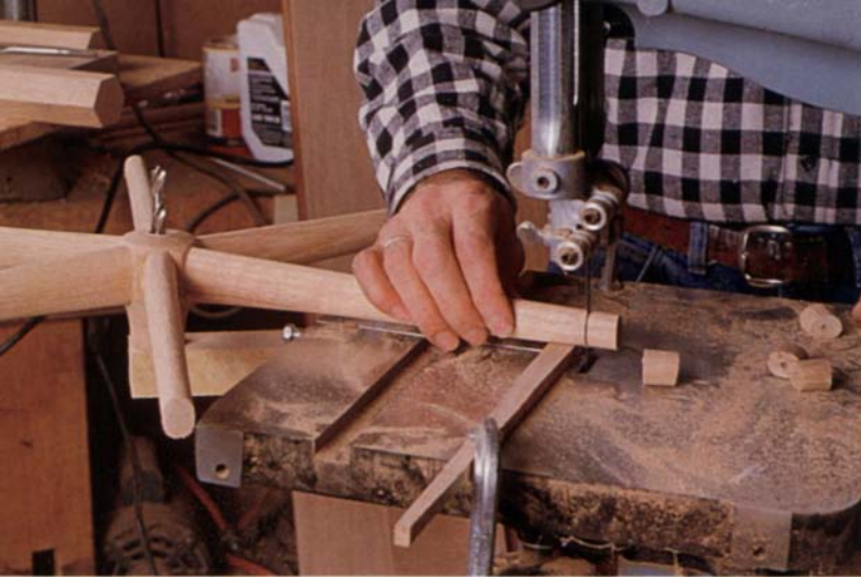
The spokes are trimmed to length after they're glued into the hub. The drill bit, which acts as the pivot point, must be aligned with the bandsaw blade and centered exactly 11 3 / 8 in. from the blade for the wheel to be 24 in. in diameter when the rim is wrapped around the spokes.
