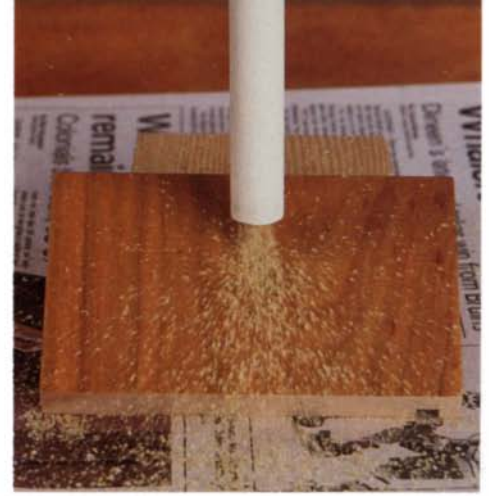
Evaluate abrasion resistance by pouring sandblasting grit through a 3-ft. pipe onto a sample. Rate the finish based on the amount of abrasion. This finish is abraded nearly to the wood. Rating: 2 to 3.
