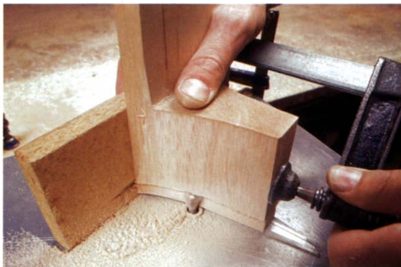
The dovetail that joins the guitar's neck to the body is shaped on the router table. A standard dovetail bit cuts the male dovetail as the neck, screwed to a Plexiglas template that rides against a stationary guide bushing, is moved over the table.
