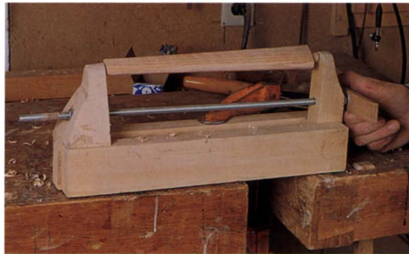
This clamping fixture holds the spokes tightly, yet allows them to be quickly rotated, to speed up the process of handplaning the spokes so that they taper from oval at one end to round at the other.
