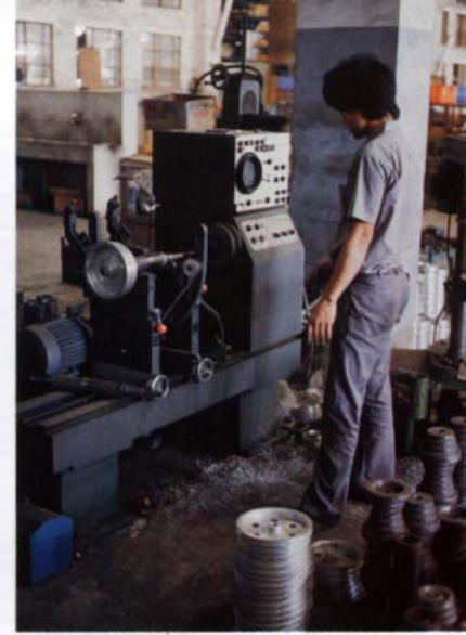
Above, left: Workers at the Chang Iron factory near Taichung assemble a batch of 18-in. planers destined for the U.S. market. Working six days a week, a handful of ambitious workers manage all the assembly tasks, bolting together parts that are mostly supplied by subcontractors.
