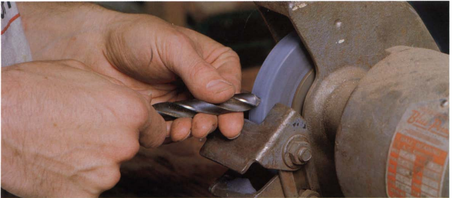
Grind standard twist drills by holding the cutting edge up so that it completely contacts the front of the wheel. Hold the shank down about 12° to relieve the back of the edge and create a positive clearance angle, which reduces the bit's friction when in use.
