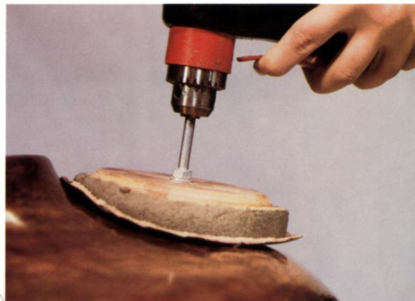
Johnson uses a shopmade sanding pad chucked in an electric drill to finish a turned vessel without swirl marks. (Photo by author.)
