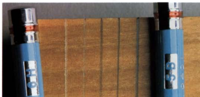
Below: The pencil-scratch test evaluates the film's hardness. The hardest pencil, 6H, scratched clear through the finish, a 4H just broke the surface, and the soft 5B left a mark that could be cleaned off. Rating: 3.
