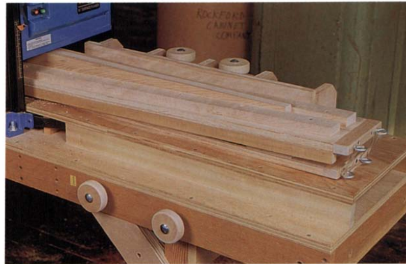
This birch-veneer plywood planer jig cleans up sawn tapers on legs more quickly and uniformly than handplaning, leaving a surface ready for final-sanding and finishing.
