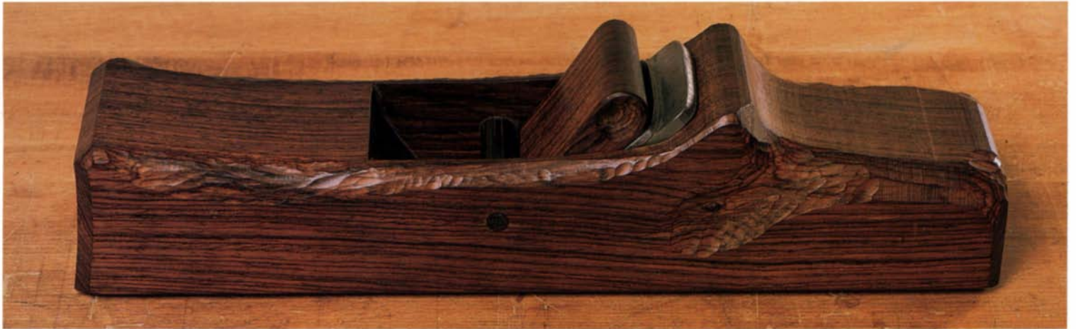
Robinson prefers rectangular shapes for his planes and doesn't spend a lot of time refining the appearance of these working tools. Finger grips are gouged into the sides, corners are chamfered on the bandsaw and the bandsaw marks are left for a better grip.
