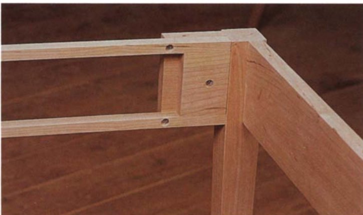
The drawer framework is screwed directly into the back of the stub aprons to keep the legs from splaying or racking.
