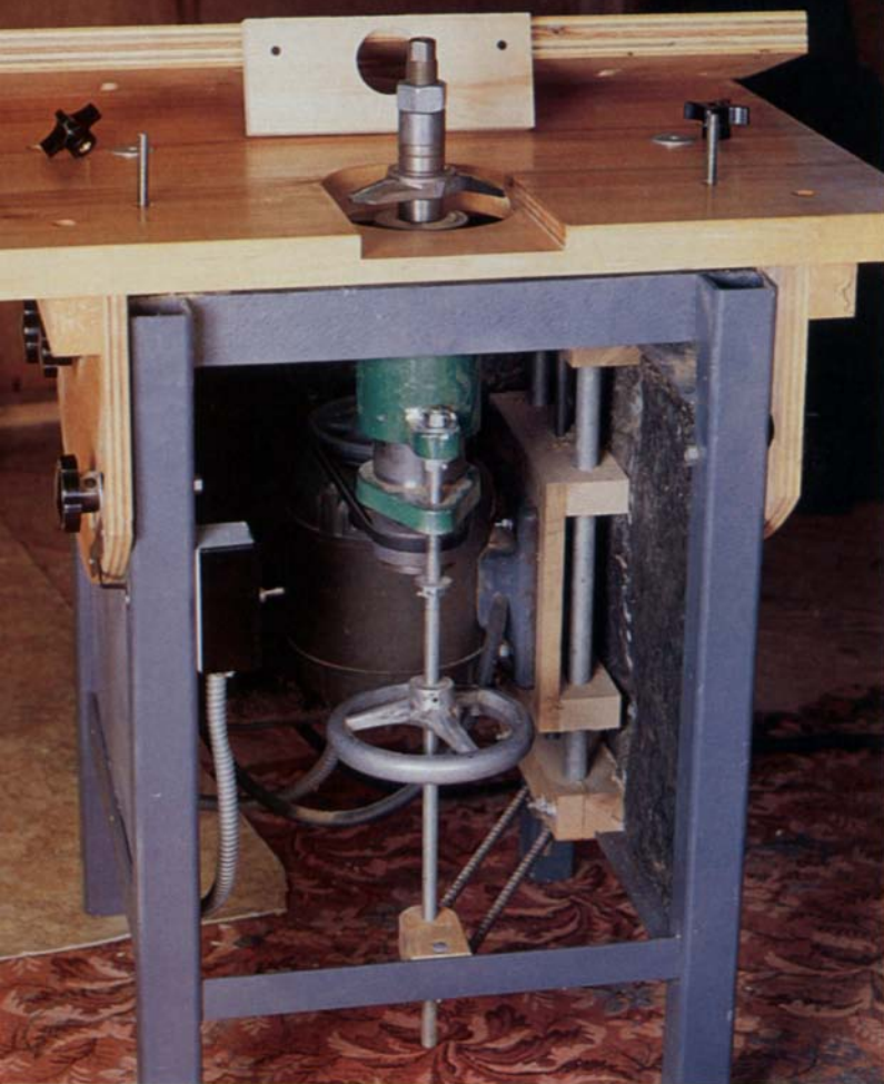
Starting with the stock spindle he purchased, Perron modified the assembly to allow the cutter to be raised and lowered via a handwheel at the back of the shaper. A chain drive at the bottom links the handwheel shaft with a sliding motor carriage and adjusts the height of both the motor and spindle synchronously, to keep their V-belt drive pulleys aligned.
