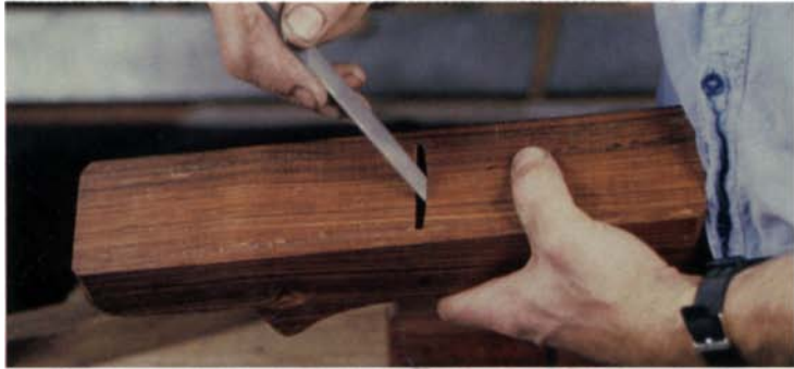
Working through the small mouth opening, Robinson fine-tunes the plane to match the shape of the iron. Paper-thin shavings are possible only with a close fit between iron and mouth.
