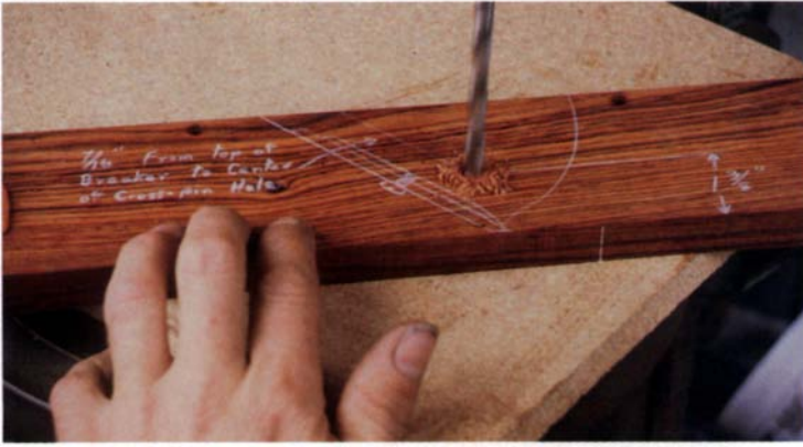
Align both cheeks using the reference line drawn across the top of the plane, clamp the cheeks together and drill a \frac{1}{16} -in.-dia. hole on the drill press to ensure accurate alignment for the cross pin.
