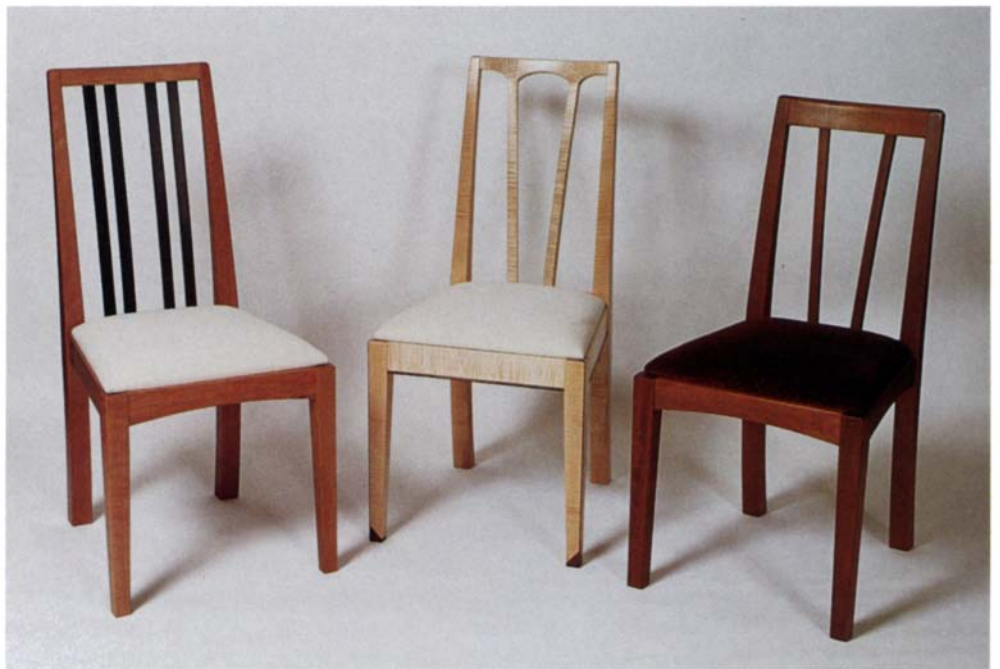
These chairs are from the same design series developed by Moore. Although each is different, they all share the same construction methods based on a series of shop-built patterns and jigs. The chair on the left is of Honduras mahogany, the chair in the middle is curly maple with rosewood inlay and the chair on the right is cherry with ebony back slats.
