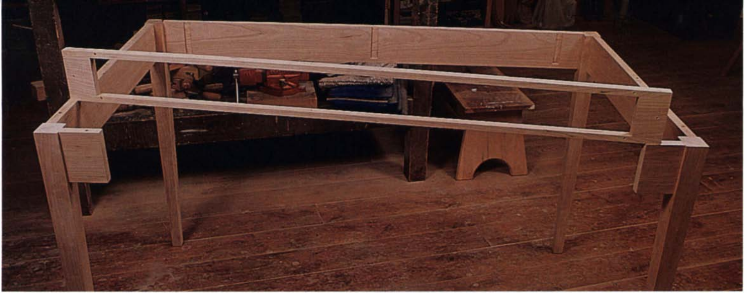
This framework is screwed into the back of the stub aprons, connecting the ends of the table and providing an opening for the drawers. Note the pins securing the aprons to the legs and the dados visible on the back apron that will accept the dividers of the drawer guides.
