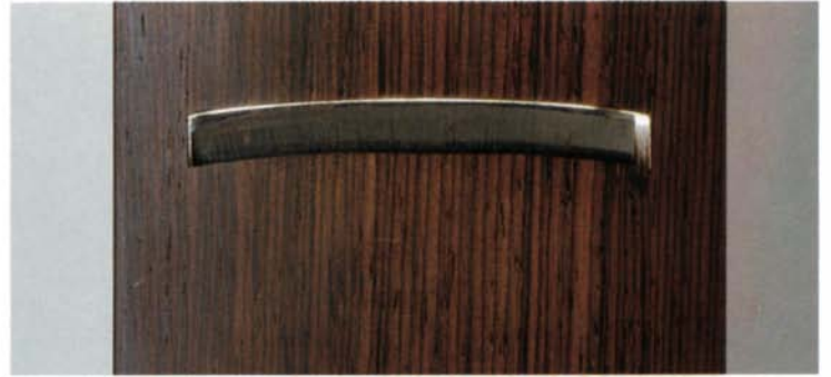
Shaping the mouth of the plane is the most tedious part of the construction, but the time and effort invested in attaining the fit shown here will be rewarded by top-notch performance.
