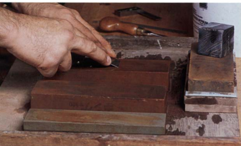
The tool's edge is ground mainly on the pull stroke. The author's hands surround the chisel and honing guide as he pulls and presses with his index fingers while honing on a wet 1,200-grit stone. On the return stroke, he uses his thumbs to push against the guide and doesn't apply downward finger pressure. The small cube is a nagura stone used to prepare surfaces on fine waterstones.
