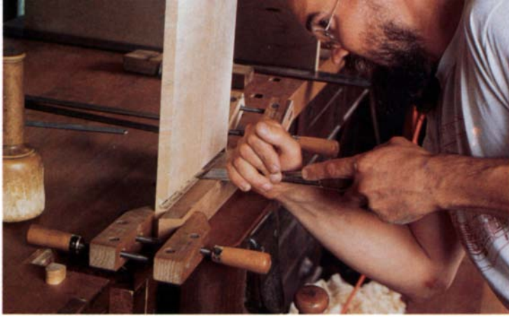
Thomas uses a guide block with an 80° bevel as accurate reference surface for paring the angled wall of the dovetail socket. Note how the socket tapers from the back of the joint to the front.
