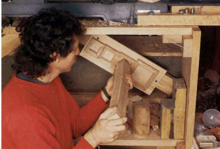
Gellman uses his shopmade center-finding jig, mounted conveniently under his lathe, to quickly mark the center on a spindle. After selecting the correct-size frame, he rotates the turning blank in the frame, automatically centering it, and then he pushes the blank against the screw in the center to mark it.
