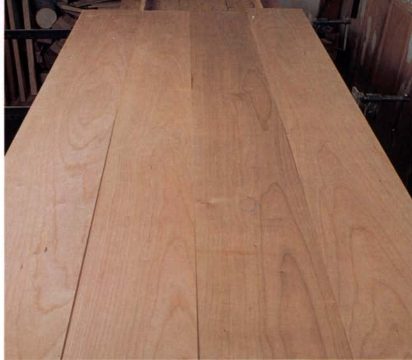
In gluing up narrow boards, the goal is to produce a panel of uniform color, with a fairly continuous grain pattern across its width, as shown in the photo above, left. A poorly matched panel, shown in the photo above, right, looks more like an assemblage of separate boards.
