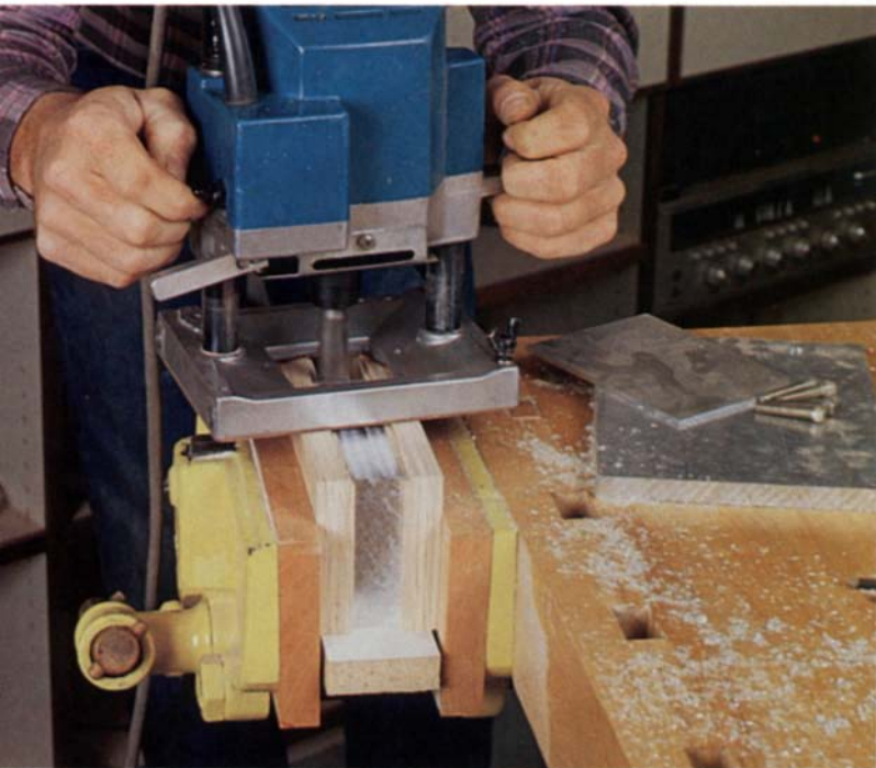
A router equipped with a carbide bit can easily machine non-ferrous metals. Here the author machines a square edge on a thick piece of aluminum plate with the router guided by a rail jig cobbled up from plywood scraps.
