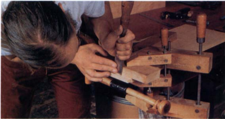
To prevent tearout when working with a plane that does not have a spur for cross-grain scoring, the author cuts a line with a chisel guided by the 90° side of the guide block.
