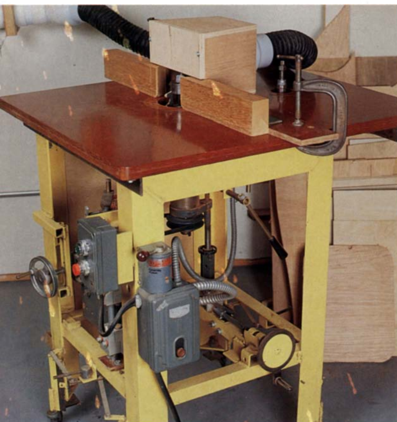
Doing metalwork in your home woodshop lets you save money and build custom machines, like the author's dual-spindle shaper shown here. The shaper has two workstations in a compact space, and the 1/2-in. and 1-in. spindles can handle a variety of cutters.
