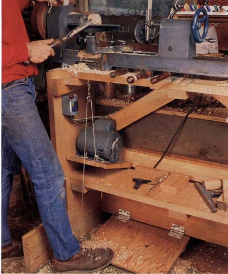
A shopmade lathe clutch, shown here fitted to Gellman's Rockwell lathe, can speed up many spindle-turning jobs because it makes it possible to disengage the motor without switching it off. The clutch also allows turning speed to be decreased during a cut.
