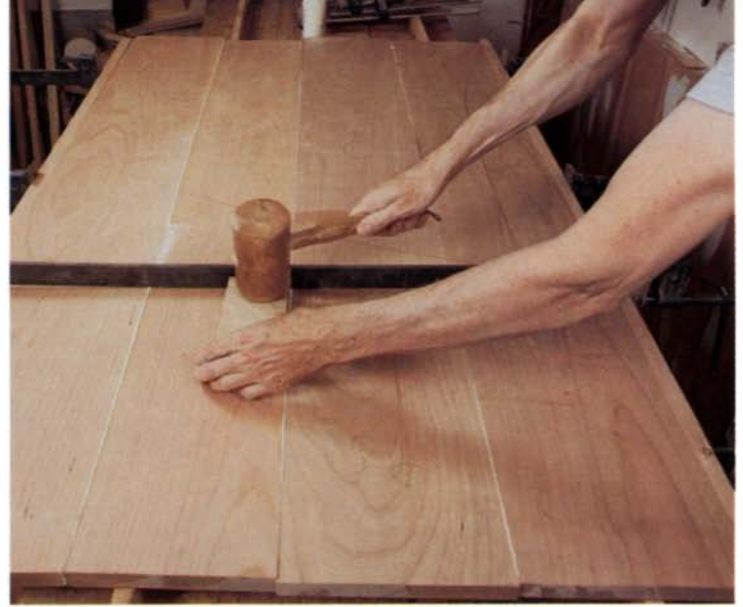
Rather than rely on dowels or other devices to align boards during glue-up, Becksvoort simply uses a mallet and a piece of scrap to hammer on the joint until the boards lie flat.
