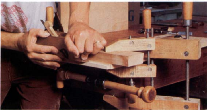
The 80° bevel on the dovetail plane automatically cuts the proper bevel on the pin. The taper shown is created by planing more off the front of the pin than the back.
