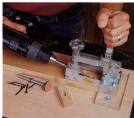
With Port-A-Guide and a 3/8-in. drill you can drill angled holes and screw face frames together in the shop or on-site.
