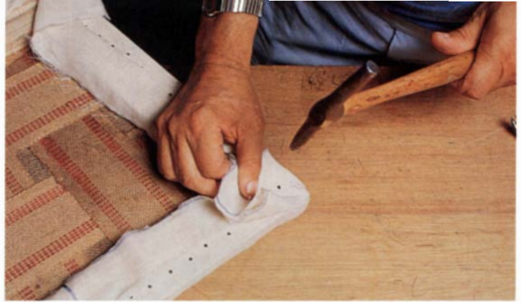
To finish the corners of the seat, pull the material toward the diagonally opposite corner and tack it in place as shown above. Cut toward the corner on either side of the just-installed tack to remove any excess material.
