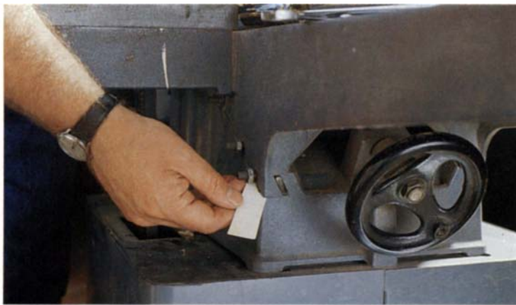
If adjusting the gibs fails to correct a table sag or tilt, brass or paper shims can be inserted as shown to lift the table.
