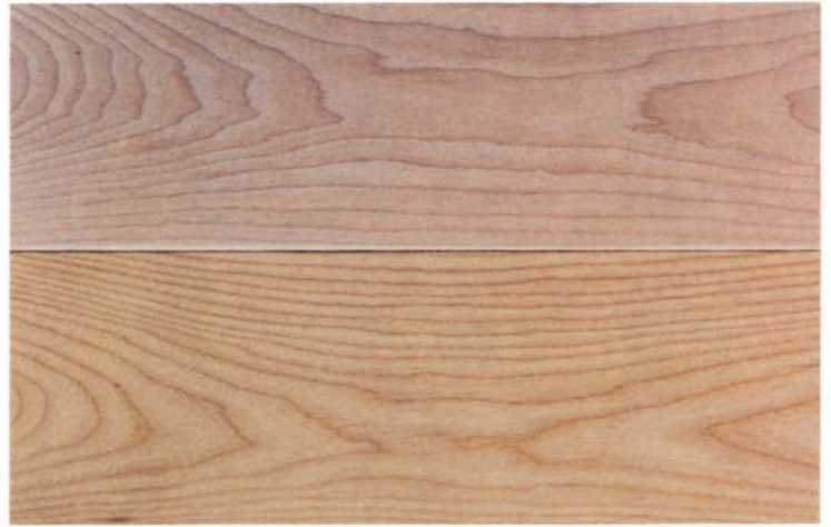
Although it's often referred to as a limed-oak finish, a limed finish can be applied to any type of wood. Here, a white ash sample, shown unfinished above, received a limed finish, which was applied directly to the raw wood.
