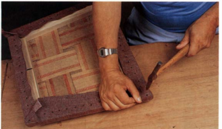
Pull the material on the front of the frame parallel to the side of the frame and tack it. The corners of the upholstery are folded first at the sides and then at the front so the seams are visible only from the sides. A cambric cover on the bottom of the seat finishes the chair.
