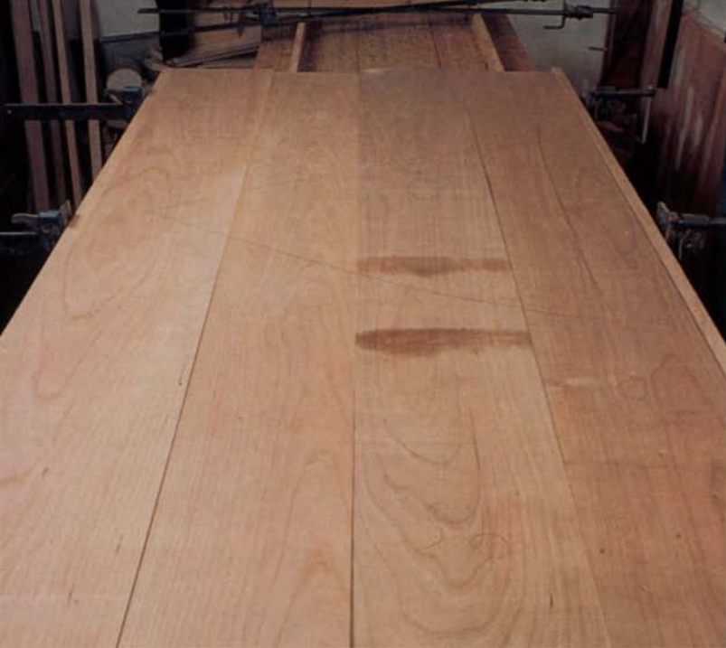
In gluing up narrow boards, the goal is to produce a panel of uniform color, with a fairly continuous grain pattern across its width, as shown in the photo above, left. A poorly matched panel, shown in the photo above, right, looks more like an assemblage of separate boards.
