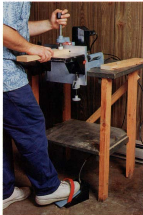
Delta's 32-100 stationary plate joiner's foot pedal action cuts slots while leaving the operator's hands free to hold the work.
