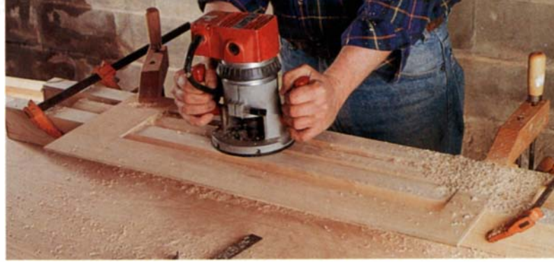
The side pieces of this jig hold the leg and provide a work surface to rout the flats that give the joints between the legs and panels a coped appearance. The flats also provide a reference surface for mortising the round legs.
