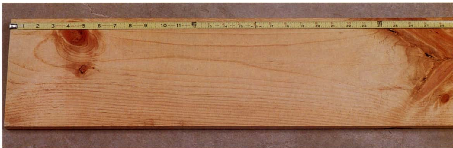
Depending upon the width needed, 18 in. or more of clear eastern white pine could be cut from this piece of #4 Common bought at the local lumberyard. By selective cutting, even boards with missing knots can provide beautifully figured, high-grade lumber.
