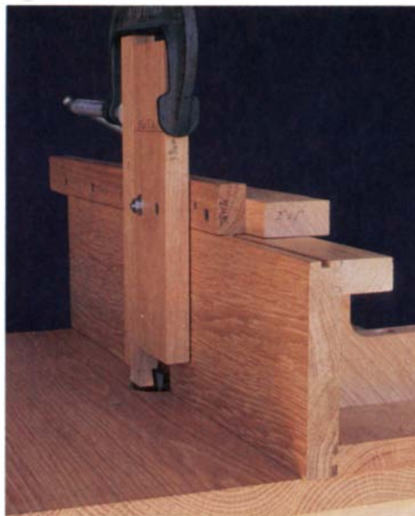
A sliding fence attachment holds the work while routing the pins. Adjust the fence so the workpiece is not trapped between it and the router bit.
