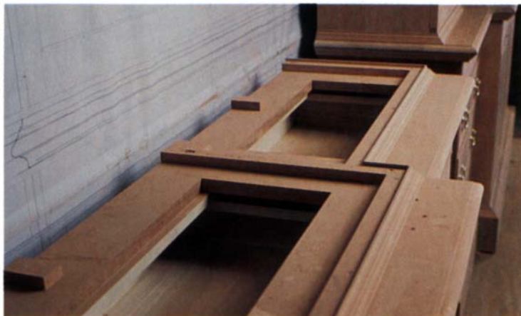
Below: The waist assembly frame, shown sitting atop the lower cabinets, is glued up with the endgrain continuous across its ends. To allow for the frame's expansion and contraction, the upper-case retainer molding is attached at the back with screws through slots.
