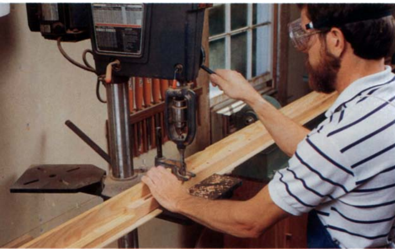
The author uses a hollow-chisel mortiser on the drill press to chop mortises in the shoji frame for the kumiko. By referencing the end of the frame against a line of blocks laid end to end (the block on the far end clamped to the fence), mortises can be accurately spaced, removing one block after each mortise.
