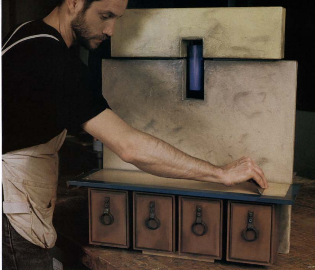
After the first three coats of Wood Armor have dried, the author uses a cabinet scraper to smooth out any dust particles. He then applies two final coats of the clear finish.
