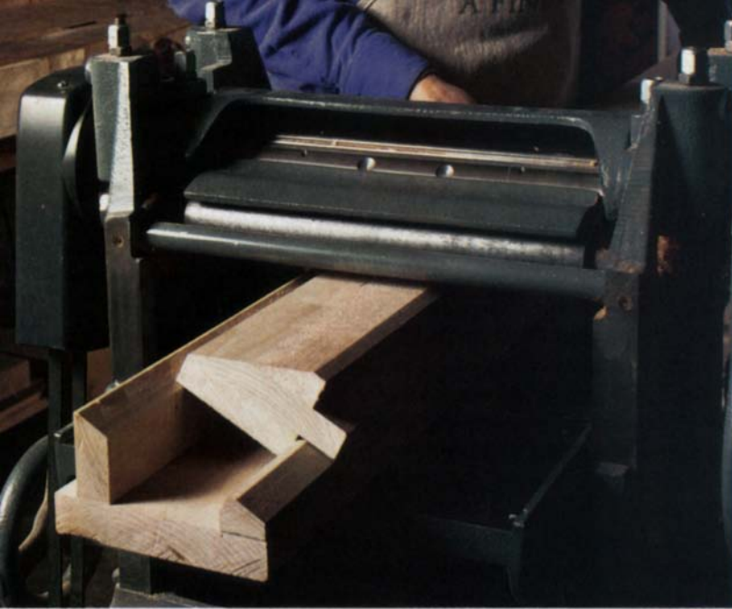
This simple planer jig makes it easy to bevel the backrests and rails for the benches and table. A stop keeps the rail from slipping in the jig, while the pressure from the feed rollers holds the rail down.
