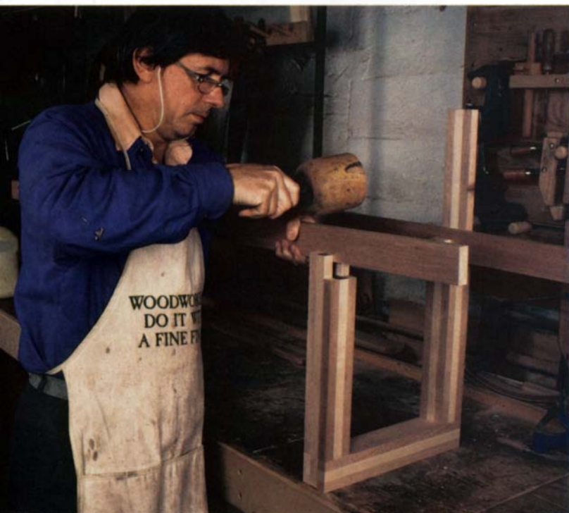
Using the bench assembly as an example, Murphy shows the simple but very accurate leg-and-frame joinery that is possible during glue-up with the nine-piece system.
