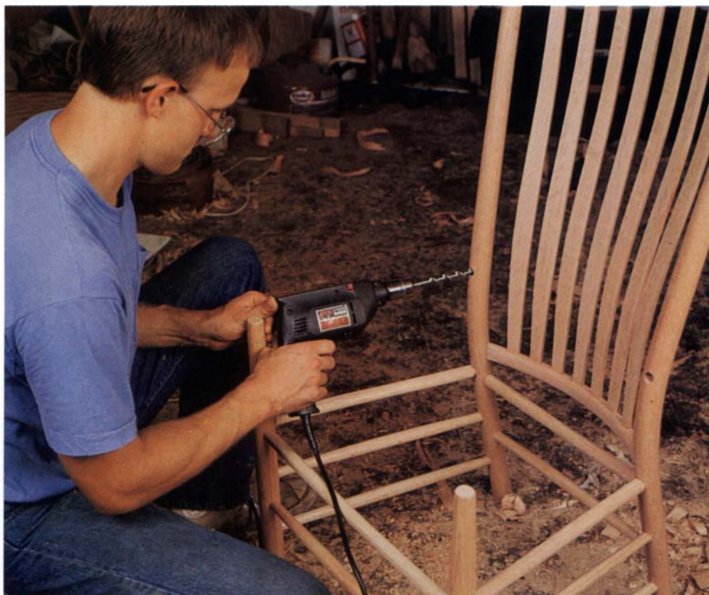
Above: Boggs' bent-back rocker design evolved as he experimented with changes in early chair models. Left: With a Forstner bit in a power drill, the author bores the armrest mortise in the rear leg post. The front leg post serves as a guide as he eyeballs the mortise position.
