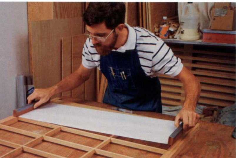
The shoji-paper covering is glued to the flush surface of the shoji frame and kumiko on the side that will face away from the room. A pair of clamping blocks helps the author keep the paper taut as it's lowered onto the shoji members that have been precoated with wallpaper glue.
