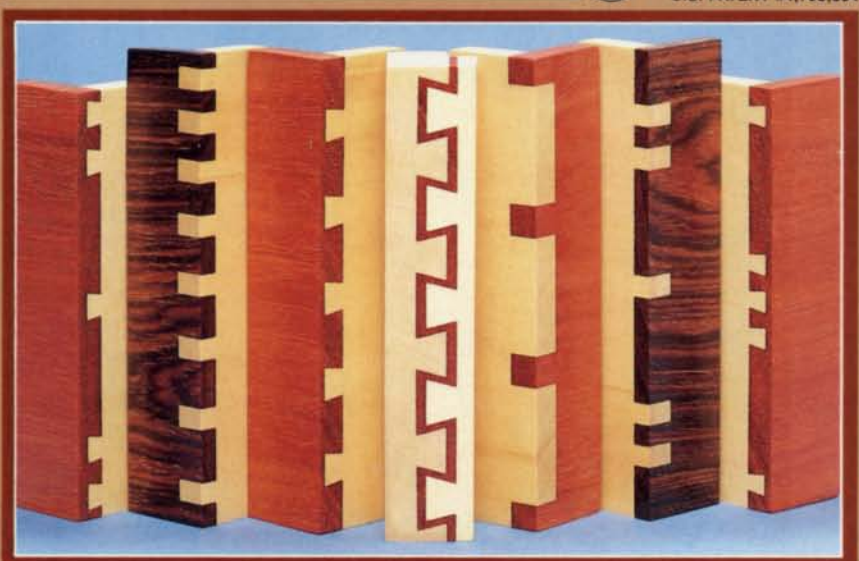
These joints were made using the new Incra Templates , with Incra Jig on the router table.
