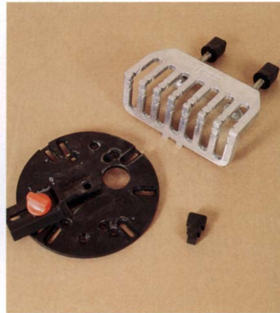
From top to bottom, the Sears model #2579, Porter-Cable model #5008 and Black & Decker model #C52331 can mill half-blind dovetails in pieces up to 12 in. wide.
