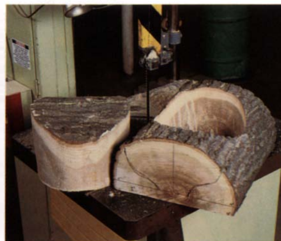
The curving profile of the bowl's lip is clear after bandsawing the circular blank. The more round the blank, the better balanced it will be when mounted on the lathe.
