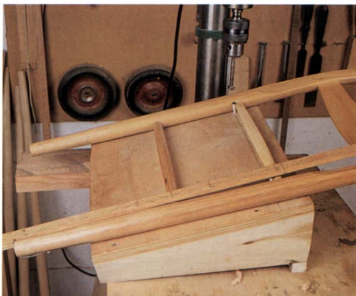
The rear frame is being set up on the drill-press table for boring the mortises for the side rungs. The frame sits on a form shaped like the bent rear leg post. This form and the shim under its far side, which raises the post being drilled, ensure that the mortises are drilled at the correct angle. Later, the front leg posts will be mortised in a similar way.
