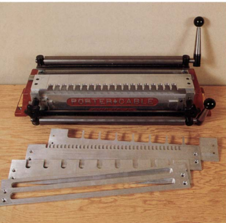
The well-built Omnijig owes its versatility to the several templates available for cutting fixed-space dovetails, finger joints, sliding dovetails and variable-spaced dovetails (not shown).
