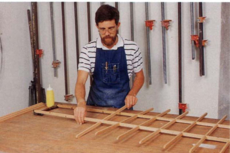
Erickson weaves the horizontal and vertical kumiko together, alternating the direction of the lap joints of each horizontal layer. A squeeze bottle is used to apply glue to each lap before it's assembled and pounded home with a hammer.
