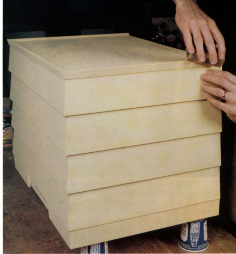
Redmond sands the first coat thoroughly to smooth any raised grain. Even the beveled edges get a once-over. You can see by the paint dust on the cabinet's top that flat latex paint can be sanded without clogging the paper.
