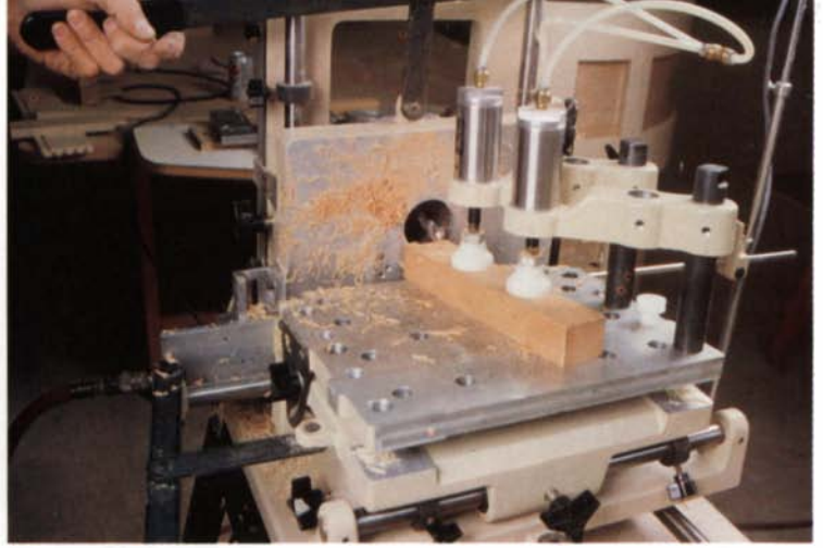
Left: To make a tenon, the wood is first clamped to the worktable, and then moved past the bit by a ball-bearing-tipped stylus that traces the template's profile, transferring its shape to the work. Right: A pair of optional air-actuated clamps holds the work firmly to the sliding table.
