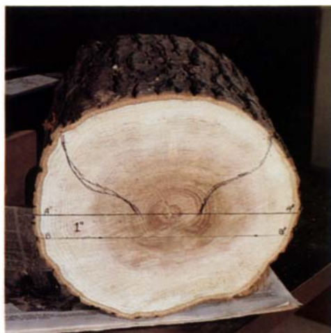
After selecting the section of log for your bowl, mark it off by drawing A-A' through the pith. The cutting line, B-B', is laid out 1 in. to the waste side of the first line.
