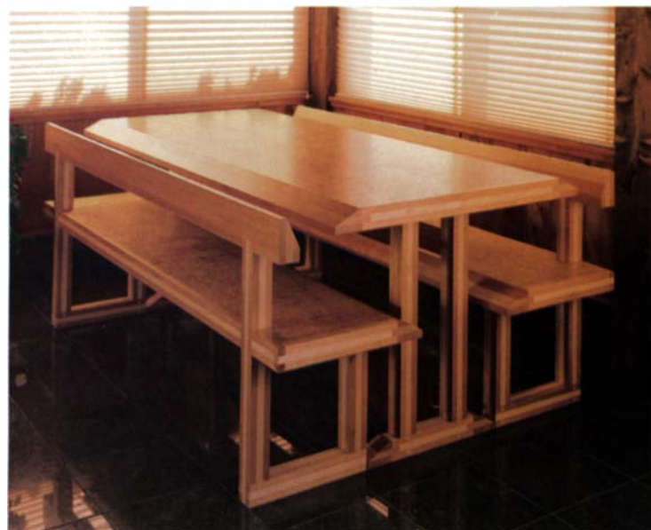
The author's nine-piece system results in very accurate mortise-and-tenon joints in this contemporary mahogany, maple and Japanese ash veneer trestle table.
