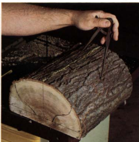
Connecting lines drawn perpendicular to the base on each end of the blank provide reference points to mark off the bowl blank centered on the growth rings.
