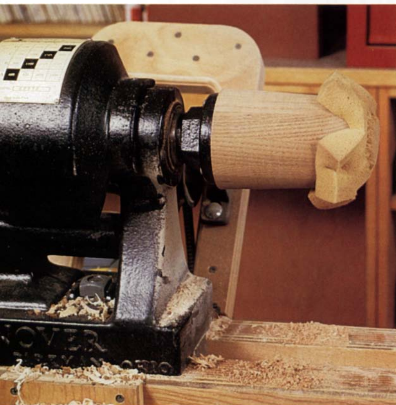
A bottom-turning mandrel is made by stapling a foam pad to a turned 4x4x6. The foam pad serves as a friction drive for the bowl that is held to the mandrel by the tailstock.
