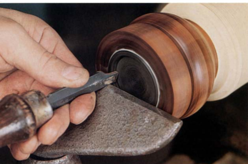
A shallow recess for a second inlay is cut into the first with a modified parting tool. The interiors of both the base and lid are turned to completion, and the lid is pressed onto the base to mount the inlays and shape the exterior of the box.
