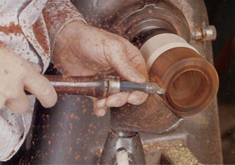
With a modified parting tool, the author turns a lip on the base to receive the lid. The base is glued to the waste block, which is mounted on a center-screw faceplate. The 2-in.-thick block holds the work away from the faceplate to allow access for tools to shape the bottom of the box.
