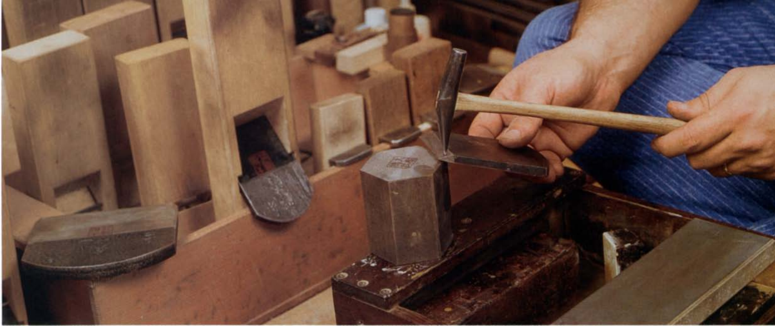
The author uses a small cross-peen hammer to gently tap out the blade, which is supported on the rounded corner of an anvil. Only the mild-steel portion of the bevel is struck. In this way, the hard tool steel, which is laminated to the mild steel, can be gently curved.
