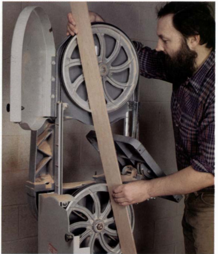
Laying a straightedge diagonally across the bandsaw's wheels allows the author to check the wheels for twist. This often requires the bandsaw table to be tilted out of the way.
