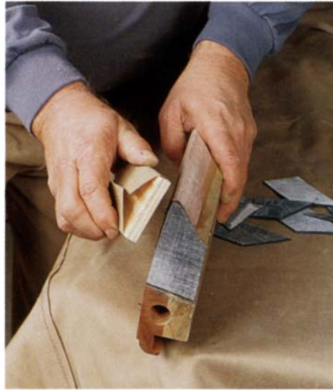
The cushion facing is contact-cemented to the angled rail end and cushion, then trimmed with scissors or a knife. The facing's sharp edge is eased with a sandpaper block so it won't tear the cloth when stretched tightly over the pocket angle.
