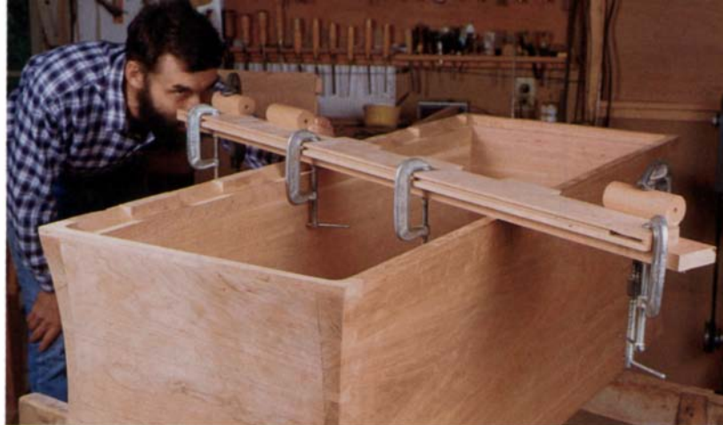
The author aligns the hinge segments by sighting through their holes while gluing them to the lid frame. The 1x4 clamped to the frame piece extends over the notched and angled edge to aid in clamping the hinge segments.
