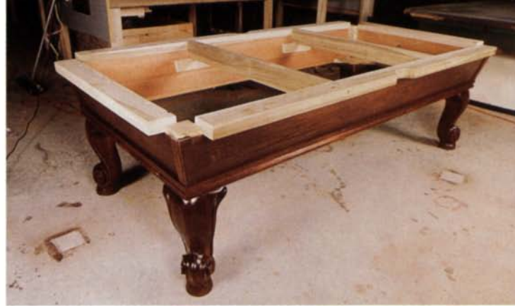
To complete the body, the slate frame is screwed to the top edge of the body frame, and the crossmembers are installed to support the joints in the slates. Glue blocks, screwed below the crossmembers, add support. The slate frame stops short of the corners to allow pocket clearance, and a 3/4-in. block ties the corner together.
