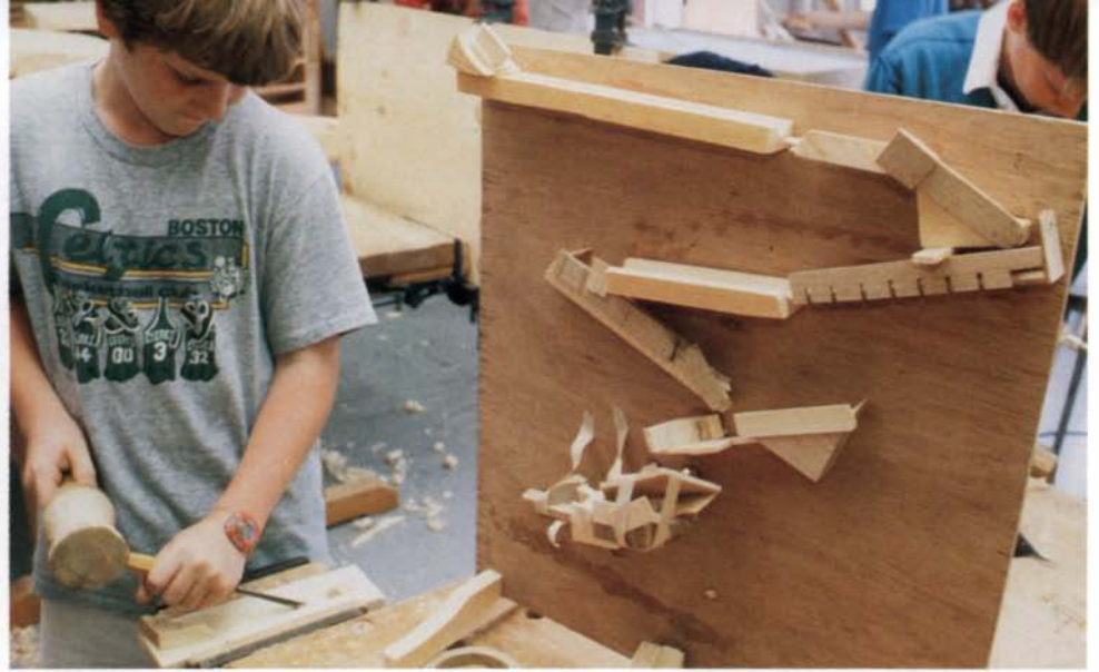
in a piece of pine. When this section of track suits him, he'll glue it in place on the plywood backboard. Masking tape provides the clamping power for odd-shape pieces used for tracks or guardrails.
