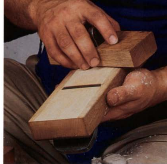
Meadow is shown here adjusting the sole of a plane, flattening its surface and removing any twist with a scraper plane. The wooden sole should be checked frequently so any necessary adjustments to compensate for wear or changes in environmental conditions can be made.
