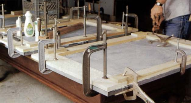
The 3/4-in.-thick poplar slate liner is glued with Titebond glue and clamped to the underside of the slate. The slate's sides are lined with 1x8s to overlap the pocket cutouts, then 1x4 crosspieces are butted between them and held back 1/16 in. from the slate edges that will butt together.
