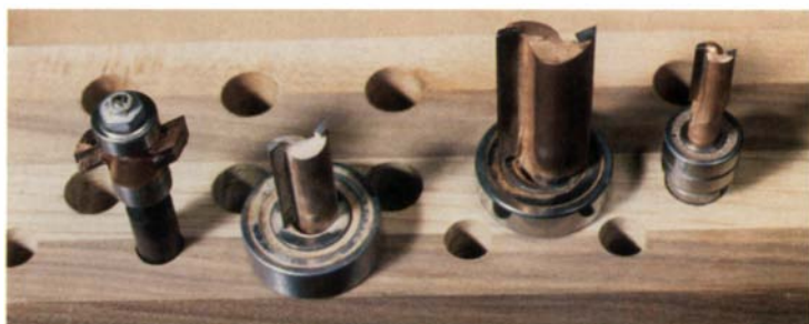
The author fits most of the router bits used for his complementary routing process with a ball-bearing or two slipped down on the shank, to serve as a pilot. Each bit/bearing combination is chosen to give a prescribed amount of offset, for snug-fitting joints.
