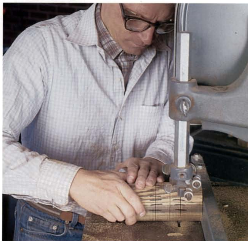
Christensen bandsaws the rough-turned cylinder into base and lid blanks. Thin kerfs, made with his narrow parting tool, are used to lay out the sections and guide the bandsaw blade. Marks across the kerfs identify lid and base sets and register the grain match.
