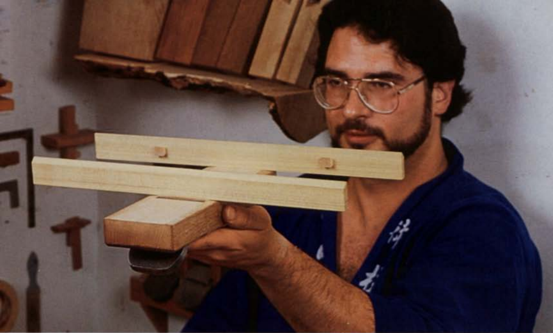
The author uses winding sticks to check the sole of this plane for twist in the plane's body. Using a single stick, Meadow will later check the sole for flatness.
