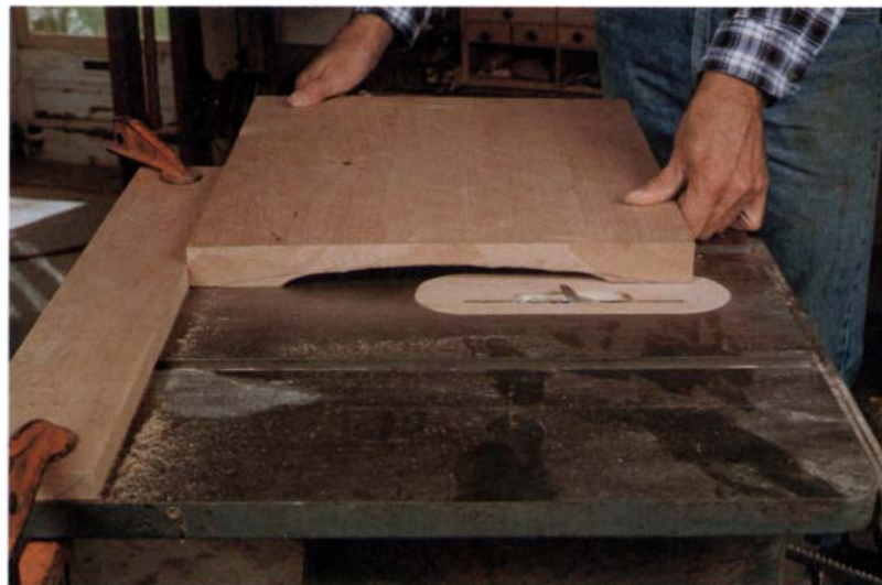
Dunham speedily roughs out the curved sides by running the work perpendicularly across a molding head fitted with ½-in.-radius cutters. To remove the waste up to his layout line, he adjusts the cutter height and the clamped fence, and runs opposite edges of the piece against the fence.
