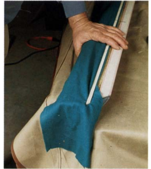
The feather strip is driven into the groove to within 6 in. of the corner-pocket ends. Here, about 2 in. of the cloth is pulled through the groove to create a wrinkle or 'pucker,' which helps stretch the cloth over the corner-pocket angle.
