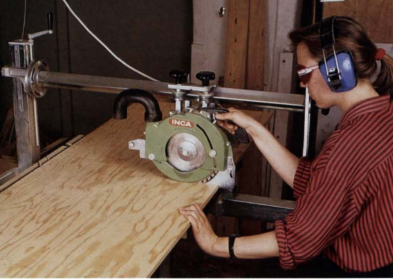
The Inca 810, shown above with the optional extension rail, is capable of crosscutting a 27½-in.-wide, ½-in.-thick panel.
