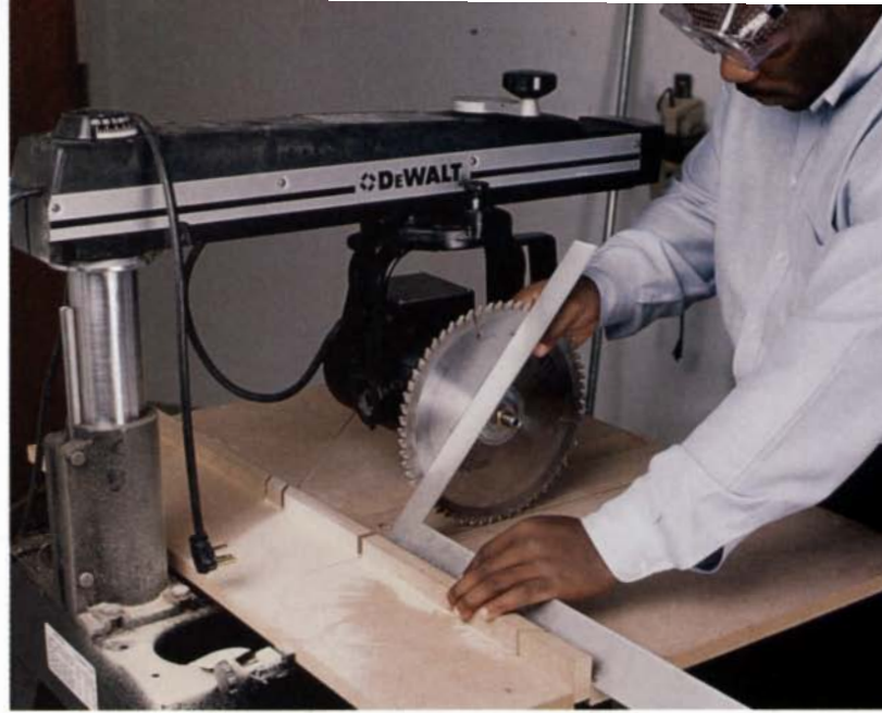
Vertical alignment is checked, above, with a framing square held at a 45° angle. One leg is against the blade and the other leg sits where the fence and saw table meet.
