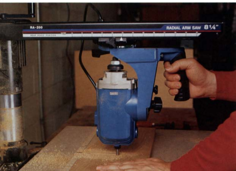
Ryobi's lightweight portable radial-arm saw (model RA200), above, has an 8½-in. blade that's capable of cutting 8/4 stock. The column and arm can be removed from the base for transport. Tapping the high RPMs of the router-type universal motor, the Ryobi is handy for plowing grooves, as shown below, or any other job using a router bit with a ¼-in.-dia. shank.
