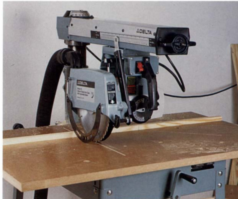
Delta's Model 10, shown above fitted with the optional leg set, is the only radial-arm saw tested with an on/off switch next to the handle for convenience and safety.
