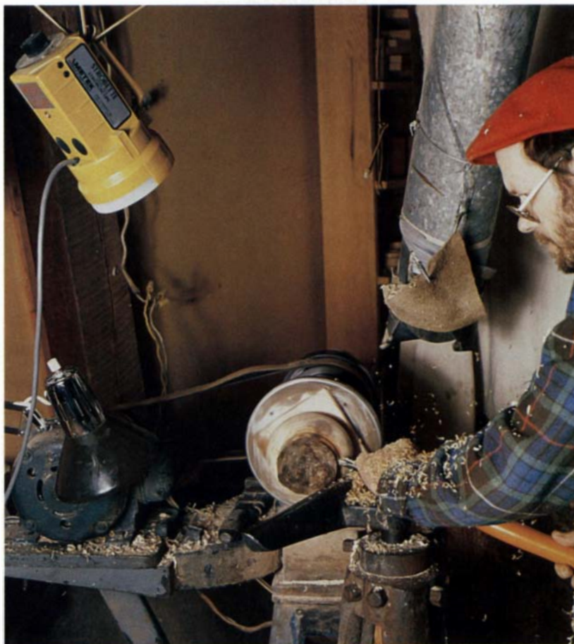
A strobe light freezes the image of a spinning natural-top box so it looks as if it's stopped and the shape of the edges and the grain pattern can be clearly seen.
