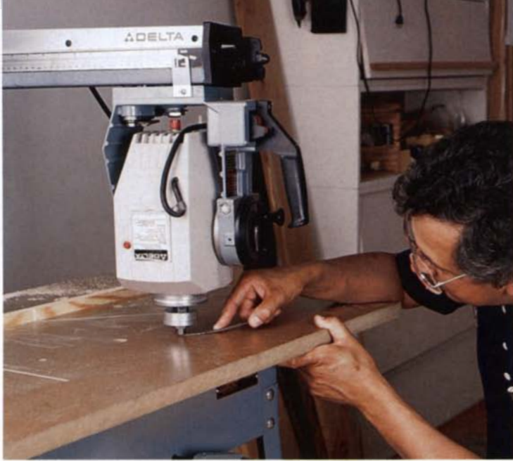
A feeler gauge checks the distance between the vertical motor arbor and the saw table so the table can be adjusted true to the arm.
