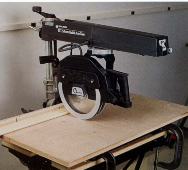
The Black & Decker 1712 is the only folding radial-arm saw with a 10-in. blade. The saw shown above is clamped to a Black & Decker Workmate to give it stability during cutting. Once the saw is positioned correctly and the loose table inserts are removed, the 1712 folds flat, below, for compact transport.
