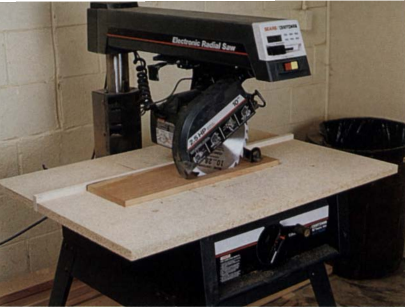
The Sears model 19825 comes with an electronic measurement display that shows the angle and height settings of the saw. The saw is set up in the photo for a rip cut, with the guard and antikickback arm in the correct position.
