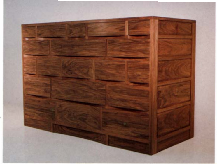
Although the author's walnut chest of drawers, above, has 19 dovetail drawers, his organized system of marking, cutting, assembling and fitting results in drawers with a piston fit. The piece has a frame-and-panel carcass and bent-laminate drawer fronts that provide a built-in pull underneath.
