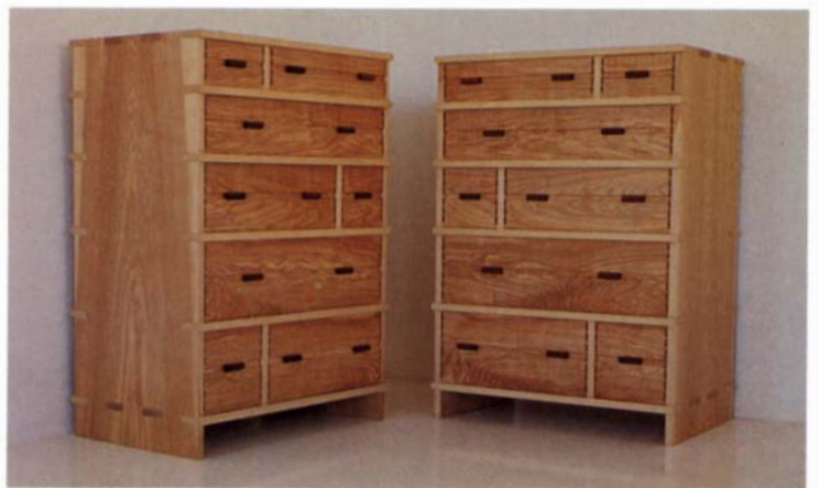
To achieve a pull that's integrated with the design of the drawer front, the author routs a cove in each front, then attaches a short section of dowel made from a contrasting wood for the pull. The through dovetails on the fronts provide another visual detail.
