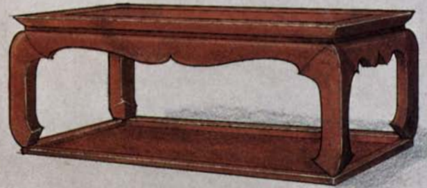
D. 15th Century A.D.—Legs are one solid-shaped piece, curved on outside. Bottom frame is still in use.
