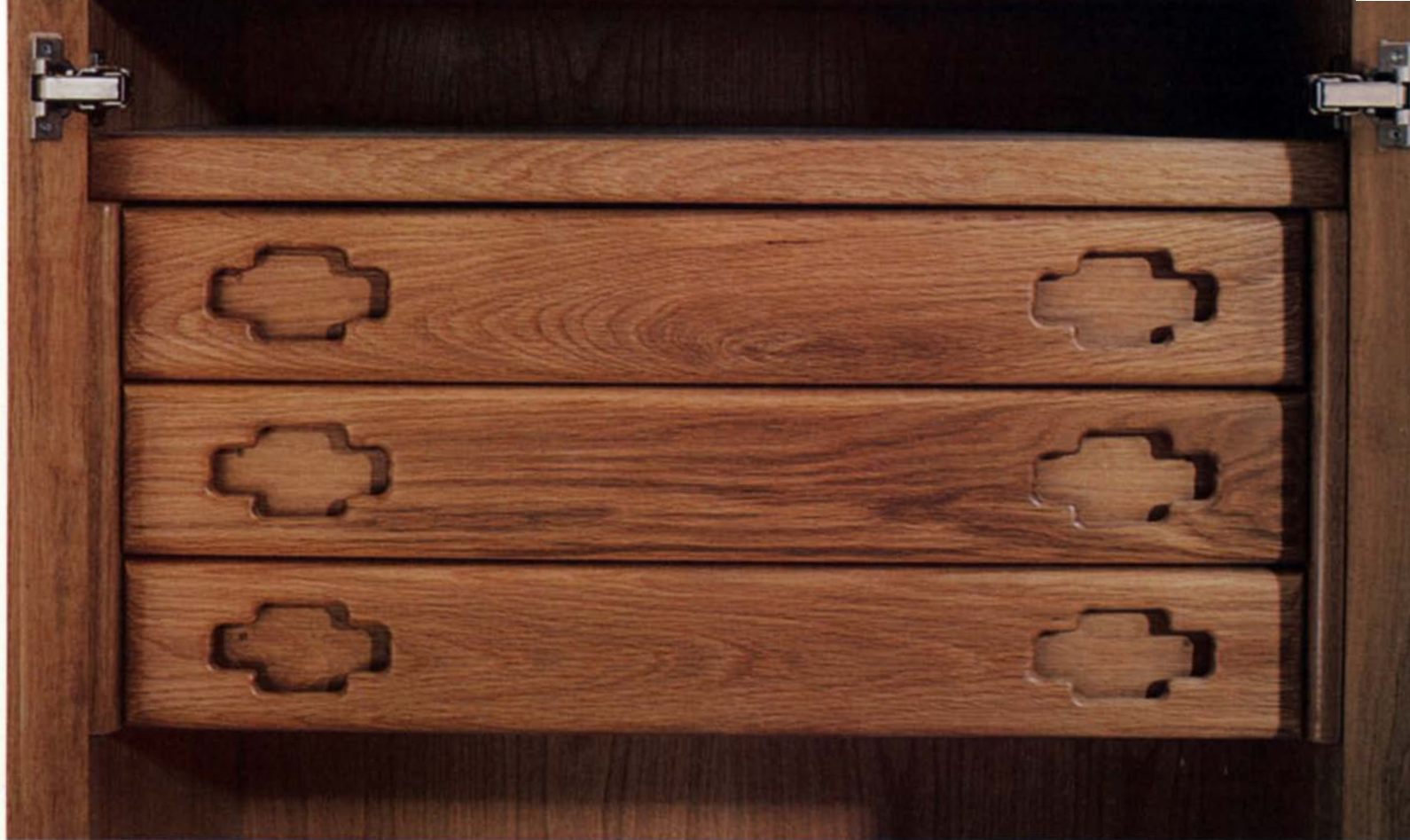
The inset pulls above were made by using the pattern-routing technique described in the text. This design can be used in solid-wood drawer fronts, or if routed into a stile then ripped in half, on adjacent door or drawer fronts.
