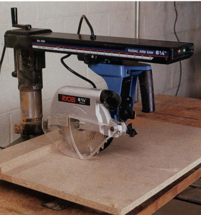
Ryobi's lightweight portable radial-arm saw (model RA200), above, has an 8½-in. blade that's capable of cutting 8/4 stock. The column and arm can be removed from the base for transport. Tapping the high RPMs of the router-type universal motor, the Ryobi is handy for plowing grooves, as shown below, or any other job using a router bit with a ¼-in.-dia. shank.
