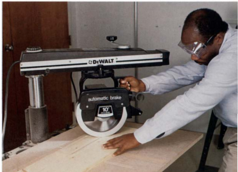
Set up for miter cutting, the DeWalt 7770-10, above, has its elevation crank atop its heavy cast-iron arm and all of its angle-setting controls within reach.
