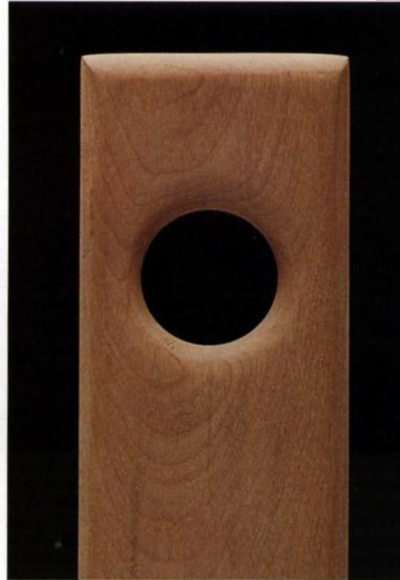
Button pulls, above, are simple to make and install. These are shaped using a plug cutter on a drill press and will be held in position with screws through the back of the drawer faceplate. Also easy to make is the stile pull, right, which requires only a drilled hole with smoothed edges. Stiles, 2 in. wide and glued to the drawer face in place of edging, provide plenty of material for routing pulls. The photo below shows routed maple stiles glued to the top of the door and bottom of the drawer face to form matching pulls.
