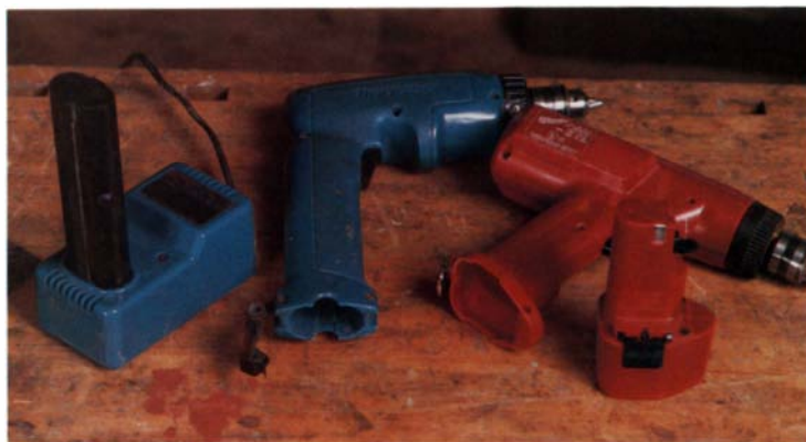
The removable battery packs on most cordless drills slide out of the grip or body for recharging, as shown here with the Makita 6093D (left) and the Milwaukee 0212-1 (right). The Makita's battery is shown in its dedicated charger, shown at far left. For continuous operation, one battery can be recharging while another battery is in the drill.
