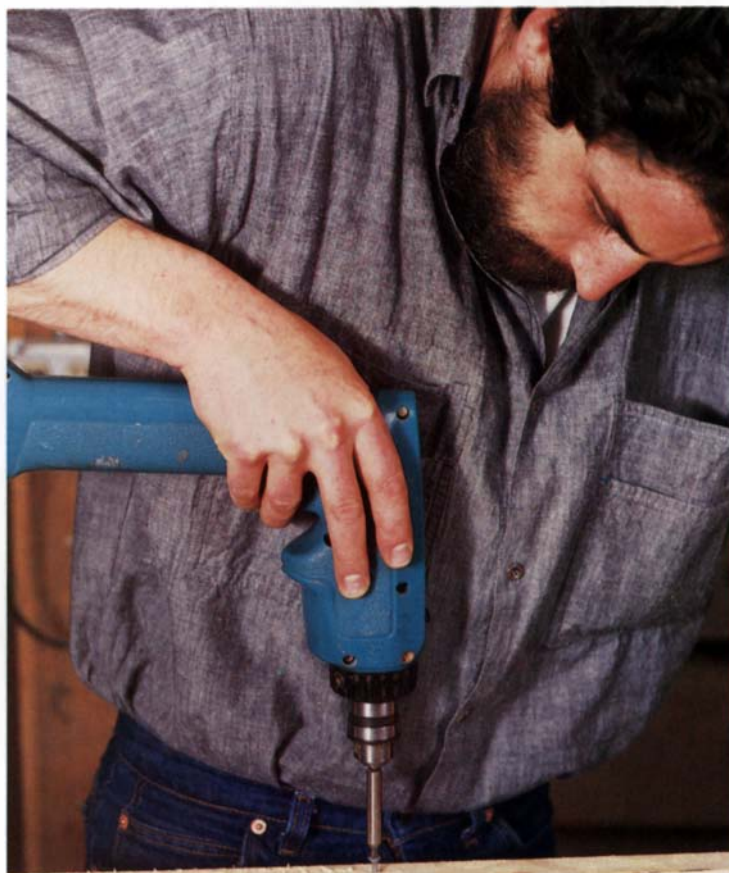
By offering a grip that's in line with the chuck, a cordless drill can be less fatiguing to hold, and it can thus allow the user to put more pressure behind the bit. Here the author uses a Makita 6093D to drive screws during the screw-driving and drilling tests performed for the survey.
