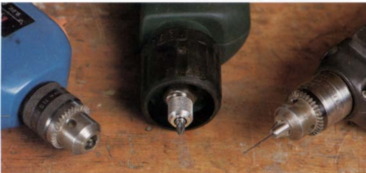
While all the cordless drills in the survey have chucks with a 3/8-in. maximum capacity, some drills, like the Skil (right), have chucks that will hold 1/32-in. bits or smaller. The cordless Metabo (center) features a special screw-driving bit holder that replaces the chuck and also allows bit change without a key. Chucks with knurled collars, such as on the Ryobi (left), make it possible to chuck up smaller drill bits without using a chuck-key.
