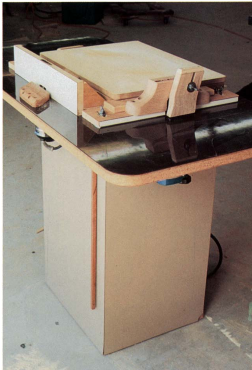
A freestanding table equipped with three routers is the key to the author's efficient and accurate drawermaking system. By moving drawer parts from station to station, a single worker can cut rabbet joints, groove the sides to house the drawer bottom and round all edges in a matter of seconds.
