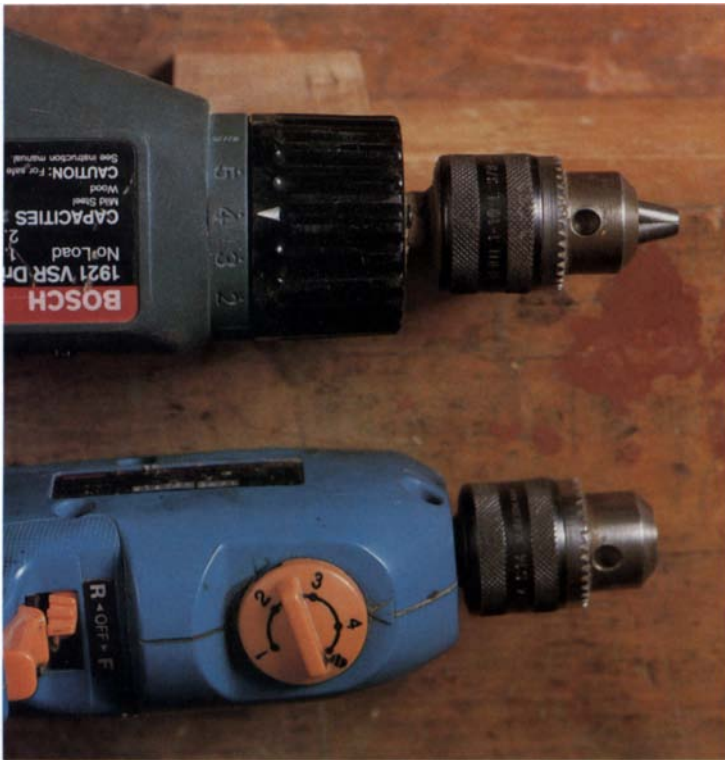
An adjustable clutch allows a cordless drill to regulate sensitively the maximum amount of drive torque delivered to the chuck—great for driving screws to the same depth. The Bosch cordless (top) has a clutch-adjusting collar just behind the chuck, while the Ryobi's (bottom) is under the body.
