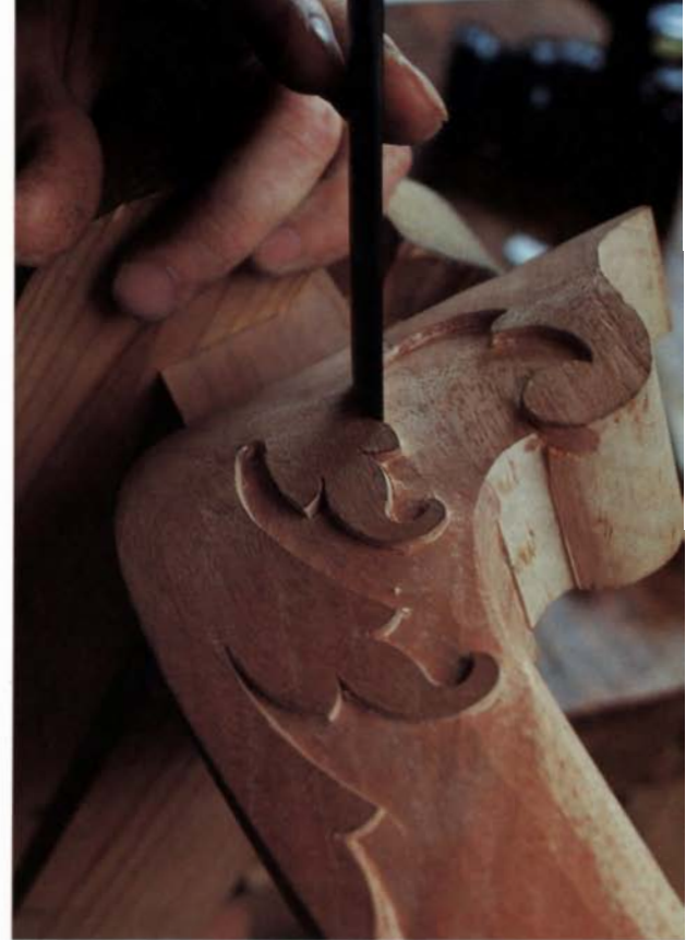
line in the same manner as the template itself is cut. Here, the background is being leveled down in a series of cuts to full depth. Stop cuts are deepened as necessary.
