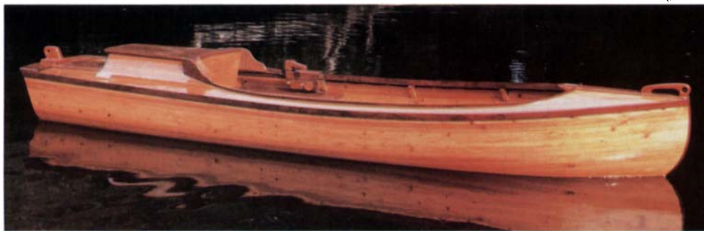
"Najos," one of Little's shallow-draft, battery-powered riverboats, is ideal for navigating the waterways in the coastal plains of North Carolina.
