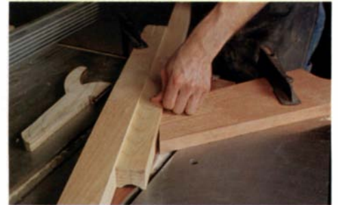
To cut a cove molding, run the workpiece along a fence angled to the blade. Make several shallow cuts, then rip the workpiece in half. Hold the work against the fence with a featherboard, using a push stick to finish the cut.
