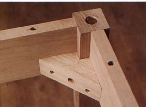
Glue blocks, above, glued and screwed at the bottom edge of the apron bolster the joint against damage from an accidental kick. The author's trademark, a penny let into the leg, dates the piece for posterity. Pulled home with clamps, the tenons, below, are pinned with 1/4-in. dowels.
