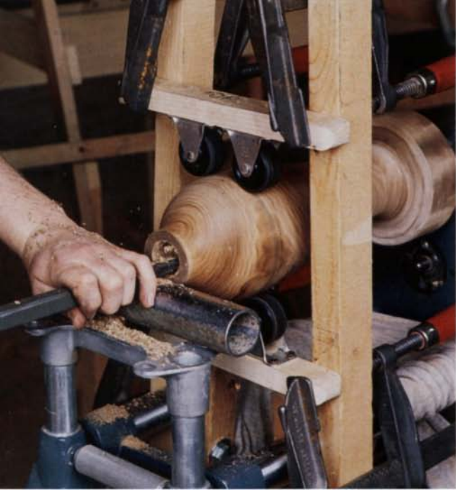
Deep faceplate work isn't the Shopsmith's forte, so Gillam ballasted the machine with granite and iron, then clamped on a steady rest made with furniture castors. Above, he's roughing the bowl's interior with a gouge made from an old file.
