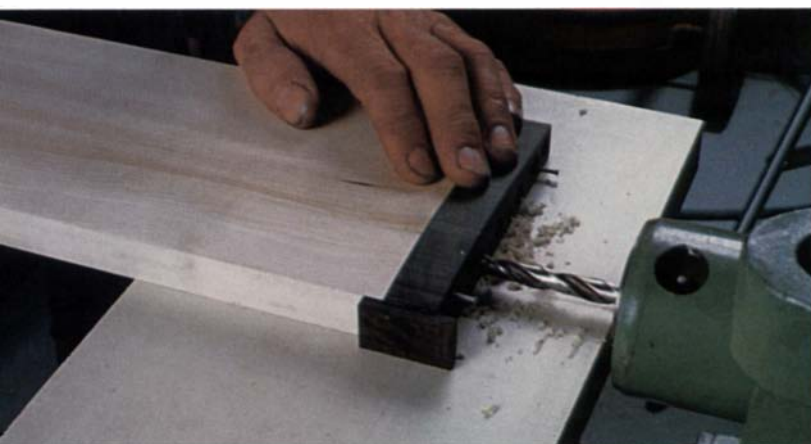
To accurately align dowels in parts being joined, the author makes a scrapwood doweling jig to serve as a boring guide. In the photo above, he has nailed the jig to the cabinet side for endgrain boring. Below, it's reversed and nailed to the cabinet bottom to bore matching holes. The doweling jig is bandsawn to the profile of the carcass side, and a heel is glued and nailed to one end to aid in alignment.
