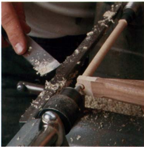
The hinges are made from a dowel turned from the same species of wood used for the box body. A shopmade caliper assures consistent diameter. A semi-circular rabbet bouses the hinge. It's cut on the router table with a core-box bit.
