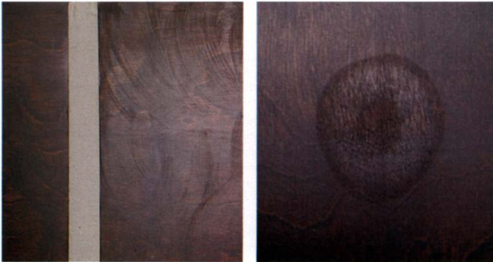
Above, left: If a wax is left on too long before the excess is buffed away, streaks will result, as seen on the right side of this test piece. Reapplying wax will soften the swirled coat so it can be buffed out evenly. Above, right: Wax will cause water to bead up and flow off, but it cannot protect against hot water after a spill. Despite the two coats of wax applied to this test sample, the grain of the maple plywood was raised and the wax dissolved after less than a minute of contact with hot water.
