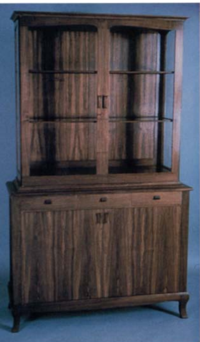
Robinson's rosewood china hutch, above, is also doweled. The lower carcass consists of a mock frame-and-panel structure doweled into a base and a solid-wood top, while the upper carcass is made of frames into which glass panes have been set. He stiffened the structure by gluing veneered panels into the solid-wood frames that form the backs of both upper and lower carcasses. Normally, panels would float freely in the frames.
