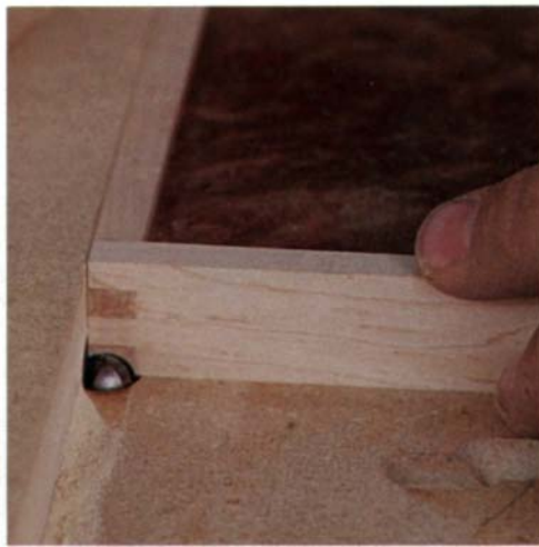
The hinges are made from a dowel turned from the same species of wood used for the box body. A shopmade caliper assures consistent diameter. A semi-circular rabbet bouses the hinge. It's cut on the router table with a core-box bit.
