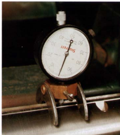
The cutterhead gauge base allows a dial indicator to be used for setting the depth of the knives in the cutterhead. While the base rides on the head itself, the indicator's tip rides on the blade's edge and registers its height on the dial.
