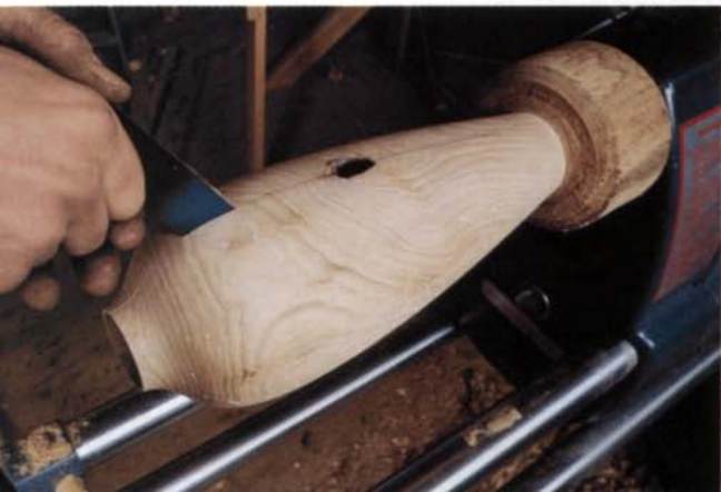
After turning, the vase is sawn along its length. The edges are beveled so they can bend past each other more easily. In the center photo, Gillam pares a teardrop-shaped bevel for clearance. Ten minutes of boiling plasticizes the butternut enough for bending.
