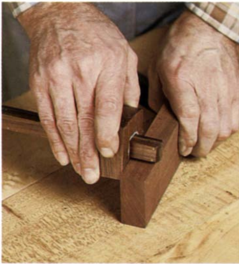
The mortise gauge scribes two parallel lines for marking mortise-and-tenon joints or grooves to be plowed out with a multiplane. The distance between the points is adjustable, as is the position of the fence on the beam.
