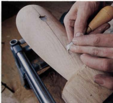
After turning, the vase is sawn along its length. The edges are beveled so they can bend past each other more easily. In the center photo, Gillam pares a teardrop-shaped bevel for clearance. Ten minutes of boiling plasticizes the butternut enough for bending.
