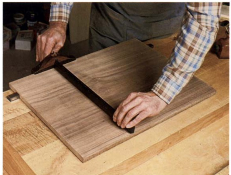
Although it's an uncommon marking tool, the panel gauge is handy for marking a panel or a wide board to be bandsawn to consistent width. Two hands hold the long-beamed gauge for stability and to get a clean scribe line.
