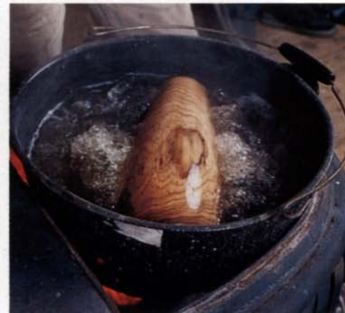
After turning, the vase is sawn along its length. The edges are beveled so they can bend past each other more easily. In the center photo, Gillam pares a teardrop-shaped bevel for clearance. Ten minutes of boiling plasticizes the butternut enough for bending.
