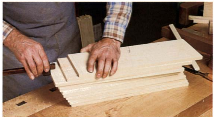
To make marking a set of drawer sides quick and orderly, stack the sides and mark your way down through the pile. Mark each set of ends in sequence to minimize the risk of mismarking similar pieces or skipping a piece.
