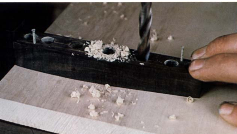
To accurately align dowels in parts being joined, the author makes a scrapwood doweling jig to serve as a boring guide. In the photo above, he has nailed the jig to the cabinet side for endgrain boring. Below, it's reversed and nailed to the cabinet bottom to bore matching holes. The doweling jig is bandsawn to the profile of the carcass side, and a heel is glued and nailed to one end to aid in alignment.
