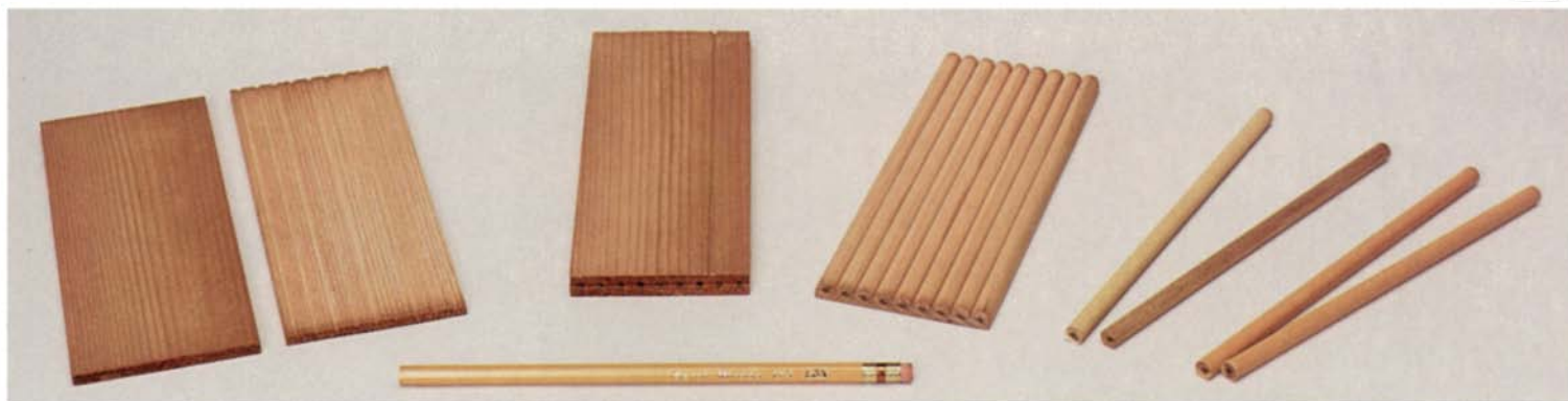
Pencils are made from clear incense cedar slats cut from California trees that are 250 to 300 years old. Nine pencil leads are glued up between two cedar slats. The glued-up slats are shaped and then cut apart to make nine pencils.
