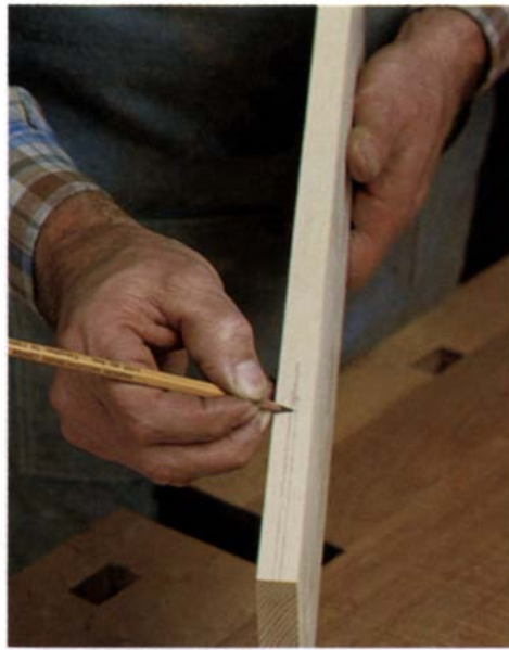
Using a tightly held pencil as a marking gauge, Klausz marks the board's edge from both sides to find its center.
