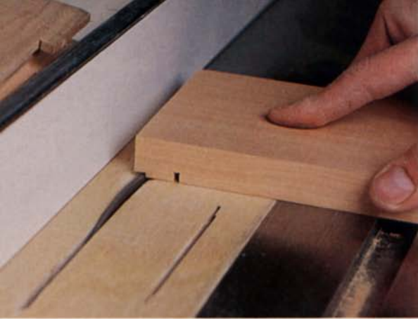
For tenoning with a single setup, above, the table saw's cutting depth is set to the shoulder depth, the fence (or a stop block) to the shoulder length. With the stock held firmly against the miter gauge, multiple passes form the cheek.
