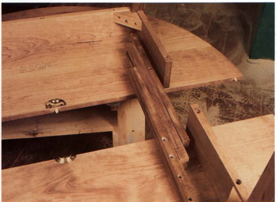
Wooden extension slides convert an ordinary table into one that expands. To install the slides, the top is attached to the base and the slides are screwed to the underside of the top. Then the base is removed so the apron rails can be table sawn, above, using a miter gauge. A scrap taped to the apron acts as a shim, preventing binding during the cut. A brass latch, below, locks the leaves together.
