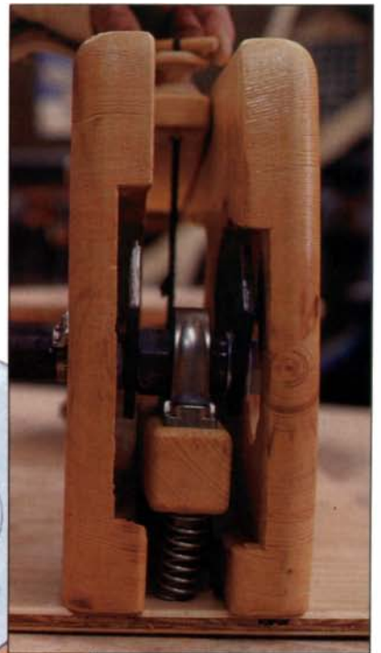
A pair of eccentrically mounted steel weights bolted to a pillow-block bearing generate the saw's reciprocating action. The motor is connected to the reciprocal drive through a rubber hose, which acts as a flexible shaft.
