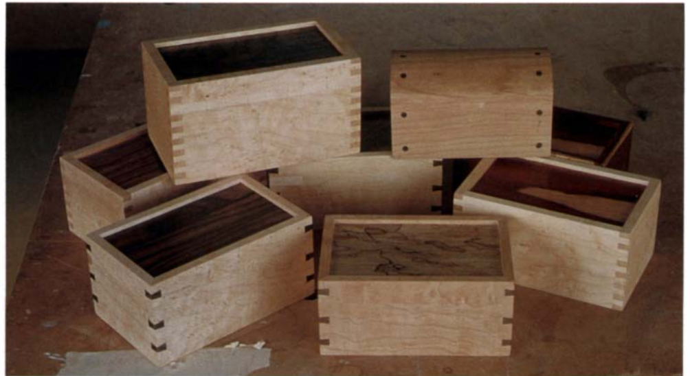
With corner joints suited for quick construction on a router table, the author's small wooden boxes are a practical, profitable craft item.
