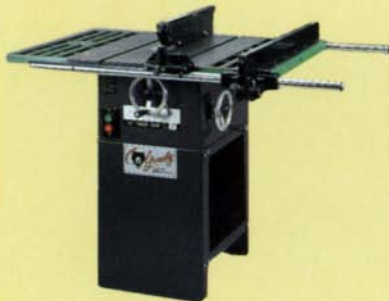
MODEL G1022 10" TABLESAW Precision ground cast iron table & wings. T-slots in table. 1 1/2 HP Motor. Weighs 235 lbs. Regularly $325.00 SALE $295.00
