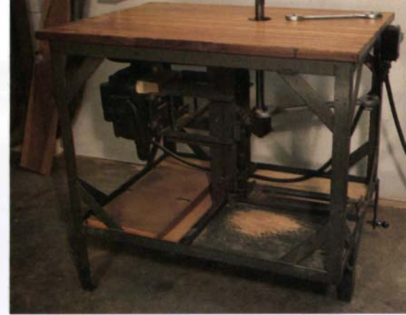
On Weaver's saw fence (left), a threaded rod sets the fence parallel to the blade, and a turnbuckle keeps the fence's face perpendicular to the table. To make it easier to change shaper cutters, Weaver welded a steel finger to the machine's frame. An open-end wrench extending from the finger to the spindle (above) locks the shaft, so Weaver has two free hands to tighten cutters.
