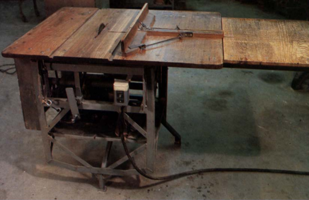
On Weaver's saw fence (left), a threaded rod sets the fence parallel to the blade, and a turnbuckle keeps the fence's face perpendicular to the table. To make it easier to change shaper cutters, Weaver welded a steel finger to the machine's frame. An open-end wrench extending from the finger to the spindle (above) locks the shaft, so Weaver has two free hands to tighten cutters.
