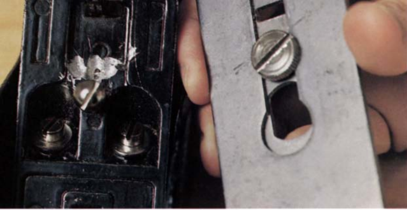
In order for the cap screw to clear the frog casting, allowing the blade to be adjusted, the author had to drill out a small area on the top side of the Menard's frog, as shown above.
