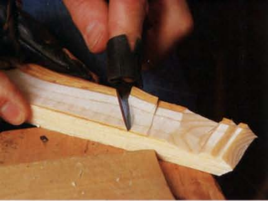
In a few deft strokes, Menard pares a point on the blank's end, forms notches that later interlock the feathers and, above, cuts a diagonal notch where the feathers meet the body. Right, the tail feathers are split out by pushing the knife into the end-grain. The cut is stopped at the diagonal notch. A central feather is removed to allow the knife additional room.
