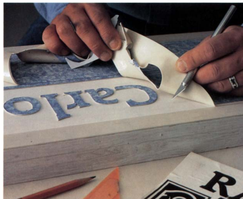
After cutting is completed, background areas of the stencil are stripped from the sign blank, leaving the stencil on the letters.
