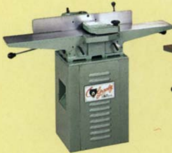
MODEL G1182 6" JOINTER 7 x 47" Precision ground bed. 1 HP. Motor. Weighs 265 lbs. Regularly $325.00 SALE $295.00
