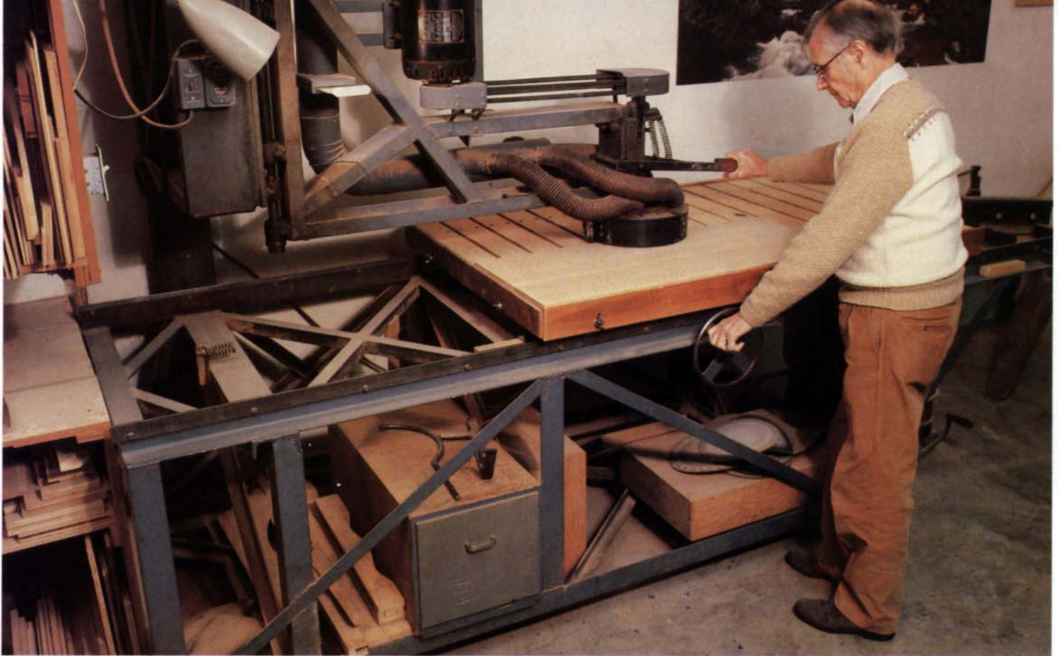
Alvin Weaver built his homemade radial-arm sander in 1948. By cranking the handle in his left hand, Weaver moves the table under the sanding head, which pivots at the column and is pressed to the work with the lever in Weaver's right hand.
