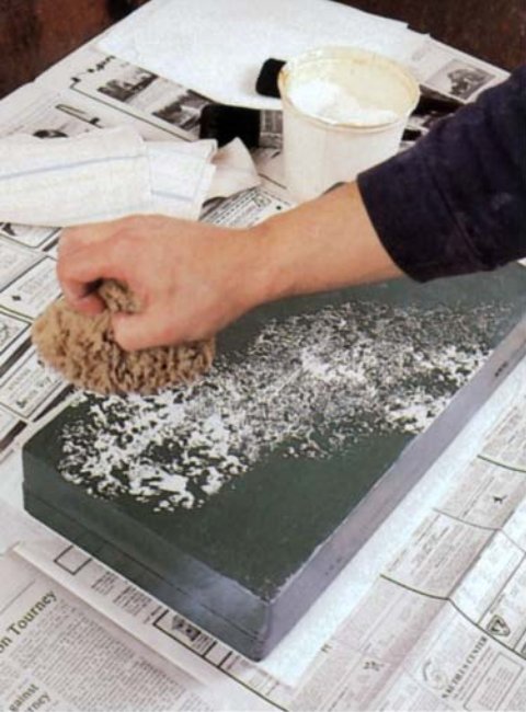
White paint—sponged on in cloudy, diagonal patterns called drifts—is applied to create the feeling of movement across the stone (above, left). A dry brush blends the drift with the green undercoat (above, right) to make the marble look more realistic.
