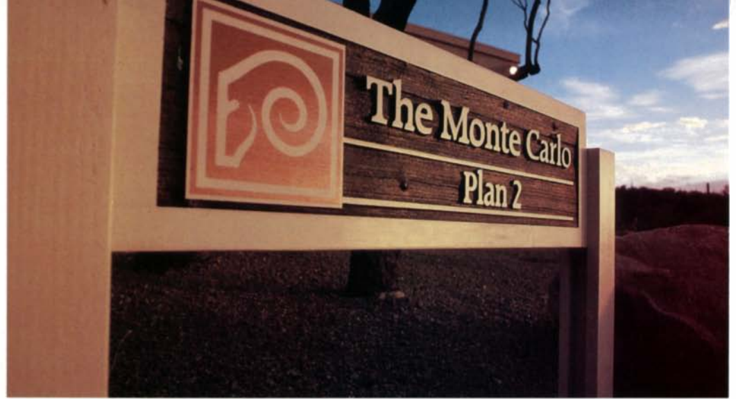
After the sign is blasted and the background is painted, the remaining stencil is stripped from the foreground, as shown at left. Quartersawn stock gives the background a linear appearance. Above, a close-up of the sign after installation. Painted with earth tones, it's noticeable but also blends well with its location.
