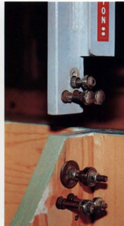
With its guard and the top wheel removed, the saw's blade-tensioning assembly (above, left) is exposed. The assembly is raised higher than normal to show the tracking assembly behind it. The blade guard slides in tracks screwed to the saw body. Blade guide bearings (top right) are made of ball bearings on threaded rods or bolts. The top backup bearing in the upper trio is smaller than the bottom backup bearing because it's a temporary replacement. The author burned out the original bearing after three years of use, milling logs into lumber.
