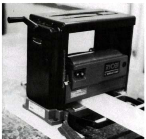
The Ryobi AP-10's small size and light weight make it ideal for on-site planing.
