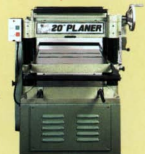
MODEL G1033 20" PLANER 20 x 8" Capacity. 2 Automatic feed speeds. 3 HP motor with magnetic switch. Weighs 960 lbs. Introductory Price $1295.00
