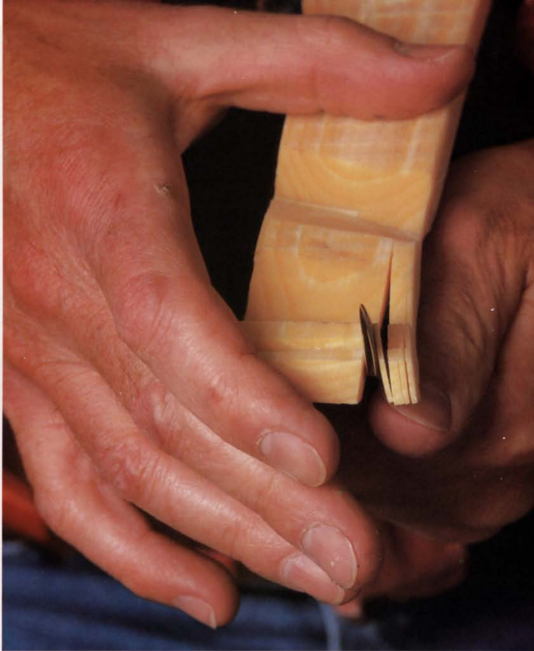
In a few deft strokes, Menard pares a point on the blank's end, forms notches that later interlock the feathers and, above, cuts a diagonal notch where the feathers meet the body. Right, the tail feathers are split out by pushing the knife into the end-grain. The cut is stopped at the diagonal notch. A central feather is removed to allow the knife additional room.
