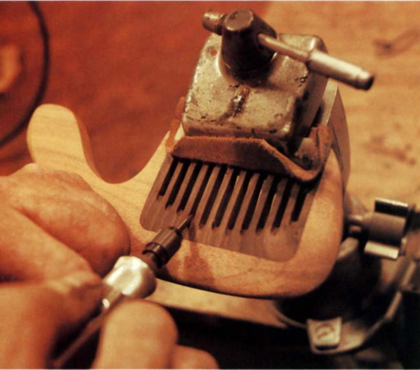
After cutting the teeth, the top of each groove is relieved with a carbide cutter in a Foredom flexible-shaft handpiece.
