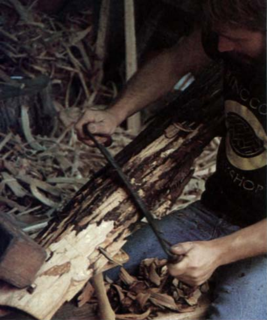
2. After soaking the peeled slabs for a day, the author removes the rough outer bark with a drawknife.
