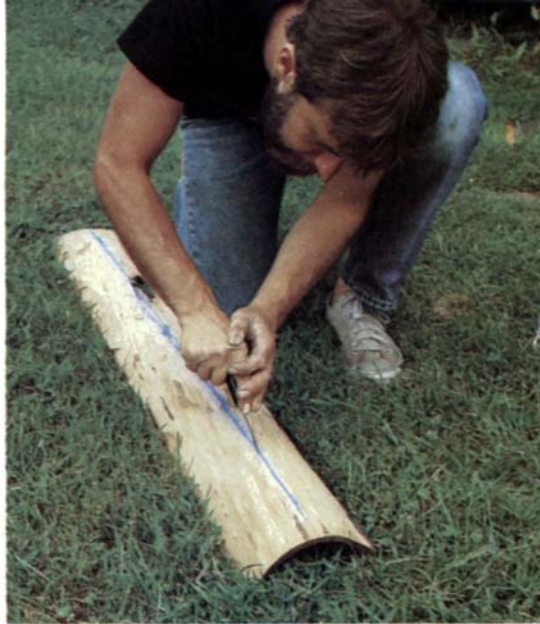
3. The debarked slab is cut into strips with a stout knife or ripped on the table saw. The hold-down shown at right makes for safe table sawing.
