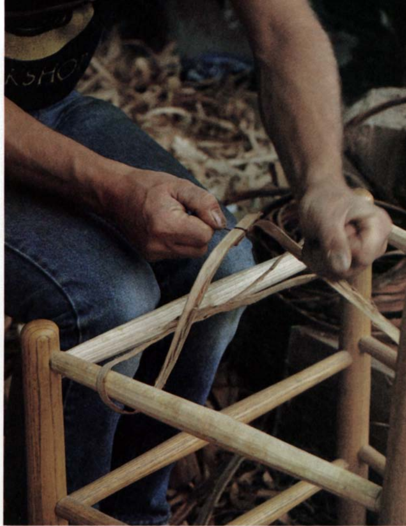
7. As more warp length is needed, bark strips are spliced on by tying them with thread let into notches cut about 4 in. from the end of each strip.
