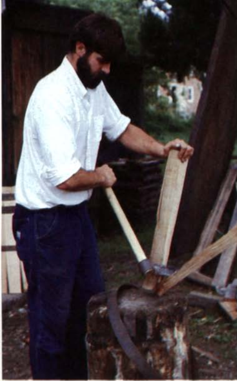
Raiselis twists his froe through a quartered block of green oak to split out stave blanks, left, then tapers and bevels each piece with a side axe. After shaping the outside of the stave with a straight drawknife, he uses a hollow shave, above, to scoop out the inside face so the stave can be more easily bent. The long butt joints on the staves are jointed and beveled on a cooper's jointer, which looks like an oversized, upside-down cabinetmakers' plane, right. The plane can be finely set, making it better than a power jointer for this operation.
