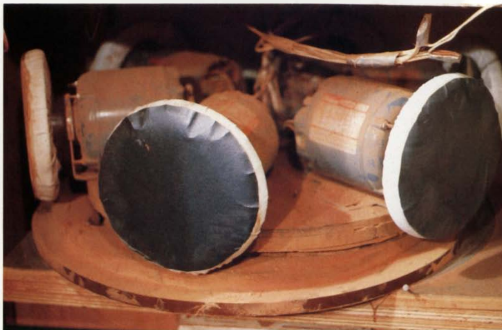
A gangsaw (above) cuts all the teeth in one pass. The cross-cut fence that holds the comb is designed to stop over the center of the arbor. At this point, the saw is switched off and the comb removed. Carpenter's sanding machine (right) consists of six 1/4-HP motors mounted on a lazy Susan. Each padded sanding disc sports a different grit paper.
