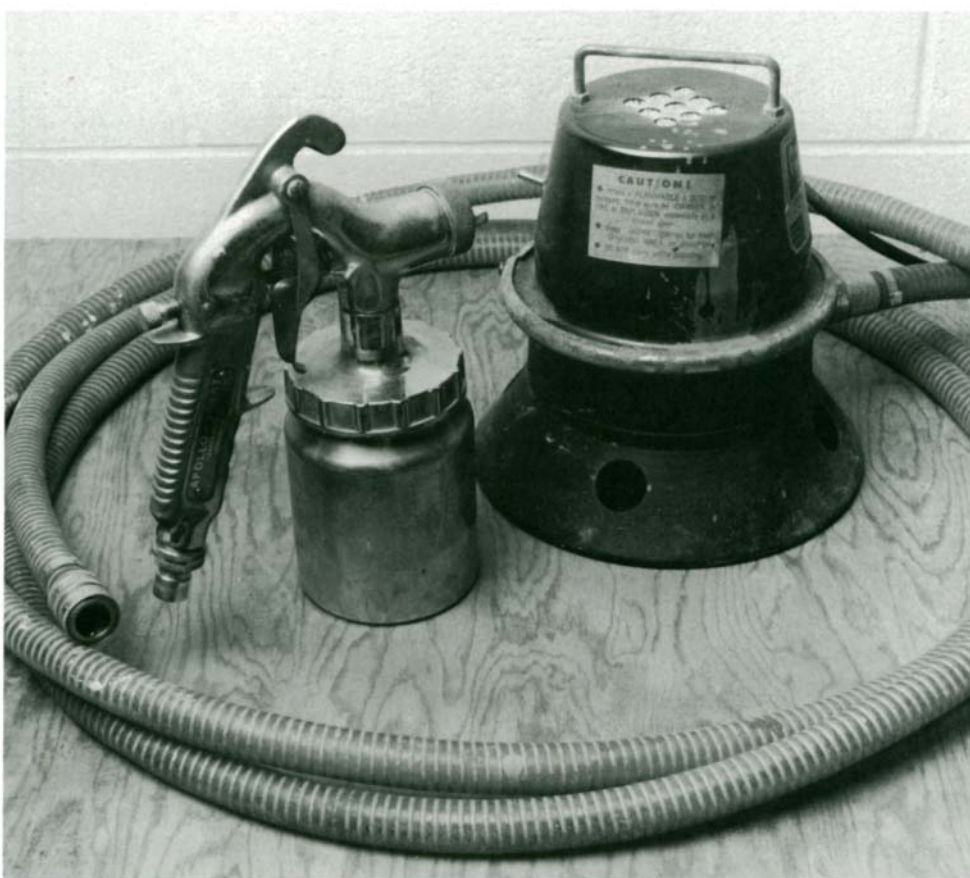
Low-pressure spray finishing systems, such as the Apollo 500 shown here, are an alternative to conventional compressed-air systems.
