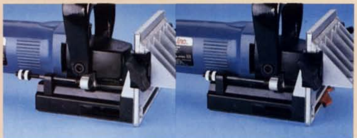
Depth can be regulated by means of two jam nuts.
