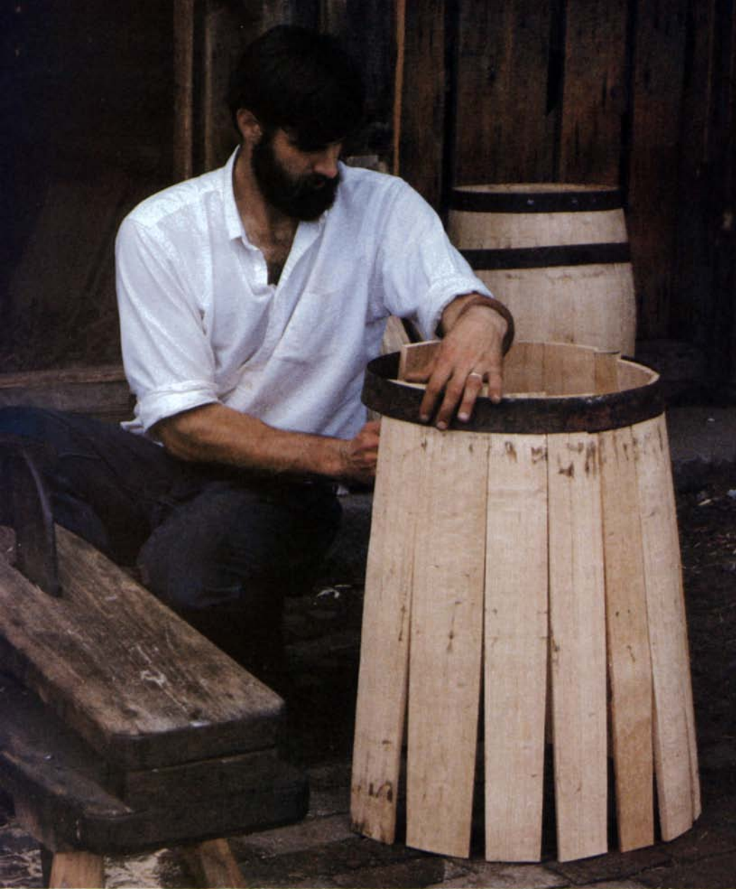
Staves are 'raised up' in an iron hoop that sets the barrel diameter. Raiselis steadies the staves with his left forearm as he adds more staves with his right hand.
