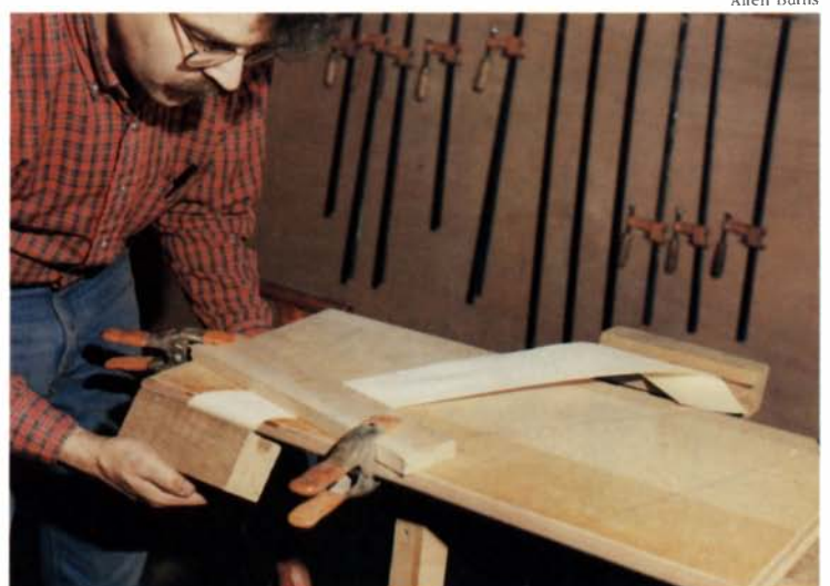
Duffy bends dampened veneer around a bullnose former. The bend is then fixed with a heat gun.
