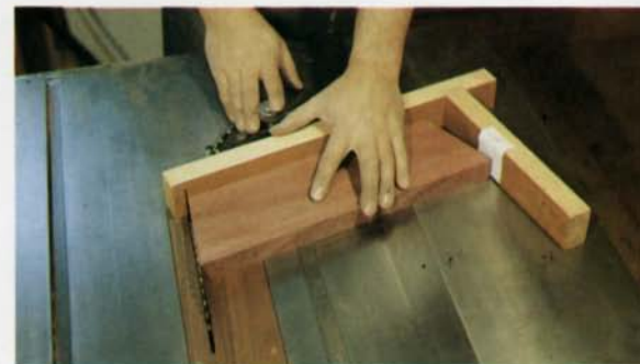
Segments of banding are precisely cut to length and end angle using this L-shaped jig attached to the miter gauge. Photo shows second end being cut, and the paper shims that allow fine adjustment.
