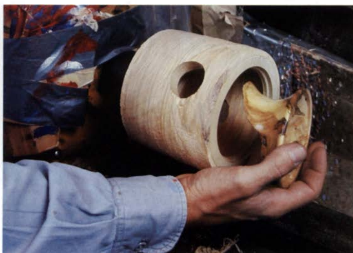
Mode's wooden chuck allows him to turn shallow-domed lids or lids with irregular projections. The holes allow him to gauge the lid thickness. A wooden collet chuck can be made with a piece of springy hardwood and a hose clamp (shown below).
