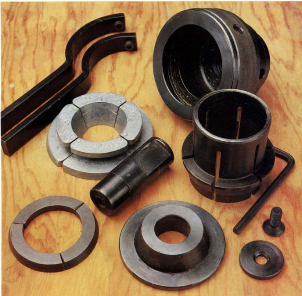
The Precision Combination Chuck comes with the accessories shown above, except for the optional spigot chuck at center right. The dovetail collets expand to grip a recess turned in the bottom of a bowl, top right. The pin chuck fits into a 1-in. hole, center left. When the bowl is rotated, it locks in place. The optional spigot chuck accessory is ideal for turning boxes. The Precision requires two C wrenches to change accessories.
