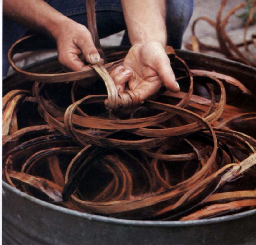
5. Before splitting, Shriver soaks his strips until they’re supple enough to bend easily around his fingers.
