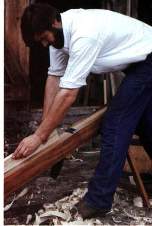
Raiselis twists his froe through a quartered block of green oak to split out stave blanks, left, then tapers and bevels each piece with a side axe. After shaping the outside of the stave with a straight drawknife, he uses a hollow shave, above, to scoop out the inside face so the stave can be more easily bent. The long butt joints on the staves are jointed and beveled on a cooper's jointer, which looks like an oversized, upside-down cabinetmakers' plane, right. The plane can be finely set, making it better than a power jointer for this operation.
