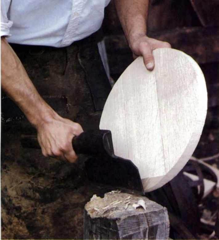
The bevel around the circular head, or end, of the barrel is roughly shaped with a side axe and finished with a heading knife.
