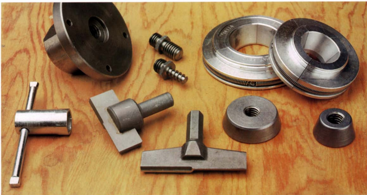
Delta's Super Chuck Kit comes with two expanding collets, two wing cutters to cut the collet recesses, and a screw chuck. The backing plate doubles as a small faceplate. The split ring expands outward to lock into a recess cut in the bowl bottom.
