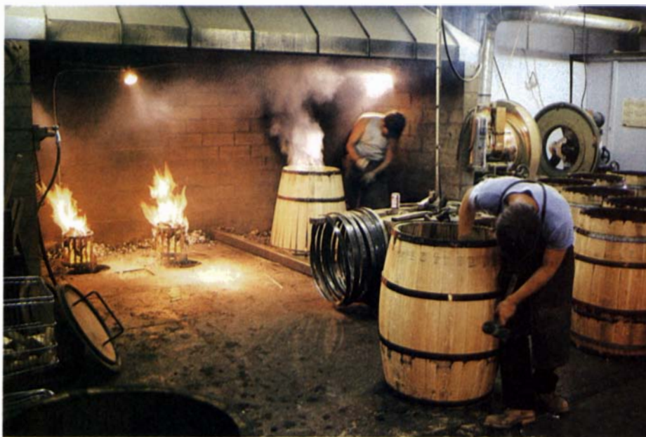
Fires burn in iron cressets as a cooper wraps a power winch cable around the hot staves. The cooper in the foreground is fitting a hoop on a 3-ft. tall barrel.
