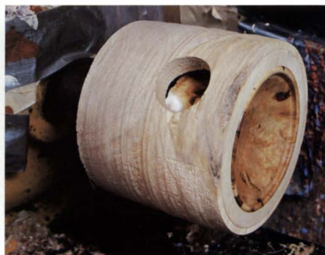
Mode's wooden chuck allows him to turn shallow-domed lids or lids with irregular projections. The holes allow him to gauge the lid thickness. A wooden collet chuck can be made with a piece of springy hardwood and a hose clamp (shown below).
