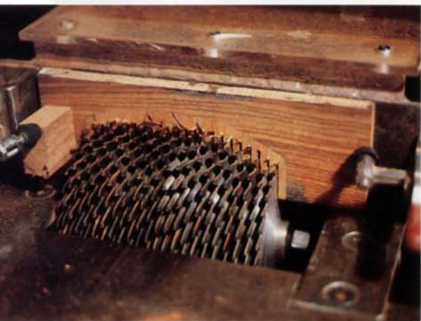
A gangsaw (above) cuts all the teeth in one pass. The cross-cut fence that holds the comb is designed to stop over the center of the arbor. At this point, the saw is switched off and the comb removed. Carpenter's sanding machine (right) consists of six 1/4-HP motors mounted on a lazy Susan. Each padded sanding disc sports a different grit paper.
