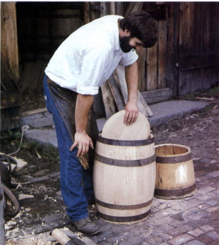
Before snapping the head into the croze, Raiselis refines the bevels with a heading knife, which is curved for cutting endgrain.
