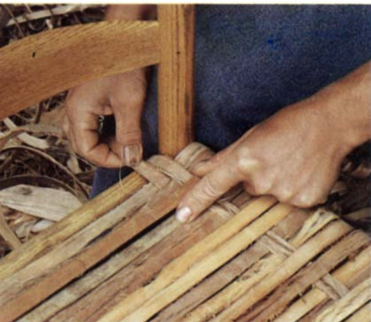
9. The first weave moves toward the front of the chair, passing first over two strips, then under two strips, and so on.
