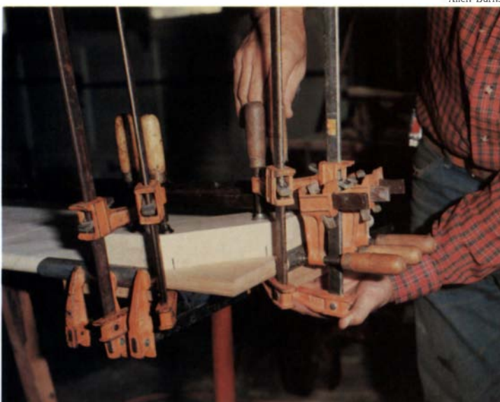
Aluminum tube, split lengthwise, serves as a caul for gluing the bend. Wooden cauls distribute pressure on the flat surfaces.
