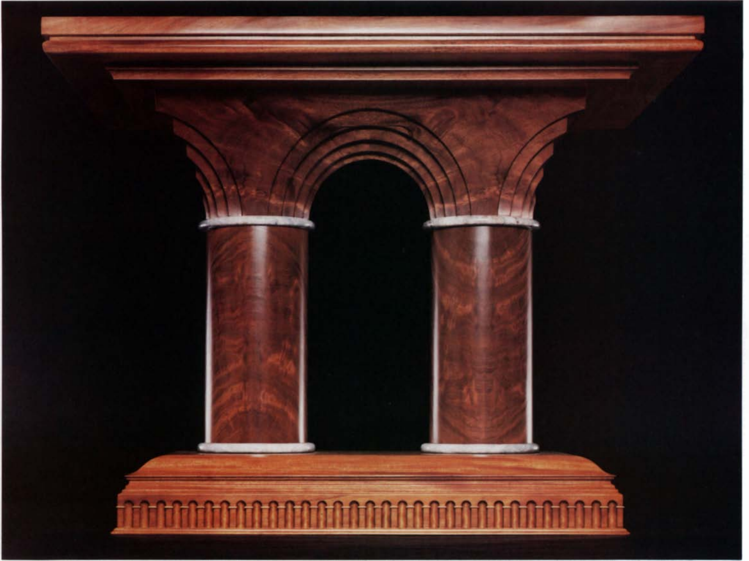
The columns of Tom Fannon's altar are veneered in figured mabogany wrapped around a plywood-covered frame. Thin marble slabs separate the columns from the solid-mabogany top and plinth.
