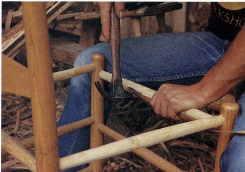
6. Shriver begins the warp by tacking a strip inside the front rung. The strip is carried under, around and over the side rungs.
