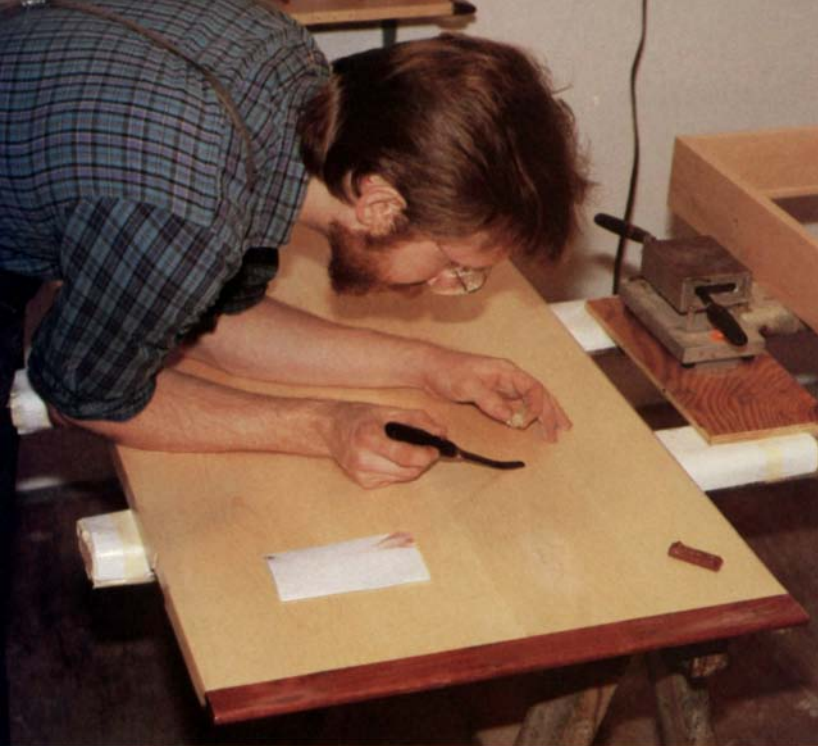
A good lacquer finish begins with a meticulously prepared surface. Above, Johnson repairs a minute flaw with a hot knife and a burn-in stick. Patches will later be matched with blending-powder stains.
