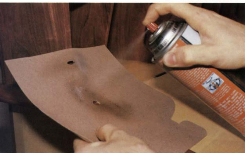
Even a multi-coat lacquer finish is only a few thousandths of an inch thick so rub-throughs are inevitable. They're repaired by spot touch-ups with aerosol lacquer. Johnson has masked the desk's pencil trap (middle) and he uses thin cardboard to mask the aerosol's spray pattern (above).
