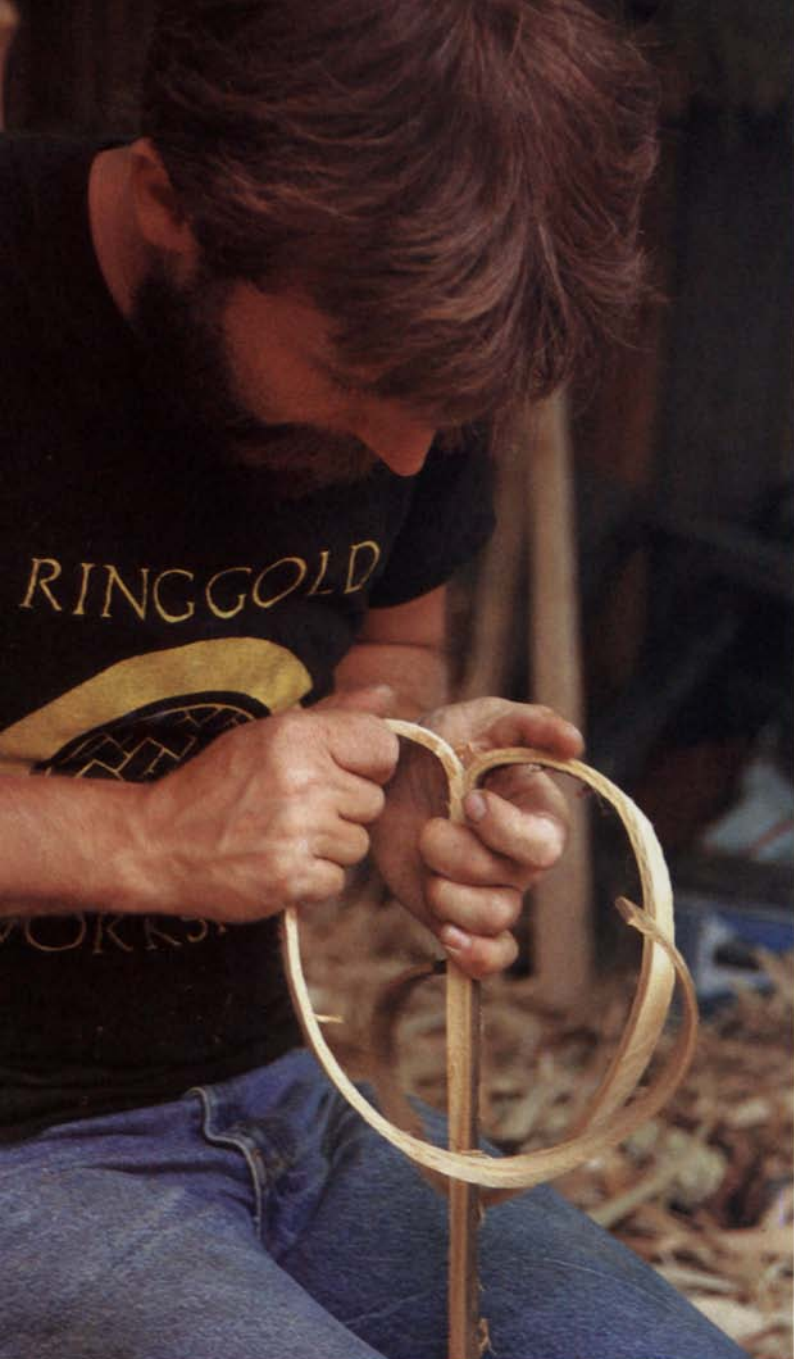
4. Bark from old trees is usually thick enough to be split three or four times, yielding weavable strips \frac{1}{8} in. to \frac{1}{4} in. wide and about \frac{1}{8} in. thick. With a knife, start a split in the end of each strip then coax the bark apart by hand, maintaining uniform thickness as you go.
