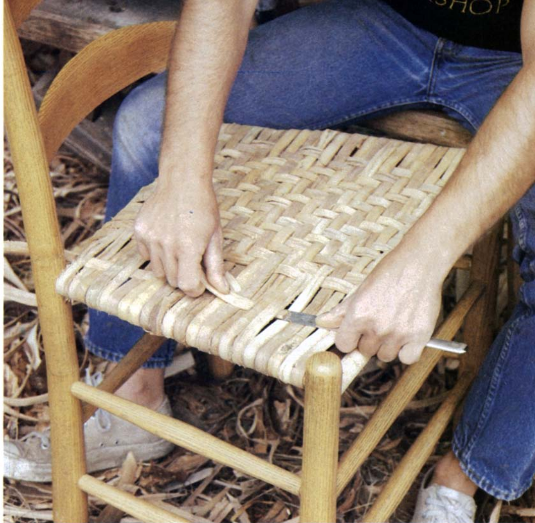
10. As the seat progresses, a butter knife acts as a ramp to ease insertion of the weavers. The chair's splay forms an unwoven section that will be filled in with separate pieces.
