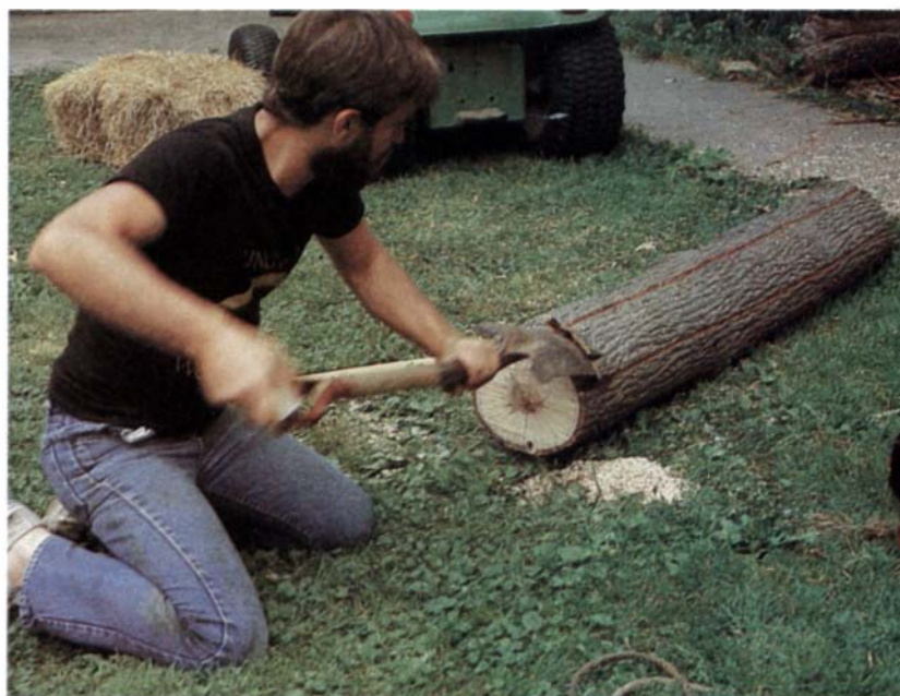
1. To remove the inner bark of a hickory log, Shriver first kerfs the length of the bole with a chainsaw. A trenching shovel slipped between the wood and the bark loosens the slab enough to be peeled by hand.
