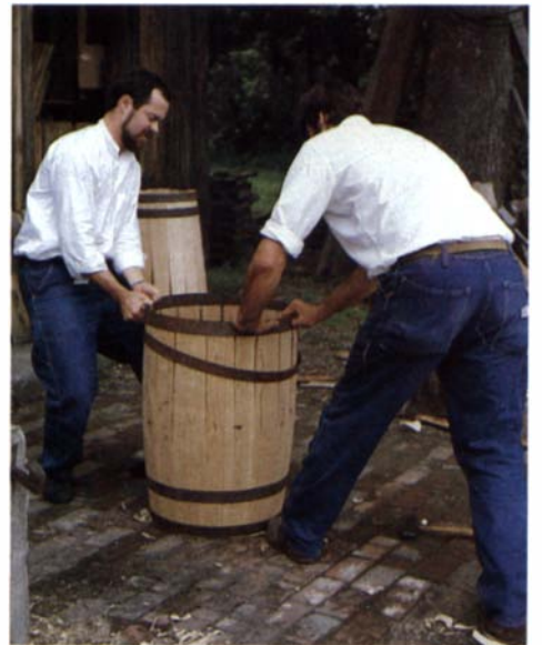
Cocking a hoop draws the staves together enough to reduce the diameter of the barrel so the next size hoop can be forced on.
