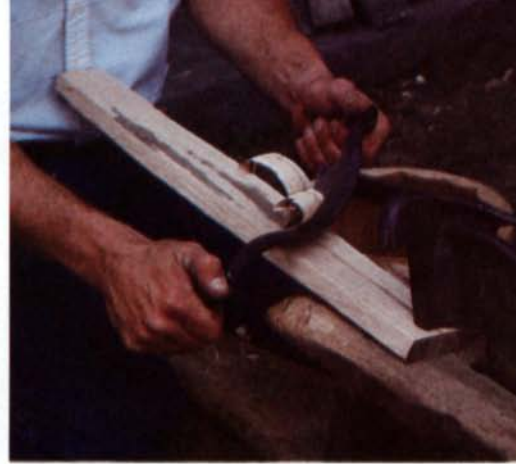
Raiselis twists his froe through a quartered block of green oak to split out stave blanks, left, then tapers and bevels each piece with a side axe. After shaping the outside of the stave with a straight drawknife, he uses a hollow shave, above, to scoop out the inside face so the stave can be more easily bent. The long butt joints on the staves are jointed and beveled on a cooper's jointer, which looks like an oversized, upside-down cabinetmakers' plane, right. The plane can be finely set, making it better than a power jointer for this operation.
