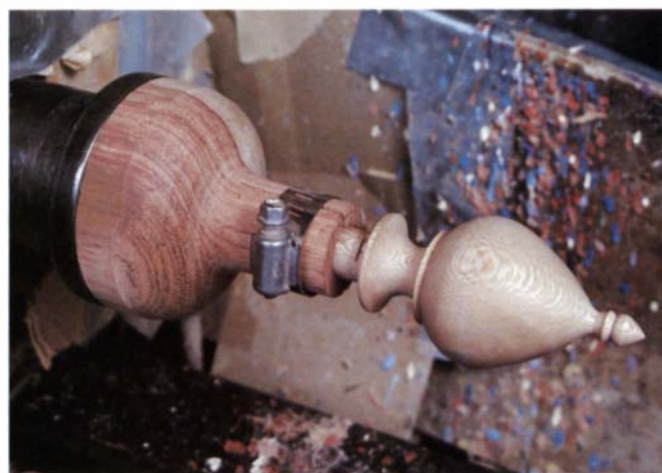
Mode's wooden chuck allows him to turn shallow-domed lids or lids with irregular projections. The holes allow him to gauge the lid thickness. A wooden collet chuck can be made with a piece of springy hardwood and a hose clamp (shown below).
