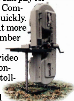
Converts to vertical band saw for ripping. (stand optional)
