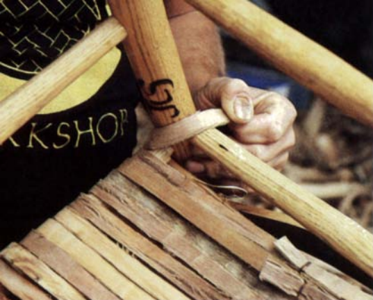
8. Warp to weave (woof) transition is made by wrapping up and over left rung, across the top of the seat, down and around the right rung to the rear rung.
