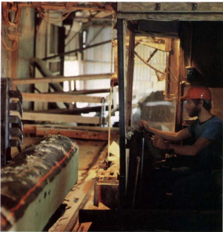
The bandsaw, a 150-HP bandsaw, can slice the length of a 16-ft. log in less than two seconds. Here the log is being manipulated for a second cut; the red line is a laser beam that shows the sawyer where the cut will be.
