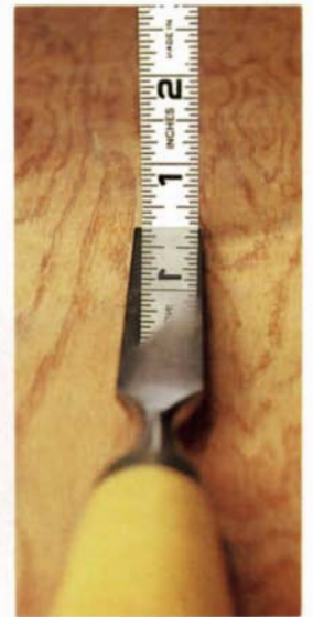
The strong point of Robert Sorby's aerosol diamond slurry is the flatness it gives to the backs of chisels and plane irons. The diamond can also sharpen carbide router bits.
