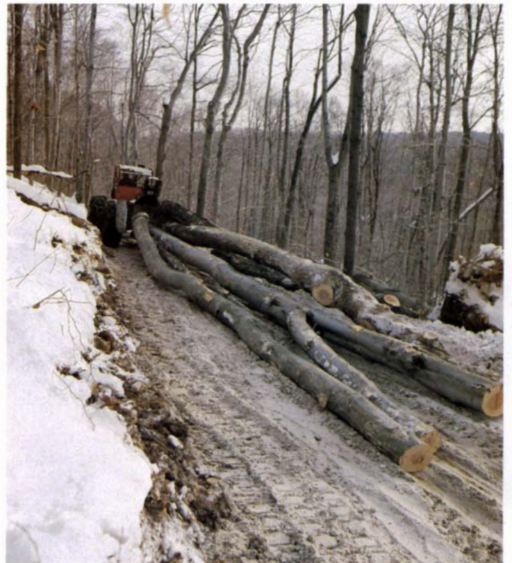
The skidder, a specialized tractor, tows a train of logs toward the decking area, where the logs will be cut to length.
