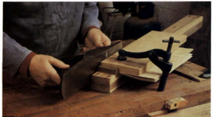
A shooting board is one way to produce an accurate straight edge on relatively straight-grained veneer. Highly figured veneer is best cut with a straightedge and knife.
