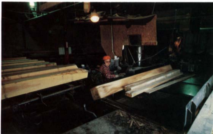
Squared-up logs, called cants, are sawn into boards on a bandsaw similar to the bead rig shown above and on p. 40. Here the sawyer has just seen a defect in the cant, and is flipping it to a new, clean face for the next cut.
