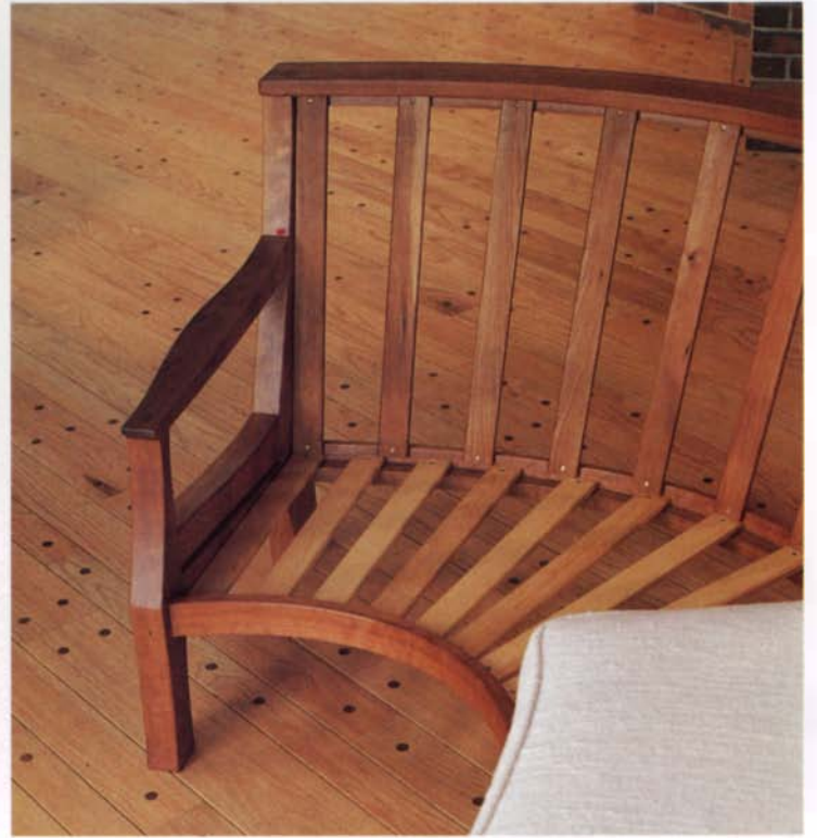
These couches neatly resolve several conflicting seating requirements. The pair of curved shapes allows easy conversation. Varying seat width permits both sitting and lying in comfort. Curved laminated rails carry slats that support the seat cushions (below).
