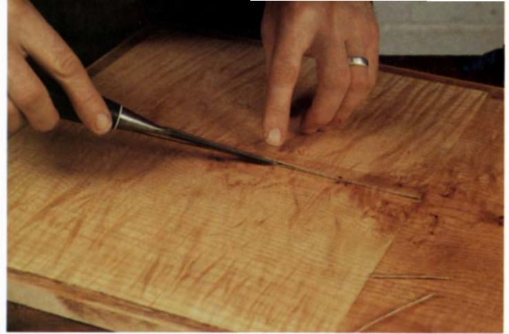
To join two leaves with the overlay method, knife through the center of the 1/2-in. overlap, then lift out the waste piece underneath with a chisel.
