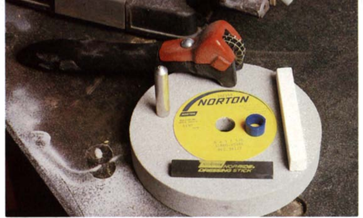
Norton's 60-grit wheel, off-white in color, with a variety of wheel dressers (shown counterclockwise from top): a star wheel, a single-point diamond, a Norbide stick and a plain abrasive stick.
