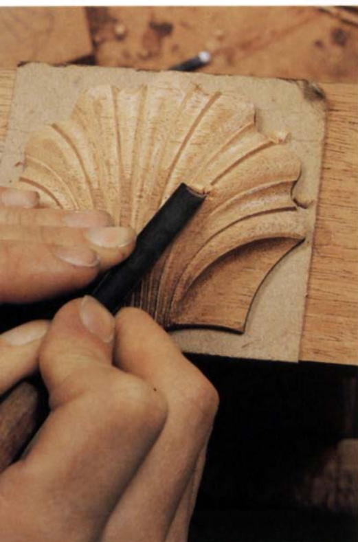
Shape tips of convex rays with a 1/2-in. #3 gouge, carefully avoiding tearout on cross-grain cuts (above). Left hand helps control the tool on concave rays (below).
