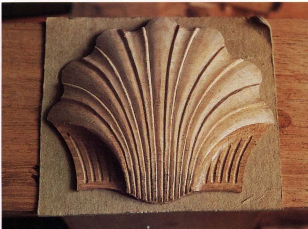
The finished shell is ready to be separated from its backing and glued on a piece of furniture. The curves and flats are designed to catch and play with light and shadow.
