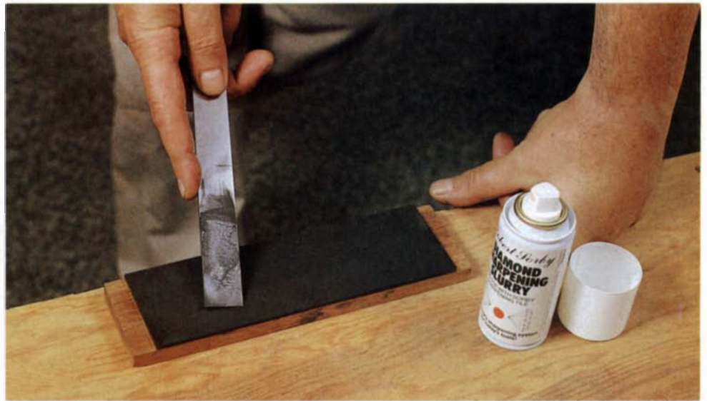
The strong point of Robert Sorby's aerosol diamond slurry is the flatness it gives to the backs of chisels and plane irons. The diamond can also sharpen carbide router bits.
