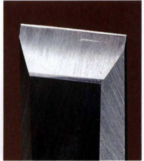
It's a waste of effort to hone the entire bevel. After four or five more honings, the polished area at the cutting edge will become wide enough that it will be worthwhile to regrind the bevel.
