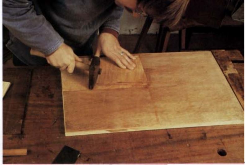
The first hammer stroke pushes from right to left, overlapping the edge. Glue on the surface lubricates the veneer hammer.
