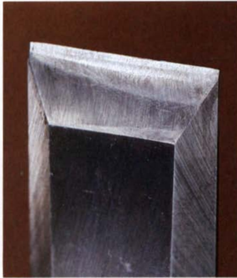
As the edge is boned sharp, the excess metal may come off as a 'wire edge.' This chisel has been deliberately boned with more pressure on one corner than the other to demonstrate the wire.
