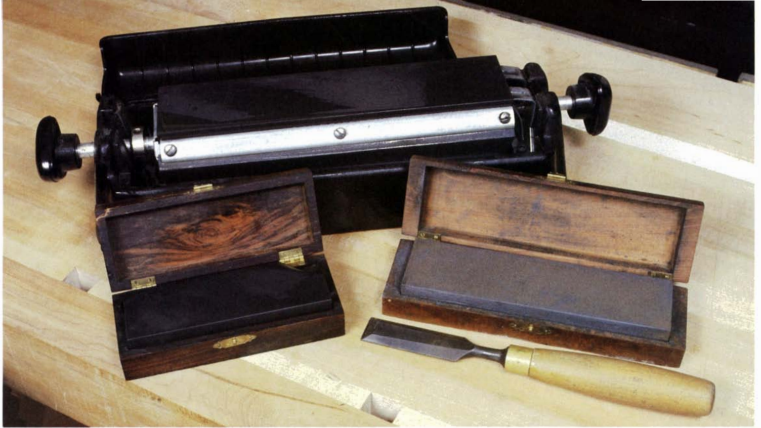
Podmaniczky's favorite sharpening setup is the Multi-Stone (rear), a set of three stones mounted so they can revolve through an oil bath to keep them clean. His boxed stones, bought 15 years ago, are a medium-grit India (right) and a hard black Arkansas.
