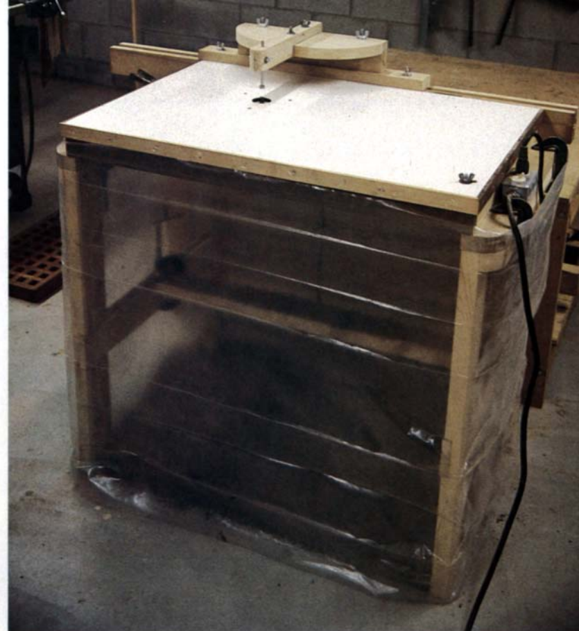
Unlike commercial models, Sporbeck's shop-built pin router has an overarm guide pin and the cutter is mounted beneath the table. The plastic wrapped around the router base keeps chips and sawdust from flying all over the shop. To clean up, just open the sheet and vacuum away the waste.
