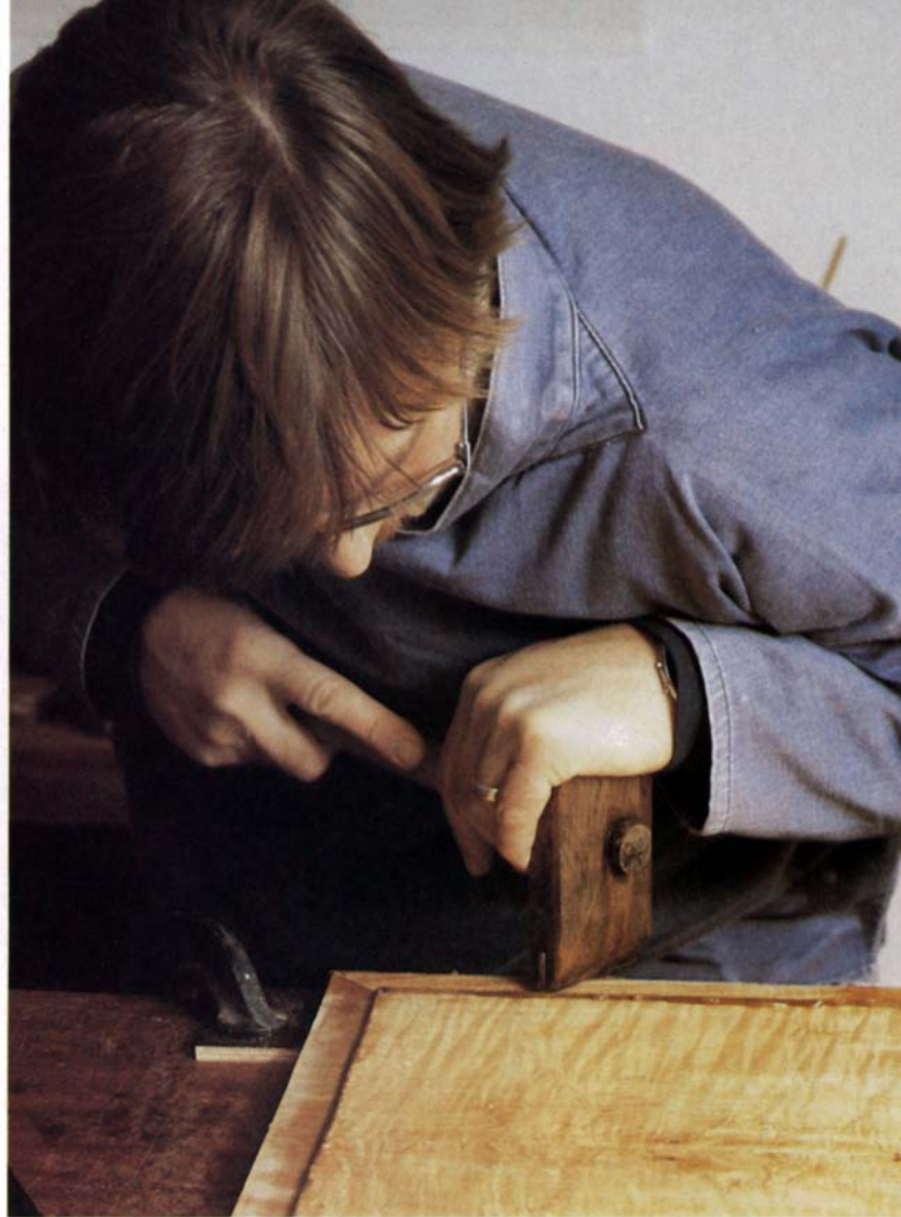
The inlaid walnut line around the border can be held in place with pins until the glue cools (top). To fix the crossband, begin with short strokes toward the center of the board then switch to strokes along the length of the crossband (right). Angle the head at 45° to the direction of the stroke. Allow the crossband sections time to expand, then square up the end with a chisel (above) before laying the next piece. The mitered corners are also cut with a chisel.
