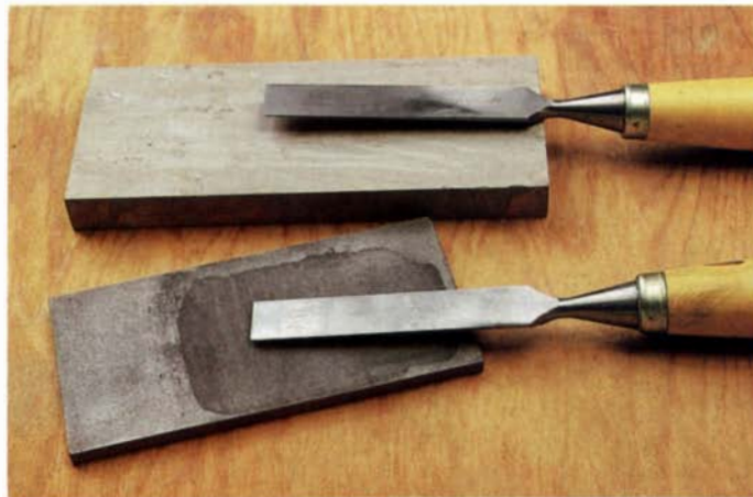
To extend the range of the typical sharpening stones, you can use a diamond plate for initial flattening, and a wooden block coated with rottenstone for final polishing. Mirror-like results are shown at right.
