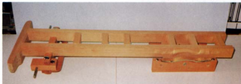
The front view of the partially assembled truck, top, shows the front spacer that sets the width of the cab and is screwed to the frame pieces. Also supporting the cab is a rigid chassis, above, a series of beech crossmembers mortised into two long frame pieces, which are, in turn, mortised into the front bumper.
