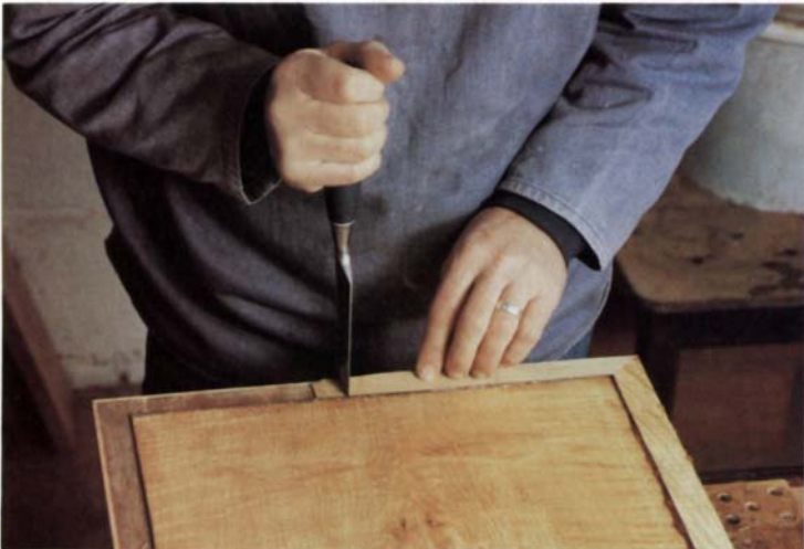
The inlaid walnut line around the border can be held in place with pins until the glue cools (top). To fix the crossband, begin with short strokes toward the center of the board then switch to strokes along the length of the crossband (right). Angle the head at 45° to the direction of the stroke. Allow the crossband sections time to expand, then square up the end with a chisel (above) before laying the next piece. The mitered corners are also cut with a chisel.
