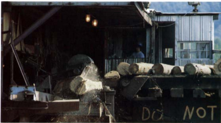
With a normal backlog of 30,000 logs on hand, high-power machinery, like this debarker, is necessary to keep things moving. Three minutes from now, this log will have been sawn into boards ready for grading.
