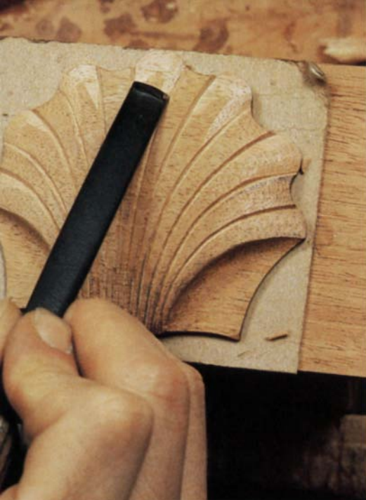
Shape tips of convex rays with a 1/2-in. #3 gouge, carefully avoiding tearout on cross-grain cuts (above). Left hand helps control the tool on concave rays (below).
