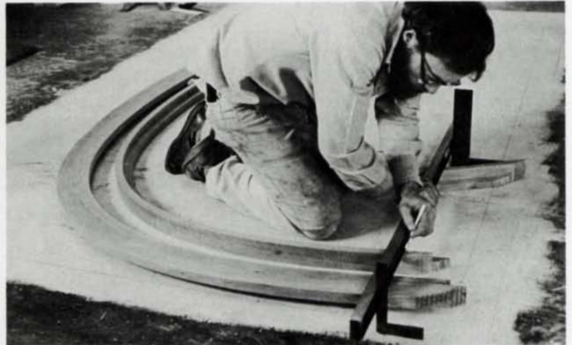
Align the rails on the floor drawing and knife their ends and shoulder lines against a straightedge. Try squares help position the straightedge exactly above the end-frame lines.
