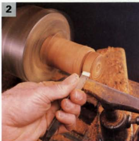
The threads on the screwtop jar (top) were cut on the lathe with 8-tpi chasing tools. The jar body is parted off (center) leaving the lid in the chuck. A 1/2-in. skew (above) turns the flange 1/8 in. larger than the opening in the top.
