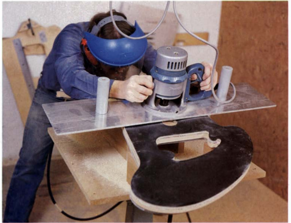
Moser is one of two shops Knoll International selected to manufacture Robert Venturi's post-modern plywood chairs. Moser cabinet-maker Michael Fleury, right, routs chair profiles using a series of vacuum-clamped templates provided by Knoll's prototype shop.
