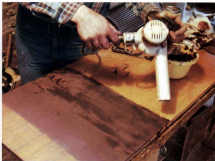
An electric heat gun speeds drying of plaster filler.
