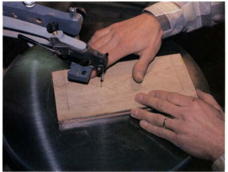
Below and at left, a puzzle with 88 pieces of kingwood, padauk, bird's-eye maple, wenge and camphorwood, 4 \frac{3}{8} in. by 9 \frac{3}{4} in. The pieces removed at the far corner (facing page) show the three layers. To make a jigsaw puzzle, the main elements are cut out in a stack (photo right), then jigsawed into pieces. Below right, an eight-layer puzzle of wenge and maple, about 8 in. square, contains 250 pieces.
