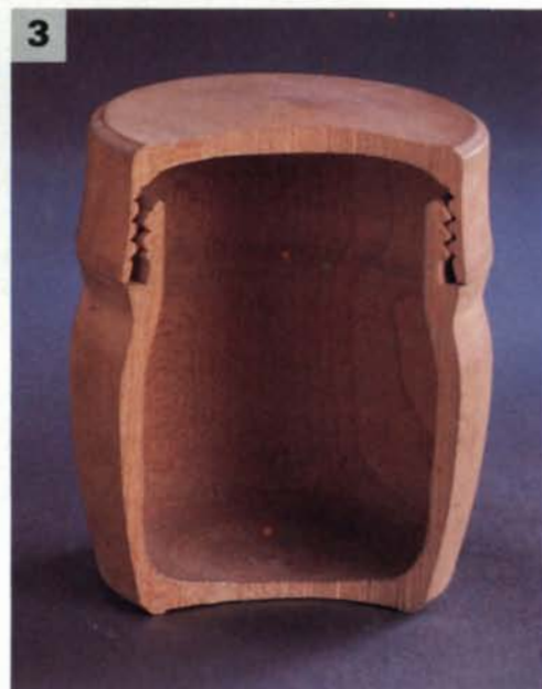
The threads on the screwtop jar (top) were cut on the lathe with 8-tpi chasing tools. The jar body is parted off (center) leaving the lid in the chuck. A 1/2-in. skew (above) turns the flange 1/8 in. larger than the opening in the top.
