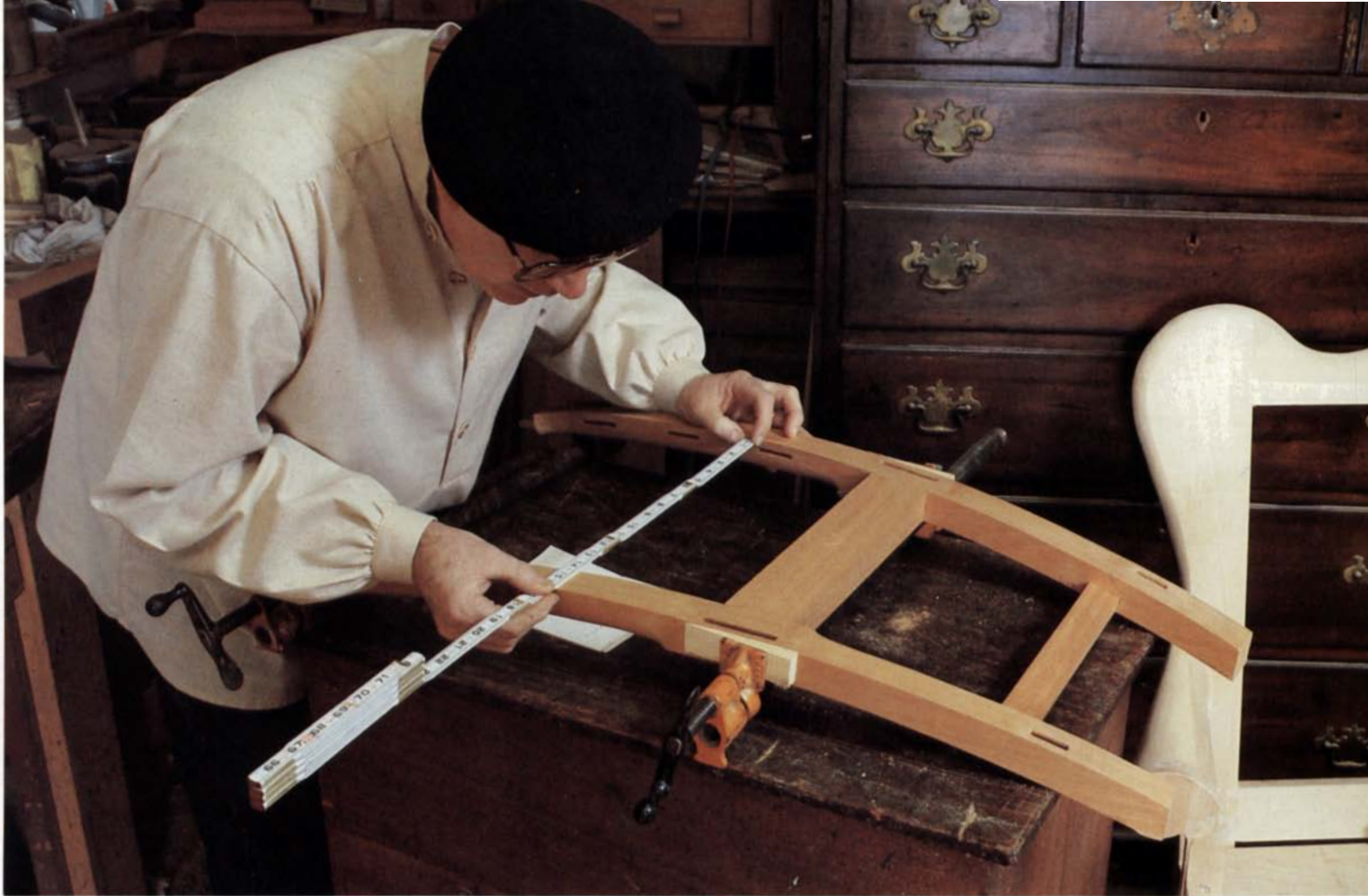
When sizing the ladders, above, a pair of clamps stabilizes the back posts. To pierce the back, left, first drill entrance holes for the scroll saw blade. The size of the drill bit used, in this case \frac{5}{8} in., conforms to the design.
