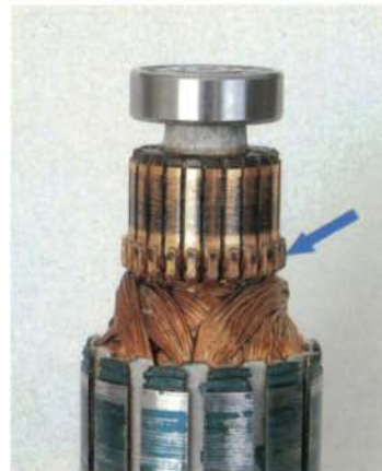
Armature windings can be connected to the commutator by a tang folded over each wire, left. The more durable punch-crimp connection, right, has no vulnerable projections.
