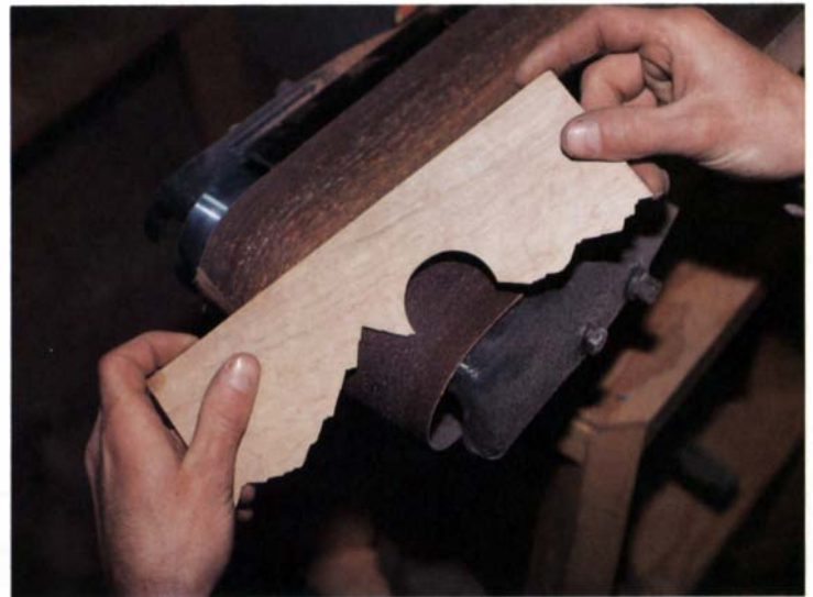
Edge-beveling, which gives an illusion of depth, can be roughed out over the end roller of a belt sander.
