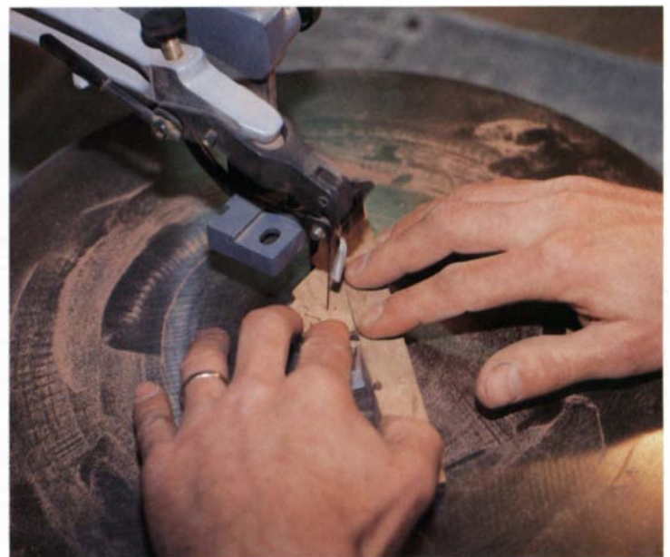
Each segment of a layered puzzle is sawn into interlocking pieces. Typical sawing patterns are shown on the facing page.
