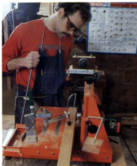
On the Easy Mortise machine, a single lever moves the sliding table in and out, as well as from side to side.
