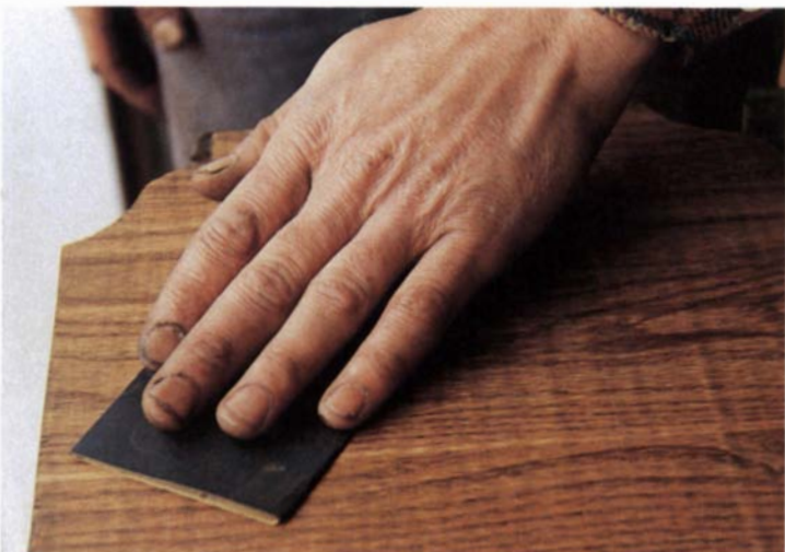
After filler dries, apply sanding sealer to lock it in, then sand.
