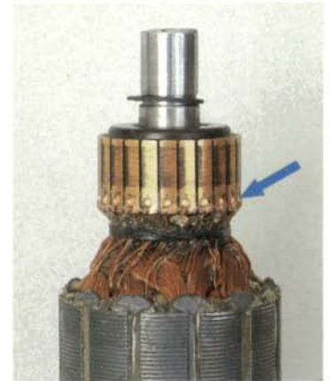
Armature windings can be connected to the commutator by a tang folded over each wire, left. The more durable punch-crimp connection, right, has no vulnerable projections.
