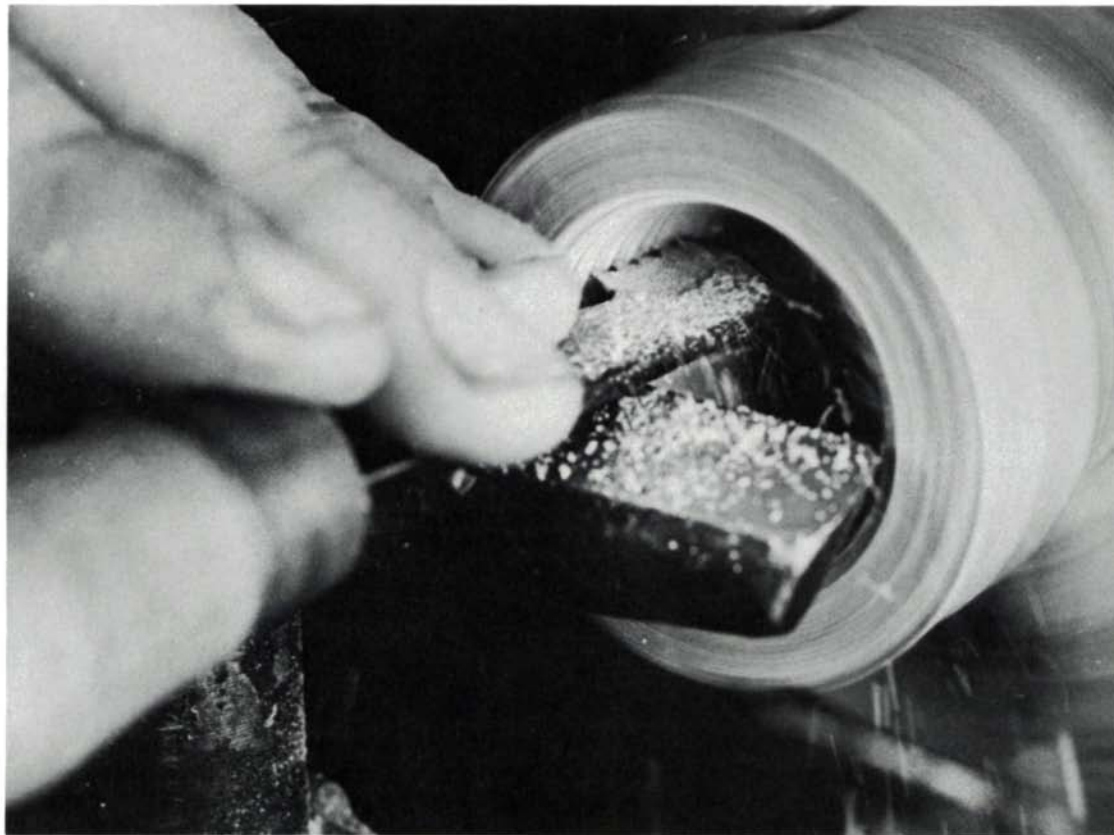
Chasing the inside thread on a screw-top jar lid (right). 'Drunken' threads (above) are an error caused by moving the tool unevenly.
