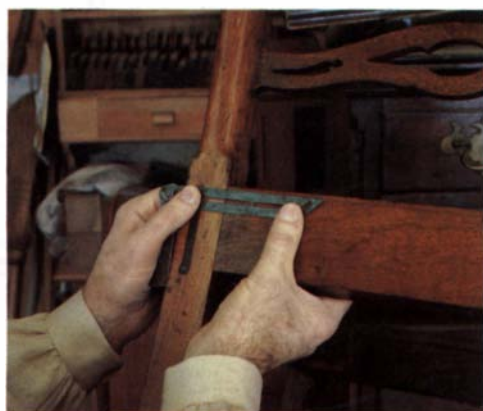
The slope of the shoulders on the back seat rail is a key angle—it determines the splay of the back posts, and thus affects the sizes of all the other parts in the back.
