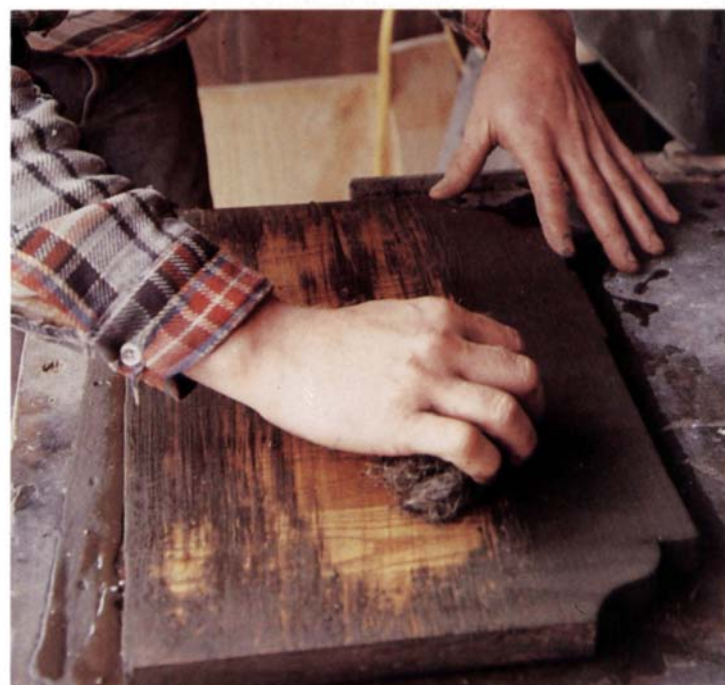
Vigorously rub off excess filler with a wad of burlap or horsehair.
