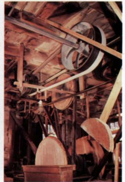
Young demonstrates oval turning on one of the Old Schwamb Mill's eccentric lathes, facing page. In its heyday, up to 30 workers would have made the Mill hum, turning out high-style frames such as the ones shown above. The old system of jackshaft and belts, at lower right, still drives most of the machinery, but two 7-HP electric motors have replaced the waterwheel as the source of power.
