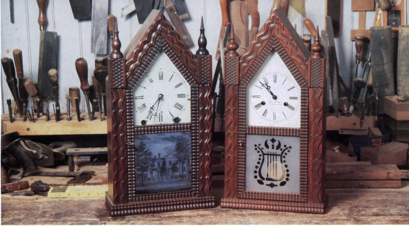
Irv Rosen's machine-made ripple molding re-creates the original charm of antique steeple clocks made in Connecticut during the 1800s. Details, facing page, highlight the unerring precision and crisp cuts produced by his molding machine.
