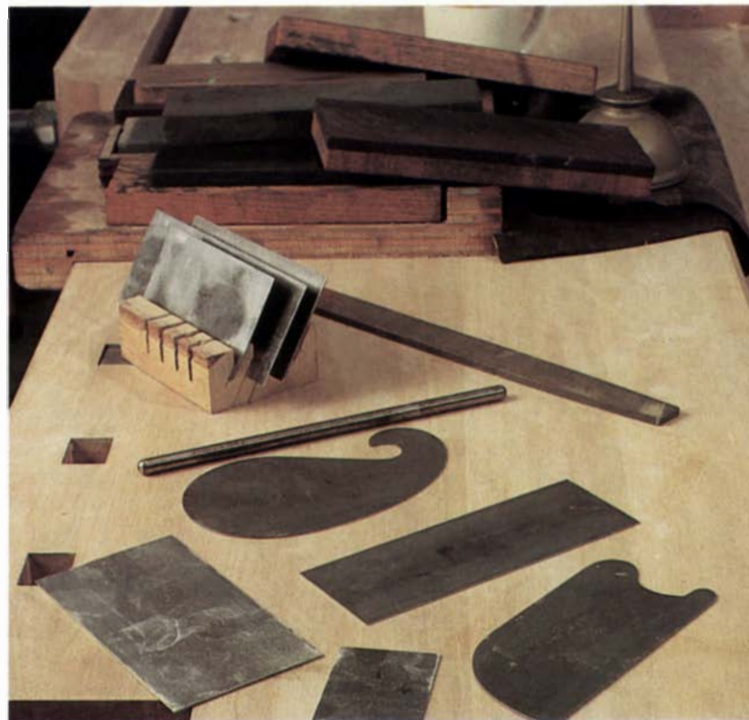
A scraper, most often nothing more than a piece of thin steel, can be any of a variety of shapes. Common commercial scrapers are rectangular and gooseneck, shown in the center above.
