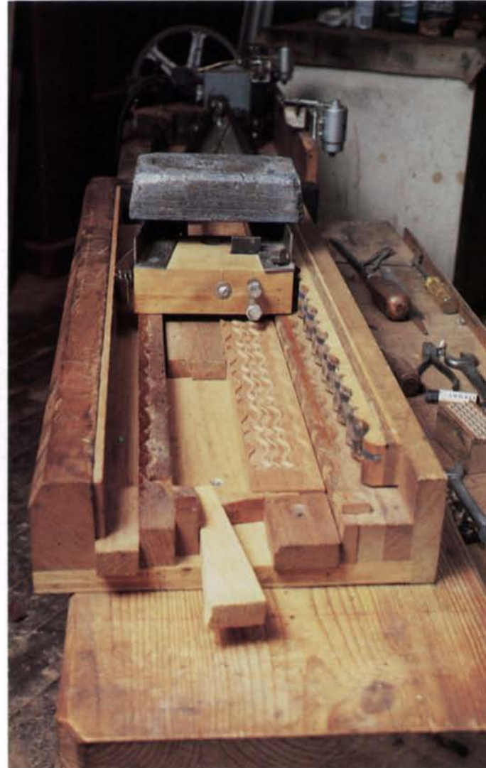
To form a left-to-right waving pattern, the cutter assembly follows a ripple template attached to the side rails of the machine.
