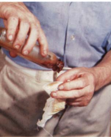
After dusting a pinch of pumice stone across the surface, the tampon is wet with alcohol and rubbed over and over the surface, filling the pores with pumice and wood dust. When the pores are filled, shellac is introduced to the inside of the tampon, and the rubbing continues, eventually building up a film of shellac.
