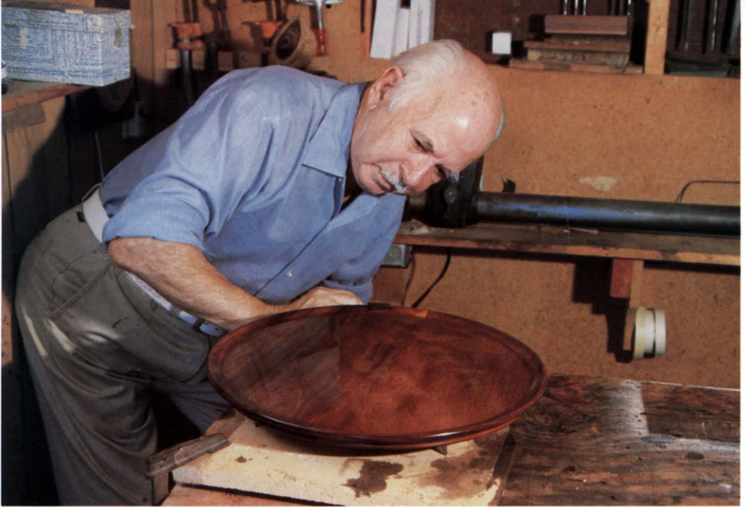
French polishing, the venerable technique for applying a shellac finish, produces a high-gloss sheen as yet unmatched by any modern finishing technique. Here, George Frank checks for flaws in the finished surface.
