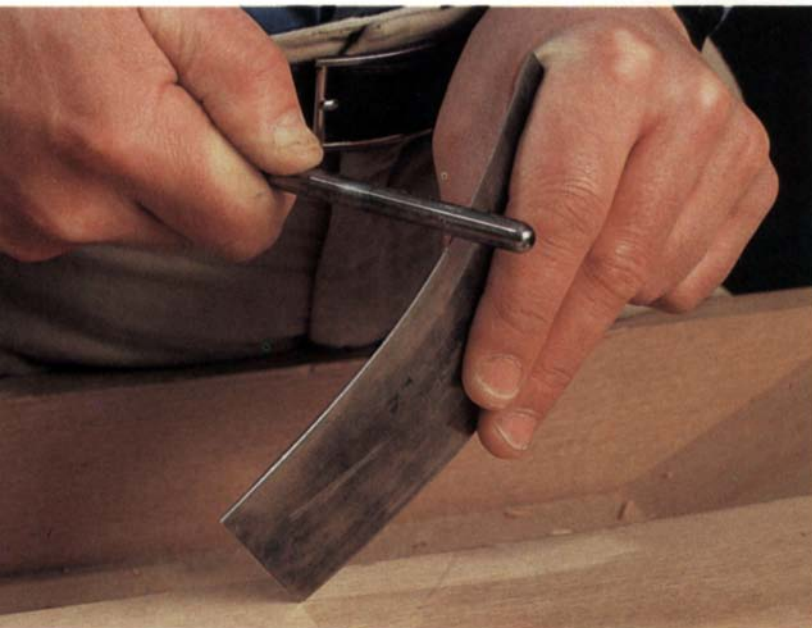
To raise the burr, hold the burnisher at a slight angle to the face and stroke it firmly back and forth along the arris. To turn the burr, make a single firm pass along the arris, the burnisher held slightly less than perpendicular to the face.
