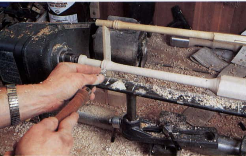
Brass pipe is ideal for binding round mallet heads (top). Make sure the rabbet is a snug fit; secure the binding with two or three countersunk brass screws. Below, Hanner turns the knuckle on a handle shank. The finished handle behind the lathe is a reminder of the desired profile.
