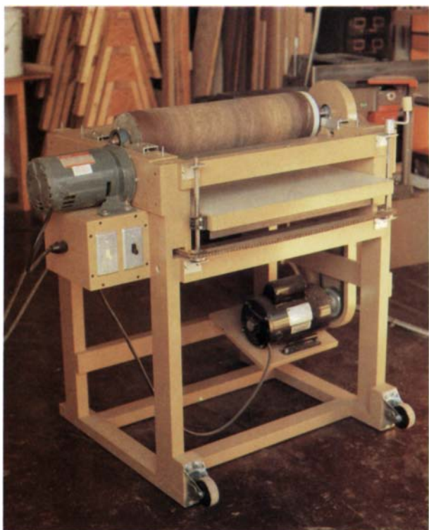
Curtis Erpelding built his 24-in. power-feed abrasive sander from a $660 kit, which he customized to handle the specialized needs of his production work. To eliminate sniping, he substituted angle-iron brackets for the machine's original aluminum brackets, which flexed enough to distort the critical alignment between the table, feed rollers and sanding drum.
