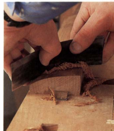
To scrape a flat surface (right), hold the scraper as nearly perpendicular to the work as possible and push or pull it to take wide shavings. A gooseneck scraper is ideal for tight curves (top). A flexed rectangular scraper can scrape shallow concave and convex surfaces (bottom).
