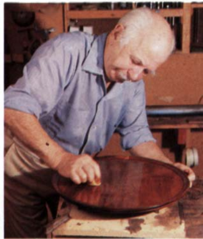
After dusting a pinch of pumice stone across the surface, the tampon is wet with alcohol and rubbed over and over the surface, filling the pores with pumice and wood dust. When the pores are filled, shellac is introduced to the inside of the tampon, and the rubbing continues, eventually building up a film of shellac.
