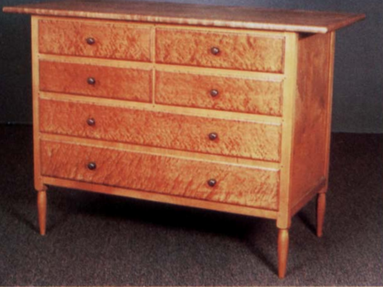
Shaker designs offer an excellent way to display highly figured hardwoods. The delicately turned legs and gracefully shaped overhang on this bird's-eye maple chest are also hallmarks of the best Shaker work. This frame-and-panel chest is 21 in. deep, with a 3-in. overhang on the front, and 45 in. wide, including a 4½-in. overhang on each side. A ¼-in. bead highlights the drawer fronts and the inside edge of the frame of the side panels.
