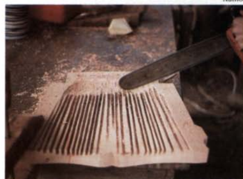
With a chainsaw and body grinder, Erickson can sculpt the tractor-seat saddle of his chairs in about an hour. After penciling the saddle outline on the top surface and the contour on the front edge, kerf the seat with a series of chainsaw cuts to approximate depth (left). Shape the seat by sweeping the nose of the chainsaw slowly from the arrises into the depressions. A body grinder refines the saddling and cleans up the chainsaw marks (right). The chair shown at top is made of California madrone.
