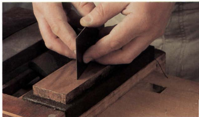
After filing, work the faces and edges of the scraper on a medium and a hard stone. Hold the scraper diagonally across the stone's width to prevent wearing the stone unevenly.
