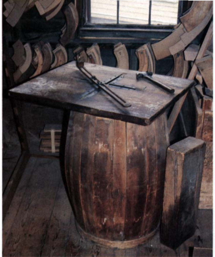
The first step in making an oval is to make a pattern. This old trammel board, above, is adjustable to draw ovals (and circles) from a few inches wide up to 4 ft. long. The four identical segments that make up an oval frame are finger-jointed on the venerable gang saw shown below, but today's blades are carbide-tipped.
