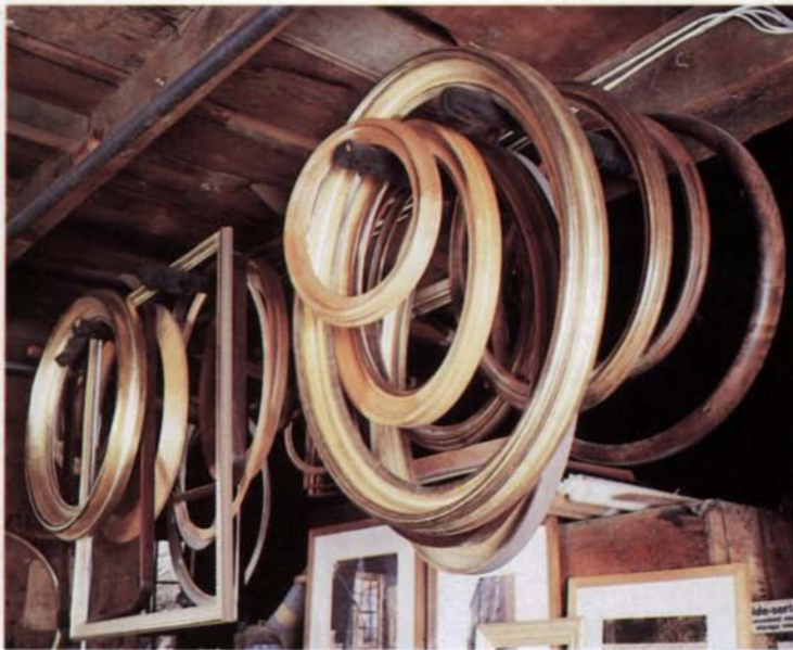
Young demonstrates oval turning on one of the Old Schwamb Mill's eccentric lathes, facing page. In its heyday, up to 30 workers would have made the Mill hum, turning out high-style frames such as the ones shown above. The old system of jackshaft and belts, at lower right, still drives most of the machinery, but two 7-HP electric motors have replaced the waterwheel as the source of power.
