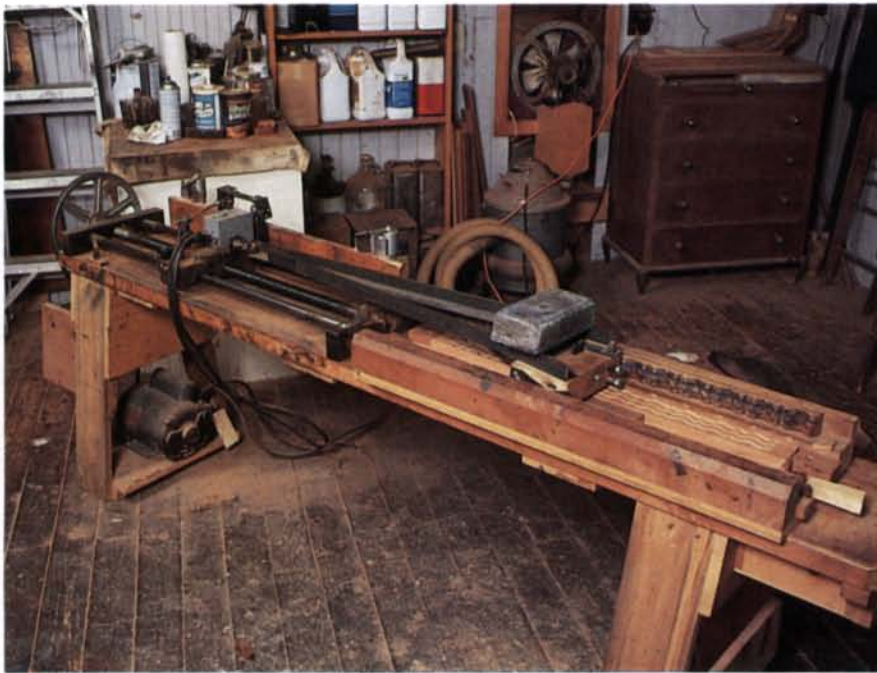
Ripple molding develops slowly from several hundred passes of a razor-sharp cutter, which is pulled back and forth over the molding stock until the desired depth of cut is reached. The rotating lead screw, foreground, first pushes the angle-iron carriage and the cutter down the length of the molding. A heavy weight on the cutter keeps it in contact with the wood during each pass. At the end of each pass, a switch reverses the motor and the rod pulls the carriage assembly back. The cutter, beveled on both sides, is shaped to match the molding profile being cut.
