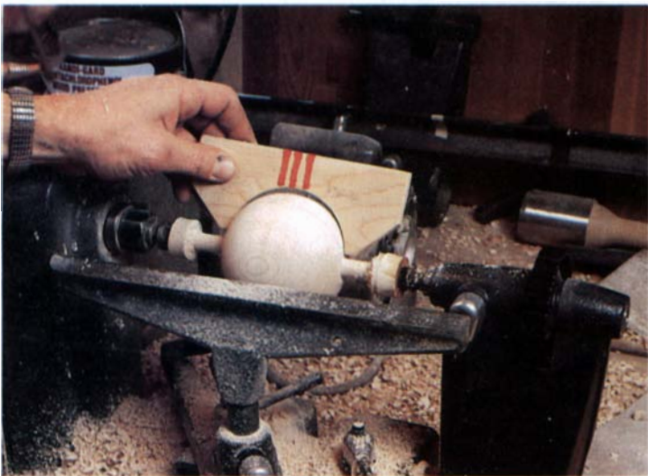
Almost-round croquet balls are relatively easy to turn. Accurate templates are a considerable help in turning truly round balls.
