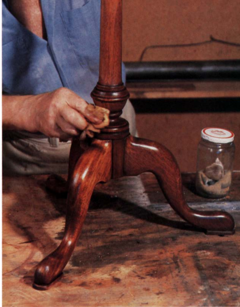
A thicker coat of shellac is built up on the table legs and column using a piece of cheesecloth as an applicator. Then, after sanding with 600-grit paper, a final coat of shellac is applied with a piece of soft foam rubber.
