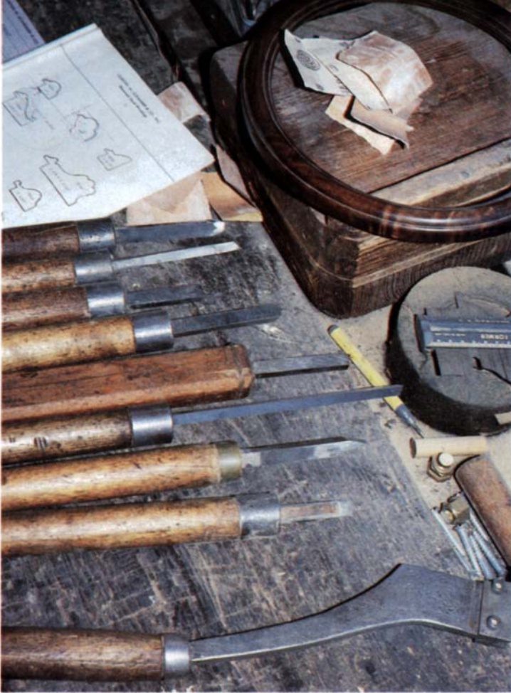
The display may be reminiscent of a barn sale, but these tools are in everyday use, turning out oval frames to match patterns that were drawn and cataloged by the Schwambs 150 years ago.
