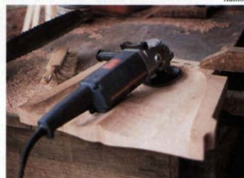
With a chainsaw and body grinder, Erickson can sculpt the tractor-seat saddle of his chairs in about an hour. After penciling the saddle outline on the top surface and the contour on the front edge, kerf the seat with a series of chainsaw cuts to approximate depth (left). Shape the seat by sweeping the nose of the chainsaw slowly from the arrises into the depressions. A body grinder refines the saddling and cleans up the chainsaw marks (right). The chair shown at top is made of California madrone.
