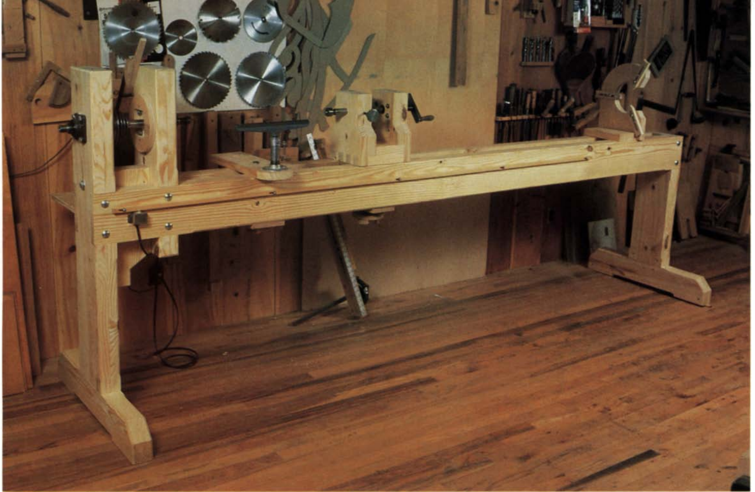
Glued up from yellow pine framing lumber, Lynch's wooden lathe cost less than $200 in materials. With its 10½-ft. bed, it can handle up to 8-ft. work. A strip of wood, screwed to the bed through slotted holes, activates the on/off switch from anywhere on the bed.
