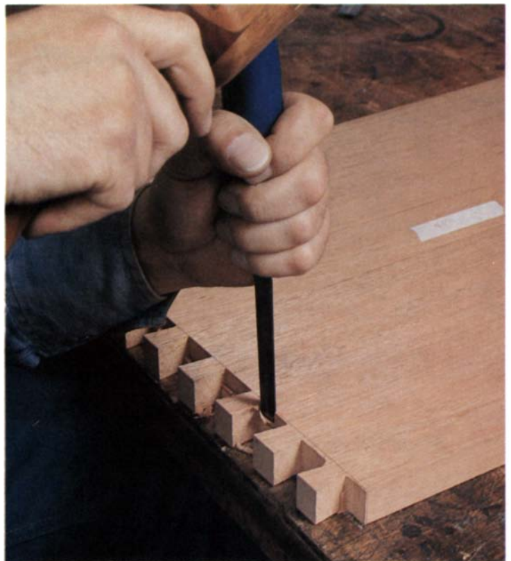
After clearing most of the waste from the sockets with a coping saw, chop to the scribe lines on both faces with a sharp chisel.
