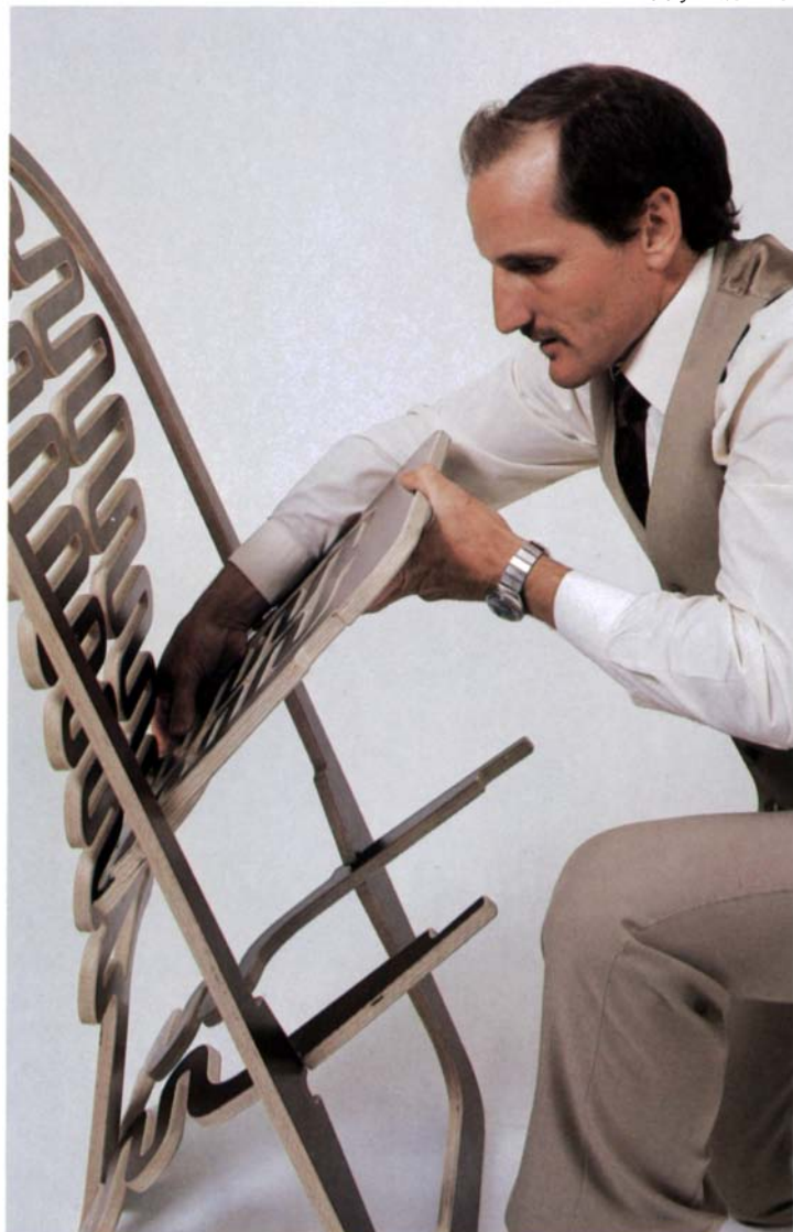
Gregg Fleishman fits slots together to assemble the two-piece "Lumbarest" chair, which is the result of 4½ years of experiments with slotted plywood panels.
