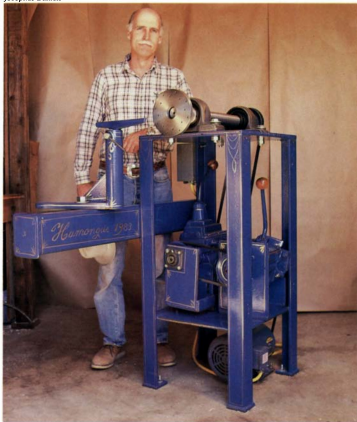
Blanchard poses with the super bowl lathe (newly pinstriped) that he made for bowl turner Neil Weston. The lathe swings 8 ft. with the toolrest removed, and 36 in. with the rest in place. The top is a 21 in. square of 3/4-in. steel plate welded to 3-in. by 3-in. angle-iron legs. Two non-synchromesh G.M. transmissions from the 1940s—a 4-speed truck and a 3-speed—provide 13 forward speeds from 33 RPM to 856 RPM, and some in reverse for final sanding. Power comes from a 2-HP, 220-volt single-phase Baldor motor, mounted on the floor to isolate vibration. The spindle is a length of 2 1/2-in.-dia. heat-treated shafting. The clamp on the toolrest post is made from Powermatic lathe toolrest clamp parts ordered from the Powermatic parts catalog.
