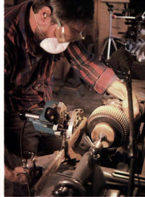
At left, large gears are cut by a router mounted on the cross-slide and compound of a South Bend metal lathe, which the author bought used for $4,000. The blanks are indexed by the pin opposite the router bit. Above, Westphale cranks the router along a stack of six wheel blanks, backed up at each end by a hardboard blank to prevent tearout.
