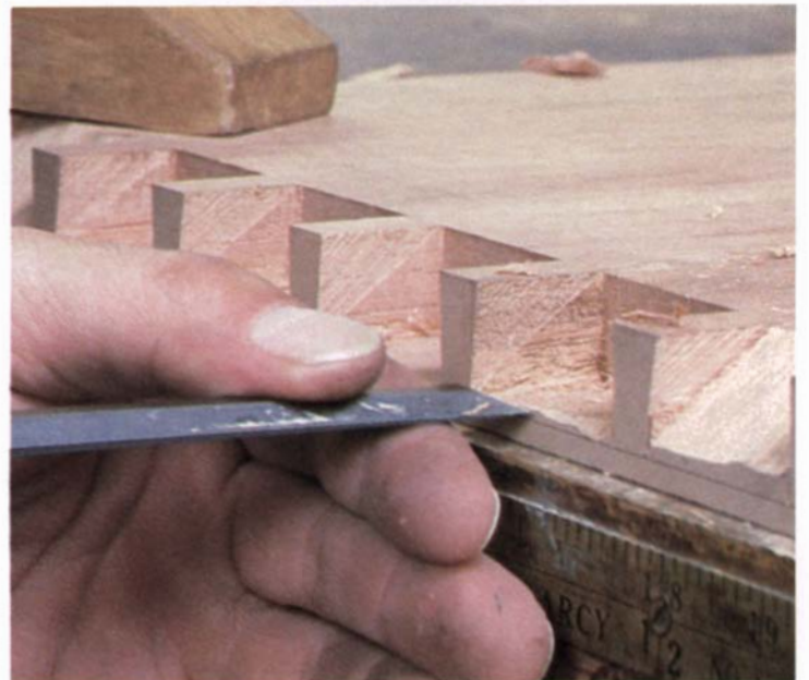
Clear waste from the sockets with a coping saw (top right), staying well short of the scribed line for the socket bottoms. Then chop the remainder of the waste, making the final paring cuts on the scribed lines (above).
