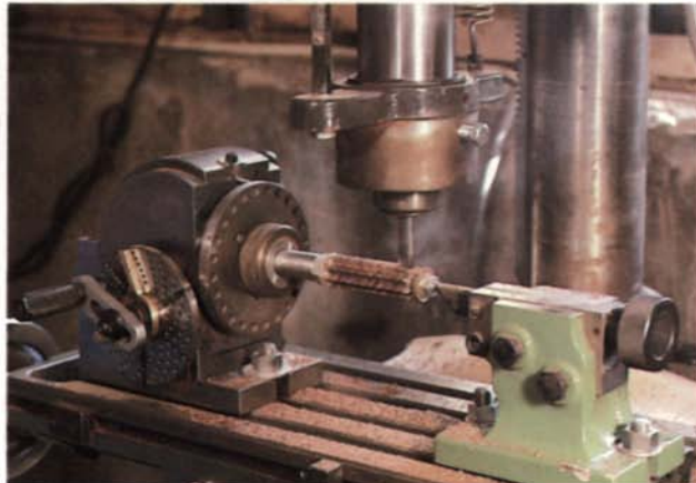
Left, a milling machine is the metalworker's precision version of a drill press, equipped with a table that can be moved horizontally on X and Y axes by hand cranks. The stack of pinion blanks is indexed by a dividing head, which calculates angles by means of perforated plates and a gear box. It takes forty turns of the crank handle to rotate the output shaft one full turn. Far left, an efficient circle-cutting jig: The board has a runner on the bottom that rides in the bandsaw's miter-gauge slot, and a number of axle holes to suit the various gear sizes.
