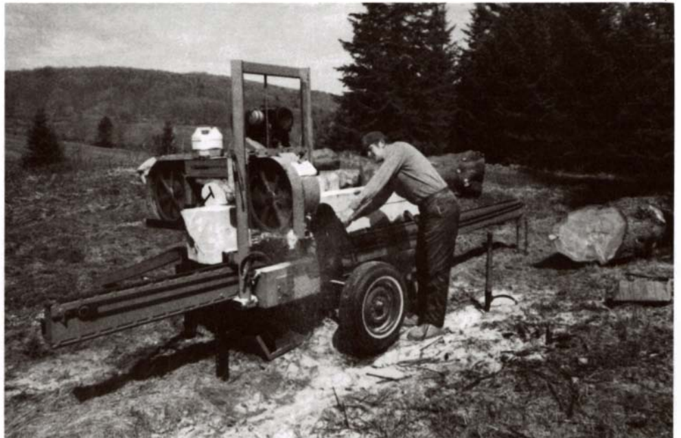
Don Lawrence fires up his Wood Mizer portable band mill. Rather than moving the log past a stationary blade, the Mizer moves motor and blade through the log.
