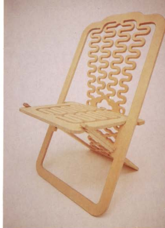
Chair #22 introduced a new way to build in additional support for the seat front. The rear legs bend forward and cross the front legs, interlocking with them. Then, they continue forward to support the seat.
