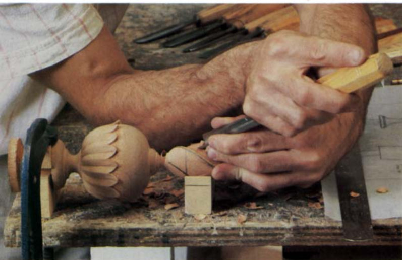
The wood between the ridges of the flame is removed with a sharp fluter or 5mm gouge, top photo. If wood begins to tear out, reverse the cutting direction by moving your hands, as above, rather than wasting time by walking around the bench.
