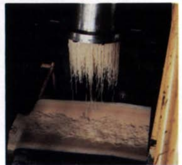
The recipe for glue begins with a mountain of hides, best shifted with a front-end loader (photo, facing page). Above, George DeBoth pauses at what must be the world's largest glue pot, a holding tank midway down the line. The photo at right shows gelled hide glue near the end of the process. The spaghetti-like extrusions will be dried crisp in ovens, then granulated.
