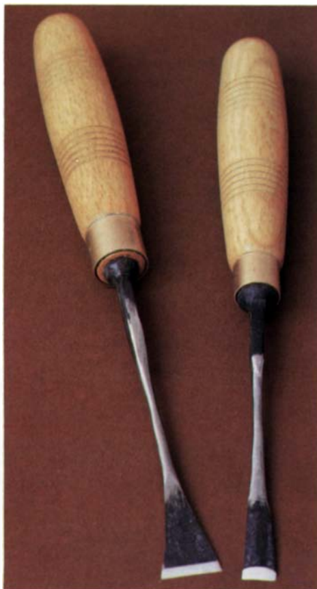
Less is better for spade tools. Upper shaft indicates how much fishtail is reground.
