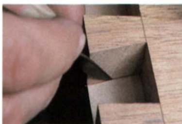
A stable, accurately aligned setup is crucial when scribing the pins from the tails. Pull any bow out of the pin board (the vertical one) by clamping it to the bench, as shown above. Scribe carefully, keeping the knife blade flush with the tail, as shown at left.
