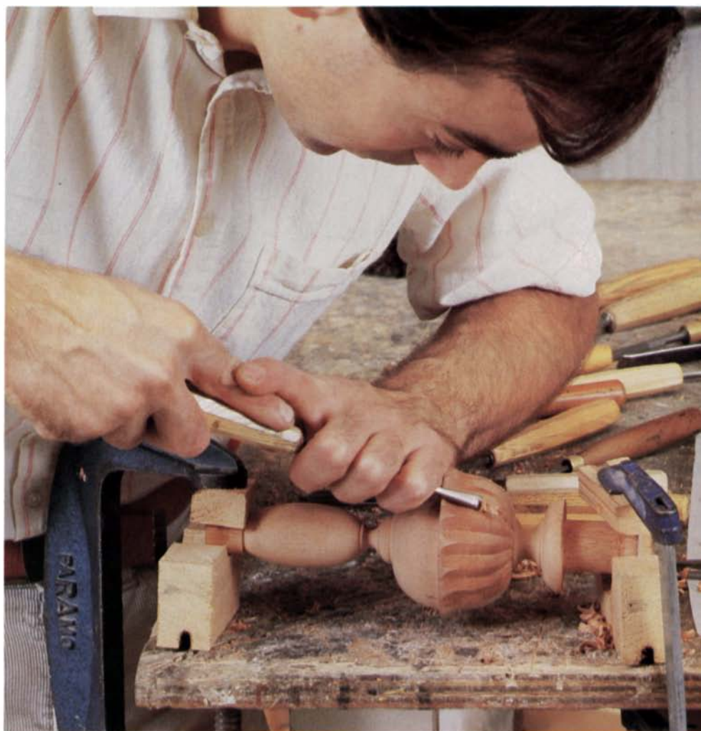
Cut a deep channel down the center of each leaf with a parting tool, top left, so that the midsection is lower than the edges. Next, round over the sides of the leaf with bevel-up gouge, above. There's no hard division between leaves, just a sharp spine created as you round each edge toward its centerline. Finally, undercut each edge with a gouge matching the leaf-tip shape, left, so it won't look heavy.
