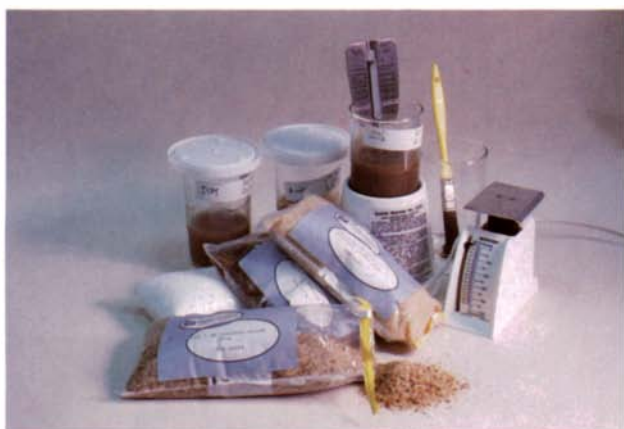
This low-tech glue lab requires only a scale, a bottle warmer and a thermometer. Various grades of dry glue are shown, along with a packet of urea, a white powder that extends gel time for making cold hide glue.
