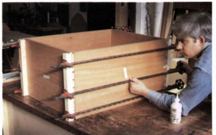
Using battens to protect the wood and distribute pressure, glue and clamp up the carcass. Work all the clamps down evenly to avoid straining the joints.
