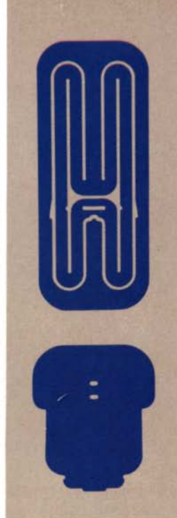
The seat on chair #6 locks into the front and rear legs. Pressure of the slightly angled seat stresses the legs, making them more rigid and stable. To make a comfortable and flexible back, Fleishman stopped the central back loop short of the seat.
