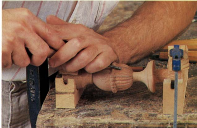
Carve a 2mm-deep channel down each centerline, top photo, with a V-shaped parting tool. The finial is clamped to the bench with wooden blocks, bandsawn from softwood so they won't dent the carving. To complete the molding, use small gouge, above, to round over the sharp inside edge of the fluter cut.
