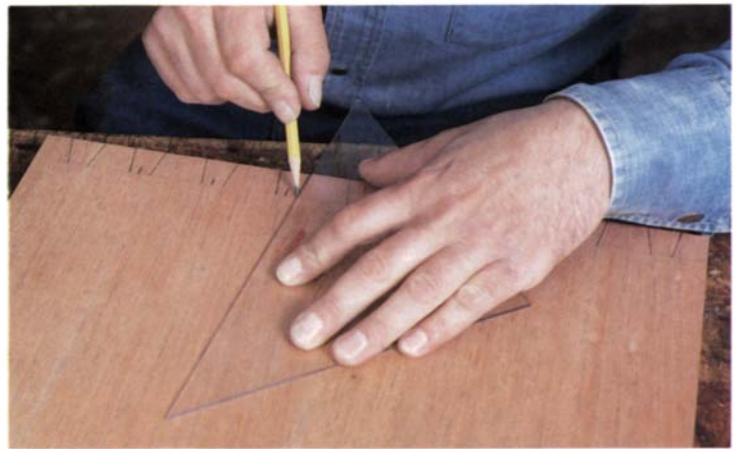
Determine the tail centerlines by eye, dividing the board in half, then quarters, and so on. You can freehand the tails' pitch with a straightedge as shown here, or use a sliding bevel for strictly uniform pitch.
