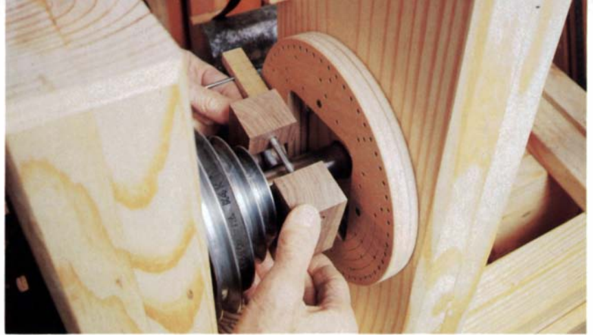
The headstock spindle turns in flange-block bearings bolted to the headstock uprights. The weight of the ½-HP motor keeps tension on the belt. Pulling forward on the lever pulls a strip of ¼-in. webbing to lift the motor forward and take the weight off the belt for changing speeds. The upholstery spring under the motor damps vibration. A birch-plywood indexing ring (above) screws on the inside of the inboard headstock upright. With the belt removed from the motor pulley, a pointer fits around the headstock spindle so that an 8d nail can slide through a hole in one of five concentric rows. A bar on the pointer passes through a hole in the spindle.
