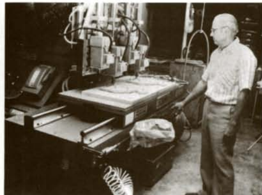
Jim Kassner's Phoenix clock kit (left) is milled largely on the $40,000 computer-controlled router shown above.
