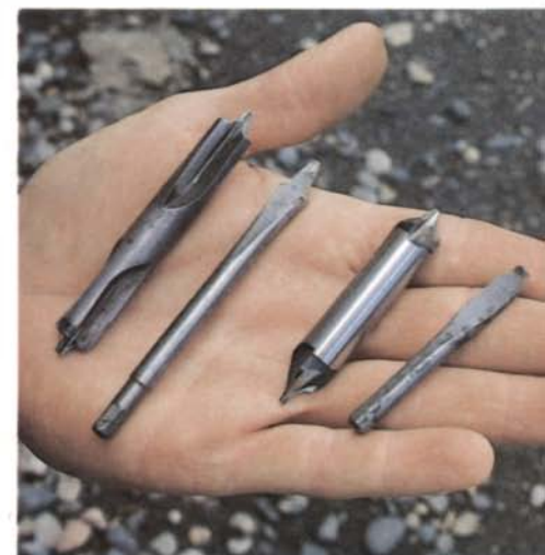
Cutters are reshaped as shown in the drawing at left. Tooling need not be high-tech. Westphale shows two of his early gear cutters, re-ground spade bits, alongside the highly evolved ones he uses today.
