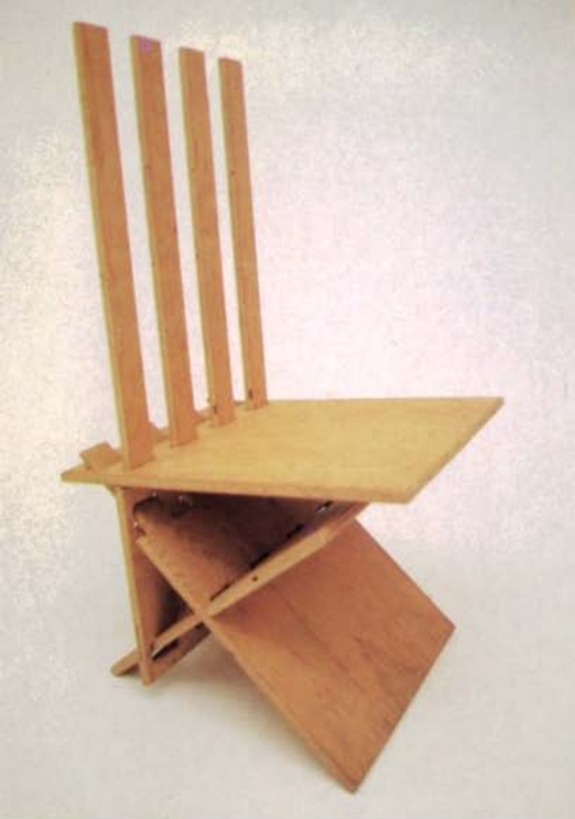
Chair #1 has a cantilevered back that looks somewhat like the tines of a fork. The pattern for this four-piece chair is shown at right. Two pieces cut to match the middle pattern crisscross and lock together under the seat.
