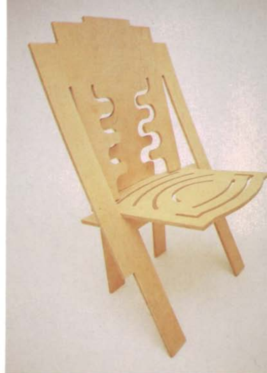
Fleishman's second chair was radically different from the first. Because of the vertical slots, he was able to bend the outer part of the back forward to become the front legs, reducing the number of panels needed from four to two.
