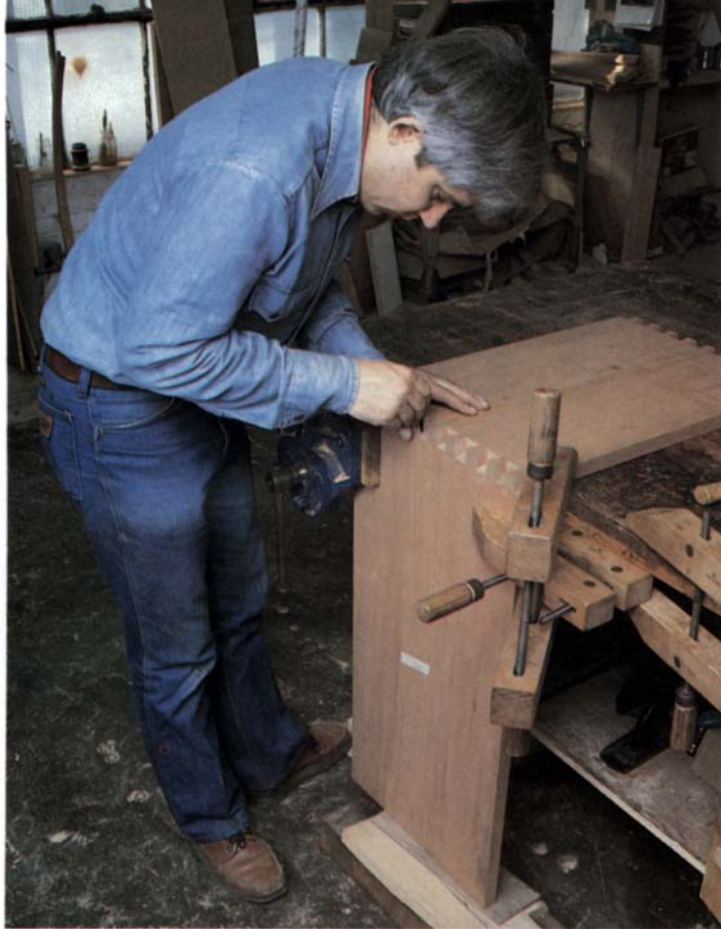
A stable, accurately aligned setup is crucial when scribing the pins from the tails. Pull any bow out of the pin board (the vertical one) by clamping it to the bench, as shown above. Scribe carefully, keeping the knife blade flush with the tail, as shown at left.
