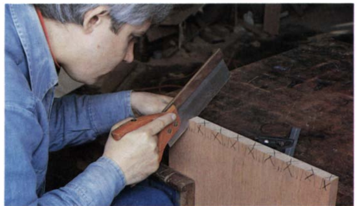
Cut down the pitch lines for each tail. Start the cut against your thumb, the saw at an angle. Lower the saw to finish the cut at the scribed lines.
