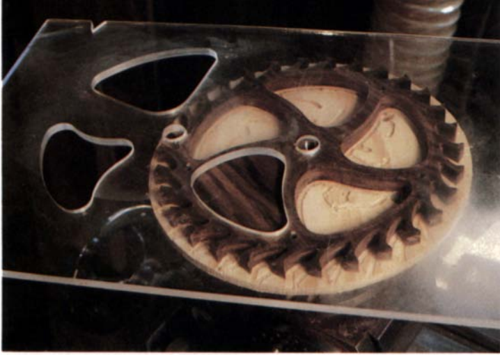
The escape wheel nearing completion. The acrylic template remains stationary, with its far end clamped to a block on the workshop wall. To rout successive spoke holes, the work is turned by the dividing head, which has been set in position to hold the wheel horizontal. Spoke-hole patterns for some of the other wheels in the clock are also visible in the photo.
