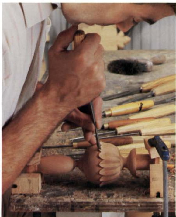
Cut a deep channel down the center of each leaf with a parting tool, top left, so that the midsection is lower than the edges. Next, round over the sides of the leaf with bevel-up gouge, above. There's no hard division between leaves, just a sharp spine created as you round each edge toward its centerline. Finally, undercut each edge with a gouge matching the leaf-tip shape, left, so it won't look heavy.
