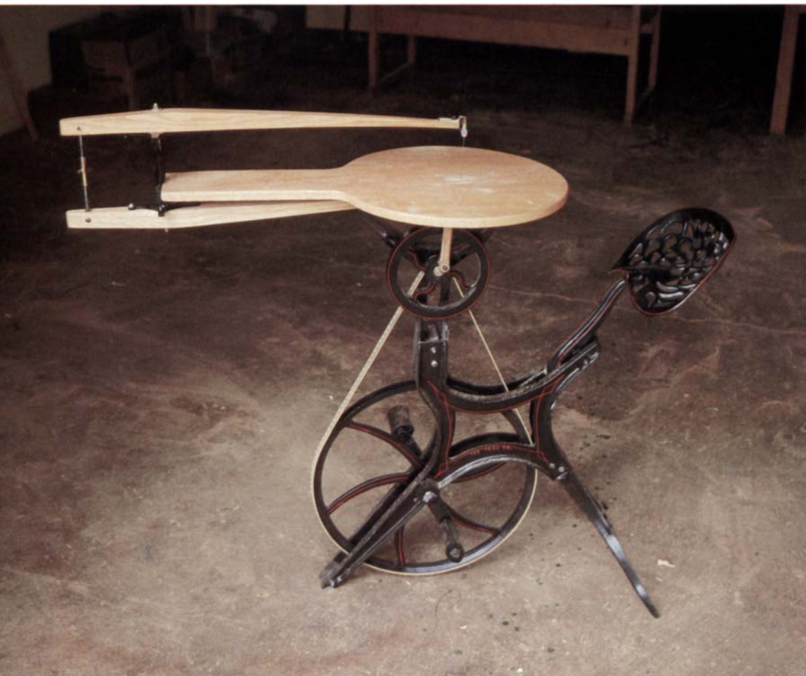
During the last half of the 19th century, the W.F. and John Barnes Co. manufactured a sophisticated line of hand- and foot-powered machinery. Bob Barnes demonstrates a No.4 crank-operated circular saw (right). The 1985 reproduction of the Barnes Velocipede (above) is virtually identical to the original, but is cast in aluminum instead of iron. It weighs 40 lb. and has a 24-in. throat. A pitman arm (above, right) converts rotary pedal motion to reciprocating sawing motion. A composition belt, whose perforations engage teeth in the pitman wheel, transmits power.
