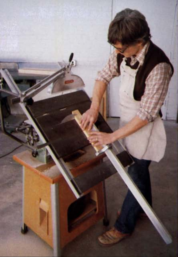
The Inca, conservatively rated at 1½ HP, passed all the precision tests with ease, but this unusual machine has what many consider to be three main drawbacks: The arbor is non-standard size, a 10-in. blade won't fully retract beneath the table surface, and the table has to be tilted for angled cuts, as shown.
