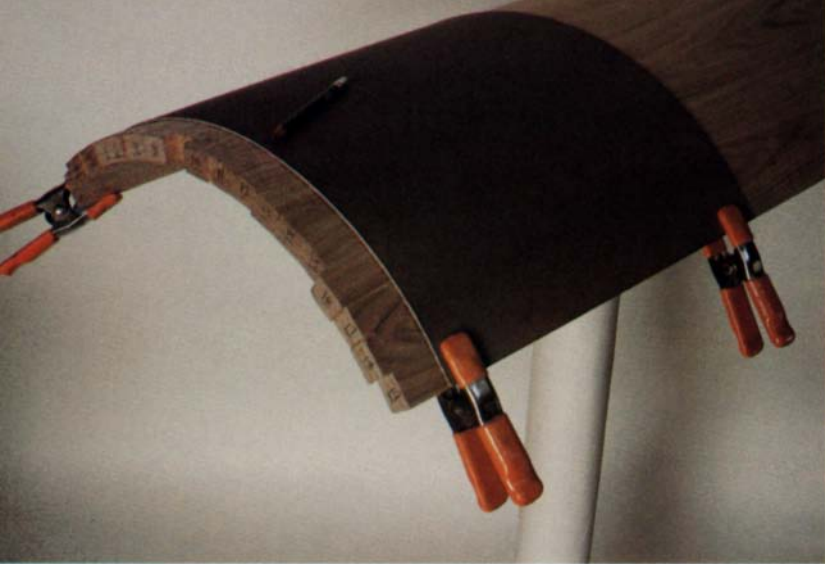
Plane panel edges, then use a squared-up piece of flexible material to scribe a line on the panel end square to the good edge.
