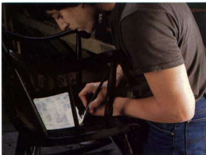
Belajonas uses his hand as a brace, above, to support his brush as he paints the center part of the seat yellow. For a mellow, aged effect, he adds a brownish-yellow glaze over the yellow, then streaks it across the width of the yellow seat with a crushed paper towel, right. He lets the glaze dry overnight, then seals it with satin varnish.
