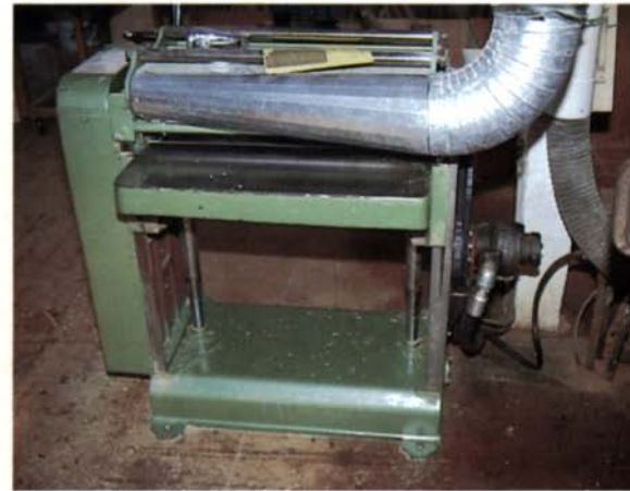
pumps (the belt driven units with hoses) circulate hydraulic fluid around the shop through steel pipes under the floor and up through hoses to motors on each machine, like the radial-arm saw and planer, top and bottom, right.
