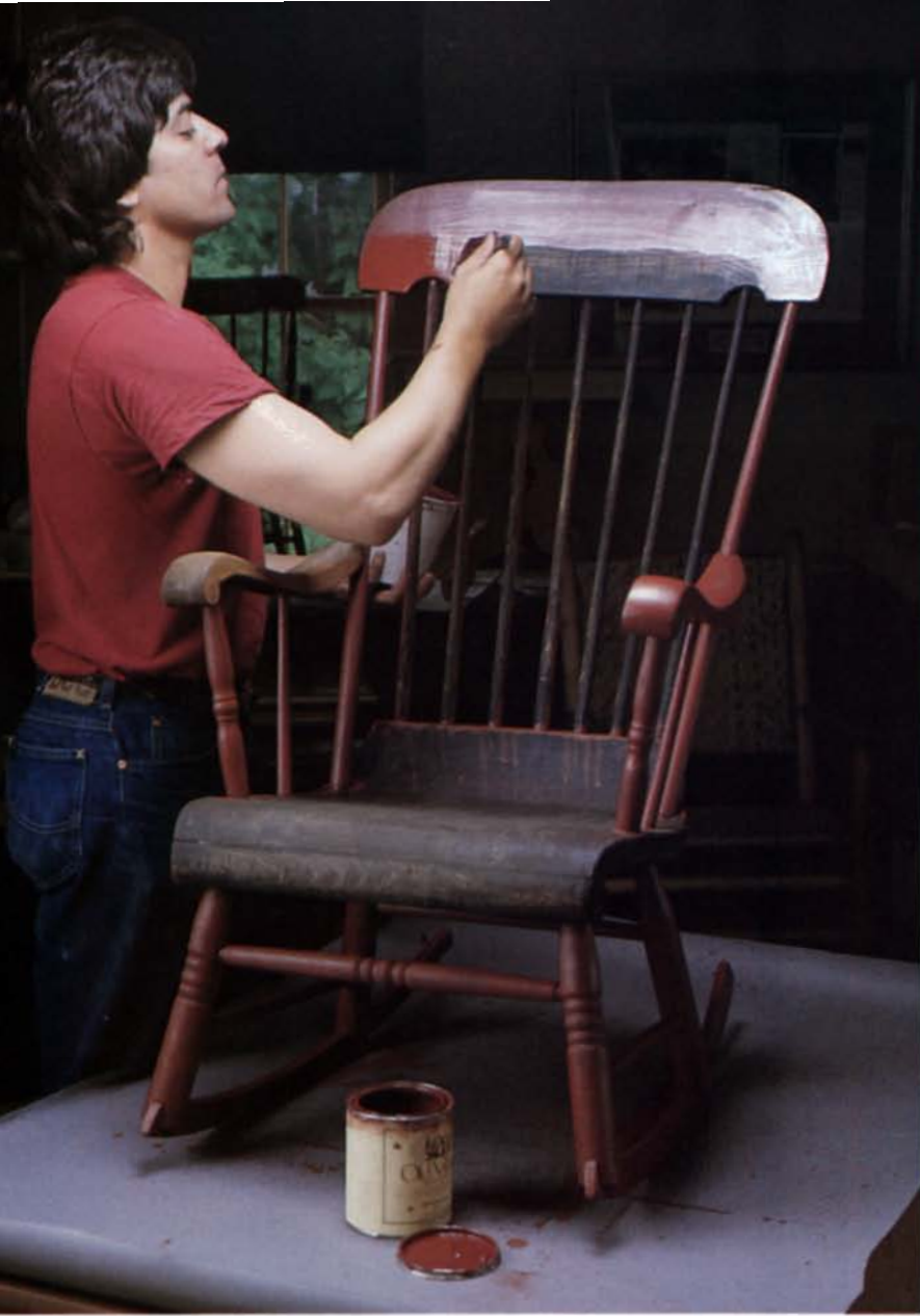
Belajonas paints a thin, brick-red undercoat on the chair, above, which has already had its old finish stripped off. Before adding a coat of black paint, he makes a graining comb by cutting different-sized notches into the edge of a 3-in. long piece of belt leather, above right. By gently dragging the comb up-and-down through the still-wet black paint on the rungs, right, he removes enough of the black to let the red show through as a tiger-stripe grain pattern.
