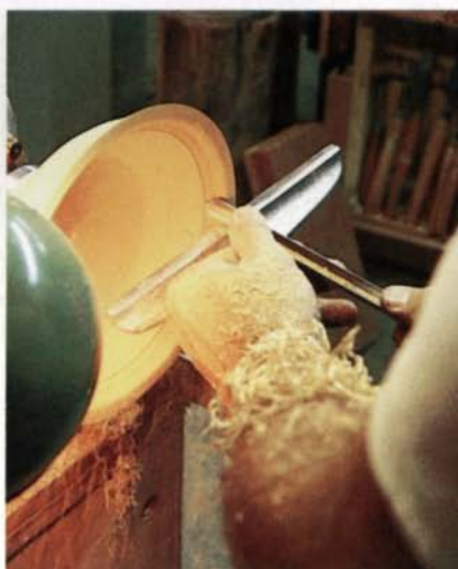
Turning student Nils Agrell, above, braces the tool handle against his hip to steady the cutting edge, while he manipulates the bevel and flute angles with his hands held high on the tool. To hollow a bowl on the lathe's outboard rest, right, adjust the flute to the 9 to 10 o'clock range and skim the tool bevel along the cut surface as you arch the chisel deeper into the blank. A fingernail gouge rides its bevel up the outside of a bowl, far right, smoothly cutting across the wood fibers. Keeping the bevel against the wood at all times prevents the cutting edge from digging into the stock.
