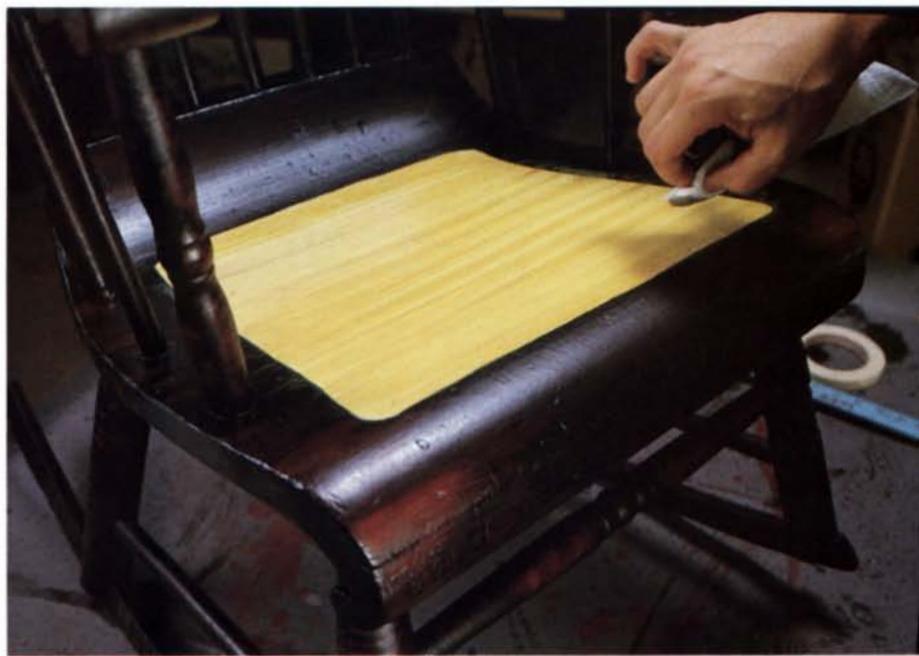
Belajonas uses his hand as a brace, above, to support his brush as he paints the center part of the seat yellow. For a mellow, aged effect, he adds a brownish-yellow glaze over the yellow, then streaks it across the width of the yellow seat with a crushed paper towel, right. He lets the glaze dry overnight, then seals it with satin varnish.
