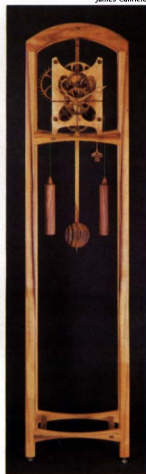
Westphale's first clock, above, ran but required 12 lb. of drive weight. He has since refined the designs—the contemporary grandfather clock, at right and on the facing page, will run on 4 lb. (the less weight, the less stress on the bearings) and is accurate to a half-minute per day. It sells for $6,000.
