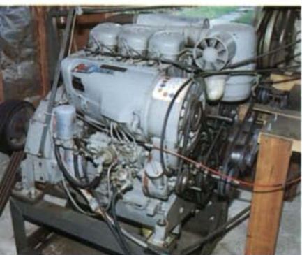
Abner Miller runs a small shop with a 3-cylinder, air-cooled diesel (above). Miller runs his smaller machines off a secondary wall-mounted shaft. The main shaft crosses under the shop floor perpendicular to the wall-mounted shaft. A V-belt with a 90° twist transfers power from the main shaft to the wall shaft.
