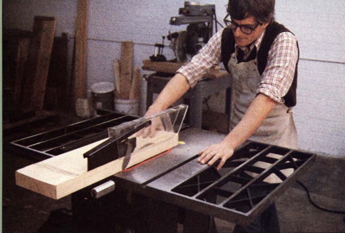
A study in patience: The Sears flexible shaft drive tablesaw will rip 8/4 stock, but at a pace that tends to put the operator to sleep. Preiss prefers the older, belt-drive models.
