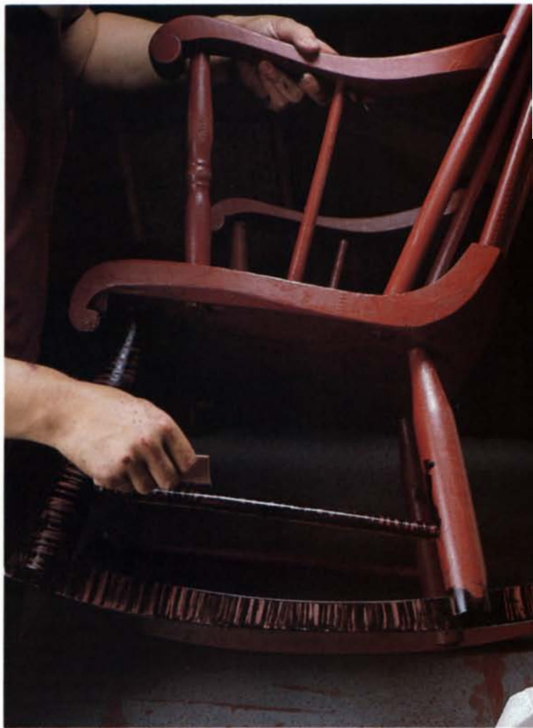
Belajonas paints a thin, brick-red undercoat on the chair, above, which has already had its old finish stripped off. Before adding a coat of black paint, he makes a graining comb by cutting different-sized notches into the edge of a 3-in. long piece of belt leather, above right. By gently dragging the comb up-and-down through the still-wet black paint on the rungs, right, he removes enough of the black to let the red show through as a tiger-stripe grain pattern.
