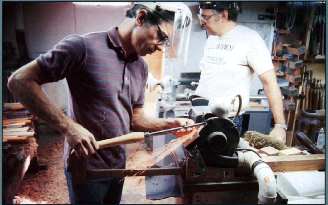
Zimmerman uses a sliding tool support to steady a long-handled gouge as he grinds the cutting edge on a 6-in. aluminum oxide wheel. Note how the tool's cutting edge rides directly on the blade and doesn't touch the grinder's tool rest, which is set for grinding skewers and other straight tools.
