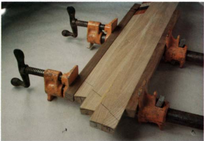
Tilting the jointer fence in toward the tables to bevel the strips allows you to joint glued-up segments (top left). When jointing narrow single strips, brad awls make good push sticks. After beveling, glue up pairs of strips, then pairs of pairs, and so on. As the glued-up segments get larger, use larger clamps to assemble them, as shown at bottom left. Dark strips are clamping cauls, which protect the strip edges. The final glue joint is on the panel's centerline. A combination of clamps and weight is usually necessary to draw the joint tight on both the inner and outer faces of the panel (right).
