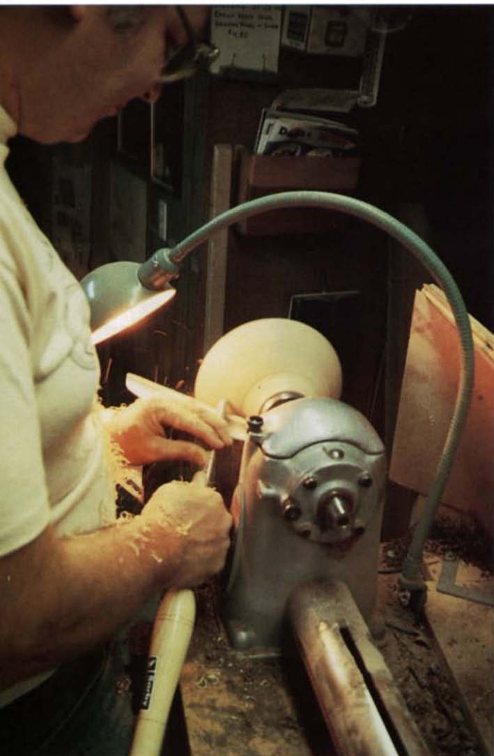
Turning student Nils Agrell, above, braces the tool handle against his hip to steady the cutting edge, while he manipulates the bevel and flute angles with his hands held high on the tool. To hollow a bowl on the lathe's outboard rest, right, adjust the flute to the 9 to 10 o'clock range and skim the tool bevel along the cut surface as you arch the chisel deeper into the blank. A fingernail gouge rides its bevel up the outside of a bowl, far right, smoothly cutting across the wood fibers. Keeping the bevel against the wood at all times prevents the cutting edge from digging into the stock.
