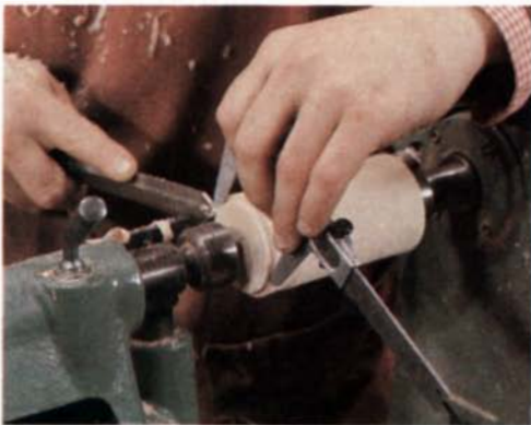
Turn a 1/8-in. tenon or flange on each end of the cylinder to fit the spigot chuck. Hold the parting tool in one hand and the calipers in the other. Stop cutting when the calipers slip over the tenon.
