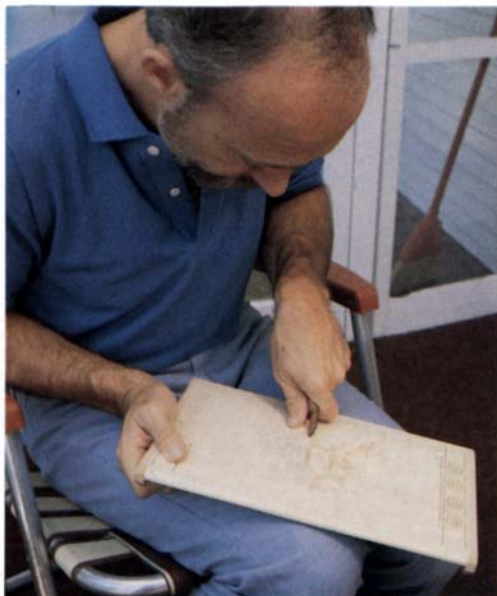
The sides and lids of Barton’s jewelry boxes (facing page), show delicate and complex patterns. Barton cuts the curved pattern with his knife held at a 65° angle to the wood. The key to the kerbschnitzen is to lock your wrist as shown, so your thumb and fingers guide the cut. Hold your elbow close to your body for better leverage and control. Barton works on his lap and rotates the wood to cut in different directions.
