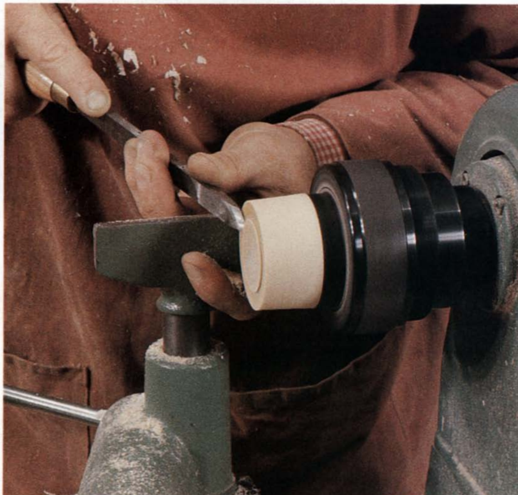
A second shearing cut with the skew chisel trues up the rim of the lid. Tilt the short point of the skew away from the wood to avoid a catch.
