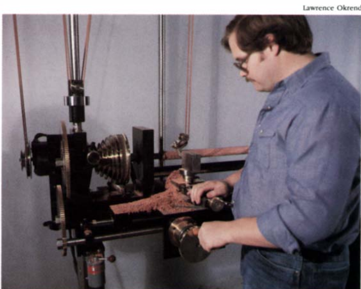
Ray Lawler demonstrates spiral cutting. The travel of the slide rest is controlled by the brass gears mounted on the headstock.
