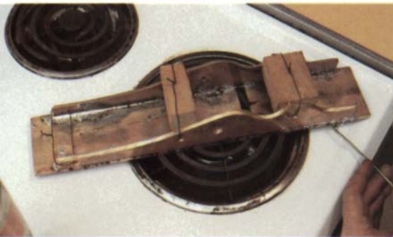
Brass can be bandsawn with an 18-TPI blade (top left). The metal has been sprayed with layout dye, a colored shellac that cuts glare and shows fine scribe lines clearly. With both sides clamped in the vise (top center), bandsaw marks can be filed away. To reach into tight corners (top right), grind the edge of a file to an angle that will fit. For soldering, pre-heat the brass on a stove (left) until it reaches a temperature where the solder almost flows. Use a propane torch to bring each successive joint up to full heat.
