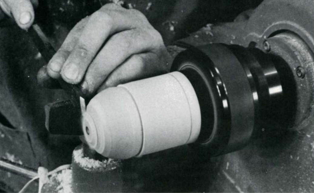
Fit the lid on the base and finish shaping the box with the skew chisel.
