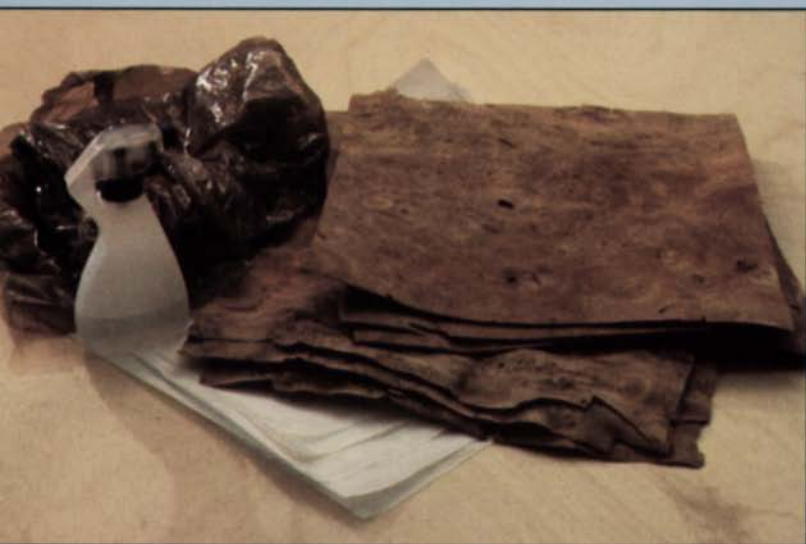
A little water, patience and pressure can transform bumpy veneers (bottom three sheets) into workable material (top sheets).
