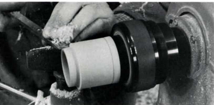
After sanding and waxing the inside, trim the flange to fit the lid. Use the long point of the skew as a scraper.
