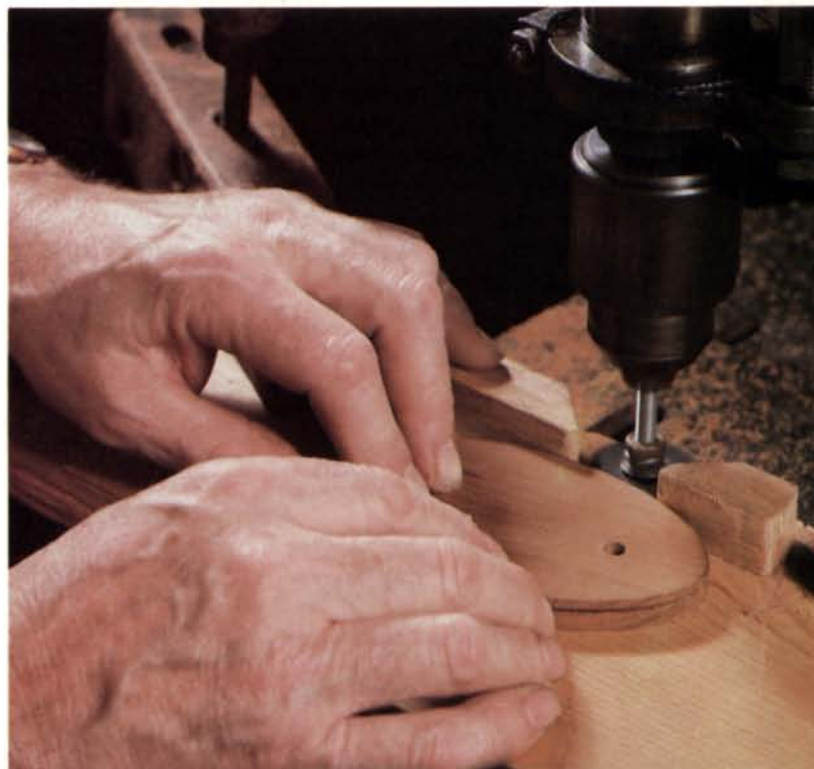
Top photo shows two partially finished baskets and the makings of another—hardwood oval base, oak staves, superfine chairseat cane and shopmade brass 'ears' as anchor points for the hinges. The middle photo shows the built-up wooden form that controls the shape. At bottom, Hilbert cuts a groove in the base for the staves, using a small circular sawblade in a drill press.
