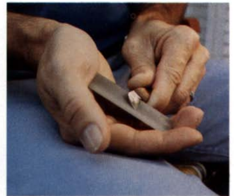
Sharpen the cutting knife at a 10° angle to the stone, as shown above. For a straight, smooth edge, always work on a stone that is large enough to hone the entire blade at once.
