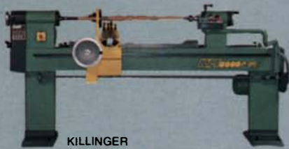
KILLINGER West German Duplicating Lathe with Electronic Duplication, 60" capacity, and three cutters KM5000SM
