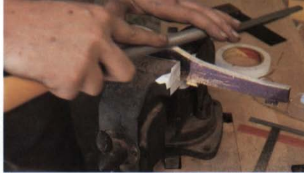
Brass can be bandsawn with an 18-TPI blade (top left). The metal has been sprayed with layout dye, a colored shellac that cuts glare and shows fine scribe lines clearly. With both sides clamped in the vise (top center), bandsaw marks can be filed away. To reach into tight corners (top right), grind the edge of a file to an angle that will fit. For soldering, pre-heat the brass on a stove (left) until it reaches a temperature where the solder almost flows. Use a propane torch to bring each successive joint up to full heat.
