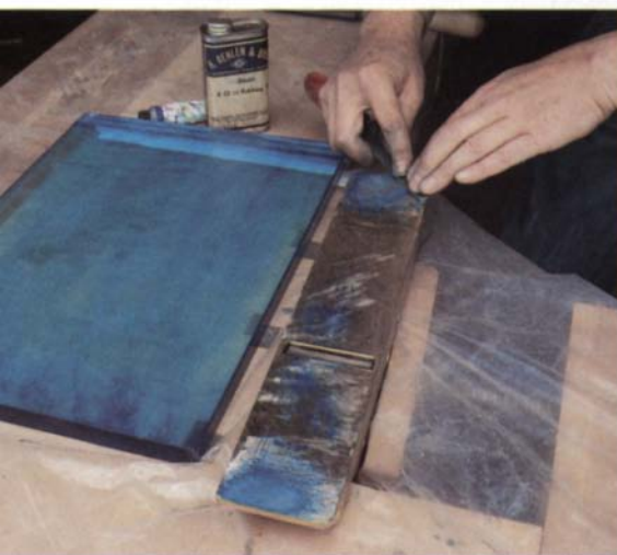
To flatten the sole, test it on a reference plate of heavy glass spread with blue oil paint (left). The thin paint transfers only to high spots on the sole. File and scrape these areas down, then test again on the glass, repeating until the critical areas at toe, heel and throat are fully covered by blue (for the rest of the sole an even spread of about 70% is adequate). A metal scraper (above) is used something like a paring chisel, working in a crosshatched pattern. The tool takes a series of fine, powdery shavings about 1/8 in. wide.
