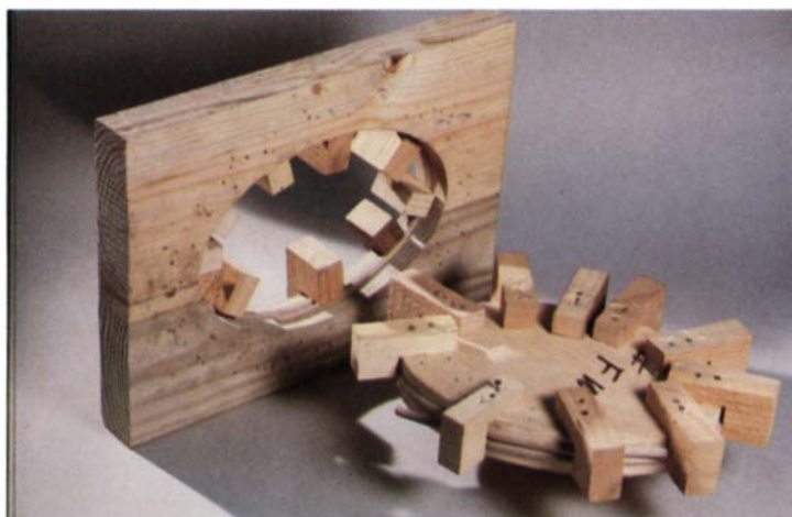
Half-round oak rims—one for the inside, one for the outside—are boiled, then wove into shopmade bending forms for drying.
