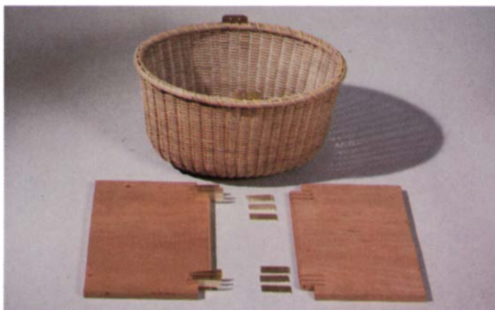
Hilbert reinforces the wood at the hinge points by epoxying brass strips into saw kerfs. Lid is bandsawn oval after fitting.
