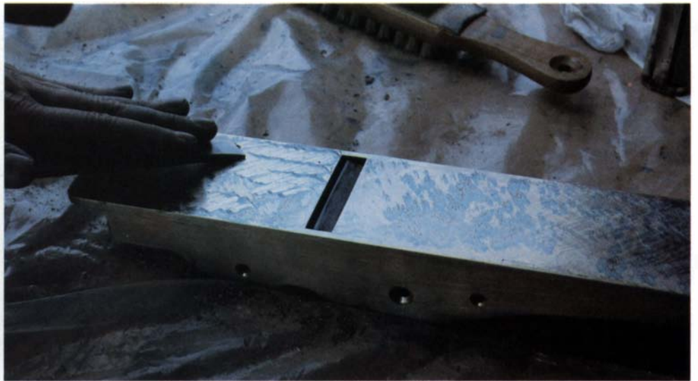
To flatten the sole, test it on a reference plate of heavy glass spread with blue oil paint (left). The thin paint transfers only to high spots on the sole. File and scrape these areas down, then test again on the glass, repeating until the critical areas at toe, heel and throat are fully covered by blue (for the rest of the sole an even spread of about 70% is adequate). A metal scraper (above) is used something like a paring chisel, working in a crosshatched pattern. The tool takes a series of fine, powdery shavings about 1/8 in. wide.
