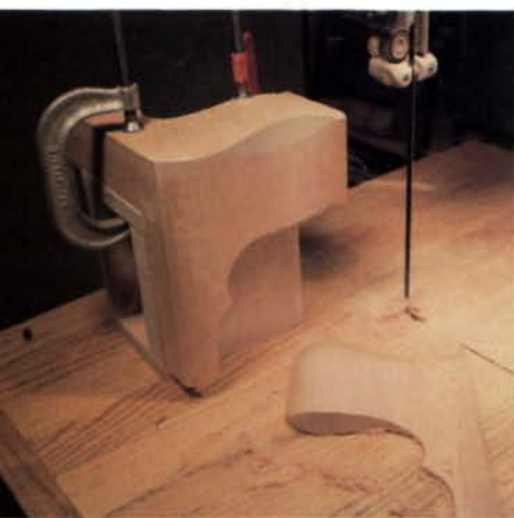
Ogee bracket feet are glued up while square then cut to shape on the bandsaw. Supporting the foot over a wooden box allows the ogee profile to be cut on the bandsaw (left). Finial is lathe turned, then flutes are marked out in indexing jig and carved by hand. To lay out the flame, divide flame into six longitudinal sections and five latitudinal sections to form a grid (below). Connect points on the diagonal to form spiral lines. Pencil holder shown marks out axis lines.
