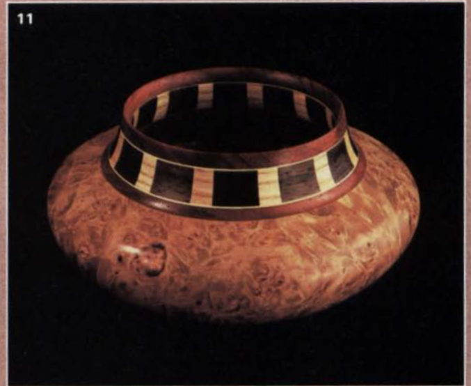
After gluing on a hardwood rim and foot, the blank is screwed to a faceplate. The center is drilled to depth with a 3/4-in. multispur bit, then the tailstock is brought up for support (8). First the outside is turned to shape with scrapers (9), then the inside is scraped, leaving the tailstock in place (10) for as long as possible to support the work. After sanding, the bowl is parted off the lathe and the bottom sanded flat before finishing with Waterlox (11).
