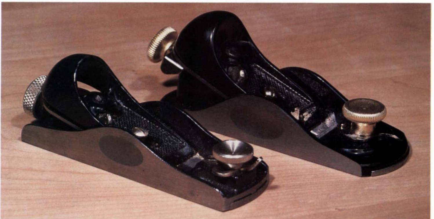
Small and light, the block plane is the choice for one-handed planing jobs. Unlike a bench plane, block plane blades cut bevel up. Top of the line models, like these Stanleys, have adjustable blades and mouths. Blade angle on the No. 9½ (right) is 20°. The low-angle No. 60½ has a 12° blade angle.
