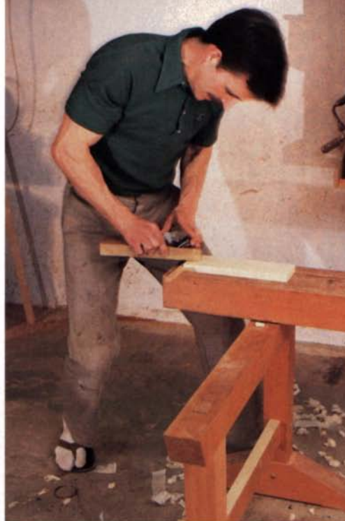
Fast, flattening or hogging work is done with the large muscles of the legs and back, while the rest of the body remains relaxed. Balance is ensured by keeping the body's center of gravity inside the broad stance of the feet.
