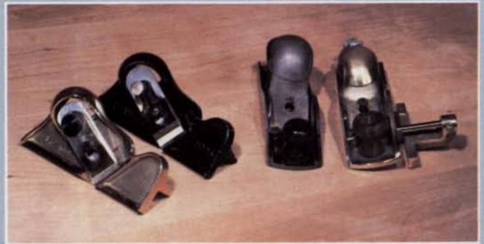
Entrepreneur Tom Lie-Nielson has brought two vintage Stanley specialty block planes back to life in flashy, manganese-bronze incarnations. Shown here with the cast-iron Stanley originals are (left) the No. 95 edge-trimming block plane and (right) the No. 140 skew-rabbit block plane.
