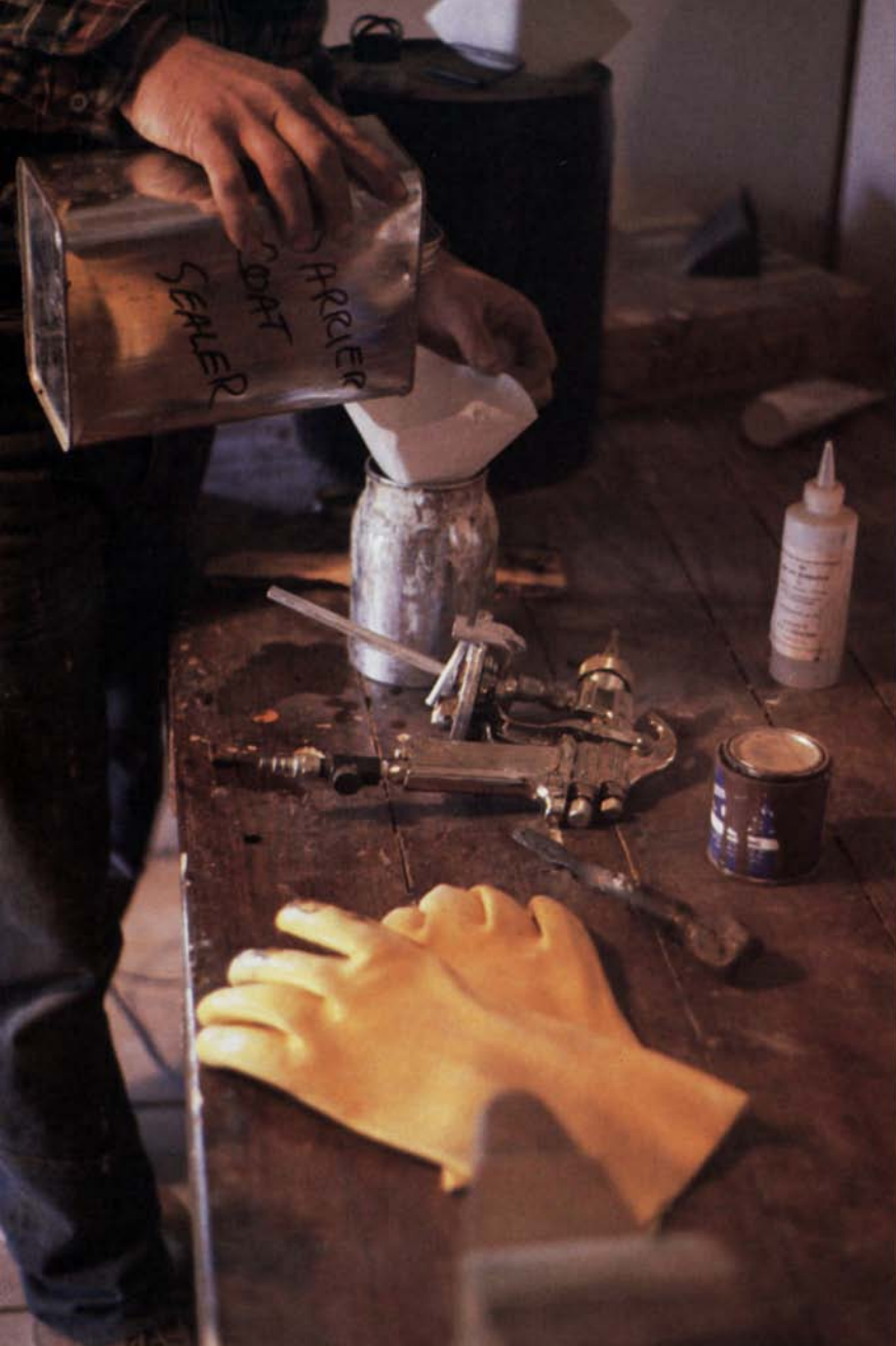
To ensure that the lacquer is free of all dust and impurities, filter each batch through a cone filter as you fill the spray gun cup.
