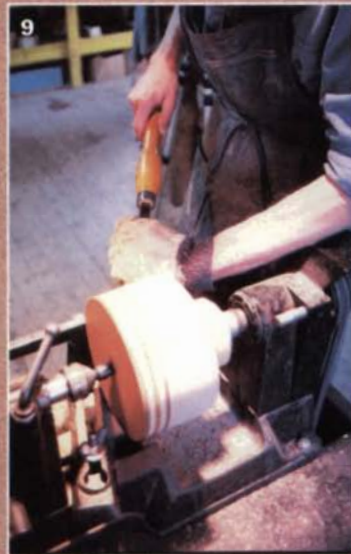
After gluing on a hardwood rim and foot, the blank is screwed to a faceplate. The center is drilled to depth with a 3/4-in. multispur bit, then the tailstock is brought up for support (8). First the outside is turned to shape with scrapers (9), then the inside is scraped, leaving the tailstock in place (10) for as long as possible to support the work. After sanding, the bowl is parted off the lathe and the bottom sanded flat before finishing with Waterlox (11).
