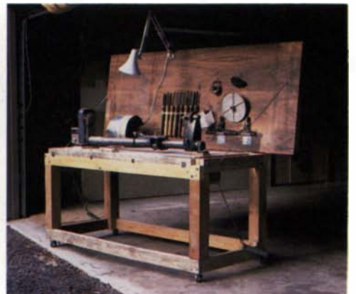
Workbench top swings up on hinges, as shown in center photo. Lathe is then raised into position. A length of angle iron on a hinged wooden strip at the front of the bench holds the lathe base up, as shown in the photo at right.
