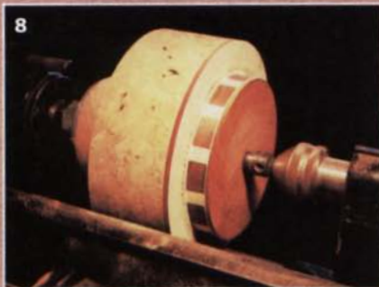
Gluing up begins with a burl-blank bandsawed round then sanded flat with a custom-made sanding disk (4). After gluing on a layer of veneer, the pre-planned segment "grid" is drawn on the blank (5) and the segments glued in place one-at-a-time. Checks for square at 90° (6), 180° and 270° reveal cumulative errors in segment size and allow corrections. The completed solid-block, multi-angle segment band (7) is set aside to dry.
