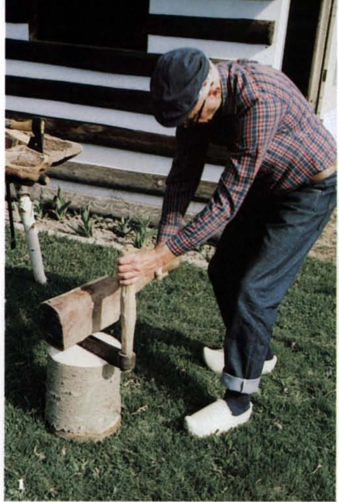
A froe and mallet split the shoe blank out of the green log (1). A 10-in. diameter log yields four blanks. Sieg uses a side ax to square the sole and one side, then begins shaping the shoe (2). The ax is beveled only on the side away from the cut, making it an efficient planing and carving tool. After bracing the shoe with his bench and thigh (3), he refines the shoe shape with the lever-like block knife that pivots in a screw eye attached to the bench. The leverage of the long block knife makes it good for heavy crossgrain paring (4).
