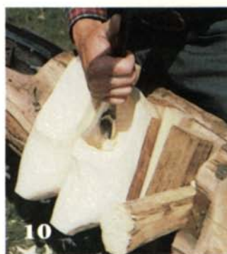
To hollow toe, Sieg turns the auger with his right hand while guiding the shaft with his left (9 and 10). The block knife creates a ready-to-wear finish (11).
