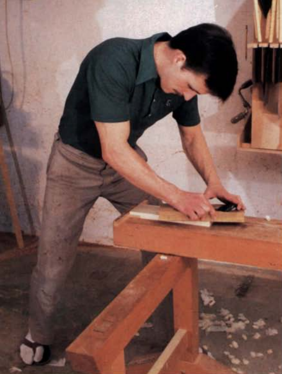
Fast, flattening or hogging work is done with the large muscles of the legs and back, while the rest of the body remains relaxed. Balance is ensured by keeping the body's center of gravity inside the broad stance of the feet.
