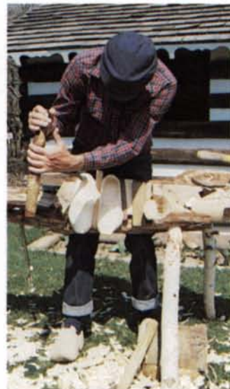
Sieg wedges the shoes to the bench, which he braces with his legs (5), then bores a hole in the heel with a T-handled spoon auger. After boring two holes, he uses the auger like a pry bar to break out large chunks of waste from between the two holes (6). After clearing the heel, Sieg uses the spoon auger like an ice cream scoop to enlarge the opening and shape it to fit the foot (7). Large curls of wood are removed from the top (8), until the wall reaches proper thickness and from the bottom until the arch is properly contoured for support and comfort.
