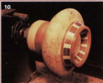
After gluing on a hardwood rim and foot, the blank is screwed to a faceplate. The center is drilled to depth with a 3/4-in. multispur bit, then the tailstock is brought up for support (8). First the outside is turned to shape with scrapers (9), then the inside is scraped, leaving the tailstock in place (10) for as long as possible to support the work. After sanding, the bowl is parted off the lathe and the bottom sanded flat before finishing with Waterlox (11).
