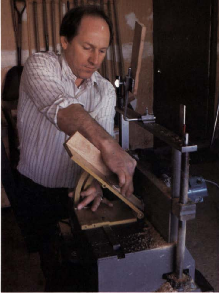
Don Strong, left, cuts a sliding dovetail on the Joint-Matic, a router joinery machine he invented and manufactures in his garage machine shop. He subcontracts foundry work, then does final assembly himself. A similar small-scale manufacturing setup turns out the Wirth Machine, a sophisticated joinery tool developed by former aerospace engineer John Wirth, right.
