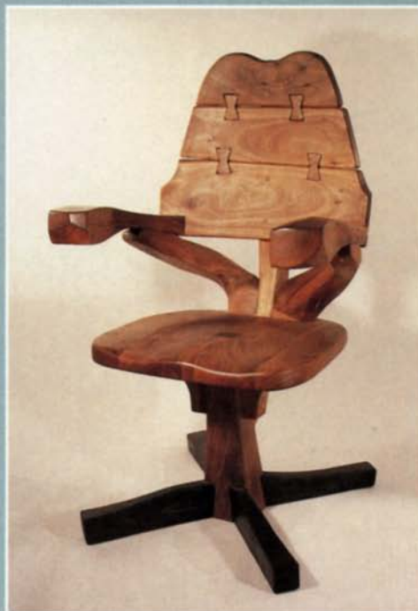
Erik Gronborg's "Big Chair" (above) is assembled using simple, exposed joinery. He bandsaws avocado logs, often mimicking the log's natural shape in the finished form. "Treasure Chest" (right) sports ceramic panels in an avocado frame. The interior is lined with velvet.
