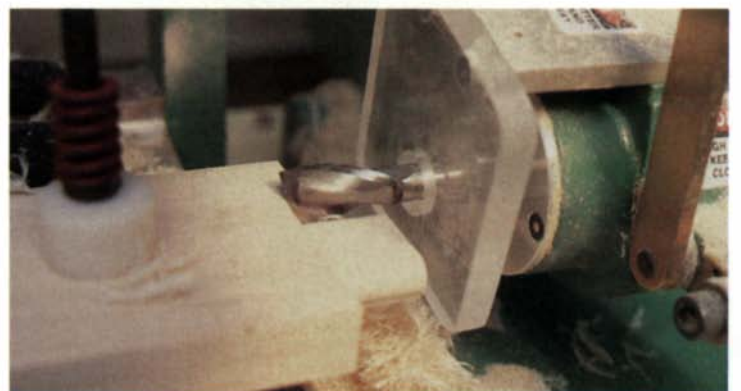
The Wirth Machine set up for tenoning. The template follower, top, traces the template, guiding the bit to reproduce its profile on the end of the stock. As the bit cuts, the wood is held firmly against a plastic plate, setting the shoulder depth.
