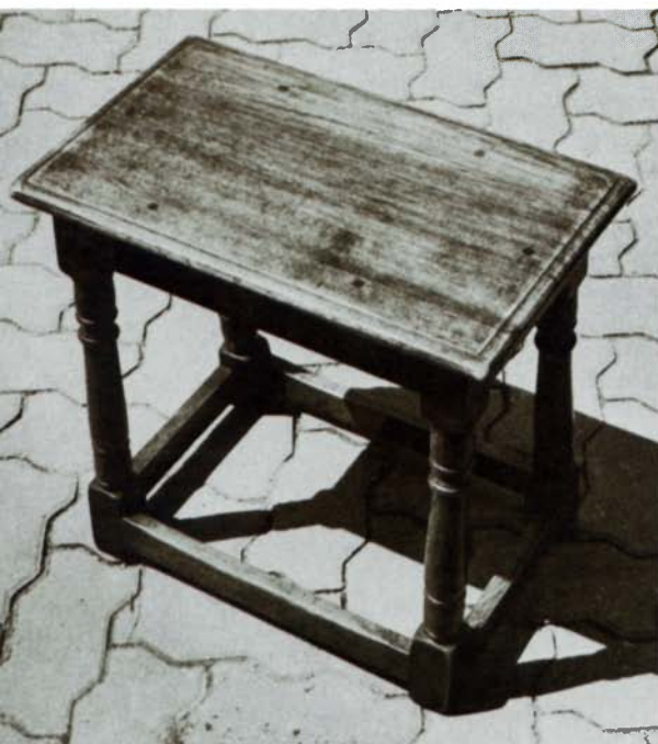
Wallace's brown oak copy of a 17th-century joynt stool, left, is held together by fox-wedged tenons. The top is attached to the apron rails with square wooden pegs. A fox-wedged tenon and mortise, above, is ready for assembly. Since the faces of the pieces are to be flush, the tenon is offset for greater strength. The mortise, right, has been too heavily undercut, causing the tenon to fracture at the end of the top kerf. The wedges and kerfs, however, are perfect.
