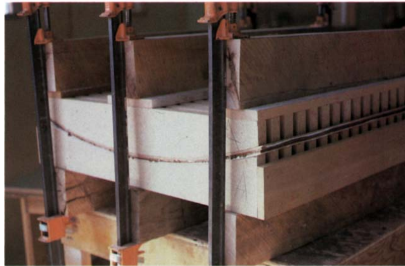
Each bent panel requires its own form constructed of 1-in. particleboard ribs spaced \frac{3}{4} in. apart and fastened together with battens and/or backing boards to keep them aligned. Stout cauls and heavy bar clamps distribute pressure evenly at glue up.
