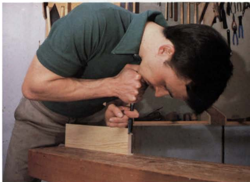
Swensson clamps the work with his thigh and shin (top photo) as he begins to tap out the waste from a dovetail. Heavy paring cuts can be driven by chin pressure (photo above), using the strong muscles of the upper body. This provides good control.
