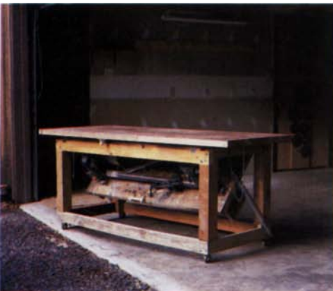
Workbench top swings up on hinges, as shown in center photo. Lathe is then raised into position. A length of angle iron on a hinged wooden strip at the front of the bench holds the lathe base up, as shown in the photo at right.
