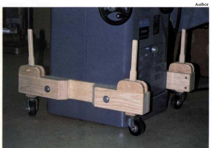
One version of Henderson's retractable casters bolts directly to the sides of his tablesaw; another version, not shown, has a four-sided wooden frame that supports his Hitachi planer.
