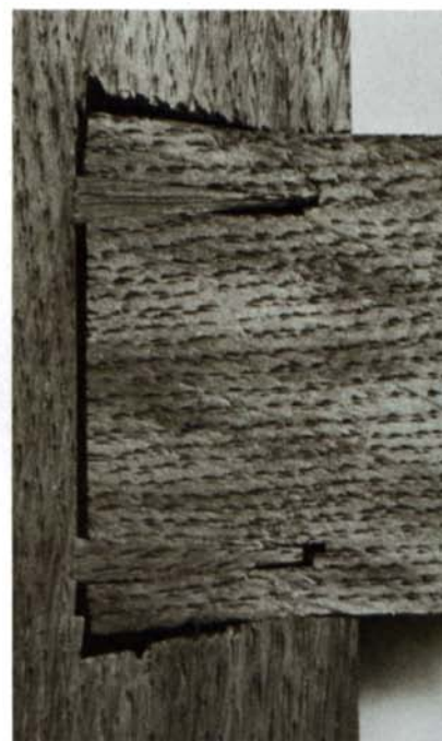
Wallace's brown oak copy of a 17th-century joynt stool, left, is held together by fox-wedged tenons. The top is attached to the apron rails with square wooden pegs. A fox-wedged tenon and mortise, above, is ready for assembly. Since the faces of the pieces are to be flush, the tenon is offset for greater strength. The mortise, right, has been too heavily undercut, causing the tenon to fracture at the end of the top kerf. The wedges and kerfs, however, are perfect.
