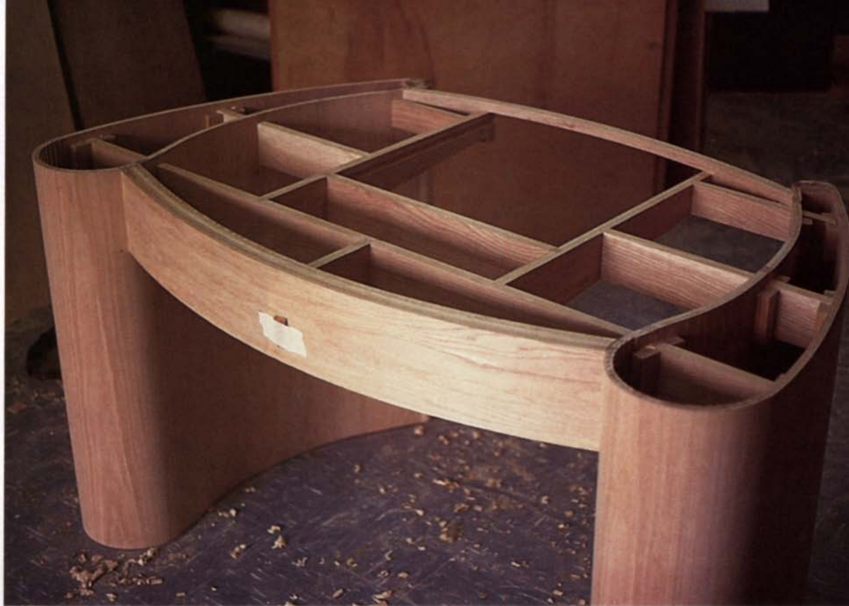
Plywood splines in tablesawn or routed grooves join bent panels together. Blocks temporarily tacked to the panel near the joint with hot-melt glue provide bite for handscrews. Scrap 1/8-in. plywood makes good spline stock. A framework of solid oak joins the desk's two columns, providing support for the top and a hanging surface for a drawer. Bent panels proved too thin for conventional joinery so McCaffrey fitted glue blocks around each frame member—in effect building a mortise around a tenon.
