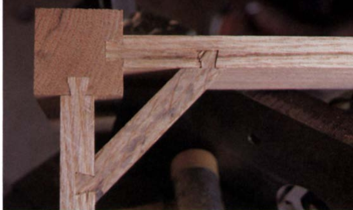
The Joint-Matic makes quick work of the sliding dovetails used in this leg-and-apron table joint with corner bracket. A compound miter gauge available as an option positions the bracket to cut the angled pins.
