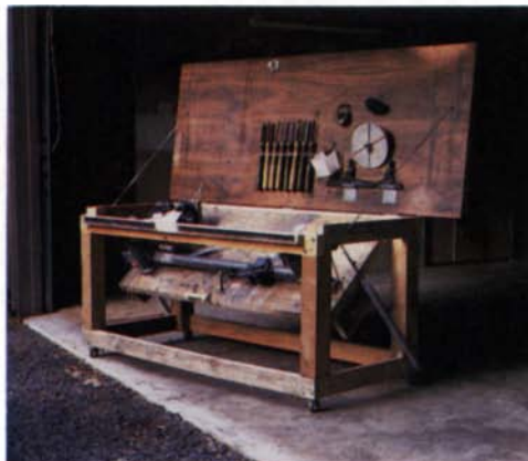
Workbench top swings up on hinges, as shown in center photo. Lathe is then raised into position. A length of angle iron on a hinged wooden strip at the front of the bench holds the lathe base up, as shown in the photo at right.
