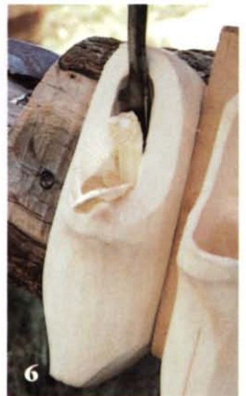
Sieg wedges the shoes to the bench, which he braces with his legs (5), then bores a hole in the heel with a T-handled spoon auger. After boring two holes, he uses the auger like a pry bar to break out large chunks of waste from between the two holes (6). After clearing the heel, Sieg uses the spoon auger like an ice cream scoop to enlarge the opening and shape it to fit the foot (7). Large curls of wood are removed from the top (8), until the wall reaches proper thickness and from the bottom until the arch is properly contoured for support and comfort.
