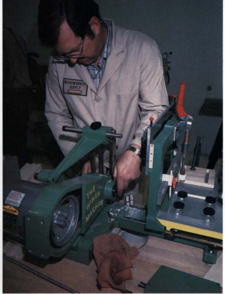
Don Strong, left, cuts a sliding dovetail on the Joint-Matic, a router joinery machine he invented and manufactures in his garage machine shop. He subcontracts foundry work, then does final assembly himself. A similar small-scale manufacturing setup turns out the Wirth Machine, a sophisticated joinery tool developed by former aerospace engineer John Wirth, right.
