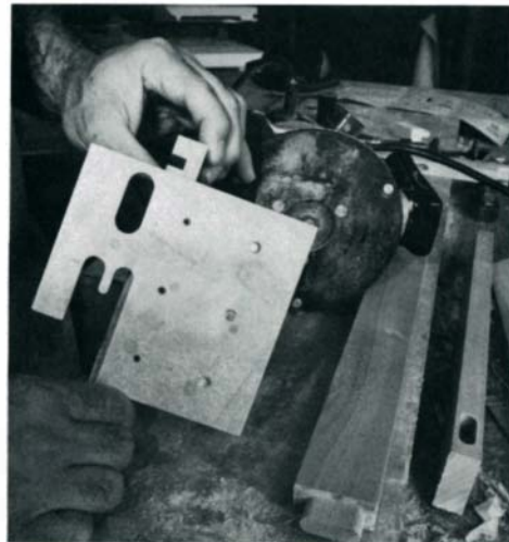
Combined with a router, Dean Martin's jig will cut both mortises and tenons. Closed slot at right guides bit for mortising and the tongue, left, is for tenoning.
