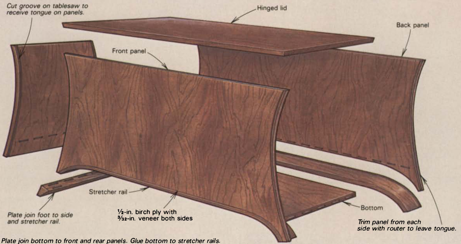
Plate join bottom to front and rear panels. Glue bottom to stretcher rails.
