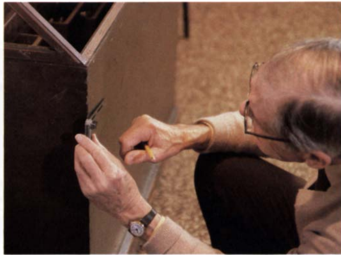
Lynch prefers a folding carpenter's rule, left, because it won't snap back as a steel tape might. Holding his bevel gauge handle parallel to the chest corner, he angles its tongue to match the dovetails, above. He records the angle with a protractor. For something as irregular as this tavern table leg, he uses a simple pen holder to trace contours. The Plexiglas edge of the wooden upright is set directly over the angled pen. As you run the plastic along the piece, the pen records the contour on paper on the instrument's base.
