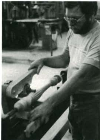
Julian Reid, above, operates a reeding jig—a carriage that rolls along the lathe ways carrying a router mounted on a pivoting arm. A bearing on the bit holder follows the contours of the work, which is locked in position by an indexing plate at the headstock. Mobile bedmaker William Blake, left, demonstrates his similar jig, which uses a simpler solid-pilot bit machined from tool steel (far left). The setscrew visible at the end of the bit locks the V-shaped cutter in place.
