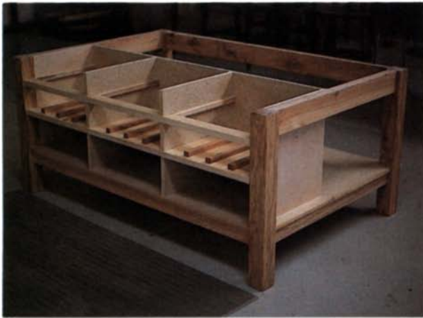
Assemble the 27-in. high utility table with mortise-and-tenon joints. Locate shelves to fit standard plastic drawers for small tools and odds and ends. Larger tools go on the bottom shelf. Make the 40-in. by 60-in. top from particleboard and 1/4-in. maple plywood. To plane long boards, right, Klausz uses a bench slave with the shoulder vise.
