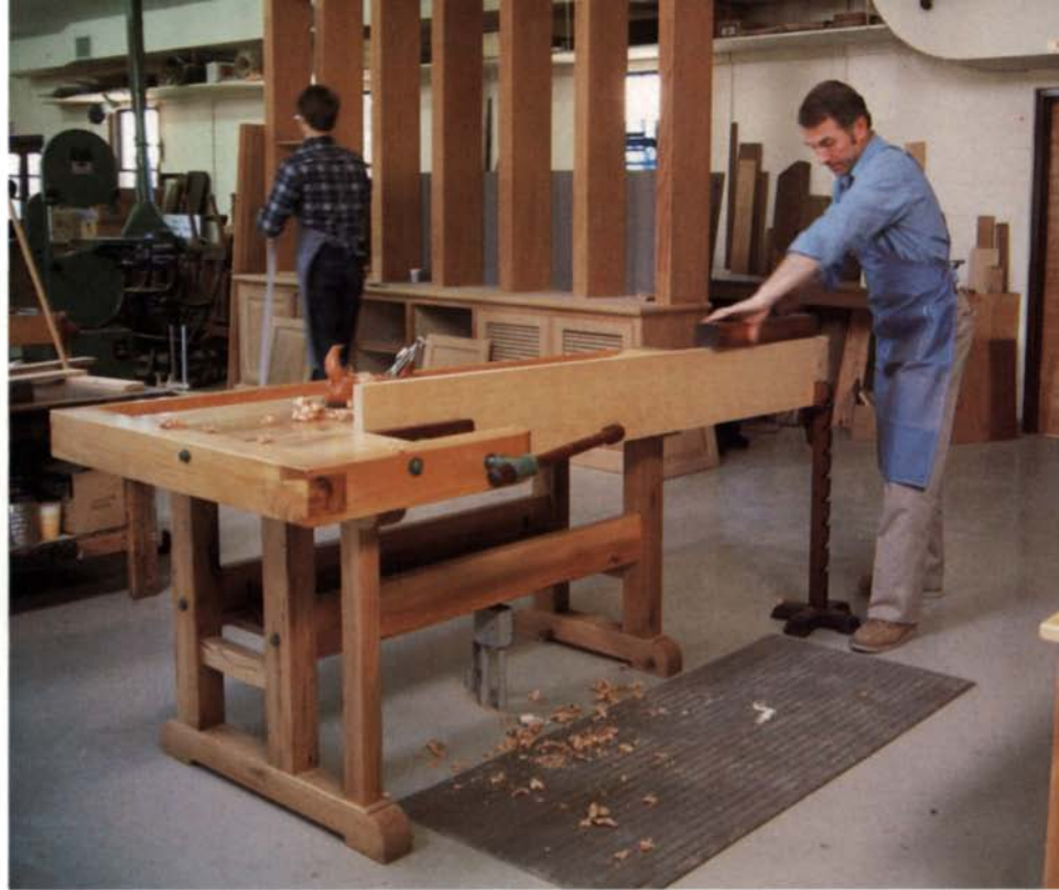
Assemble the 27-in. high utility table with mortise-and-tenon joints. Locate shelves to fit standard plastic drawers for small tools and odds and ends. Larger tools go on the bottom shelf. Make the 40-in. by 60-in. top from particleboard and 1/4-in. maple plywood. To plane long boards, right, Klausz uses a bench slave with the shoulder vise.
