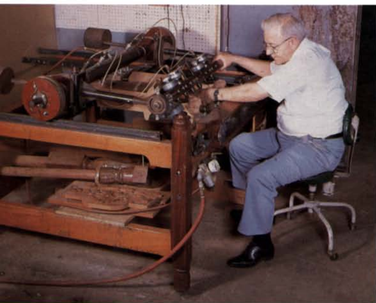
Robert Reid's shopmade duplicating router carves four knees at once, following a pattern mounted in the center.
