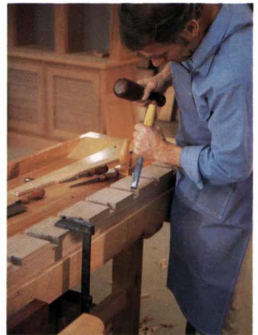
Benchtop is positioned on the base by bullet-shaped dowels, left. The base itself is low-grade hardwood. Before assembling the top, above, chisel out dadoed slots so L-shaped dogs fit flush with top.
