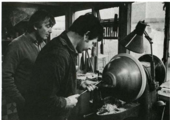
Michael Dickson watches Liam O'Neill finish off a large walnut bowl with a ¼-in. gouge. The rim of the bowl is jammed into a groove turned into the pine disc, which is screwed to a faceplate. Above are two bowls by Liam O'Neill and below a large elm bowl by Michael Dickson.
