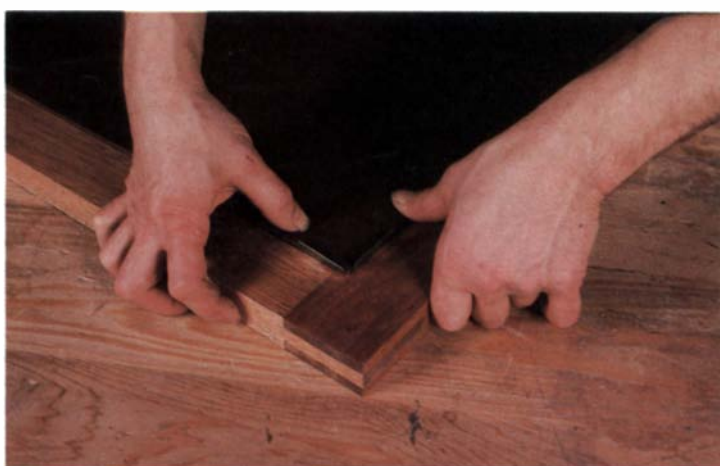
Single-edge razor blades help ease a tight-fitting panel into place in a rabbeted frame.
