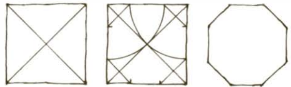
Scribe diagonals; then compass shows true octagon.
