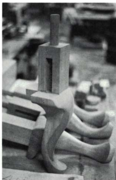
A bed with cabriole legs must have unusually heavy corner posts to withstand the strain put upon the rails. Note that this section of the post carries the tenon. If the tenon were on the upper section, the corner post would have to be mortised, weakening the construction.
