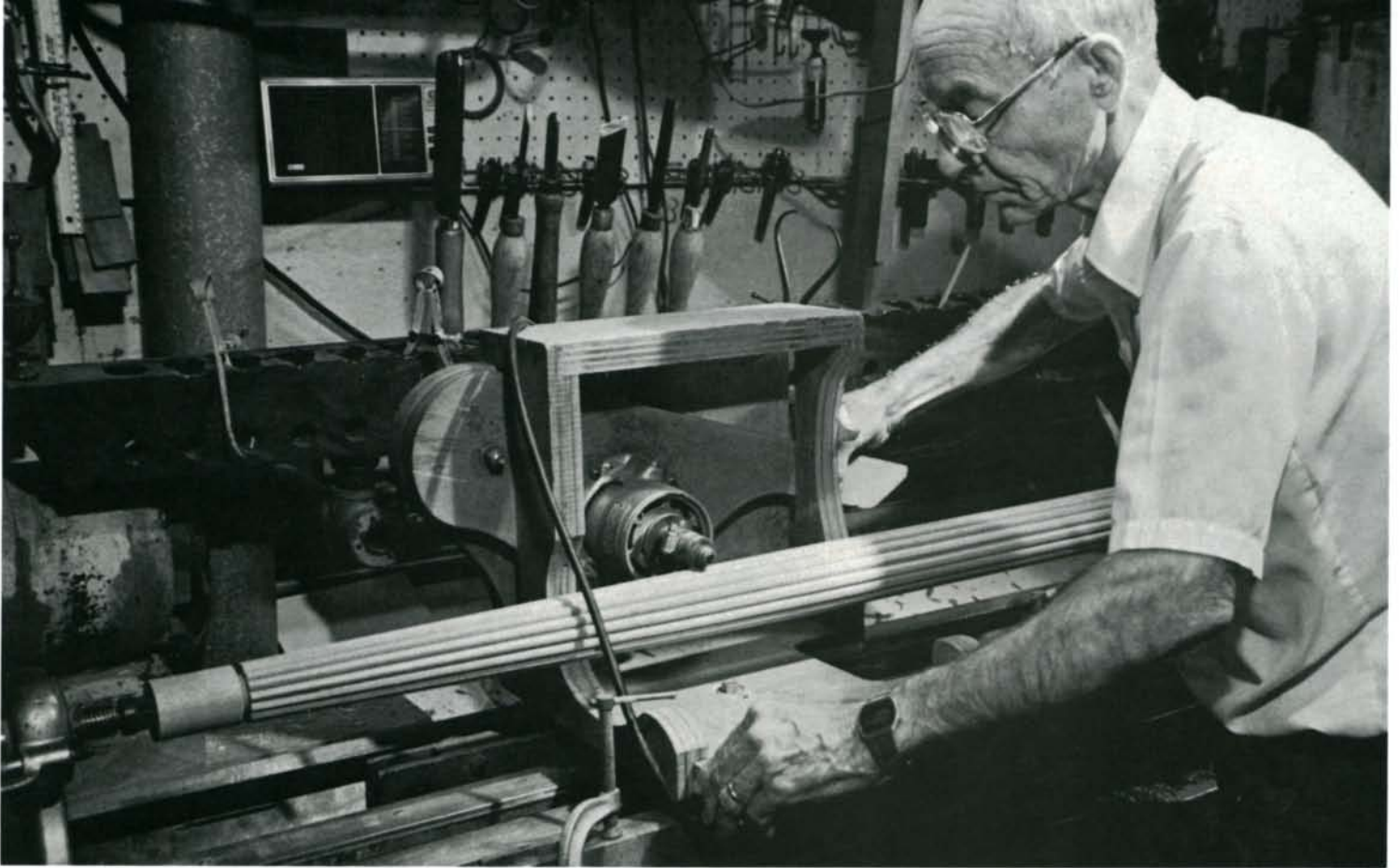
Julian Reid, above, operates a reeding jig—a carriage that rolls along the lathe ways carrying a router mounted on a pivoting arm. A bearing on the bit holder follows the contours of the work, which is locked in position by an indexing plate at the headstock. Mobile bedmaker William Blake, left, demonstrates his similar jig, which uses a simpler solid-pilot bit machined from tool steel (far left). The setscrew visible at the end of the bit locks the V-shaped cutter in place.
