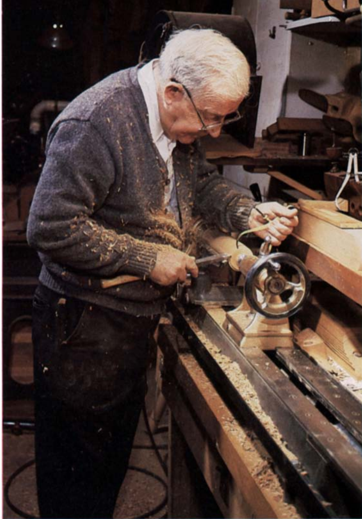
Robert Reid gauges a bedpost tenon to the right diameter, using calipers and a parting tool at several places along its length.
