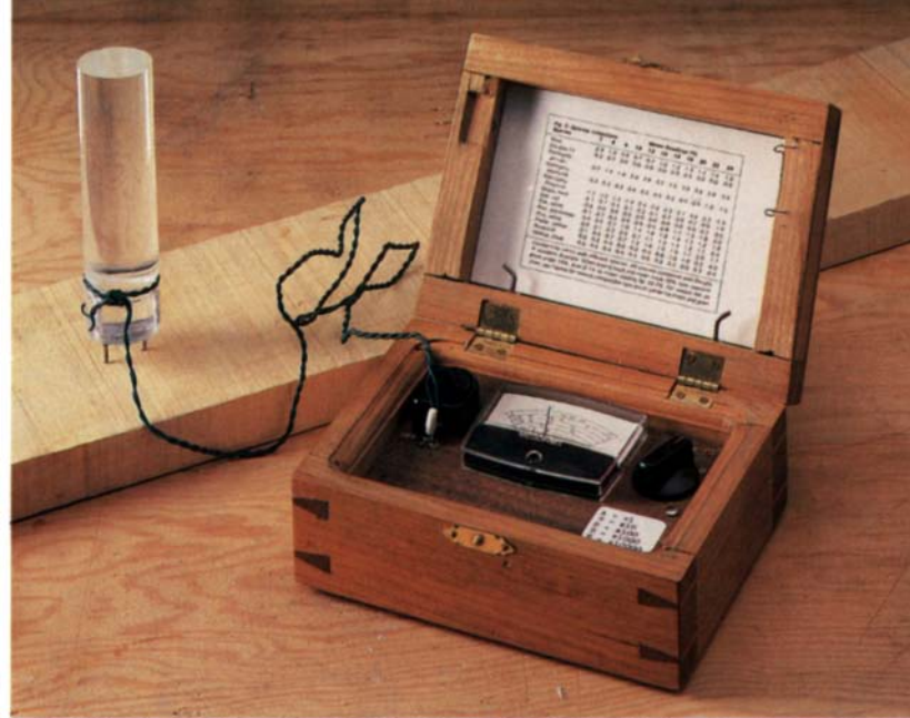
A few common electronic components, a plastic probe and species chart let you gauge moisture levels and anticipate wood movement for about $30. Jazz the unit up with a custom made box.
