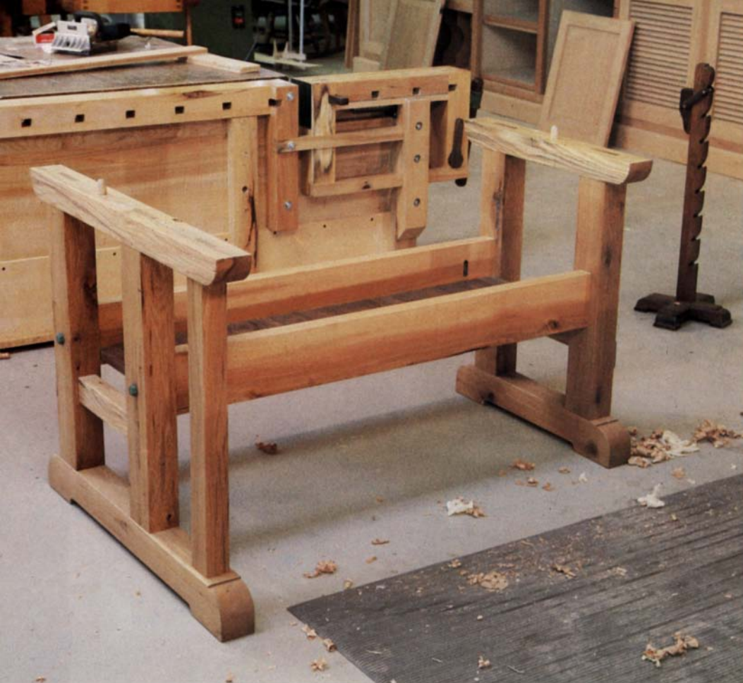
Benchtop is positioned on the base by bullet-shaped dowels, left. The base itself is low-grade hardwood. Before assembling the top, above, chisel out dadoed slots so L-shaped dogs fit flush with top.
