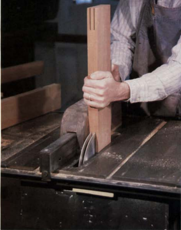
With two blades on the tablesaw arbor Erickson cuts both rail tenon cheeks in one pass, above. Rather than risk fingers cutting free-hand, he's designed a tenoning push stick that rides the rip fence and holds the stock upright. A 1x2 table and fence support the stile while drilling the louver holes, right. The block system shown below ensures accurate hole spacing.
