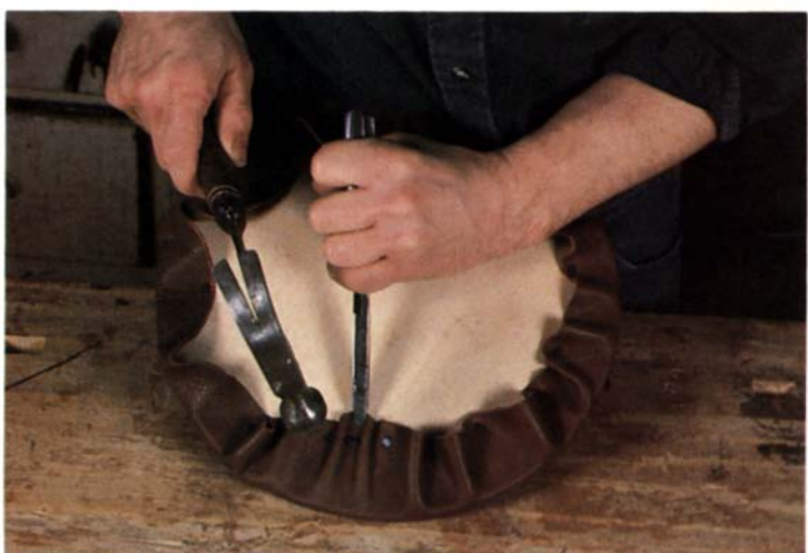
Flat-nosed pliers give added pull when tacking the leather to the seat panel.
