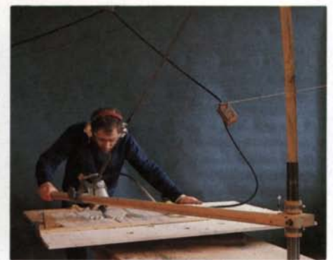
To make one version of Calibrated Earth , top, author built the small milling machine, right. The arm is less cumbersome and the work can be mounted on a turntable, making possible more the fluid, painterly compositions shown at far left and right. By painting the routed squiggles, Hogbin achieved an illusion of depth which suggests a cloud-filled sky or a flock of birds.
