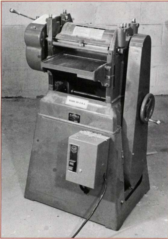
The 12-in. Parks 95 planer, with optional sheet-steel base and magnetic starter, is a comfortable 37½ in. floor to table.
