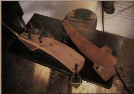
The chair's curved parts were produced with shaper profiling jigs such as the two shown for the arms, above left. Two were needed for each arm because clamp anchor points keep the jig from being fed past the knives in one continuous motion. Parsons, above right, has bandsawn a rough arm blank and is shaping it to the final profile with the first jig. He'll mount the part in the other jig to finish the job.
