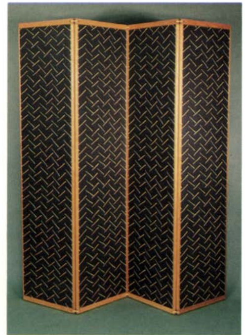
Author's lightest screen consists of wallpapered or fabric-covered panels contact-cemented into a cherry frame. The top and bottom rails (drawing at left) are permanently hinged but removable, so the panels can be pried out for re-covering.
