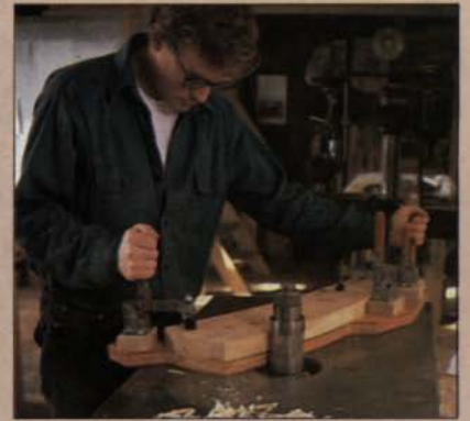
The chair's curved parts were produced with shaper profiling jigs such as the two shown for the arms, above left. Two were needed for each arm because clamp anchor points keep the jig from being fed past the knives in one continuous motion. Parsons, above right, has bandsawn a rough arm blank and is shaping it to the final profile with the first jig. He'll mount the part in the other jig to finish the job.
