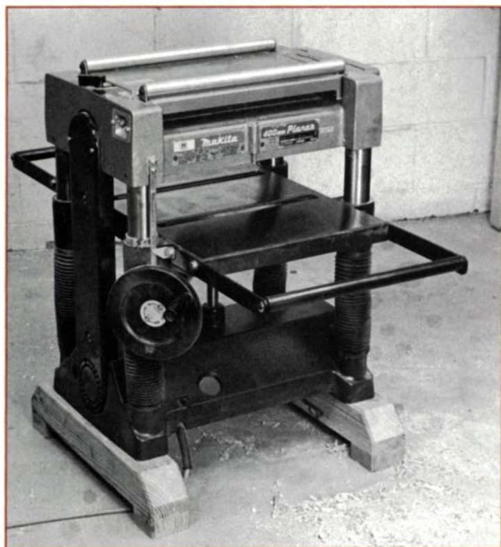
The Makita 2040 needs a boost. Without blocks, the table is only 20¼ in. from the floor in its highest position. A small, high-RPM, 110-volt, universal-type motor is concealed in the base.
