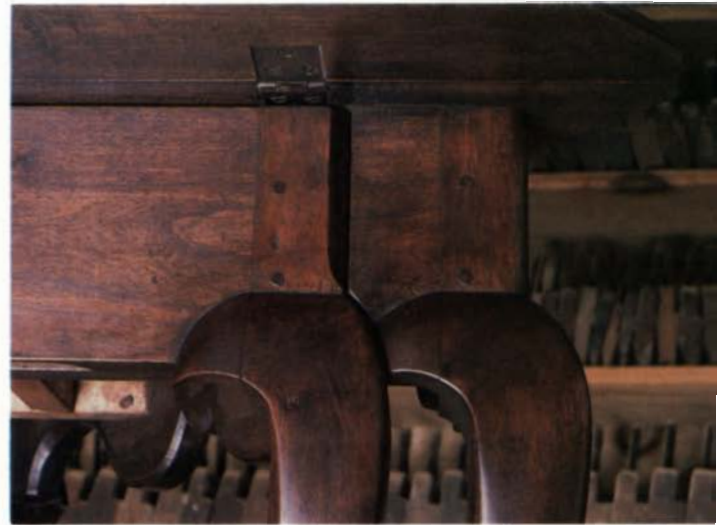
A look at the table's back corner (left) shows how the knee and post have been shaped to conform to the 45° angle. The hinged back leg nests as shown at right; note in the drawing on the facing page that both legs are oriented in the same direction. Below, Landon demonstrates the setup for starting an angled mortise. He supports the corner post in a V-block, and presses the leg against his forearm for extra control. Paring the tenon's angled shoulders is shown at right below. The first step is to bandsaw close to scribed layout lines. Then finish up with a chisel and a 45° guide block.
