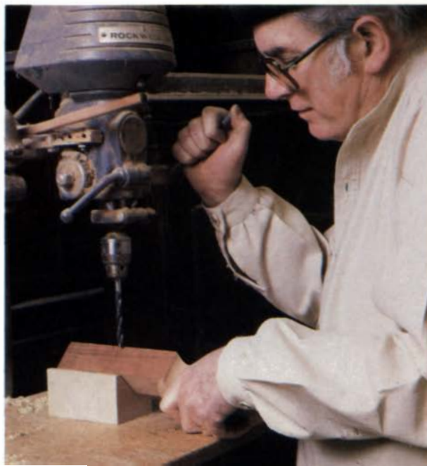
A look at the table's back corner (left) shows how the knee and post have been shaped to conform to the 45° angle. The hinged back leg nests as shown at right; note in the drawing on the facing page that both legs are oriented in the same direction. Below, Landon demonstrates the setup for starting an angled mortise. He supports the corner post in a V-block, and presses the leg against his forearm for extra control. Paring the tenon's angled shoulders is shown at right below. The first step is to bandsaw close to scribed layout lines. Then finish up with a chisel and a 45° guide block.
