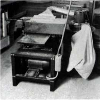
Four-inch metal duct, a 30-gal. drum and blower service Harrison's planer (above and left). The metal nozzle is extended under the planer's cover with ¼-in. plywood. A powerful vacuum cleaner collects from the two nozzles attached to the radial-arm saw's blade guard (below). An inner tube suspends the flexible hose from the ceiling, permitting the saw to travel easily.
