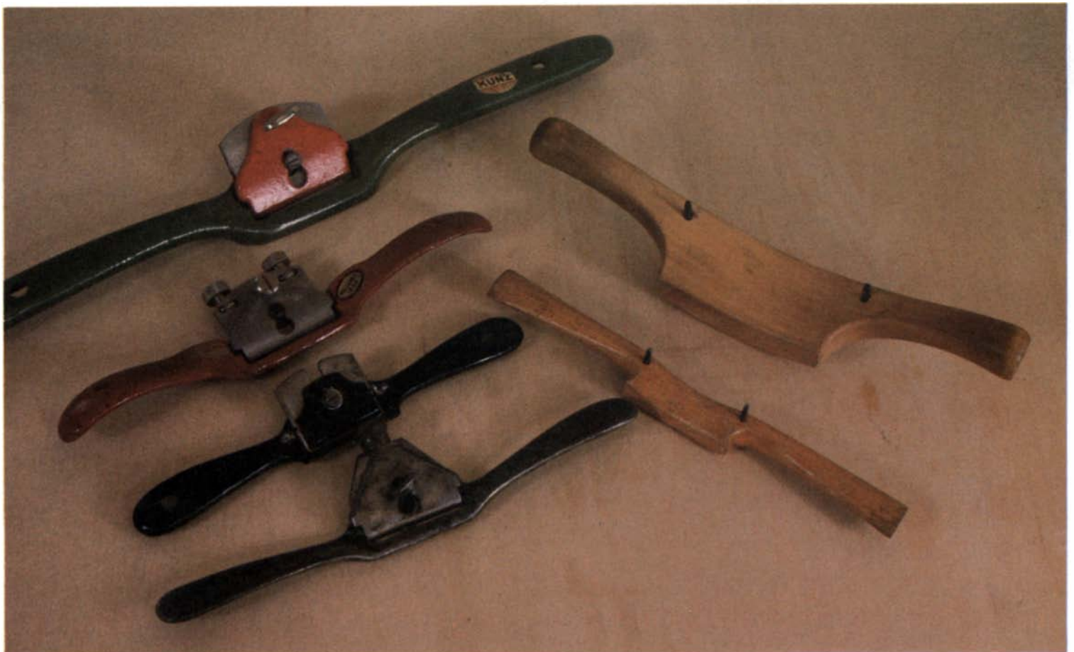
for shaping chair seats; cooper's spokeshave; flat-soled metal with dual screw adjusters; author's favorite 9-in. Kunz (painted black); metal shave with single adjuster.
