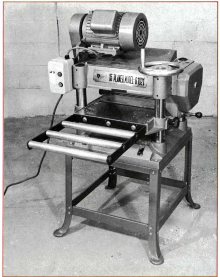
The Grizzly as shown weighs in at 480 lb.—the heaviest of all the small planers. Extension bed rollers are standard equipment, front and back. The table moves up and down on the four steel columns. Base, table and cutterhead assembly are cast iron.
