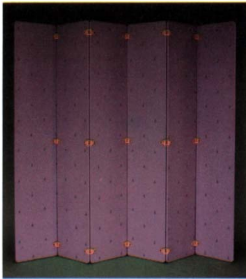
A lighter screen with plywood panels called for a new hinge, so Mackintosh designed a knuckle hinge that pivots on dowels (drawing at right). Maple knuckles are let into mortises routed in the panels, then fastened with anodized aluminum interscrews.
