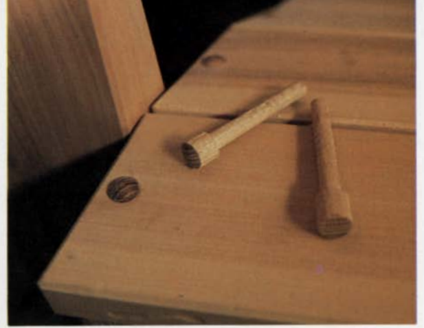
Old Adirondack chairs were fastened with rust-prone nails, a shortcoming the authors improved with mechanically sound joints and shipbuilders' trenails.
