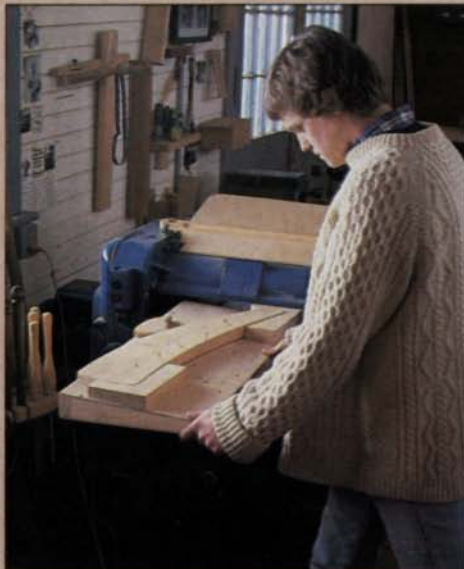
By tapering its arms and legs, the authors gave their Adirondack a lighter, more refined personality, while leaving enough wood for strong joints. Above, Parsons feeds the arm-tapering jig through the planer. The arm is tapered in three passes by raising the bed after each cut.
