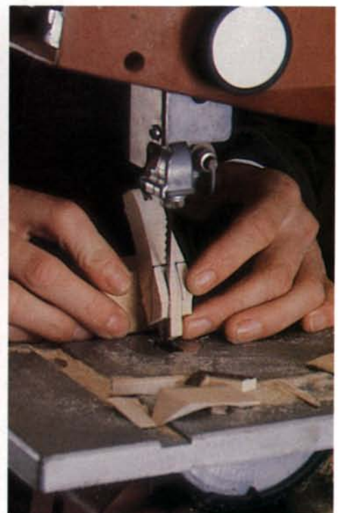
Steady the cone-shaped hip section with a scrap wedge while bandsawing the notches that accept the thighs, above left. Hold the leg piece on end and bandsaw parallel cuts to establish ¼-in. tenons, above right. Carve the shoulders with a knife.
