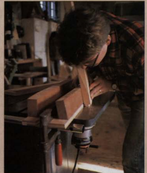
The authors' tablesaw doubles as router table, and the fence shown also does double duty. Above, Beeken uses one side of it to mill an angled dovetail pin for the chair's front-leg-to-arm joint. By reversing the fence, he can rout the straight pin for the lower back.
