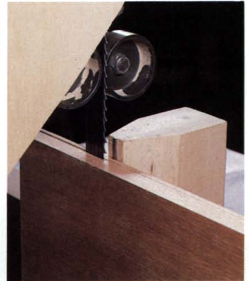
With the trailing edge of the fence positioned \frac{1}{8} in. in front of the blade, begin the cut by pressing the board against the fence just ahead of the blade. Follow the marking-gauge line (pencil-darkened for clarity) by pivoting the board on the fence.
