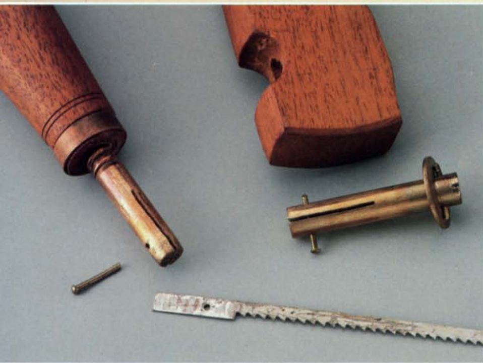
The saw's blade holders are made from bronze lag bolts. One is screwed into the handle and its head ground off; the other is sawn from the bolt's shank. Hacksawn slots accept the blade, and pins or cotter pins inserted through holes drilled perpendicular to the slots hold it fast.
