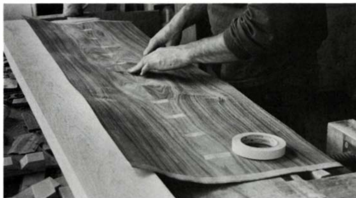
After joining the veneers with masking tape, March flips the sheet over and props a plank under one leaf to pinch the veneer seam tight. The seam is then secured with veneer tape before the masking tape is pulled off.
