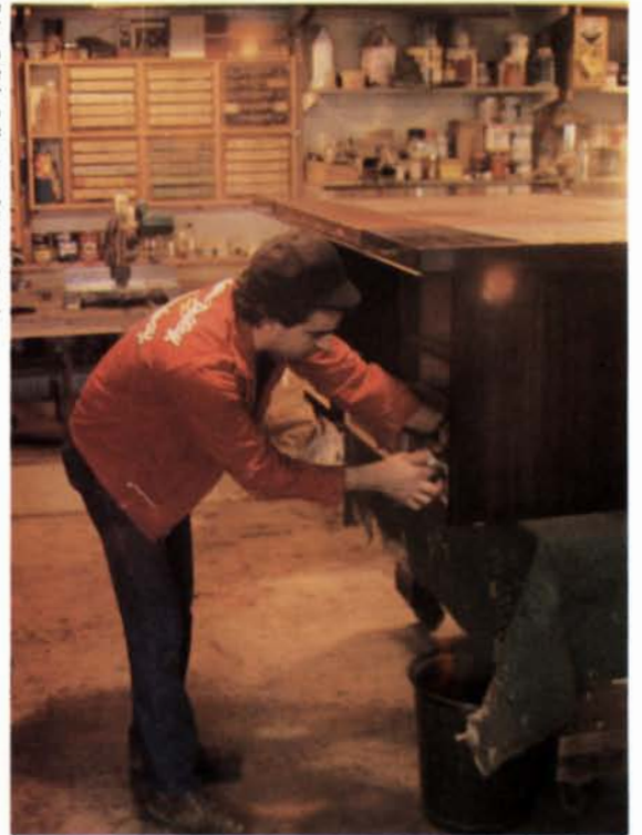
Nick Monjardo prepares a late Rublmann desk for polishing after the last coat of finish has cured.
