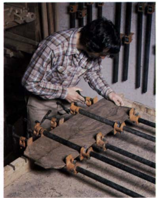
Thick veneers are stiff enough to be glued up just like boards. Flush up the show surfaces, and alternate clamps top and bottom so the leaves won't buckle.
