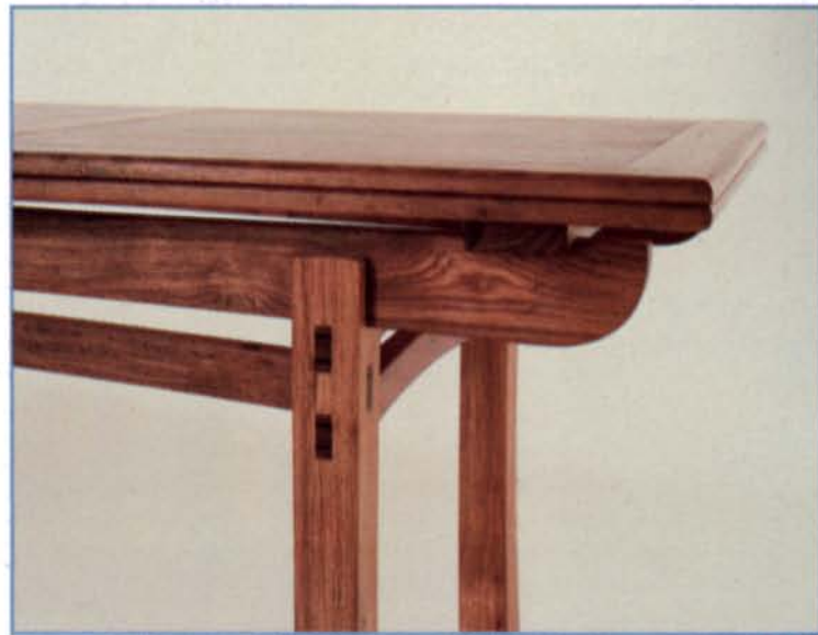
Ebony wedges accent the exposed mortise-and-tenon joints where the rosewood legs intersect with the front and back stretchers and the dual side stretchers. A bridle notch carries the top stretcher out to braces under the double-leaf top.
