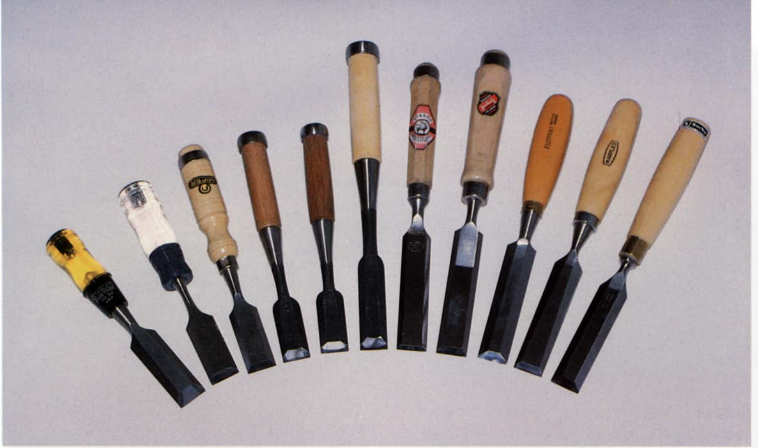
The test chisels had a wide range of handle styles and blade lengths—both important factors to consider when selecting a chisel. From left: Stanley, Craftsman, Mifer, Sentora, Oiichi, Iyoro, Hirsch, Spannsage, Footprint, Marples and Sorby.
