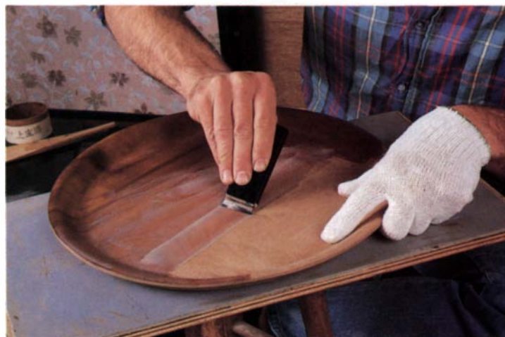
Apply the urushi with a short-bristled brush. The first, soaking coat creates a dramatic color contrast between the raw wood and the finished area. The glove keeps oily fingerprints off the wood.
