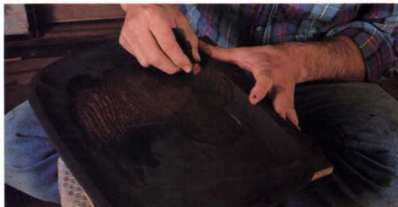
Removing hardened stone paste is tedious. Wet-sand the layer to create a mud-like slurry, above, then wipe the area with a wet cloth. Wood grain is visible through the semi-transparent areas. Sandpaper is too rough for final coats, which must be polished with powdered charcoal dust and a cloth wrapped around a cotton pad, right. The polishing motion resembles that associated with French polishing.
