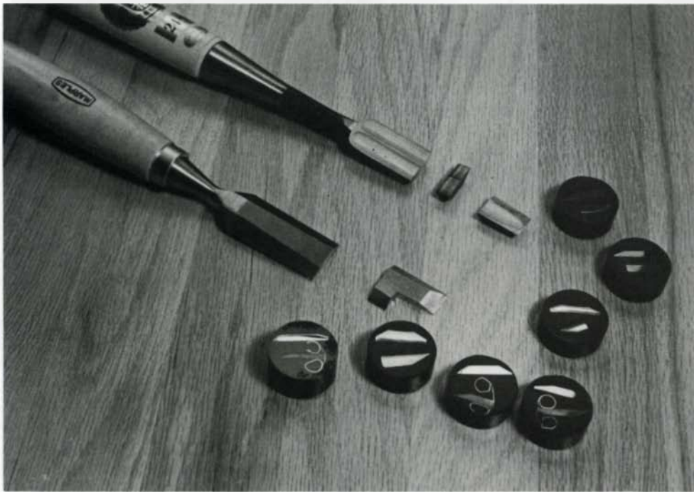
To measure hardness, two slices from each chisel were cast in plastic and polished, then they were mounted on the Tukon tester (above right), which calculates hardness by measuring the penetration of a diamond stylus.
