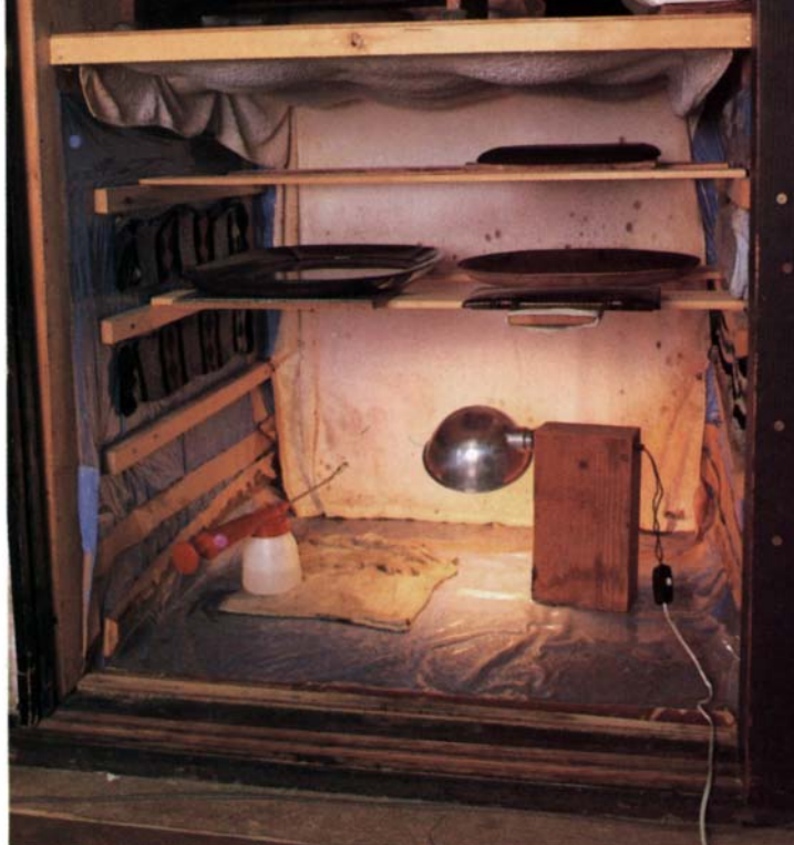
This typical wet box, shown with its door removed, is a rough container equipped with a wet/dry thermometer to monitor humidity and temperature. Towels dampened with a plant sprayer provide moisture. Lamps supply heat when the box is sealed.
