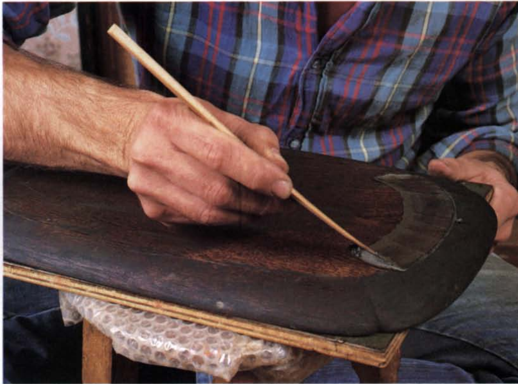
Holding one end of a nylon cloth filled with stone paste in his teeth, Roche twists the other end with one hand and uses the hera to pick up the paste as it is filtered through the cloth. Then he uses the spatula, right, to smear stone-paste filler over the wood and into its open pores.
