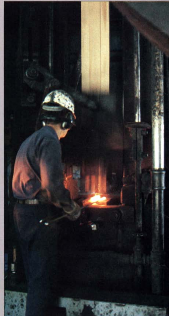
At Buck Bros., chisels are drop-forged in two-part dies. The monstrous drop hammer above slams the die halves together with a force of 1600 lb., squeezing the hot plastic steel between them. Two quick blows forge a chisel.
