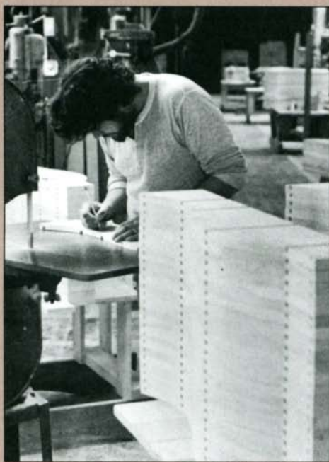
Careful sanding removes \frac{1}{64} in. to bring each piece to final dimension.
