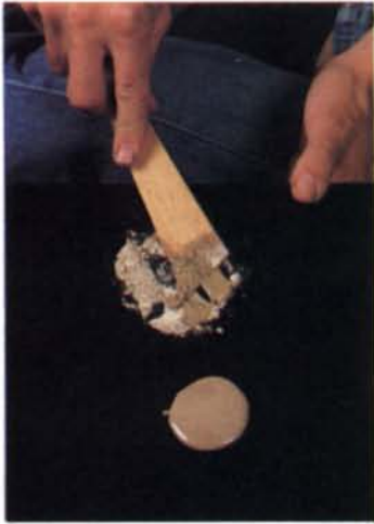
To make a wood filler, use a hera (wooden spatula) to mix pulverized stone powder with water, then work in a small amount of lacquer until the paste can be smeared easily.
