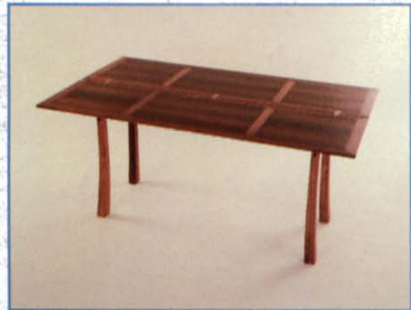
March's table folds open from 18 in. to 36 in. Sliding brackets allow the top—a Honduras rosewood frame holding panels veneered with lighter-colored Santos palisander rosewood—to be centered over its base in both the closed (right) and open positions (above).
