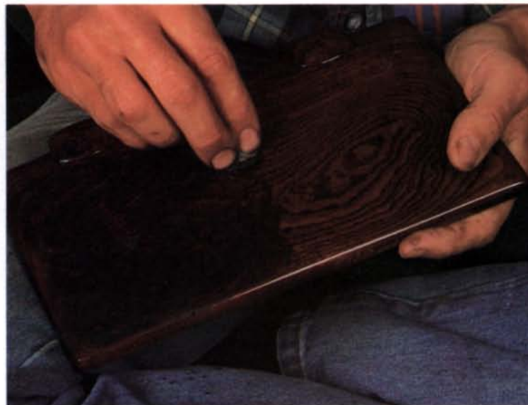
Removing hardened stone paste is tedious. Wet-sand the layer to create a mud-like slurry, above, then wipe the area with a wet cloth. Wood grain is visible through the semi-transparent areas. Sandpaper is too rough for final coats, which must be polished with powdered charcoal dust and a cloth wrapped around a cotton pad, right. The polishing motion resembles that associated with French polishing.
