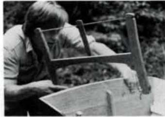
The bowsaw is excellent for joint-cutting or cutoff work. See p. 52 for plans. Photo: Simon Watts.
