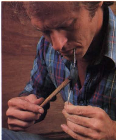
Holding one end of a nylon cloth filled with stone paste in his teeth, Roche twists the other end with one hand and uses the hera to pick up the paste as it is filtered through the cloth. Then he uses the spatula, right, to smear stone-paste filler over the wood and into its open pores.
