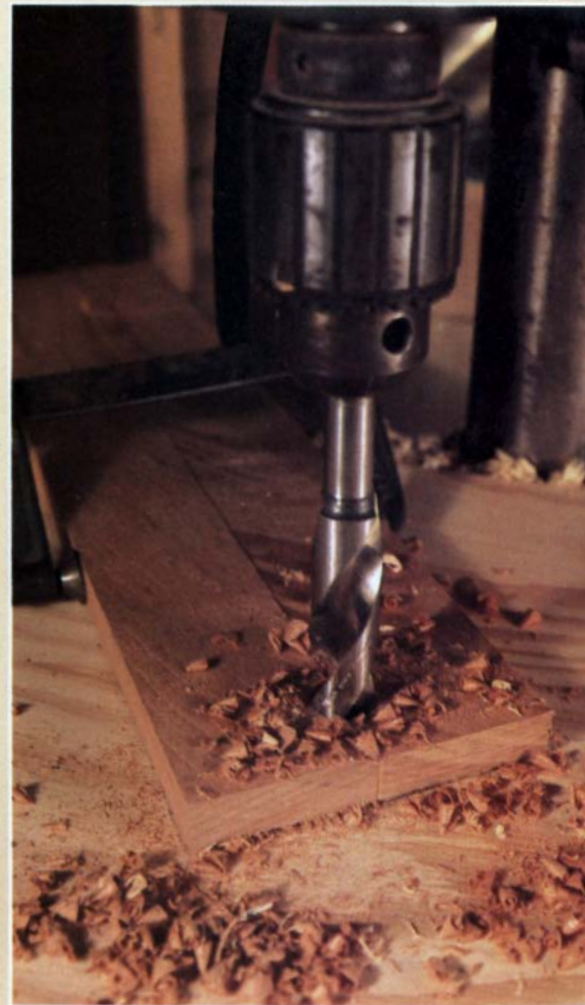
To bore notches for the blade holders and tensioning cord, clamp the uprights together and center the bit line between the parts.
