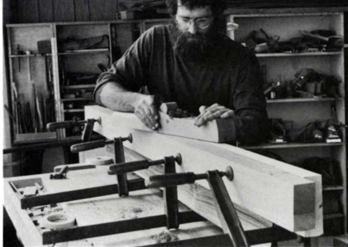
With the veneer sheets clamped between boards so that the matched edges stand proud, March hand-planes the edges.
