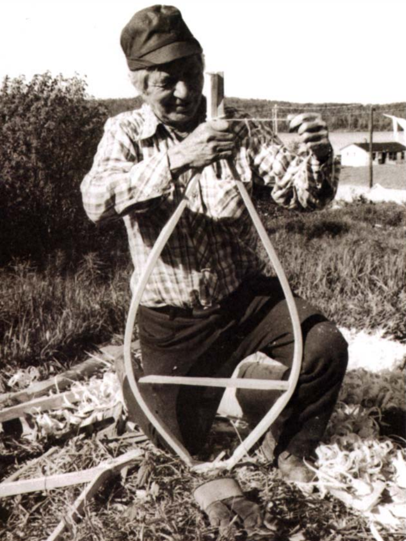
A temporary horizontal spreader establishes the characteristic snowshoe shape as the ends of the staves are pulled together. Twine holds the tails together until the green frame has dried.
