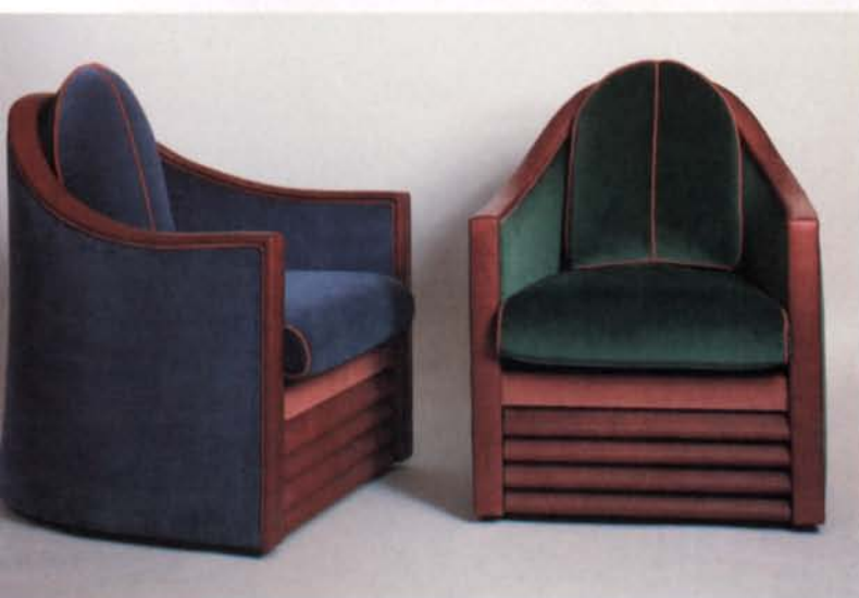
In Jack Larimore's chair, poplar verticals connect a plywood platform on the floor to a laminated-in-place plywood rail/arm. Upholstery is burlap, thin foam, wool mohair and leather.
