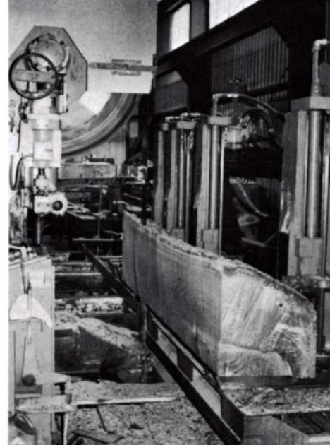
A large bandmill can handle bigger logs than can a circular sawmill. Even so, the buttress of this 46-in. dia. log had to be trimmed with a chainsaw to fit.
