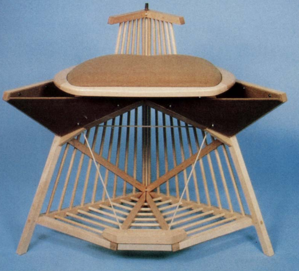
Maple dowels are the main structural components in this weavers' bench. The triangular compartments on each side of the 31-in. high seat are for yarn and tools.
