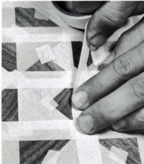
The patchwork marquetry tray/table shown at left features the traditional 'Ohio Star' quilt pattern in oak, mahogany and birch veneers. To reinforce the show side of a marquetry sheet, tape along the seams of the triangles (above). Overlap the border strips at the corners to miter the veneer border (right). With a razor-sharp X-acto knife guided against a steel rule, cut through both strips at once.
