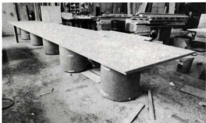
Though sophisticated machines and jigs ensure consistent results, there's a place for handwork in the mill shop. The radiused corner moldings of the conference table shown at left were hand-turned (above) to match the profile of the machine-cut straight moldings. In the photo below, the disc has been bandsawn into quadrants which will neatly connect the straight moldings.
