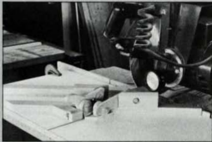
Radial-arm saw jig (above and in drawing below) produces triangles in quantity.
