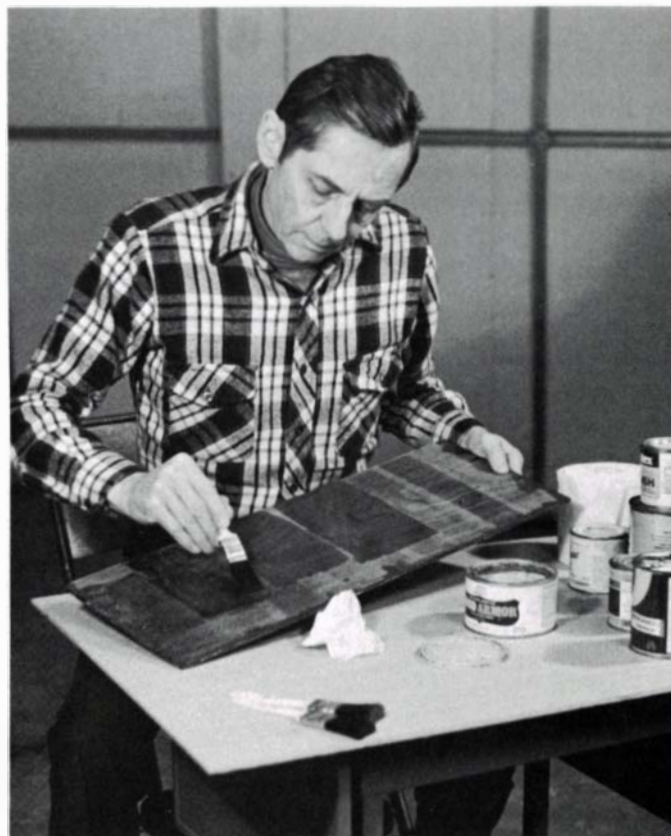
Each brand of water-based varnish tested had its own brushing characteristics. Some were watery, others were much like regular varnish. Brushing all five brands on the same board allowed Newell to compare the quality of the films side-by-side.
