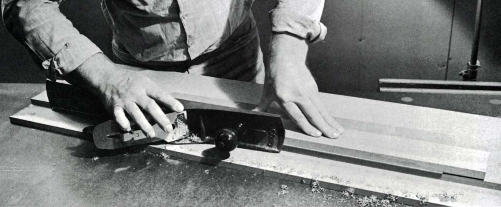
For butt joints, the sheets of veneer must be straight-edged. Hold the veneers in place on the shooting board while truing the edges with a jointer plane.
