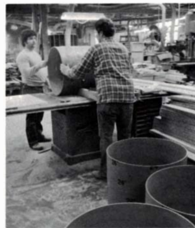
Cover: Millworker Herman Unger veneers a conference-table pedestal for a high-rise refit. Above, cardboard concrete forms serve as pedestal cores. For more on millwork, see p. 30. Photos: Jeff O'Hearn.
