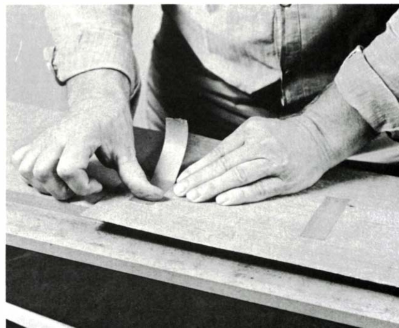
To temporarily join veneers into sheets, stretch pieces of veneer tape across the seams on the face side. The tape keeps the veneers from moving around in the press.
