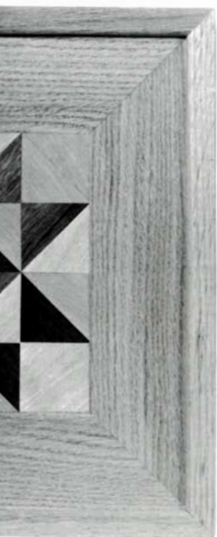
The patchwork marquetry tray/table shown at left features the traditional 'Ohio Star' quilt pattern in oak, mahogany and birch veneers. To reinforce the show side of a marquetry sheet, tape along the seams of the triangles (above). Overlap the border strips at the corners to miter the veneer border (right). With a razor-sharp X-acto knife guided against a steel rule, cut through both strips at once.
