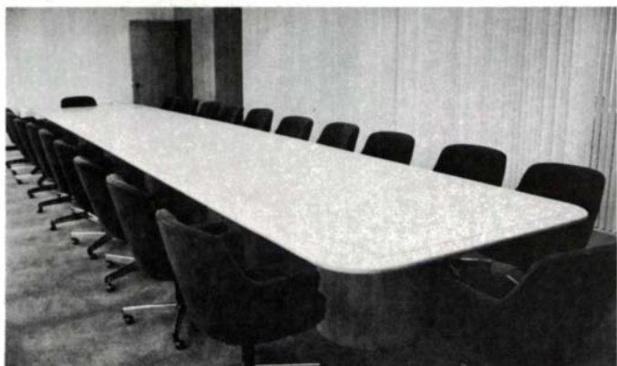
As the height and rent of a commercial building rise, so too do the scale and cost of the furniture that goes inside. The 26-ft. long conference table shown above is particleboard veneered with white ash burl. Too large and heavy to fit in the building's elevators, the table was made in five sections, then assembled on-site with Lamello plates and knockdown fasteners (photo, left). The pedestal legs are oak-veneered cardboard Sonotubes.
