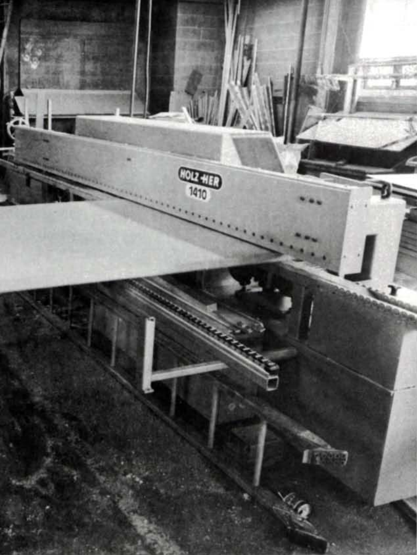
Millworkers get out enormous quantities of work on time by relying on big, expensive machines. In the photo at left, cabinetmaker Herman Unger feeds particleboard through an edgebander, which glues on a solid-wood edge strip before the panel faces are veneered. Below, two veneer leaves are fed through a stitcher, which sews them together with a thread of hot-melt glue.
