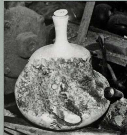
Osolnik turns a rhododendron-burl weed pot between centers with a roundnose chisel (left). The nearly finished pot is shown above. The hole in the neck is bored after turning.
