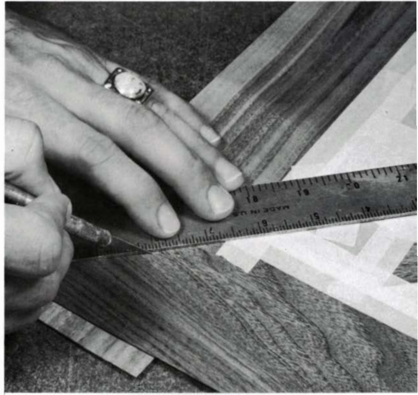
The patchwork marquetry tray/table shown at left features the traditional 'Ohio Star' quilt pattern in oak, mahogany and birch veneers. To reinforce the show side of a marquetry sheet, tape along the seams of the triangles (above). Overlap the border strips at the corners to miter the veneer border (right). With a razor-sharp X-acto knife guided against a steel rule, cut through both strips at once.
