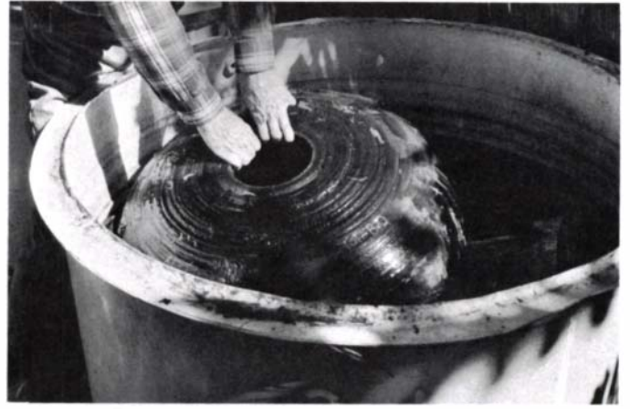
D. Several months in a solution of PEG stabilizes the wood.
