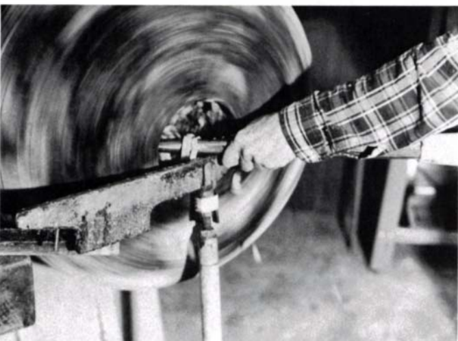
C. Undercutting the inside.
