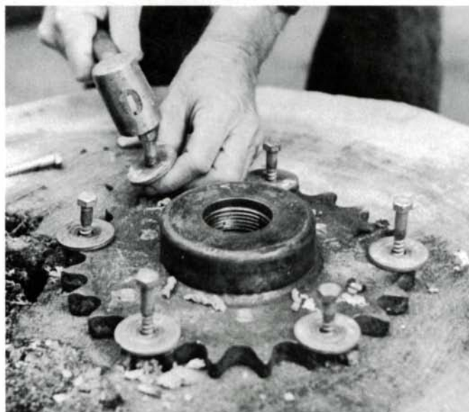
Attaching the faceplate with lag bolts.
