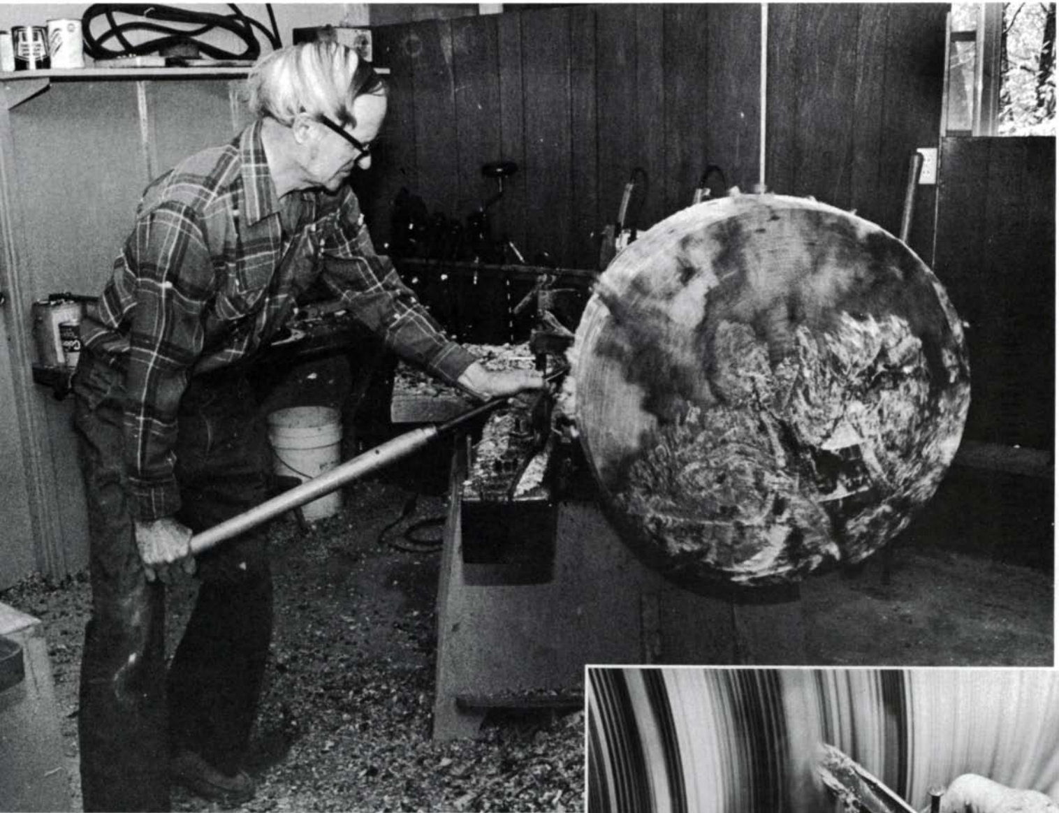
First cuts with the lance braced on the thigh.
