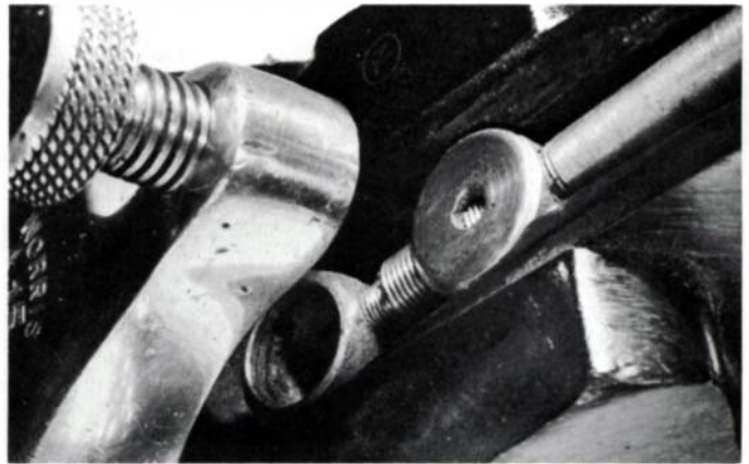
The Norris adjuster mechanism consists of a steel eyelet with an attached rod threaded into the adjuster shaft. The eyelet engages the cap-iron screw to raise or lower the iron. To align the cutting edge, the shaft pivots on a cylindrical knuckle.
