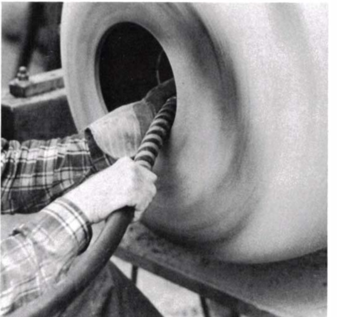
F. The flexible shaft also reaches the inside of the bowl.
