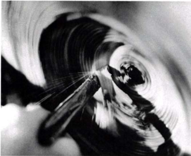
B. The hook begins hollowing the bowl.
