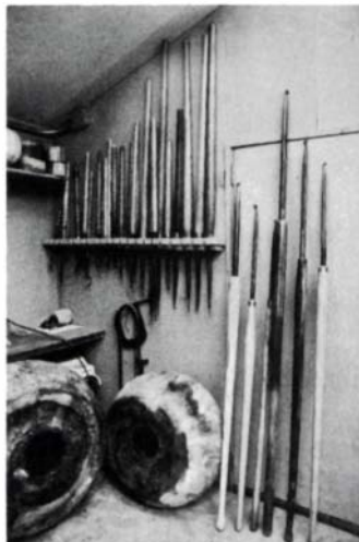
Moulthrop's tools include hooks and lances up to 96 in. long.
