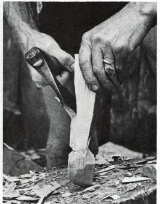
Making a spoon begins with a green crook that you split at the pith using the ax, driven by a maul, as a wedge (above). The top and bottom of the spoon are shaped first (above right), then the sides (right). Careful, measured strokes, always aimed below the hand that holds the blank, define the basic shape.
