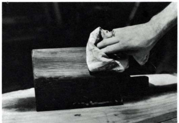
When the surface is evenly wiped, some carbon particles remain as a coloring agent, and will be sealed in by top coats of polyurethane. Under the finish, the wood continues to age naturally.
