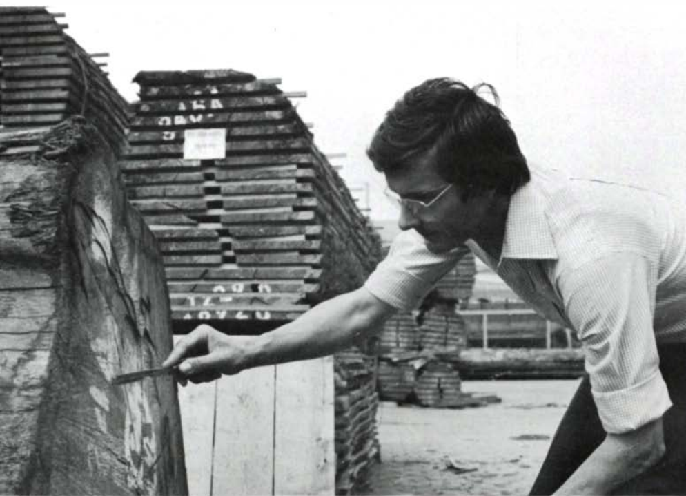
Peter Wiese, above, uses a timber gouge to inspect a bubinga log. Scooping into the log's end grain reveals the wood's color and texture. Behind him is lumber 'sawn in the boule.' Wood is more commonly sawn in this manner in Europe and is stacked in the order it comes from the log, thus preserving the relationship of color and figure from board to board. Theodor Nagel & Co. is a principal supplier of musical instrument woods and provides its customers with custom-sized blanks and billets. At right, a worker dips the end grain of billets in wax to guard against checking during drying and shipping.
