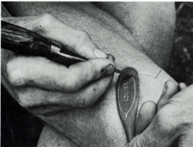
Gift spoons warrant decoration. Sundqvist first pencils in the shapes and letters, then uses the tip of the knife locked at about 60° to the surface, first in one direction, then the other, to remove a triangular chip of whatever length.
