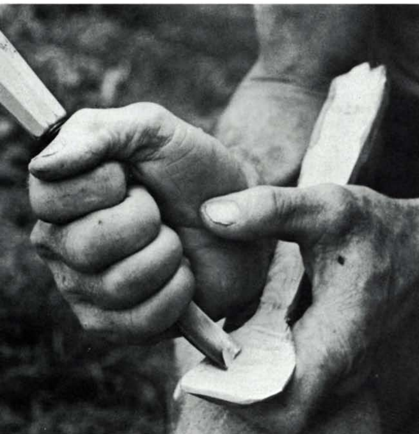
Most of us pare by slicing from the stout end of a knife toward the tip. Sundqvist gets greater power arcing the blade from tip to handle, often using his thumb for leverage. Each stroke has its safety. Above, the thumb is held out of the knife's direction on the spoon end. At right, Sundqvist modifies this stroke to slim the middle of the spoon's handle by repositioning the thumb 90° to the stroke and rotating the knife in the palm about 30° toward the blank. Short, arced strokes stop before the thumb is touched.
