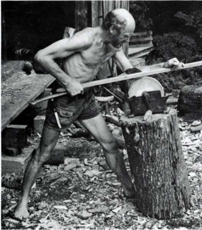
Sundqvist demonstrates the grip and stance for grinding an ax. The backing board helps to maintain even pressure on the ax head as it is run diagonally over the grindstone.
