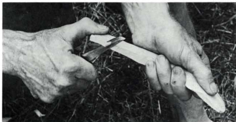
Most of us pare by slicing from the stout end of a knife toward the tip. Sundqvist gets greater power arcing the blade from tip to handle, often using his thumb for leverage. Each stroke has its safety. Above, the thumb is held out of the knife's direction on the spoon end. At right, Sundqvist modifies this stroke to slim the middle of the spoon's handle by repositioning the thumb 90° to the stroke and rotating the knife in the palm about 30° toward the blank. Short, arced strokes stop before the thumb is touched.
