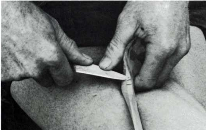
These two strokes are both powered by the hand not holding the knife. They show how Sundqvist uses the whole length of the blade: the stout portion for heavy cuts, the tip for fine work. At top is the still-green blank. Wet wood is easier to shape, but to smooth the surface, the spoon is first dried overnight. Dry wood, above, frays less.
