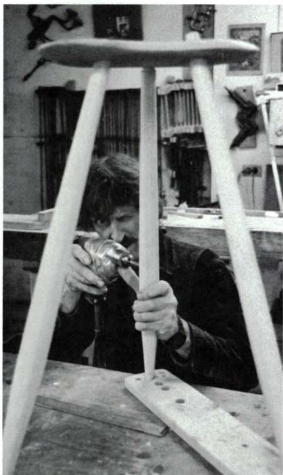
Ron Curtis eyeballs a mortise as his foot jig steadies the work, left. The stool has an elm top and legs, and is about to be fitted with ash rungs. Curtis prefers native woods and will go out of his way to get them, but admits, 'I usually cut up some South American stuff for the wedges.'
