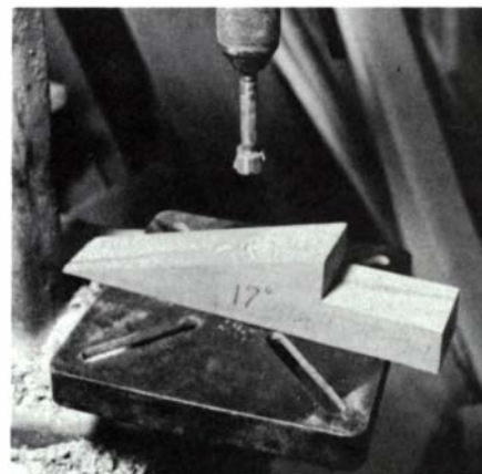
Instead of tilting the table, Curtis uses this angled block. He sets the seat blank on it when he drills the holes for the legs.
