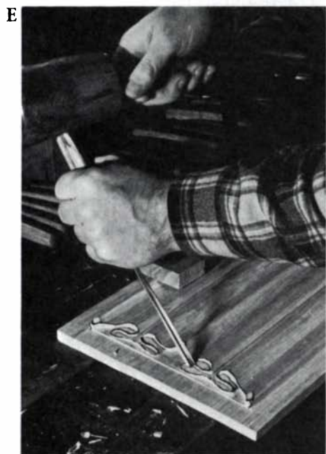
Outline the edges with a V-tool, cutting with the grain as much as possible.
