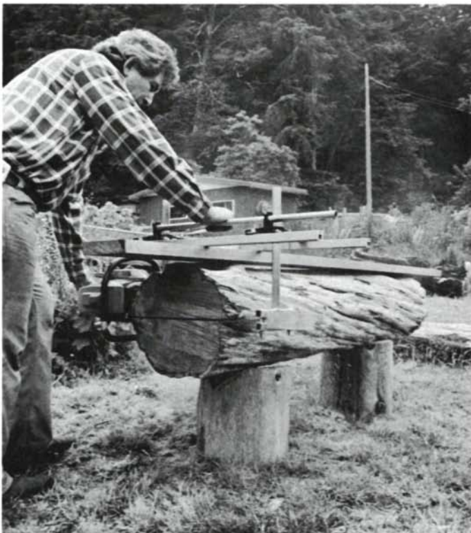
Minimum milling: a chainsaw mill, a plank to guide the first cut, and a few nails to hold the plank on the log. Malloff, a chainsaw logger by profession, has improved every aspect of this setup, developing the rig shown on the following pages.
