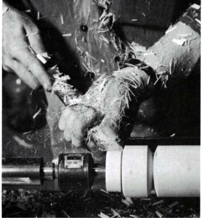
The skew can quickly remove waste. Keep the bevel rubbing, and the edge moving forward, as the diameter goes down. A firm grip is necessary.
