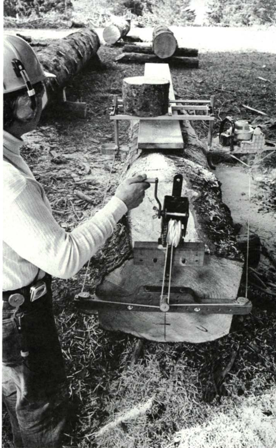
A yoke, fastened just below the line of cut, keeps the cut straight as Malloff cranks the winch, above. One rope is attached to the modified Granberg mill; the other rope is connected, by means of an adjustable bridle rope, to the saw itself and to a lever that controls its throttle. The mill, with its log-section counterweight, will be pulled to the end of the guide plank. Then the plank will be slid forward on the supporting lag bolts until it rests on the end board. The winch is attached to the plank itself, and the cut continues. Subsequent cuts don't require the plank and lags because the mill can ride directly on the flat-cut surface of the log. At left, with steel end dogs in place to control twisting, milling is well under way.
