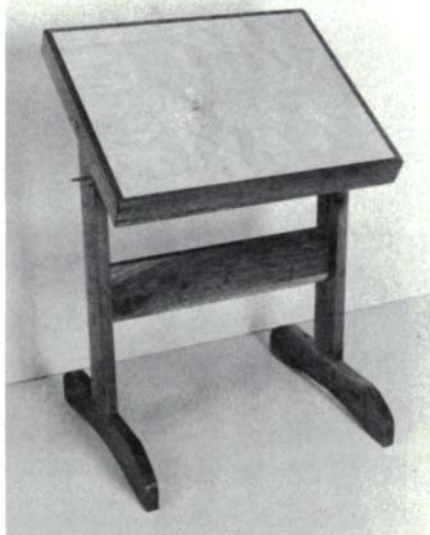
'The drafting table is walnut and cherry, with a 3/4-in. birch plywood drawing surface. The top has a hinged bottom that swings down to allow for paper storage.' —Ben Erickson, Eutaw, Ala.
