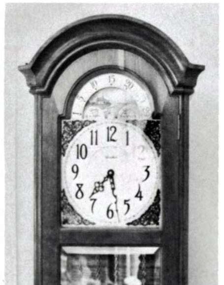
This is the radiused molding on one of the twelve clocks Haserodt made for his grandchildren. The molding is returned along the sides of the case.
