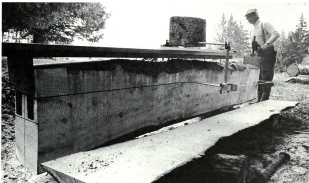
Careful layout is the route to precision milling. Above, Malloff checks the height of the lag bolts that will support the guide plank. The end boards have been carefully aligned with vertical and horizontal layout lines drawn on both ends of the log. In this case, he's milling directly through the heart center of the log. If the heart were off center, he might mill to the average center instead.
