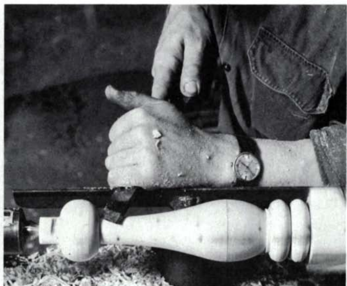
The planing cut, with the bevel rubbing the work to support the cutting edge, leaves a smooth, polished surface. Darlow guides the skew with his thumb while his left hand dampens vibration in slender stock, above. Generally, as shown at top right, neither the short point nor the long point should contact the work. The bottom right photo shows a modification: the slide cut, a planing cut that gradually leads up to using the extreme short point to cut the end of a curve without marring the side of a bead. As in all turning where most of the tool movement is horizontal, the conventional overhand grip is used.
