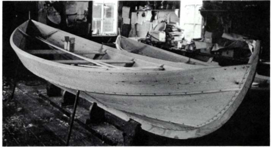
Norse boatbuilding survives yet today. The Oselver boat, above, built by Alfred Sovik, is a descendent of early Viking lapstrake craft discovered in ancient burial mounds.
