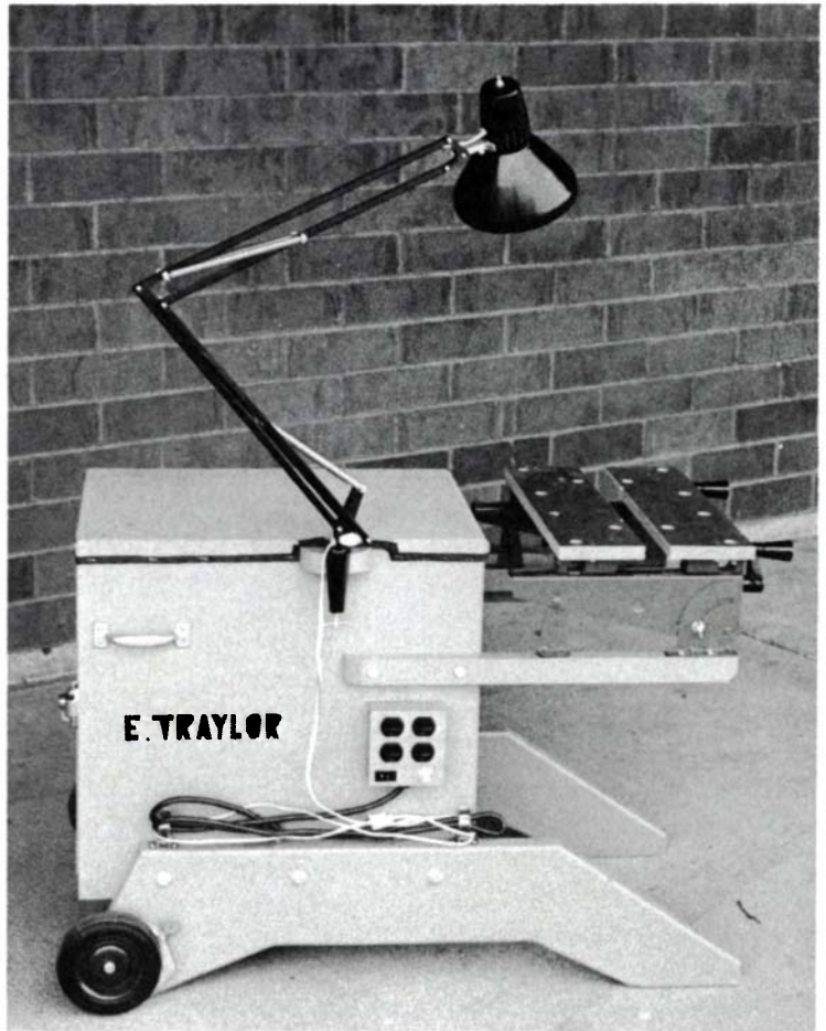
Traylor's portable carving bench has a work hold-down, storage space, a lamp and electrical outlets. Wheels, pirated from an old lawn mower, retract to keep the bench from rolling around when in use. Traylor added a drawer to the storage compartment and made the tool tray removable. The top is covered with tough corduroy to protect work from being marred.
