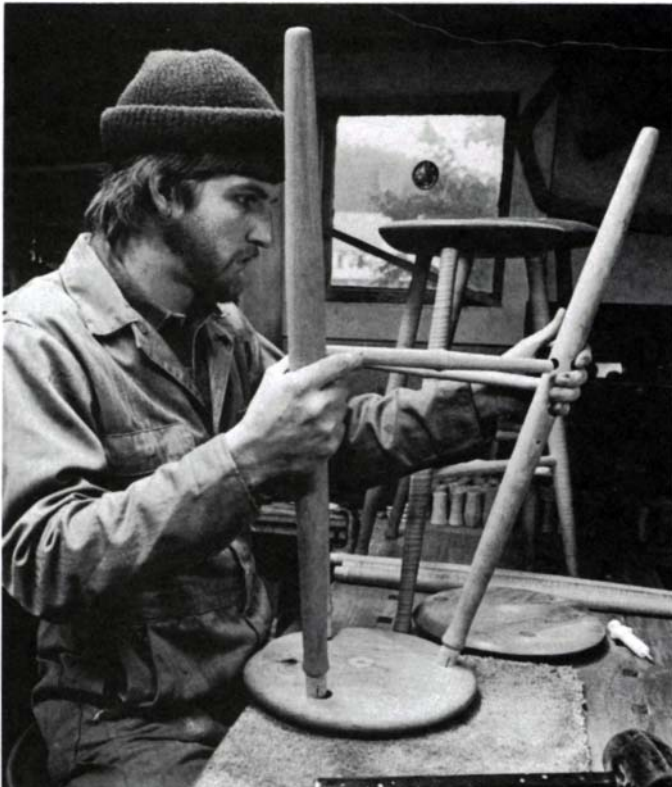
When easing a stool together dry, Scott makes sure the joints all draw up at the same time, or the last pieces will be difficult to get into place.
