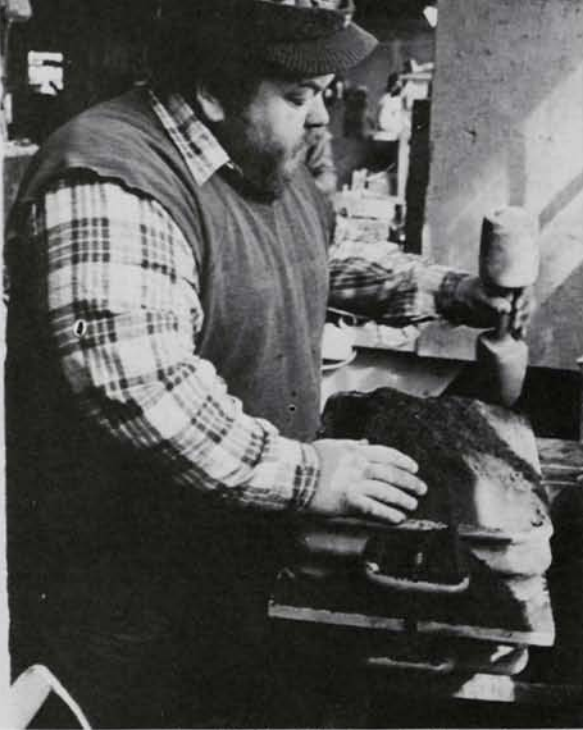
Sand-casting is slow, highly skilled work. Above, foundryman Joe Bossio of Franklin Alloys tamps sand around a pattern which will then be removed to form a cavity shaped like the hardware to be made. At the Horton Brasses foundry, right, co-owner Jim Horton and an assistant pour brass into a gate, an opening in the mold. Too much moisture in the mold can cause the hot brass to geyser back out of the gate, an occupational hazard of foundry work.
