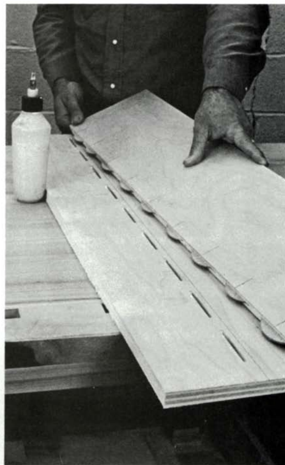
To cut slots with the Elu, above left, the cutter index is aligned with each pencil mark and the motor-cutter assembly is pivoted, plunging the blade into the stock. The edge of the mating board acts as a fence and must not be moved during the plunge, or an oversize slot will result. Slots in the mating part are cut by repositioning the machine, left. Above, glue has been squirted into the slots, and the beech plates inserted. The metering nozzle and glue bottle sold by Lamello are on the bench. Now the joint is assembled and pulled up tight with clamps, screws or nails. Clamps can be removed in as little as 10 minutes, because the plates swell, locking the joint.
