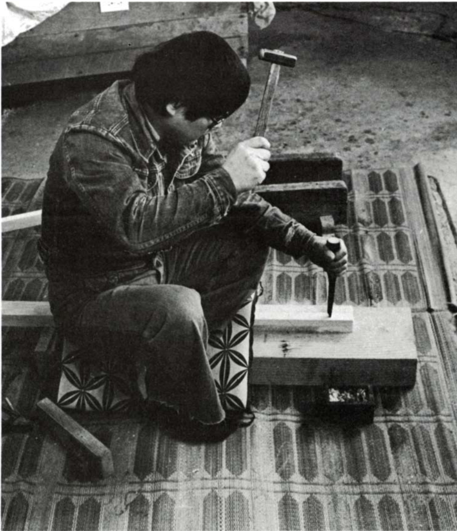
The tategu-shi sits on the wood to steady it while he mortises it, above, stabbing his chisel frequently in a box of cotton wadding soaked with vegetable oil, to reduce friction. The chisel has three concave sides and a hollow-ground face (figure 9 and photo, top of facing page). He chops from the middle out, always with the face toward the middle of the mortise, except for the final cuts at either end of the mortise. These are angled slightly from the perpendicular (photo, right, includes a square for illustration only) to taper the mortise for a tight fit when the tenon is driven in.
