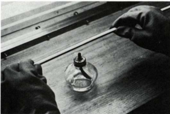
Heat from an alcohol lamp softens the bamboo fibers and allows rod straightening. Keep the rod moving to avoid scorching it.
