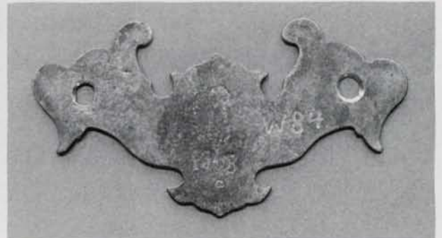
A close look will reveal the difference between cast and stamped parts. The Chippendale pull, above left, is all cast—backplate, bail and loose posts. The pull, above right, is a thin stamping with its edges bent down to create the illusion of thickness. The bail is of bent brass wire, and instead of loose posts the pull is attached to the drawer with studs fastened to the backplate. The assortment of knobs, bails and escutcheons, left, has just come from the sand mold. Even after polishing, you can recognize them as castings by the slight irregularities and traces of the flash lines where the two parts of the mold met. Below, backplate cast in a sand mold is recognizable by the pitting and unevenness on the back side. The front will be polished smooth. This plate has an identification number cast into it at lower right.
