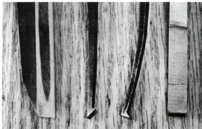
The tategu-shi's mortising tools. From left to right, a mortising chisel, with hollow-ground face (ura); a mori-nomi, whose harpoon-like hook is tapped down and jerked up to remove chips; and a sokozarai-nomi, which scrapes the mortise bottom flat and also lifts out chips. Last is a steel rod for tapping flat the bottoms of small mortises.
