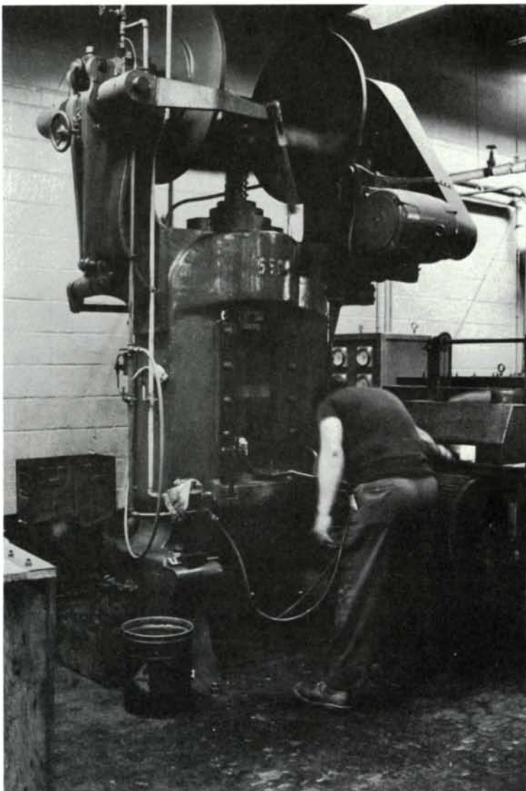
Baldwin Hardware Manufacturing Corp. uses four of these English-made power forges, above. At right is a lower die into which a hot brass rod will be placed. When the upper die slams down, a new piece of hardware is instantly formed, needing only edge-trimming and a shine. Forged parts can be made with fair detail, but each one is identical to the next.
