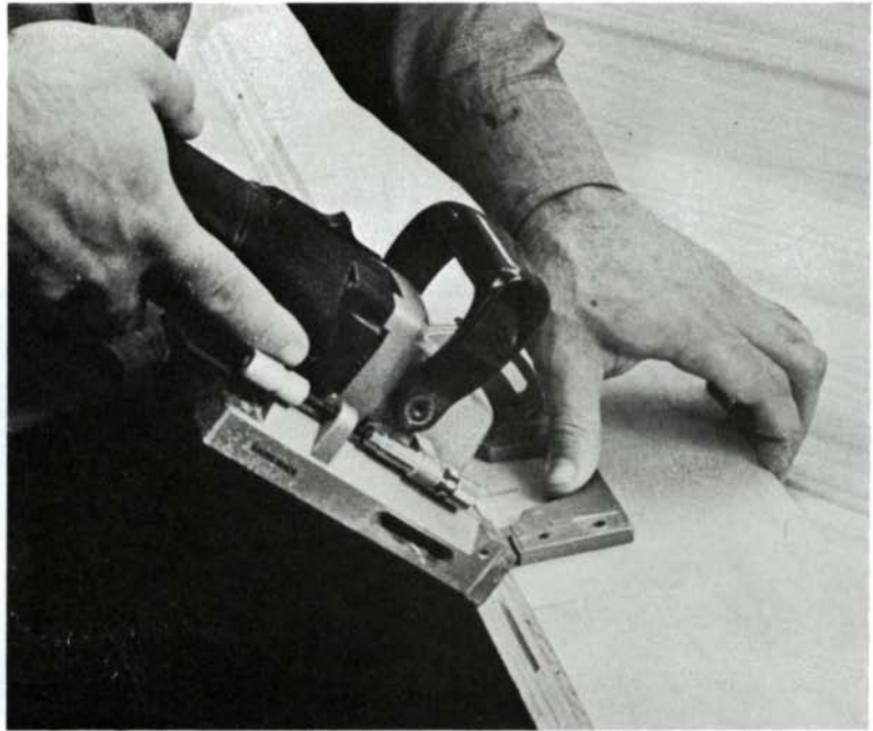
The Minilo's front fence can be set at 45°, making it the better machine for slotting lengthwise miters. Spring-loaded pins in the machine's front guard lock the Minilo against sliding during the plunge, a feature lacking in the Elu.
