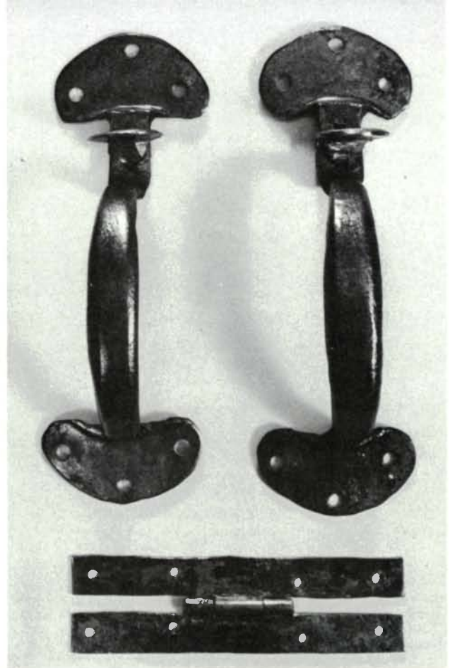
The basic tools of the blacksmith—fire, hammer and anvil—have remained unchanged for hundreds of years, and the smith's products are similar to those made by his colonial forebears. Wrought thumb-latches and H-hinge by Woodbury Blacksmith and Forge Co., right, show the distinctively varied profiles left by the process—no two are identical, and the marks left by the smith's hammer and anvil are evident.
