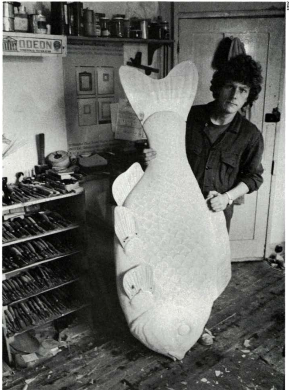
Raybould's tiny workroom is well-stocked with carving tools. The fish, about ready for painting, is made of jelutong, one of the soft, easily workable woods that Raybould prefers.
