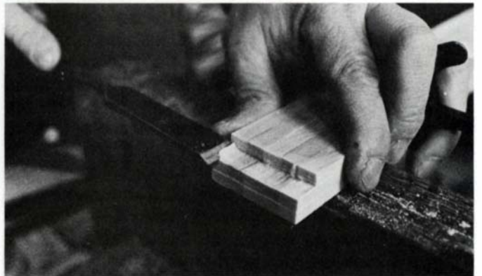
With the kumiko still clamped together, Odate makes their tenons. First he saws the shoulders, then breaks off the waste with a chisel pushed in from the end grain (top). The index finger on the bottom of the chisel acts as a stop to protect the shoulder. He cleans up the tenons by paring with the chisel across the grain (above). When all the tenons have been formed and their top and bottom corners chamfered with a few strokes of a plane, he unclamps the stack, fans out the kumiko and chamfers the other two corners (below).
