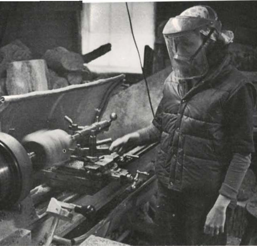
Chuckling up odd-shaped pieces, Holzapfel rounds them off as quickly as most turners would with hand tools. Standing to the side, above, keeps her out of the path of flying chips. Rounding off at low speeds, she runs the lathe slowly and since it's bolted to the floor, vibration is minimal.
