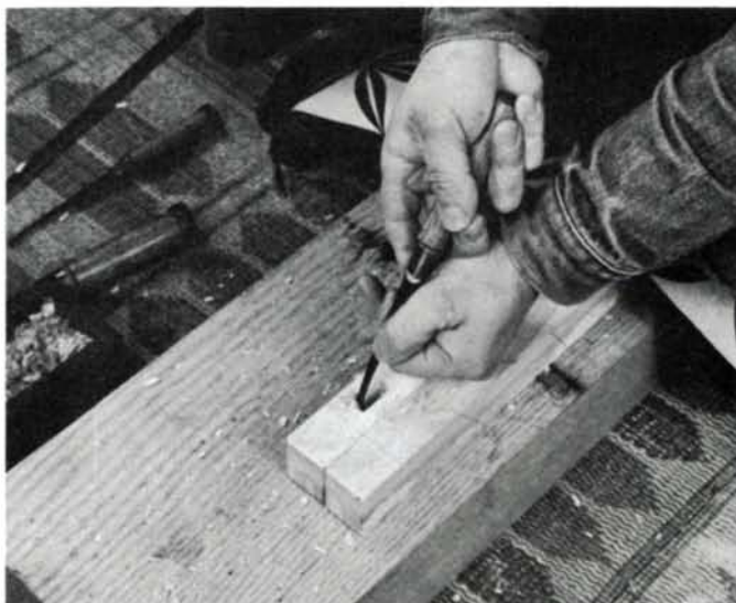
Scraping the bottom of the mortises with the sokozarai-nomi.
