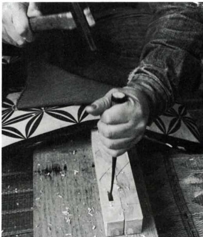
Removing chips with the mori-nomi.
