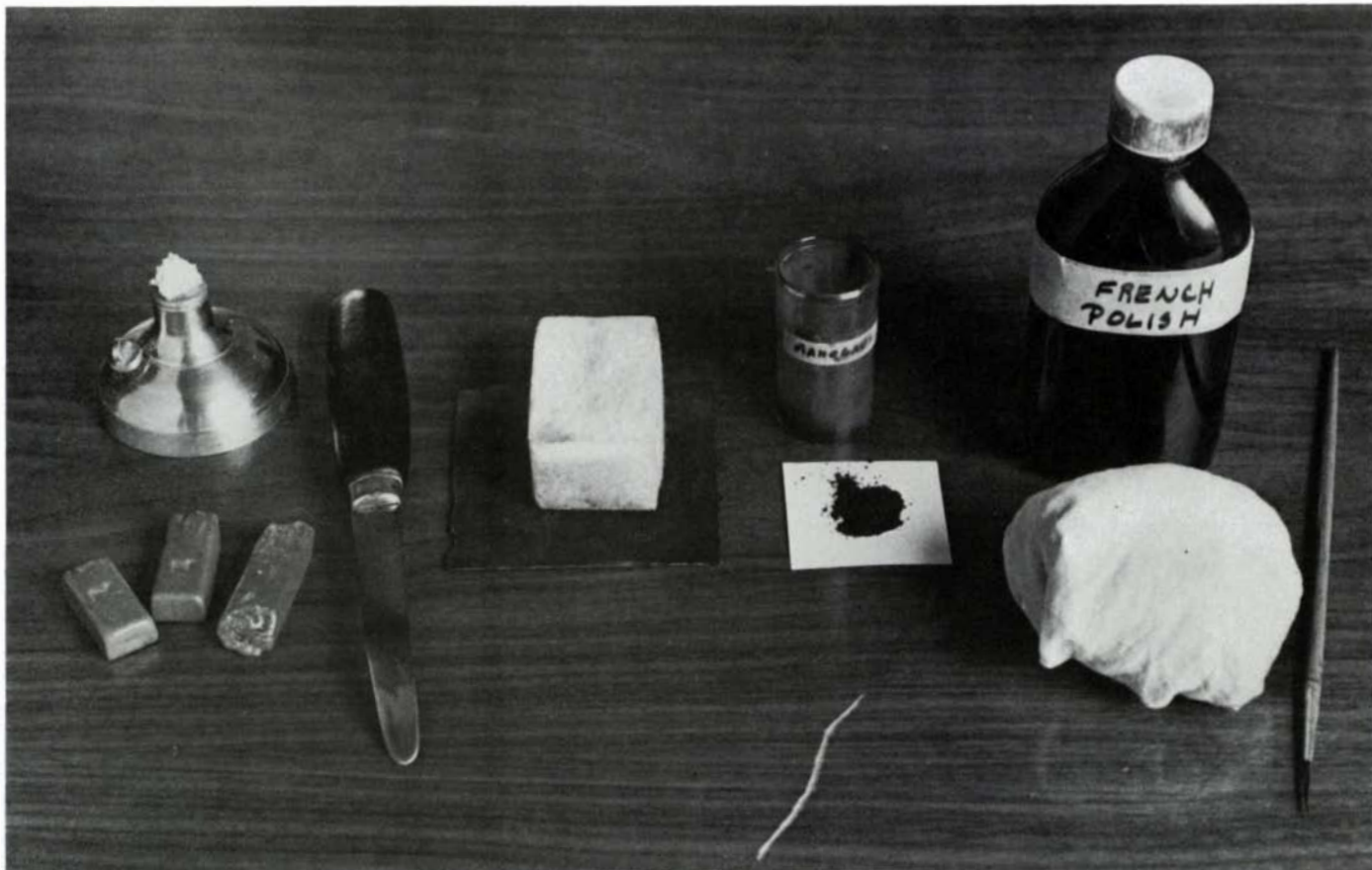
For repairing finishes you'll need (from left to right) an alcohol lamp, resin sticks, a burn-in knife, and a felt sanding block. To match colors, blending stain, French polish or padding lacquer, a cloth pad and a fine brush are used.
