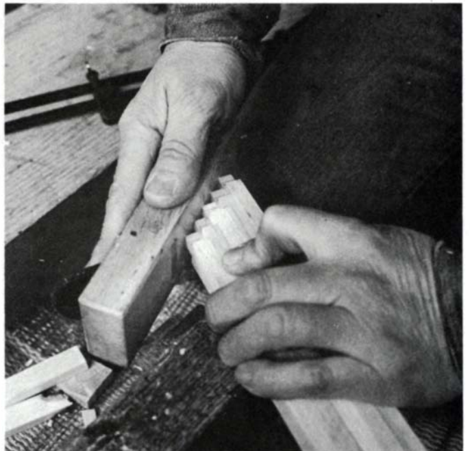
With the kumiko still clamped together, Odate makes their tenons. First he saws the shoulders, then breaks off the waste with a chisel pushed in from the end grain (top). The index finger on the bottom of the chisel acts as a stop to protect the shoulder. He cleans up the tenons by paring with the chisel across the grain (above). When all the tenons have been formed and their top and bottom corners chamfered with a few strokes of a plane, he unclamps the stack, fans out the kumiko and chamfers the other two corners (below).
