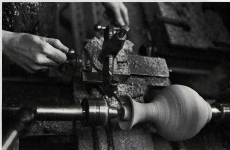
Holzapfel uses a diamond-point tool, top, to shape a cherry vase. Having become accustomed to the machinist's lathe, she finds it easy to trace a contour while reducing its diameter, a feat of considerable coordination with a compound tool rest. Above, she uses a left-hand cutter to shape a vase's flaring top. Cross slides and compounds are available for many woodturning lathes and old metal lathes of all sizes can be adapted for woodturning.
