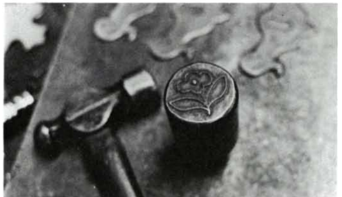
Jim Horton of Horton Brasses, is an expert in the hand-chasing of brass pulls. A drilled backplate is placed on a steel surface, top, and detail is stamped in the surface with a single hammer blow to a steel die. Horton uses dozens of stamps with various designs, as above. Below is a close-up of a flower-motif stamp.
