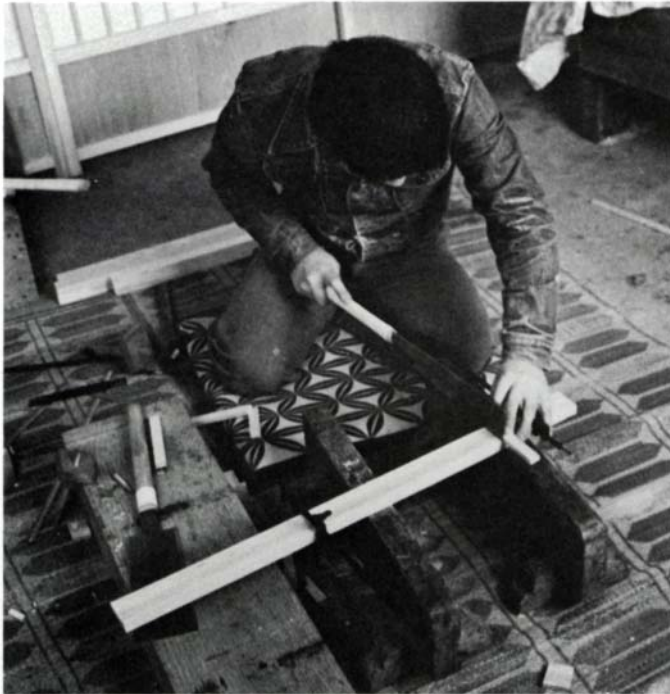
Odate clamps the kumiko (the thin strips that form the shoji grid) together in a stack and saws the notch shoulders a hair more than half-way through. A piece of scrap starts the saw correctly.
