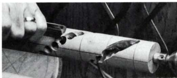
E After the drill press, it's back to carving by hand. The final shape of the hollow spiral is done with chisels, knives, rasps and sandpaper. Lathe-mounting allows the work to be positioned while carving.
