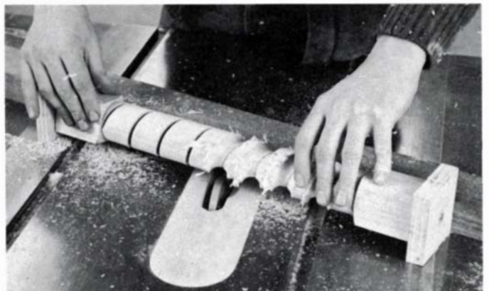
Dowel pin set in fence will guide kerfed cylinder past molding head (right). Cut must be deep because a second cut is not possible (below). Go slowly to minimize tear-out.
