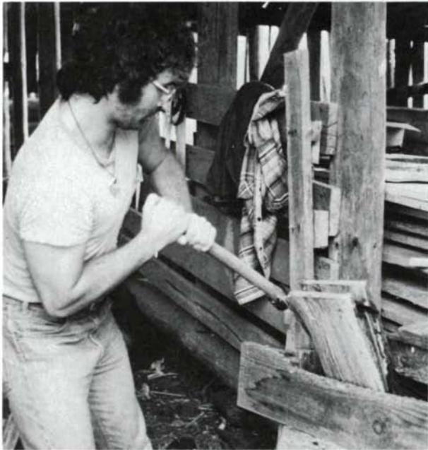
Top, Sawyer marks the end of a bolt for splitting with a froe. The finished rungs have to be \frac{7}{8} in. in diameter, and Sawyer lays out squares only \frac{1}{8} in. oversize. He controls splitting by arranging to split relatively equal portions (figure 2, p. 56), by splitting slowly, and if the split begins to run out, by exerting pressure against the heavier side of the split (figure 3, p. 56, and cover). Above, a student splits rung blanks in a small brake—two boards mounted like scissor blades to hold the work. By the end of the workshop's first day, we had shaved more than a hundred rungs, trying various styles of shaving horses and drawknives. The two horses, top right, are roughed out from thick slabs; the large stone holds them steady. At right, Sawyer loads the rungs into an oil-drum kiln.
