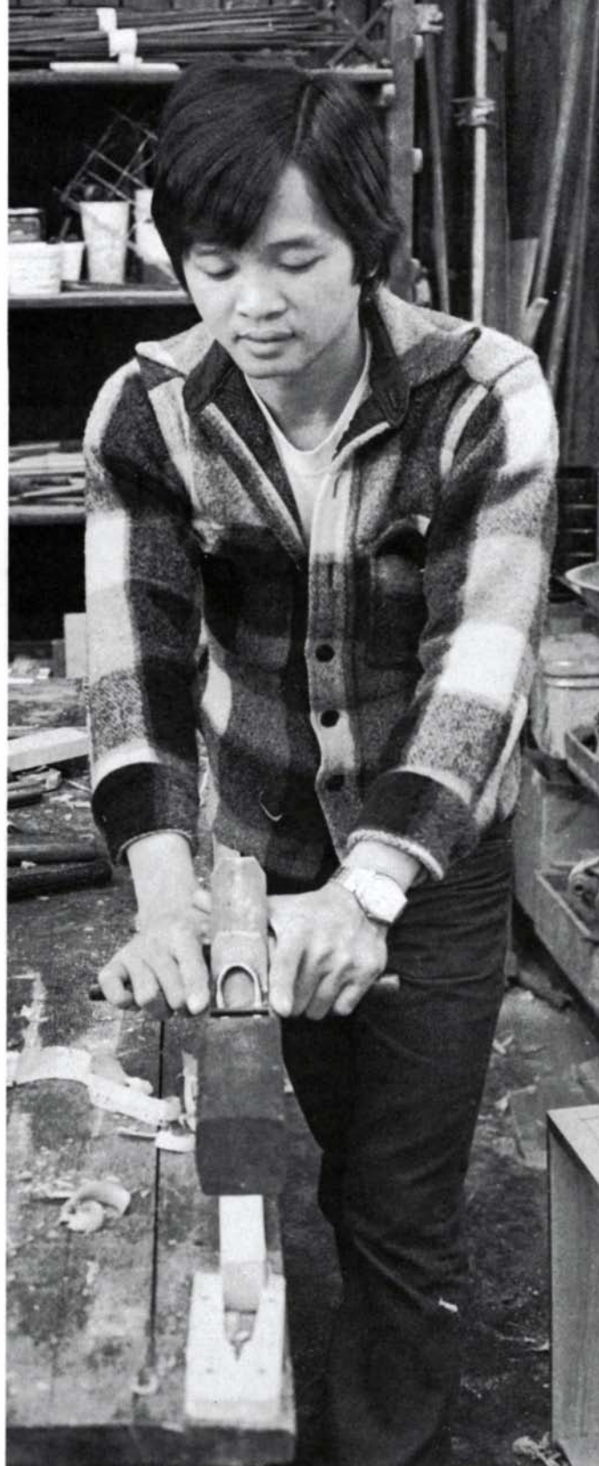
Grasping his homemade jack plane by the handles set behind its blade, Cong planes an edge. He controls the cut with his wrists, index fingers and thumbs.
