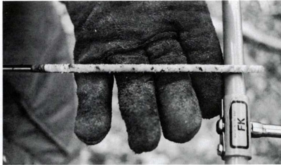
Short of felling trees and counting the annual rings, an increment borer, left, is the best way to tell the age of trees. The tool removes a small, fragile cylinder of wood, right. The rings aren't as easy to see as in a cut tree, and must be counted carefully.
