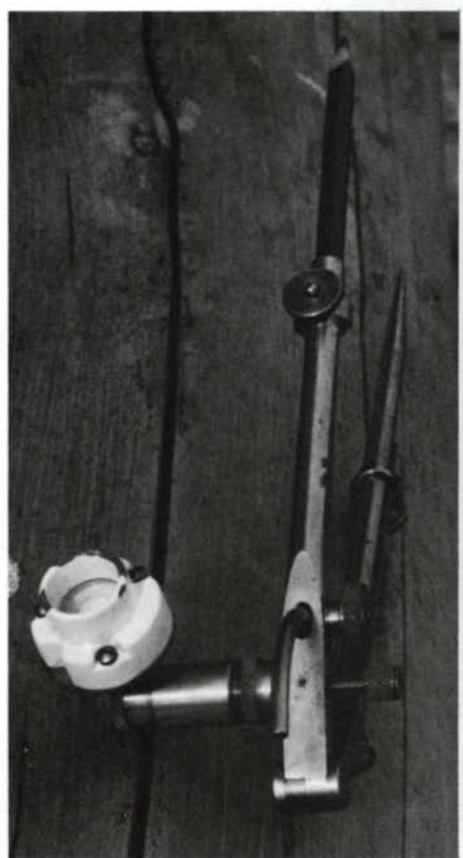
Author uses a ship auger with extensions to bore for the all-thread that secures the vertical web and brace logs, photo right. A pair of Starrett No. 85 dividers with a custom-made, adjustable target-bubble level, below, scribes the contour of one log onto the end of an adjoining log. The level helps keep the points of the divider plumb while scribing. Below right, Robinson has oriented the vertical web log horizontally to scribe its contour to the end of a brace log.
