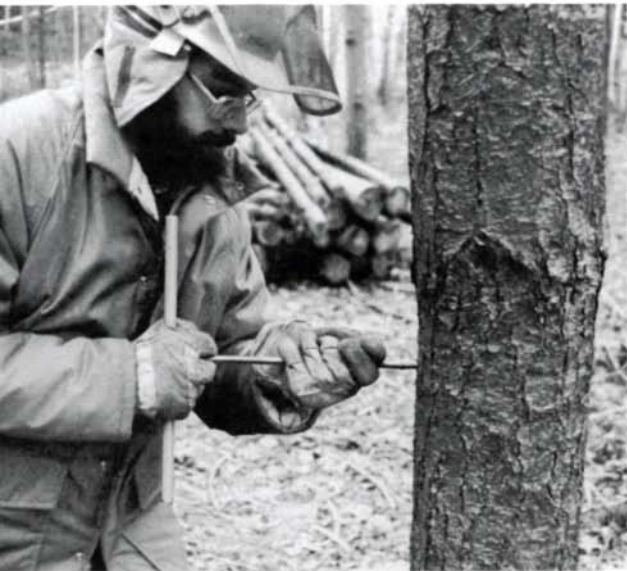
Short of felling trees and counting the annual rings, an increment borer, left, is the best way to tell the age of trees. The tool removes a small, fragile cylinder of wood, right. The rings aren't as easy to see as in a cut tree, and must be counted carefully.
