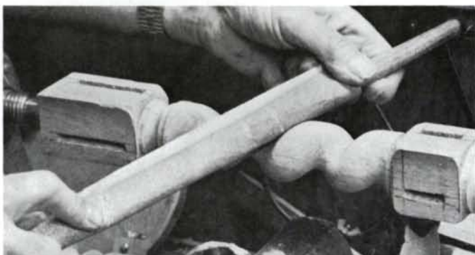
C After carving, use rasps and sandpaper to form the spiral in the shape you want. Here, sandpaper is wrapped around a rasp that acts as a sanding block to maintain the radius.
