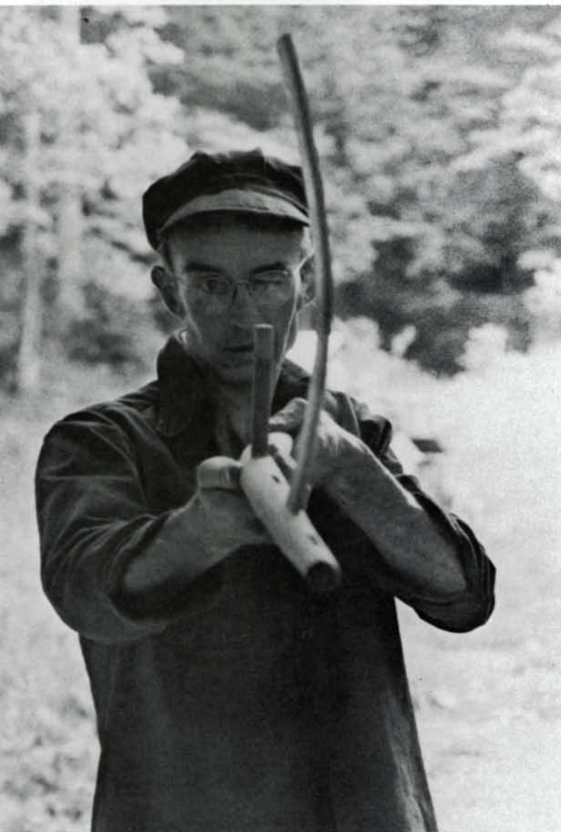
Sawyer produces as many as 50 ladderback chairs a year without using jigs. "In my power-tool phase," he said, "I made some very fancy jigs. But it turned out to be mindless. . . . And I'd be looking for them and fiddling with them, and they'd end up in the fire." So now Sawyer just clamps the posts to the bench, shims to "close enough" and guides his brace and bit with a T-bevel and his eye.
