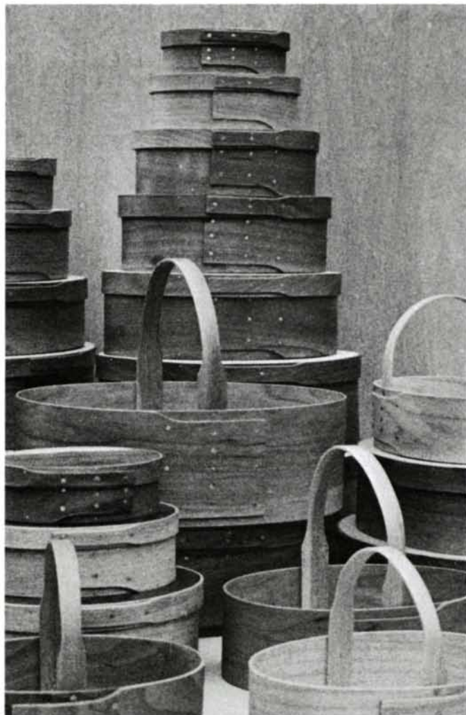
Author's Shaker-style oval boxes and carriers are steambent from various hardwoods, glued and nailed at the splice. Boxes nest one inside another. Below, rack of dowels inside steambox holds the stock, sawn and planed to about \frac{1}{8} in. thickness, on edge for a 15-minute soak in unpressurized steam.
