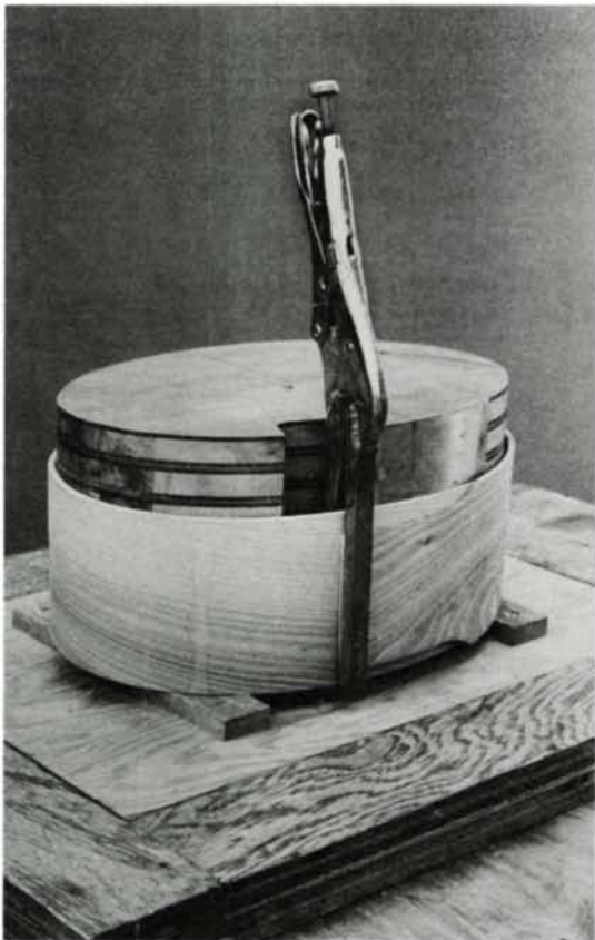
After steaming, box sides are wrapped around the bending form and clamped in place, above. The clamp shown here was made by welding two steel bars to the jaws of a Visegrip pliers. When the piece has cooled enough to retain its shape, the scarf joint is glued and minimally nailed, then clamped with C-clamps and clothespins, upper right, until the glue has dried. At right, author drives and clinches the remaining nails against an anvil made from 1½-in. galvanized pipe. Below, one of McFadden's boxes, with carved lid.
