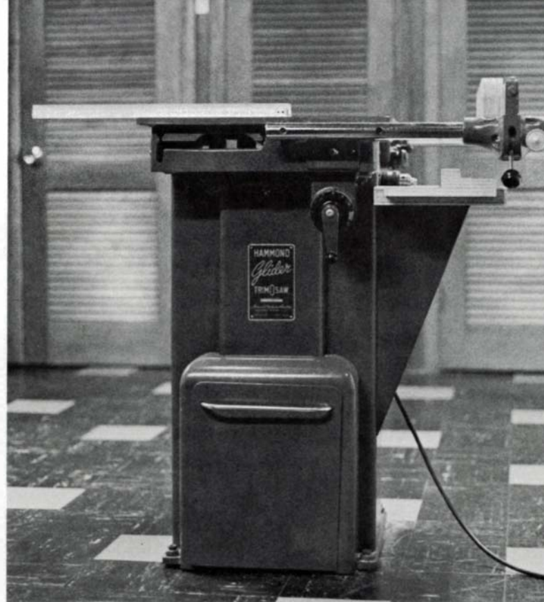
The Hammond Trim-O-Saw, originally used for cutting lead type in newspaper composing rooms, becomes an accurate woodworking machine for mortising and precise cutting.
