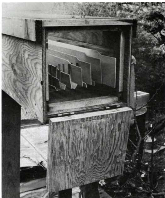
Author's Shaker-style oval boxes and carriers are steambent from various hardwoods, glued and nailed at the splice. Boxes nest one inside another. Below, rack of dowels inside steambox holds the stock, sawn and planed to about \frac{1}{8} in. thickness, on edge for a 15-minute soak in unpressurized steam.
