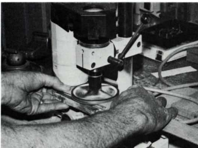
For final finishing, he chucks a sanding disc in his Unimat drill press and draws the stock between the disc and the milling table beneath.
