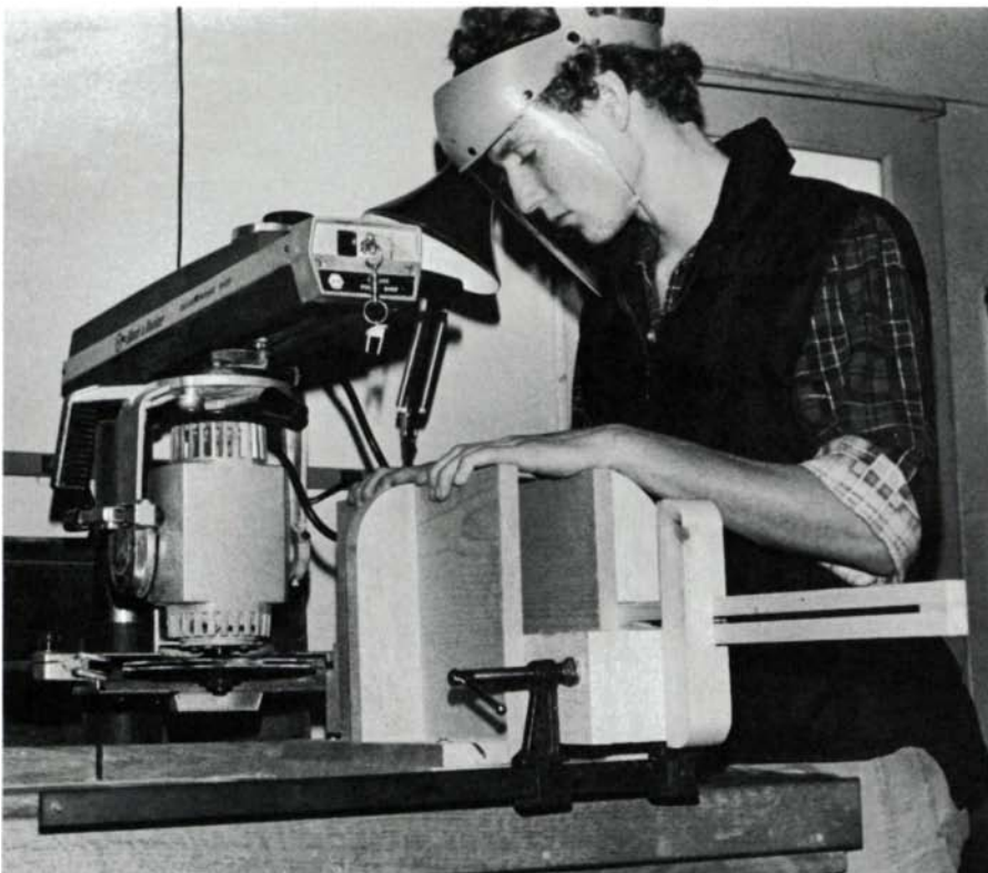
With the stock aligned and clamped together between the two fences on the sliding jig, the work is passed through the blade. The jig is guided by a bar that rides in a slot at the front of the table. The adjustable stop block is secured in place along the slotted rail and determines the depth of cut. Photos: Ken Mitchell.
