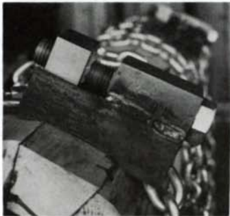
A jointing plane with metal fence, top left, is useful for correcting any irregularity in the joint interface. Leeke prefers the hand plane over his power jointer for this operation. For gluing and clamping the one-third sections into a full cylinder, Leeke devised and fabricated chain clamps like the one at left from ½-in. chain, steel plate, solid mild steel (for the tapped hook block) and a 1-in. bolt for tightening the chain. The clamp heads are staggered around the column, above, to help equalize the pressure and keep the column's diameter from being squashed into an ellipse.
