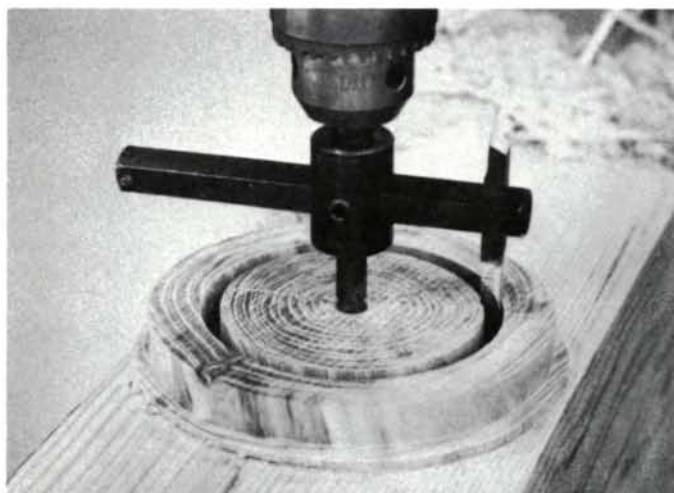
2. Adjustable circle cutter defines inner circumference of rosette; outer circumference has already been cut. If either one of these cuts produces tear-out, try regrinding the cutter to the opposite angle. Slab has been glued to a large, square beam and is thick enough for two rosettes, about the depth limit of the circle cutter.
