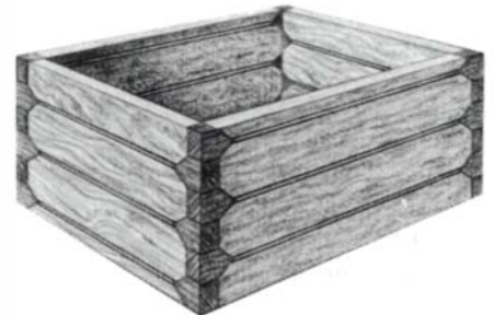
semble using plywood splines. A veneer strip can be added between the panels, as shown in the drawing at right, to visually link the corners of the carcass.
