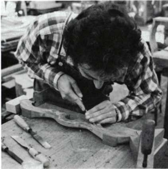
Carl Mesrobian carves the crest rail for a Chippendale arm chair. Using notched clamping blocks in conjunction with vise dog and handscrew gives him free access to the entire length of the rail.
