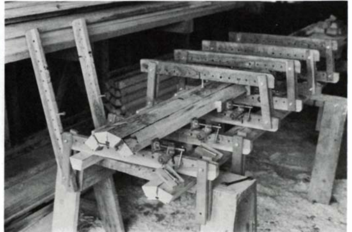
Pairs of splined staves are glued up using notched blocks and clamping heads (available from Woodcraft Supply Corp., 313 Montvale Ave., Woburn, Mass. 01888). Using two sets of clamps per bar makes handling easier and gluing faster.
