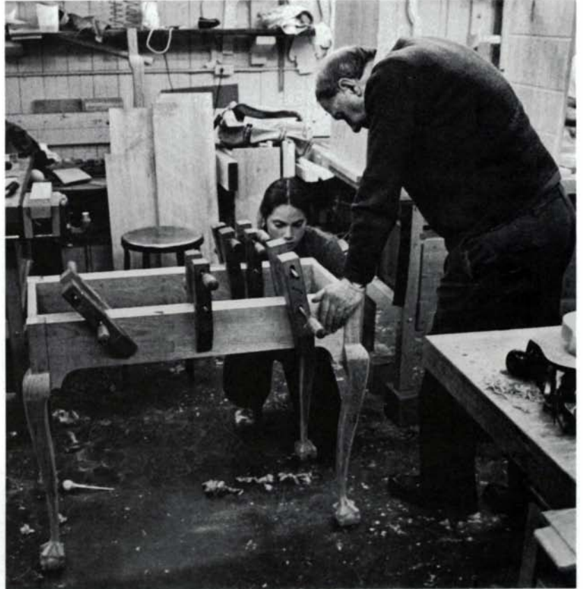
To signal the end of their novitiates, students construct tool chests like the one at left, little tours de force of dovetailed casework. Made to prescribed dimensions, the chests fit neatly out of the way beneath workbenches. Above, senior instructor George Fullerton eyes the joinery and checks the progress of a more advanced project, Catherine McGarty's butternut drop-leaf table. Boards leaning against bench in rear will be glued up to make the oval top.
