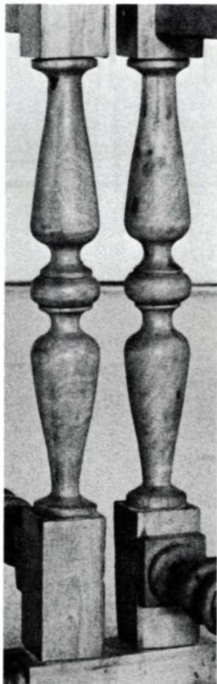
Graceful symmetry of Yorgey's table legs in dogwood belies its lathe-less origins.
