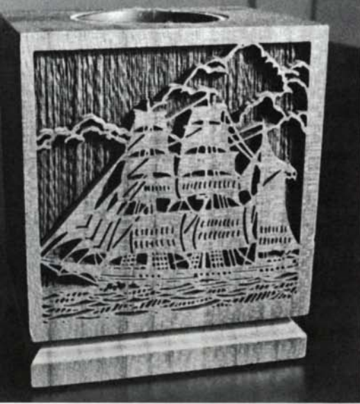
Laser engraving produces fine detail, recessed background. Left, paper-clip holder by Lasercraft. Right, Turntables move work under laser beam.
