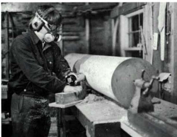
Routing from headstock to tailstock, with the router carriage canted at 55°, causes the cove-cutting bit to push itself away from the cut instead of digging into it. At left and center, the staved shaft is being roughed into round in a single light pass. At right, the completed shaft is sanded using a belt sander turned upside down and slid along the column as it turns.
