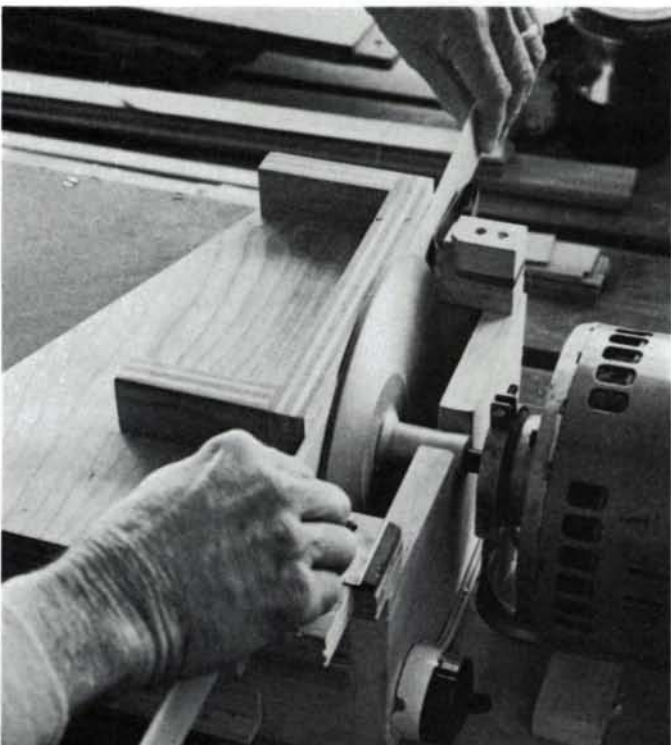
A better method for thickening stock employs a tapered sanding disc mounted on a direct-drive mandrel opposite an adjustable fence. This device will give accurate results, thickening 1½-in. wide planks to tolerances of 0.003 in. edge to edge.
