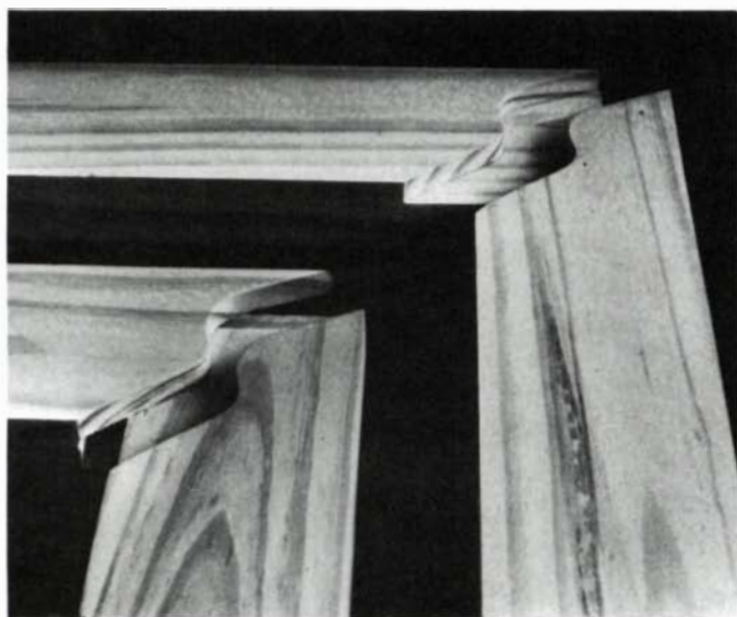
Reverse curve defines joining shoulders of rail and stile, left. A variation of the technique can produce a curved half-lap joint, right.
