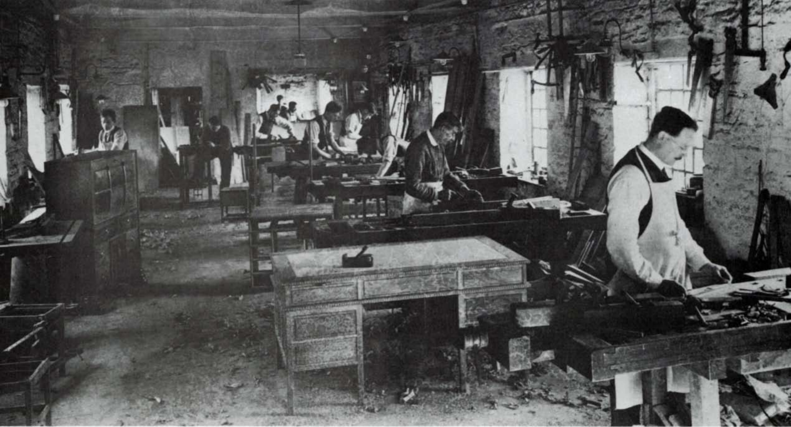
Unlike Gimson and the Barnsley brothers, Peter Waals was not averse to the use of woodworking machinery, though even in his shop at Chalford shown here (c. 1925), most of the work was done with traditional hand-tools. Note the treadle-powered table saw in use in the rear of the shop. Edwardian cabinetmakers such as these were perhaps the finest in history. Photo: Graham Light, Abbey Studios.
