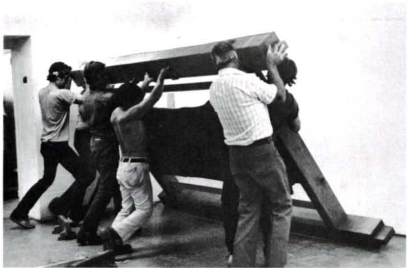
Odate (shirtless) commands one of the top members into place, above. More help was required to upright the 3-in. thick white oak flitch mounted in mortise-and-tenon timber frame, right. Screen frame, center right, was drawn to flitch frame with clamps.
