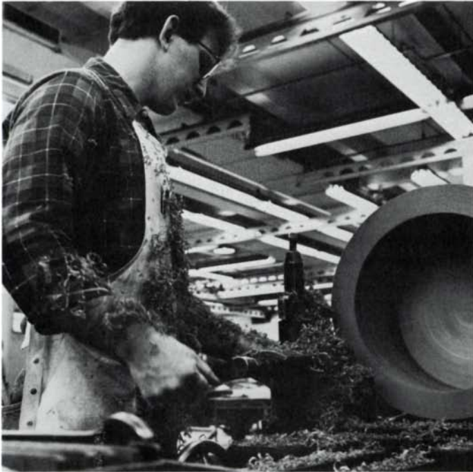
Patternmakers use wood lathes with screw-driven crossfeed tool posts, like those on metalworking lathes, to achieve maximum accuracy when turning. Pattern being turned here is made from stacked, segmented rings, glued one atop another.
