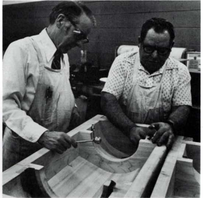
Patternmakers apply leather fillets to a completed core box. Fillets create radii at sharp junctures of a casting's elements, adding considerably to the strength of the metal at these points and helping to prevent cracked castings.
