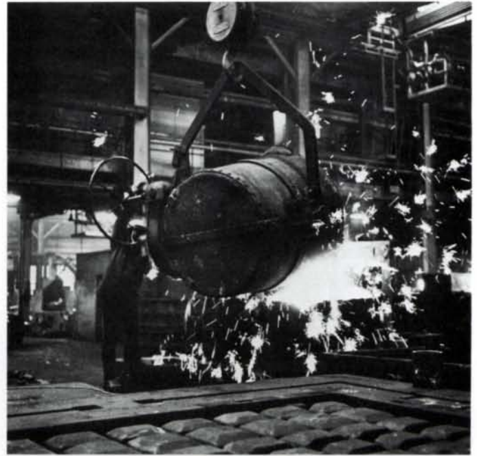
Foundryman pours a medium-size casting. Encased in a metal flask, the drag mold in the foreground is filled with cores that will form the internal ribwork of a machine frame.
