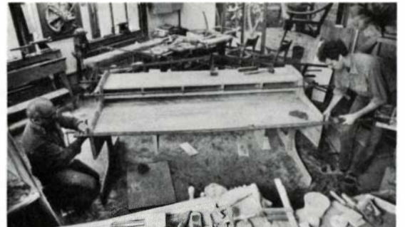
Assistant Jerry Marcotte helps position an 8-ft. bar clamp on a brown oak desk.
