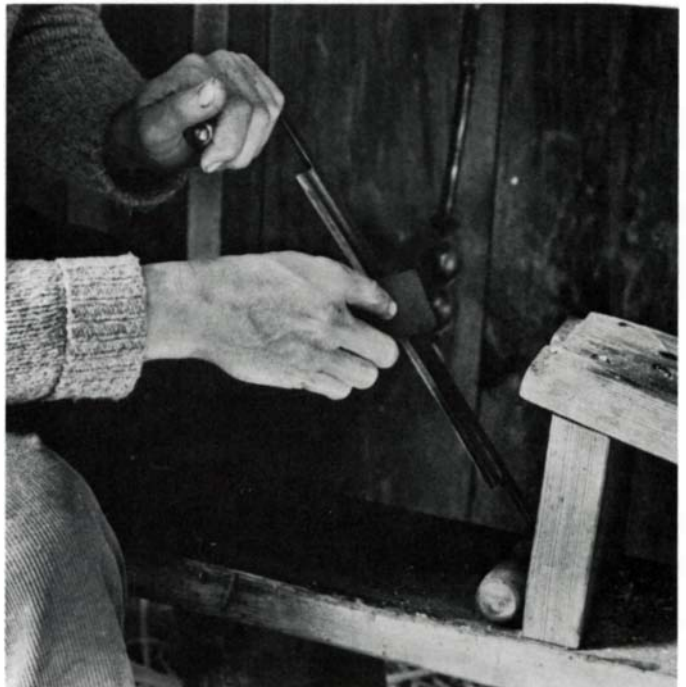
Drawknife and shaving horse offer an ideal combination of direct shaping and quick, sure gripping of green stock.
