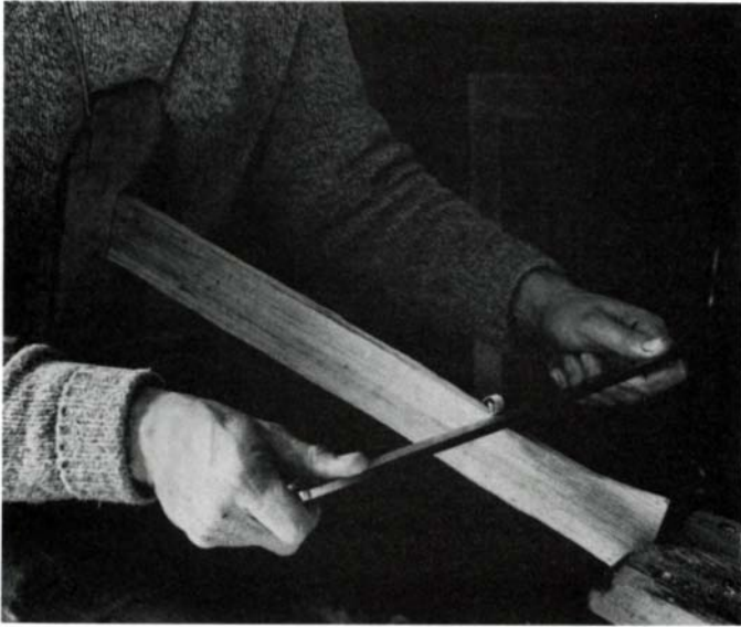
Pieces that do not fit under the shaving-horse head can be held between the end of the shaving horse, in a notch or rabbet, and a roughsawn breast bib. Note that cuts do not start on the end grain; the waste at the far end of the stick will be removed after the stick is turned end for end.
