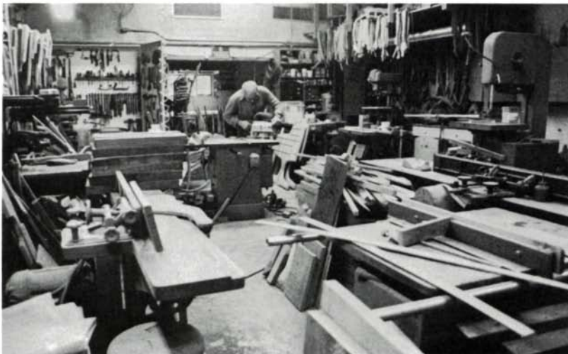
The 1,000-sq. ft. machine room is the largest of the three rooms that make up Maloof's shop. He's got two table saws, an 18-in. planer, two jointers (16 in. and 8 in.), a 20-in. and a 14-in. bandsaw, a 1-in. shaper, two cut-off saws, a hollow-chisel mortiser, a drill press, a horizontal-boring machine, two disc sanders and three lathes. Maloof's tool cabinet, right, is well stocked with routers, rasps and files.
