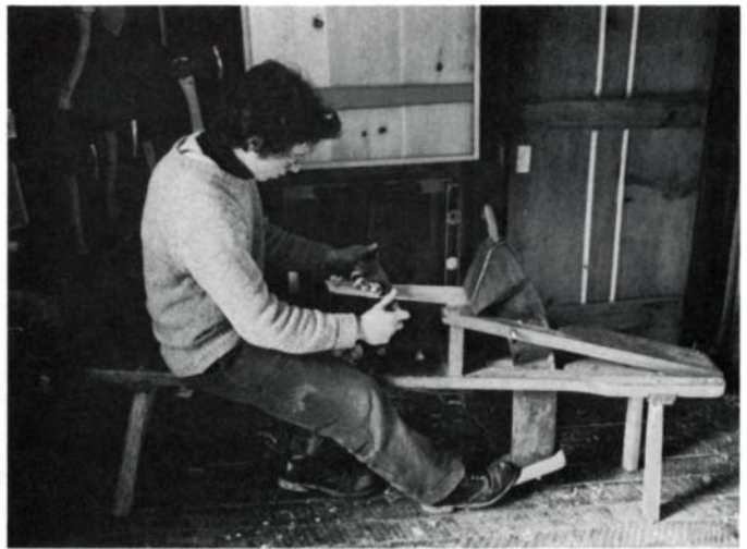
Drawknife and shaving horse offer an ideal combination of direct shaping and quick, sure gripping of green stock.
