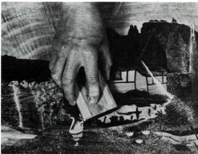
Before the top coats are applied, varnish, painted in with a small brush, fills deep scratches and gaps in veneer joints. The 18-in. by 20-in. picture, by the author, includes holly swans in a black beam pond under an aspen sky.
