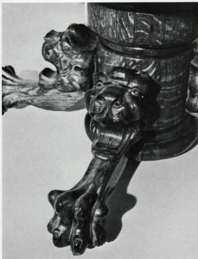
This quartersawn oak table was made toward the end of the American oak period, probably in the 1920s. Reproducing it involves a challenging range of procedures. The lions' heads, arms and paws are carved from laminated stock. The pedestal is coopered and turned. And the top, aprons and parts of the pedestal are veneered. Scale drawings appear on the following pages.
