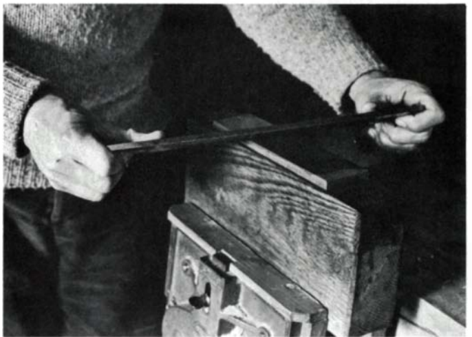
Two methods of sharpening drawknives. A Swiss cooper teaches supporting the drawknife on the shaving horse, center, and rubbing a handstone first over the bevel, then over the flat face, moving it up and down the length in small circles. A Swedish woodworking instructor teaches mounting the stone in a block of wood held in a vise, above. The drawknife is drawn diagonally over the stone, toward you and toward your right, so the entire length of the blade is whetted in each stroke.
