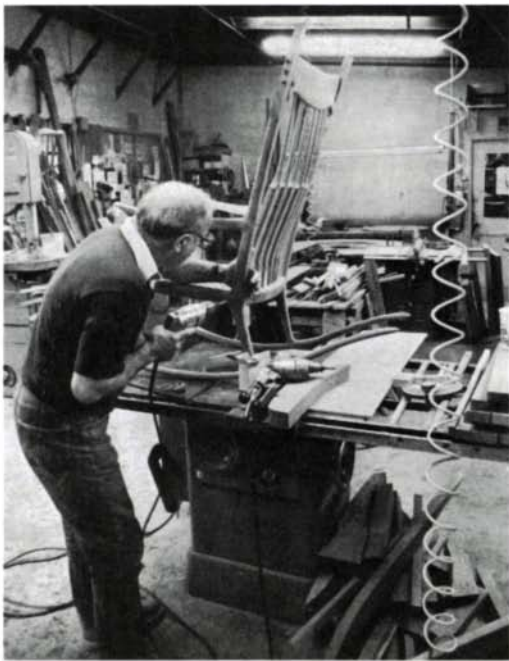
Custom rocking chairs, now $2,500, remain Maloof's most popular design—he's built more than 100 of them and has 60 on order now. Working atop his table saw, left, Maloof drives 4-in. sheet-metal screws into the glued leg joint at opposing angles, then plugs with ebony.
