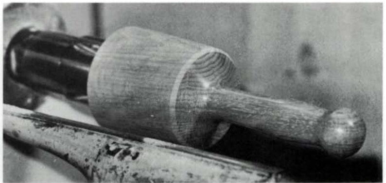
With wooden pot chuck, left, screw chuck can turn the tiniest of goblets. Alone it grips larger stock for vibration-free turning along the full length of mallet, right. Mushroom boxes with putumuju tops, below, evidence more of the versatility and precision possible.
