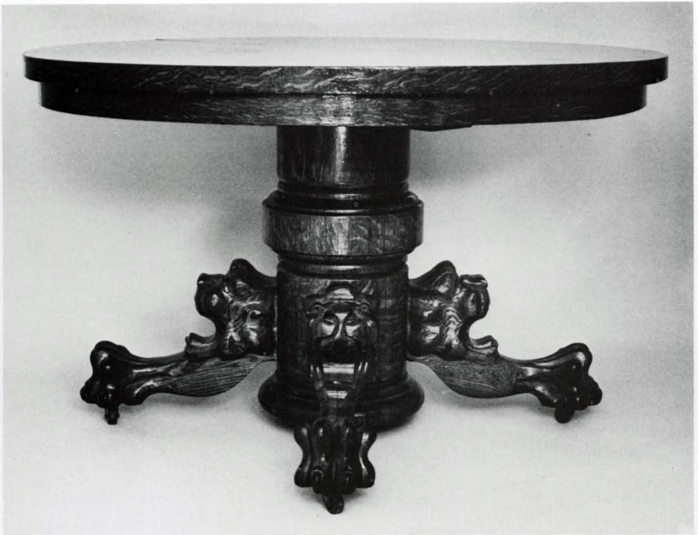
This quartersawn oak table was made toward the end of the American oak period, probably in the 1920s. Reproducing it involves a challenging range of procedures. The lions' heads, arms and paws are carved from laminated stock. The pedestal is coopered and turned. And the top, aprons and parts of the pedestal are veneered. Scale drawings appear on the following pages.
