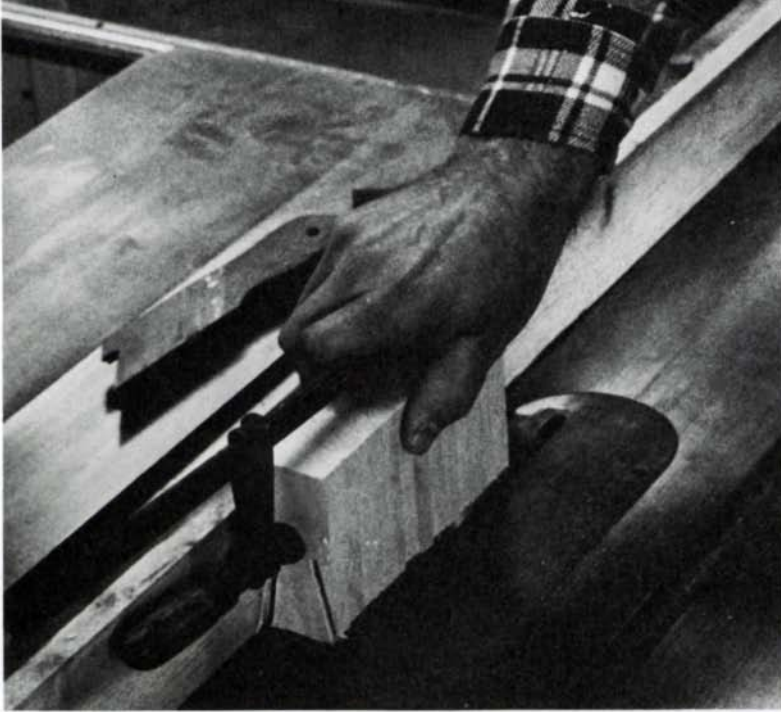
Cutting a dozen keys at one time on his table saw, Klausz uses a bar clamp to help grip the stock. This is a dangerous cut. Do it safely by making sure that the blade clears the clamp jaws and that the thumb is placed high on the workpiece.
