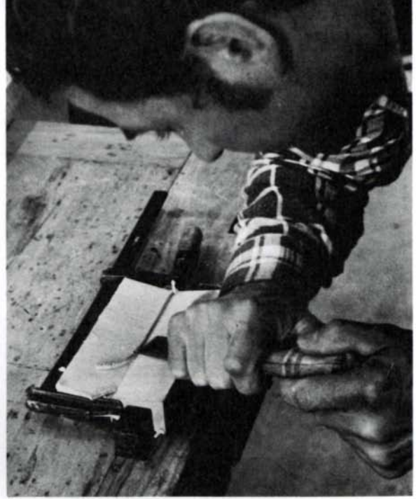
To clean up the unsawn center portion of the stock, Klausz holds the chisel askew and slices at the waste, moving from left to right.
